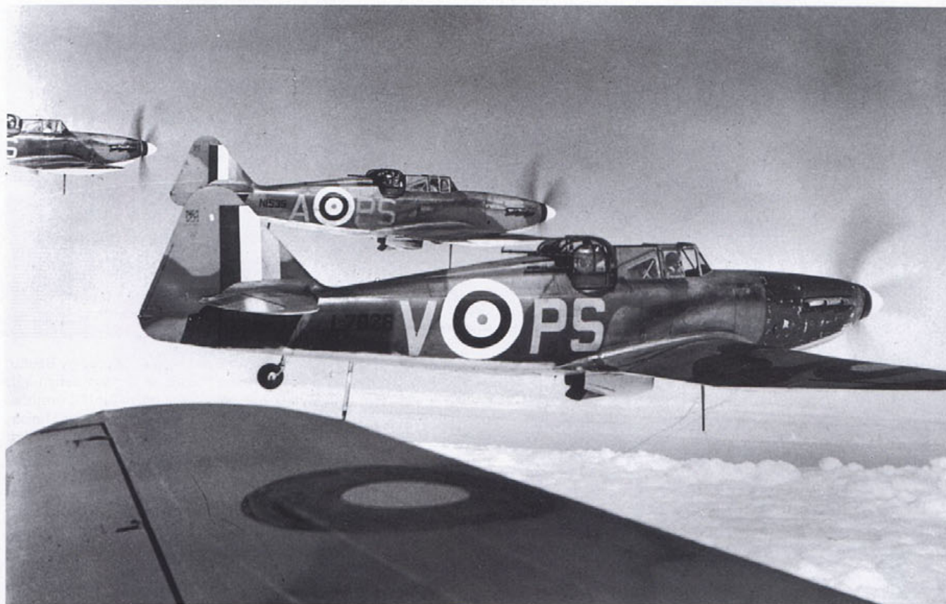
No.264 Squadron's Defiants in formation. This picture shows the extent of the under-fuselage radio mast so positioned that the gunner did not shoot it off. (IWM)
