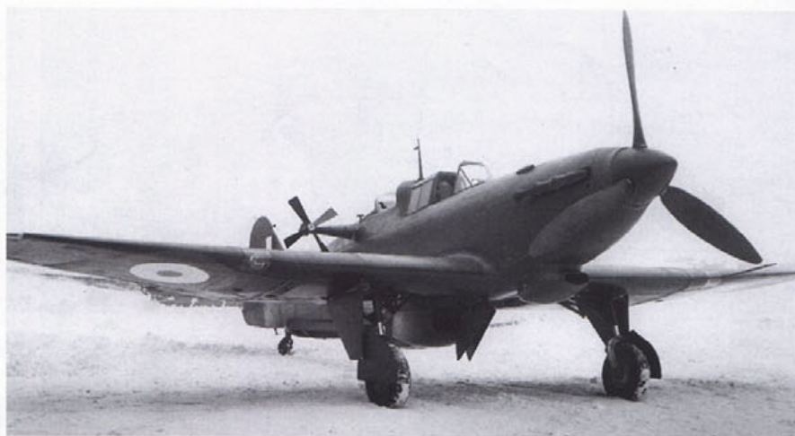
Two views of an early conversion to target towing standard of an all-black night fighter Defiant. The serial or previous squadron is not known but it is interesting to note the considerable changes to the aircraft's outline that took place. The turret has been replaced by an observer's position, a four-bladed wind driven unit was placed on the starboard side of the fuselage and the targets placed in a container under the rear fuselage. The deeper radiator of the Mk.II should be noted and the radio aerial moved to the top of fuselage position behind the pilot.
