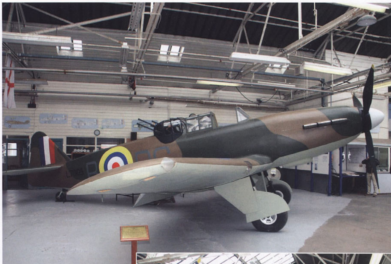
Above and right: Rebuilt from the remains of a Boulton Paul Defiant turret and other parts, the Boulton Paul Association members constructed this full scale replica using plastics, wood and metal over a period of four years. The aircraft which has been serialised L7005 and painted in the colours of No. 264 Squadron during the Battle of Britain, was unveiled to the public for the first time at the Boulton Paul Association's museum, near Wolverhampton, on 15 September 2002. (Mark Ansell)
