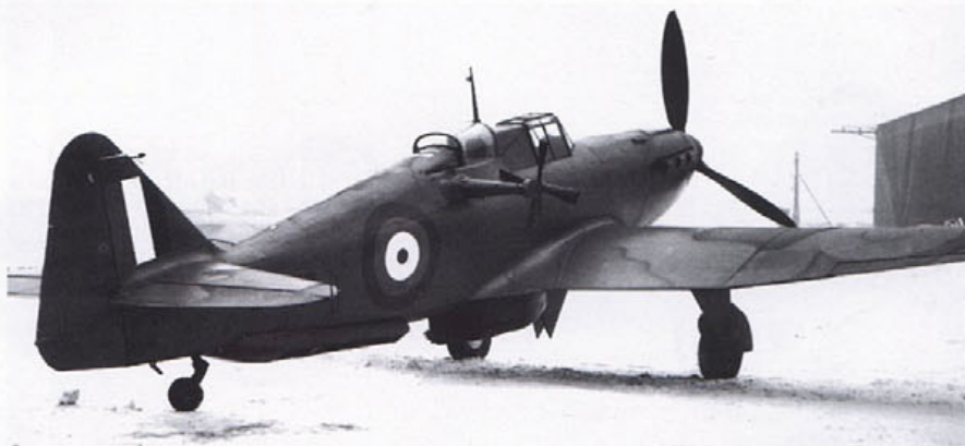
Two views of an early conversion to target towing standard of an all-black night fighter Defiant. The serial or previous squadron is not known but it is interesting to note the considerable changes to the aircraft's outline that took place. The turret has been replaced by an observer's position, a four-bladed wind driven unit was placed on the starboard side of the fuselage and the targets placed in a container under the rear fuselage. The deeper radiator of the Mk.II should be noted and the radio aerial moved to the top of fuselage position behind the pilot.
