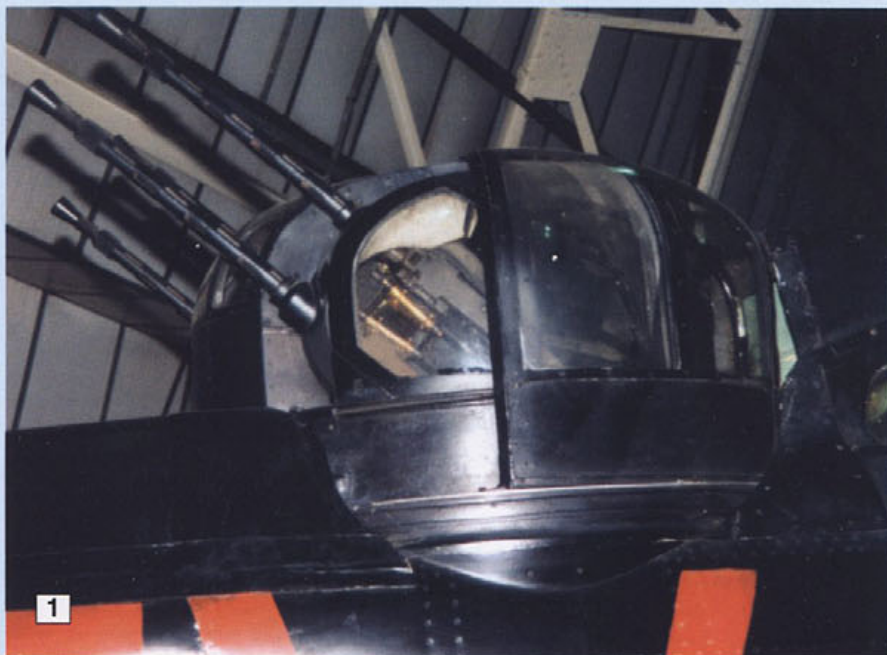
1. The Boulton Paul gun turret fitted to the Defiant had four .303 Browning machine guns and could fire at most angles but not forward over the aircraft's nose. 2. Defiant's tail unit and tail wheel. Construction was of simple frames and metal skinning making it easy to construct and repair.
