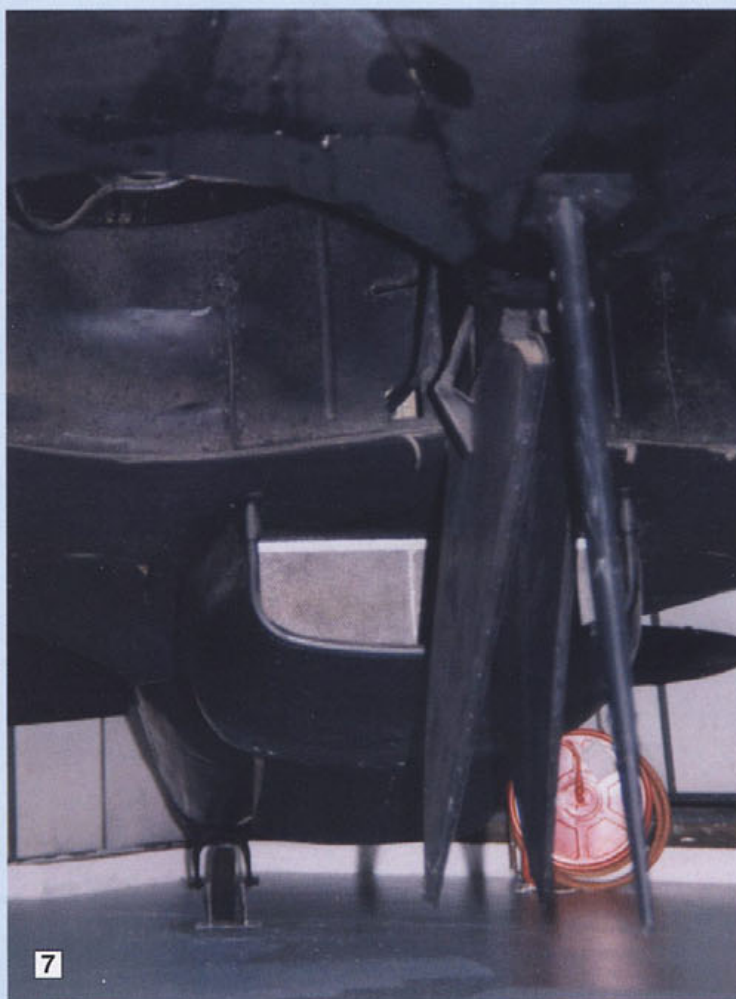
5. The underside of the Defiant's nose. 6. Left hand undercarriage leg and wheel. 7. Under fuselage showing the radiator. Note that the rear radio aerial is retracted but that it is offset to the right hand side of the fuselage. 8. The landing light in the starboard wing. A similar light was fitted in the port wing. 9. The size and shape of the roundel and the colour of the codes. Some doubt has been expressed that N1671 in the RAF Museum should have been coded EW:W and not EW:P as shown. 10. The Defiant's cockpit cover slid backwards to allow the occupant to get in or out. The turret had to be swung at 45 degrees to allow entry and exit. 11. The Defiant's nose showing the ejector exhausts
