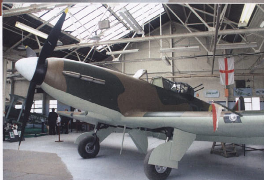
Above and right: Rebuilt from the remains of a Boulton Paul Defiant turret and other parts, the Boulton Paul Association members constructed this full scale replica using plastics, wood and metal over a period of four years. The aircraft which has been serialised L7005 and painted in the colours of No. 264 Squadron during the Battle of Britain, was unveiled to the public for the first time at the Boulton Paul Association's museum, near Wolverhampton, on 15 September 2002. (Mark Ansell)
