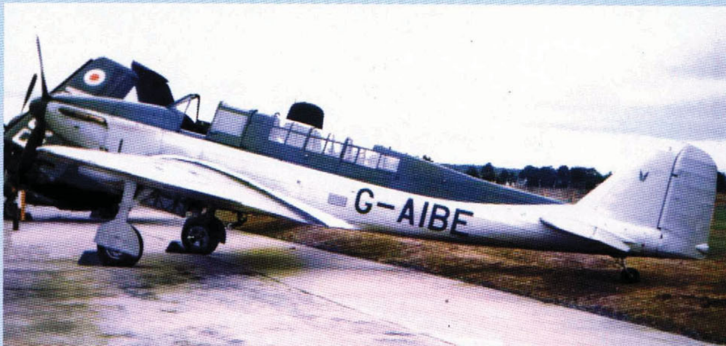
Above: The first production Fulmar Mk.I N1854 was civil registered as G-AIBE after the war and used by Fairey as a two passenger communications aircraft. It was converted to a Mk.II by the change of engine to a Merlin 30. The aircraft was returned to the Fleet Air Arm as N1854 and although in a non-flying condition is now on display at the FAA Museum, Yeovilton. (via Ray Sturtivant)
