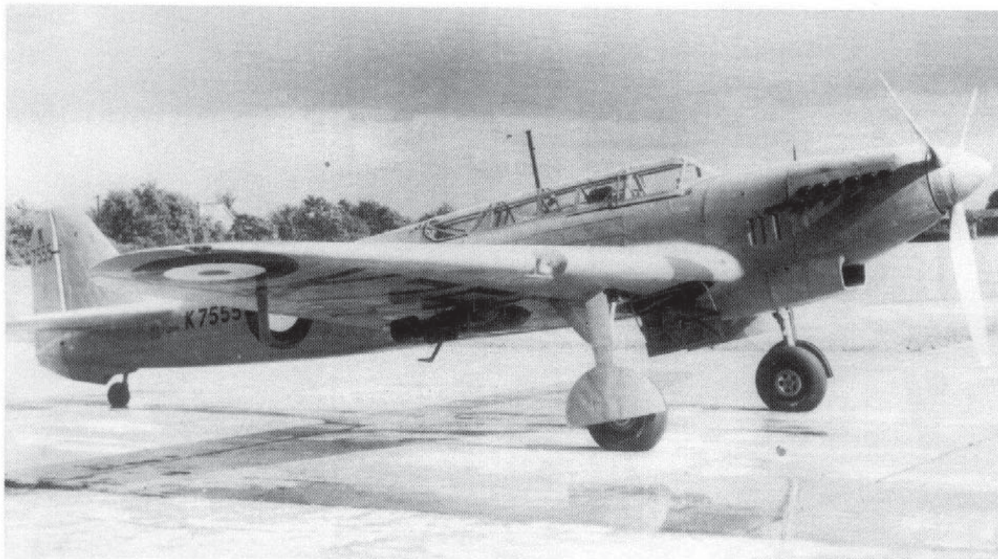
Fairey P4/34 K7555 seen at Heston aerodrome shortly after rollout in April 1937. It was powered by a 1,030 hp Rolls Royce Merlin F in its initial form which was later changed to a Merlin VIII. Because it was stressed for dive bombing and had a long range it was an ideal choice as a Fleet fighter to replace the Skua. (MAP)
