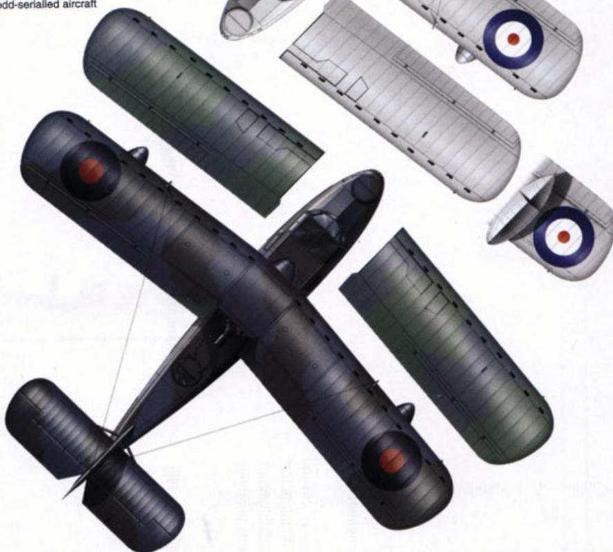
Below: Position and size of markings on shadow-shaded camouflaged aircraft; 'B' pattern was usually applied to odd-serialled aircraft
