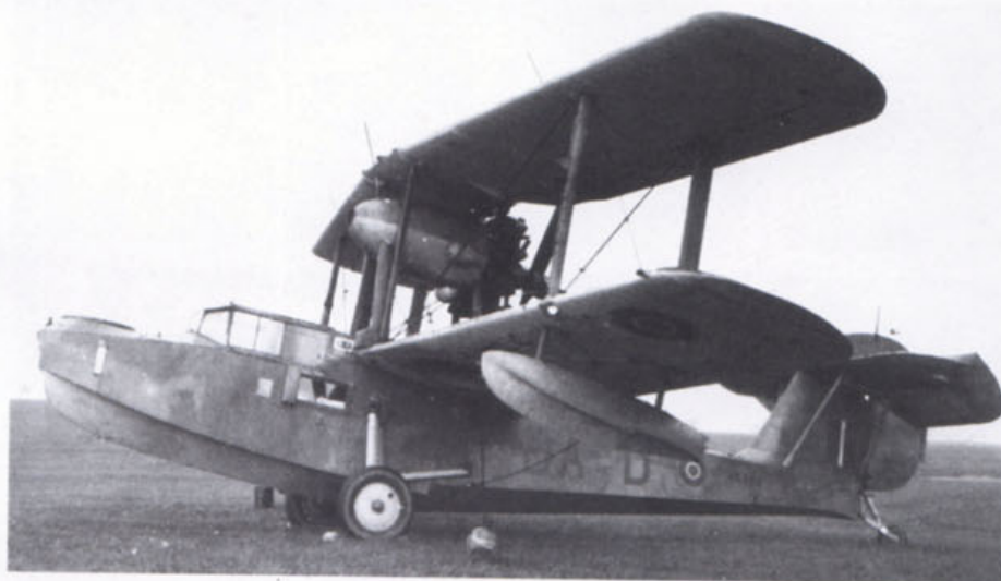
Above: A slightly dodgy cross wind landing for this Walrus from 1700 Squadron landing on the deck of HMS Ameer on 8 July 1945 after having rescued a downed Hellcat pilot from 200 yards off the Japanese held coast. (via R.L.Ward) Below: Walrus II HD908:BA-D of 277 air sea rescue Squadron when based at RAF Digby in 1944. Note the tail wheel instead of a water rudder (via Ray Sturtivant)
