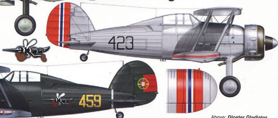
Above: Gloster Gladiator Mk.I, 423 , Royal Norwegian Air Force, 9 April 1940. Standard 'silver' scheme. Bands in the same colours as rudder are repeated above top wings and below bottom wings; codes in black
