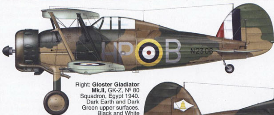
Gloster Gladiator Mk.II, N2306:HP-B, N° 247 Squadron, 1940. Shadow-shaded top surfaces in Dark Earth and Dark Green with Light Earth and Light Green on top of lower wings, lower half of fuselage sides and rudder. Black spinner and Sky undersides. Grey codes and large fin flash in Red, White and Blue. 'B' type markings above top wings
