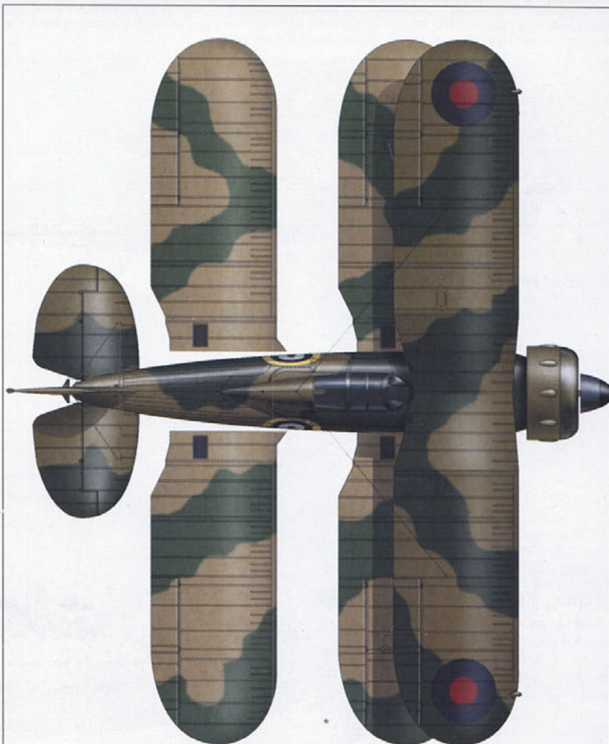
Four-colour upper surface pattern for Gloster Gladiators. Upper surfaces of top wings, elevators and top fuselage decking in Dark Earth and Dark Green; upper surfaces of lower wings and lower half of fuselage sides in Light Earth and Light Green. 'B' type roundels are 36ins diameter (with 16ins diameter central red sector)
