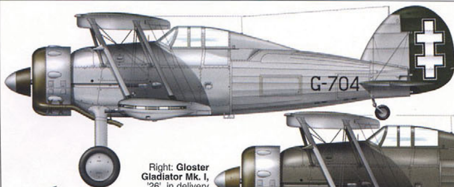
Gloster Gladiator Mk.I, G-704 , Lithuanian Air Force, 1939. 'Silver' scheme; Dark Green top surfaces of wings and elevator. National marking over a Dark Green base on rudder and below wings; normal above wings
