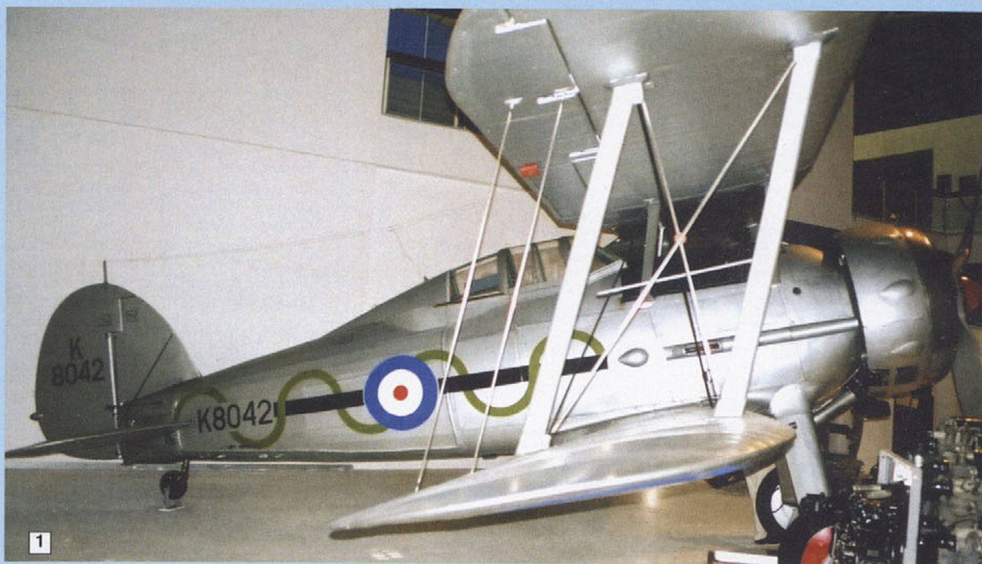
1. General arrangement view of the RAF Museum's Gladiator K8042. 2. Starboard wing .303 machine gun and housing. 3. View of the tail unit, bracing and control wires. 4. Port fuselage .303 machine gun housing and blast shield. 5. The interplane struts, bracing wires and the cockpit windscreen. The front part of the fuselage is all metal, painted Aluminium.
