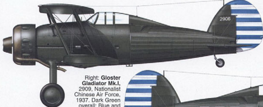
Gloster Gladiator Mk.I, 2906, Nationalist Chinese Air Force, 1937. Dark Green overall; Blue and White striped rudder; national markings above port top wing and below starboard lower wing only
