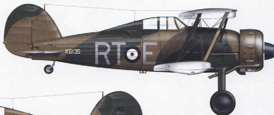
Below: Gloster Gladiator Mk.I, K6135:RT-E, N° 112 Squadron, 1940. Matt Dark Earth and Dark Green upper surfaces. White undersides of starboard wings and tailplane; Night undersides of fuselage, port wings and tailplane
