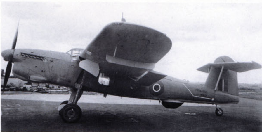
Above: This Barracuda of the British Pacific Fleet shows how small an area it could be folded into for deck handling and hangerage space. Below: Barracuda TR.III MD837 in August 1944 still with a three-blade propeller and the radar scanner under the rear fuselage. The white line is the revised route for the dinghy lanyard. (via Tony Buttler)
