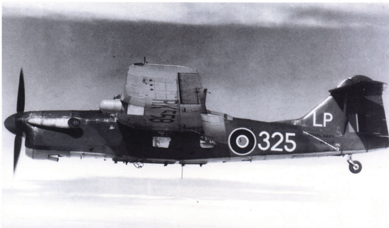
Above: Barracuda TR.V RK558 325:LP of 783 Squadron based at Lee-on-Solent during 1948. ASH nacelle is under the port wing, as is the aircraft serial number – but no roundel. The extended fin area is shown to good effect in this picture. (via Ray Sturtivant)
