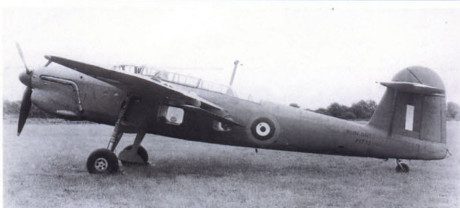
Above: The second prototype Barracuda P1770 which was manufactured with the revised tailplane layout and first flew on 29 June 1941. In all other respects it was the same as P1767. It was allocated to the TRE at Defford where it served from 1942 to 1945 on ASV Mk.II development. (Ian Huntley) Below: Barracuda I P9655 was built at Fairey's Heaton Chapel works in Stockport. Aircraft were moved to Ringway for final assembly and test flying. This photograph was taken in October 1942 and shows the wing fences and torpedo crutches. (Authors collection)
