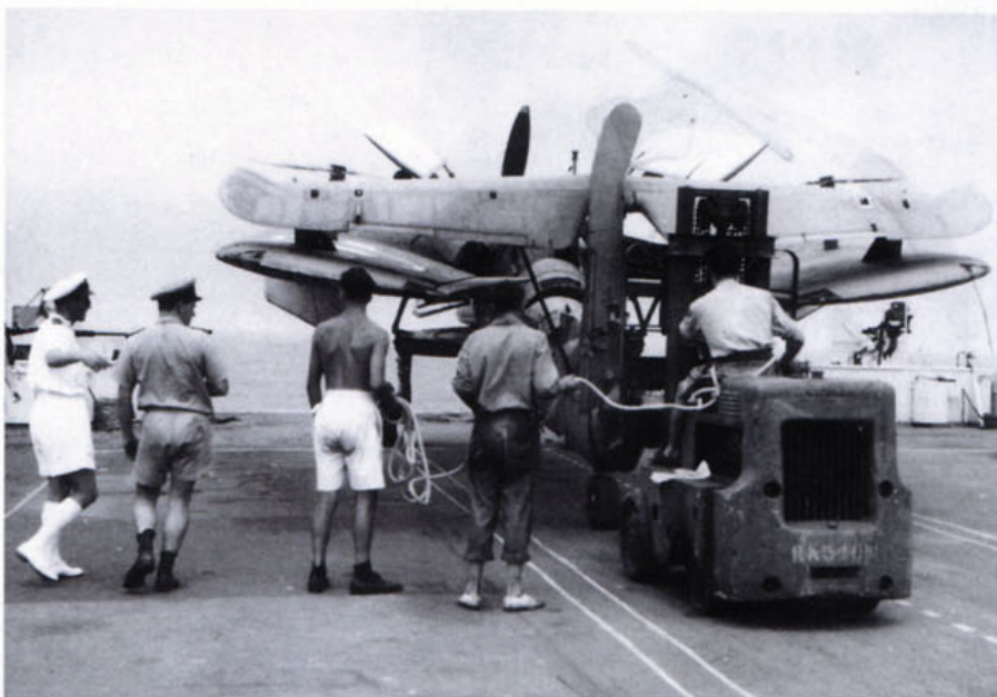
Above: This Barracuda of the British Pacific Fleet shows how small an area it could be folded into for deck handling and hangerage space. Below: Barracuda TR.III MD837 in August 1944 still with a three-blade propeller and the radar scanner under the rear fuselage. The white line is the revised route for the dinghy lanyard. (via Tony Buttler)
