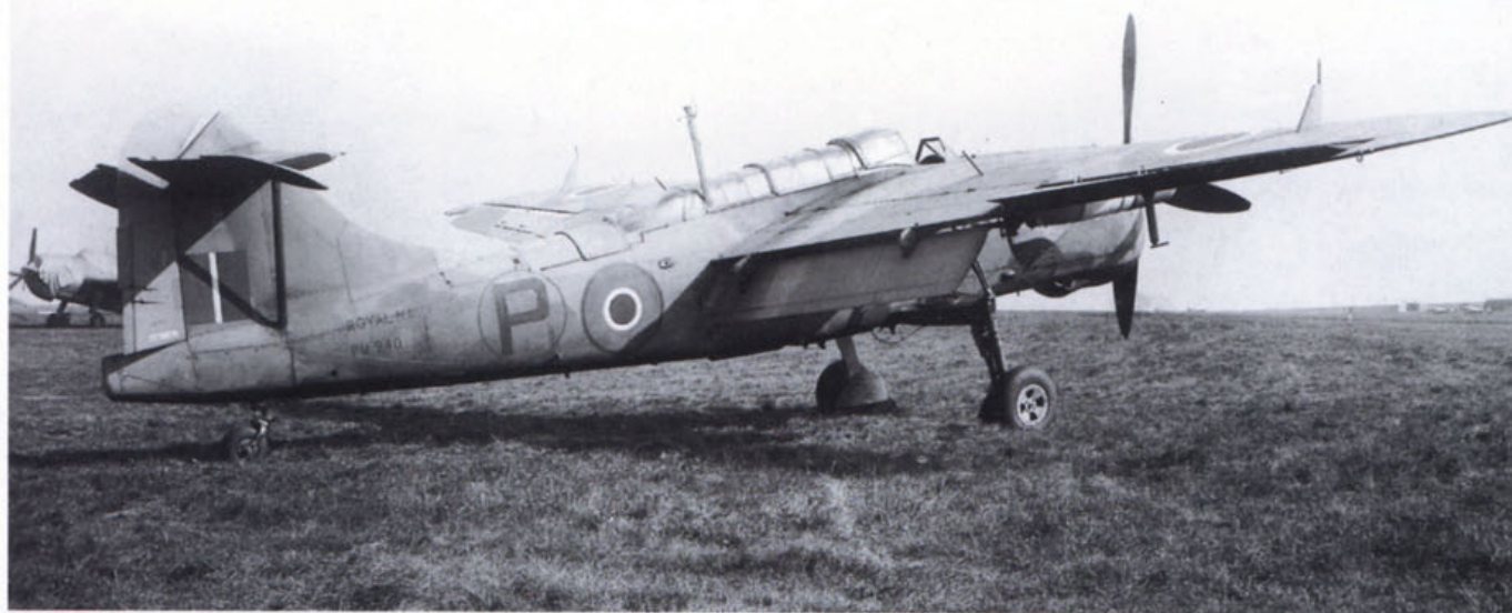
Another view of Barracuda V fifth prototype PM940. Not apparent is the ASH radar nacelle, which was located under the starboard wing, later moved to the port wing. (Crown Copyright)
