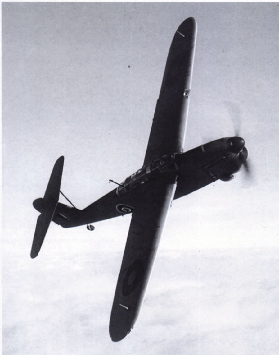
Above and below: Barracuda Mk.I P9659 out on a photographic sortie for Charles E Brown in November 1942. Noteworthy are the revised shape carburettor air intakes with a grill over the front. The 'V' shape near each wingtip is a pull-down rail to facilitate ground handling by maintenance ratings. The wing fence was to prevent disturbed airflow from bombs and carriers interfering with aileron control. (Charles E Brown via Tony Buttler)
