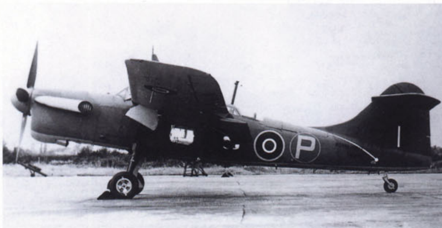
Above: This picture of Barracuda TR.III coded E shows the small area required for storage when the wings were folded. (Eric Watts/Air-Britain) Below: Barracuda PM940 became the fifth TR.V prototype in October 1945. A large fin area has been added to compensate for the extra power from the Griffon. (via Ray Sturtivant)
