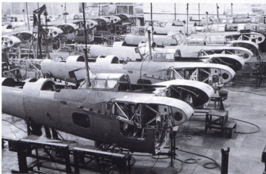
Barracudas galore! Three production lines, at Heaton Chapel, above, showing the solid centre section to which the wings were attached. (Ian Huntley) and below, the Blackburn production line at Brough. For identification purposes, until camouflaged, the aircraft serial number was painted on the rear fuselage by hand. Once finally spray painted the serial was stencilled on next to the words Royal Navy. (BAE)
