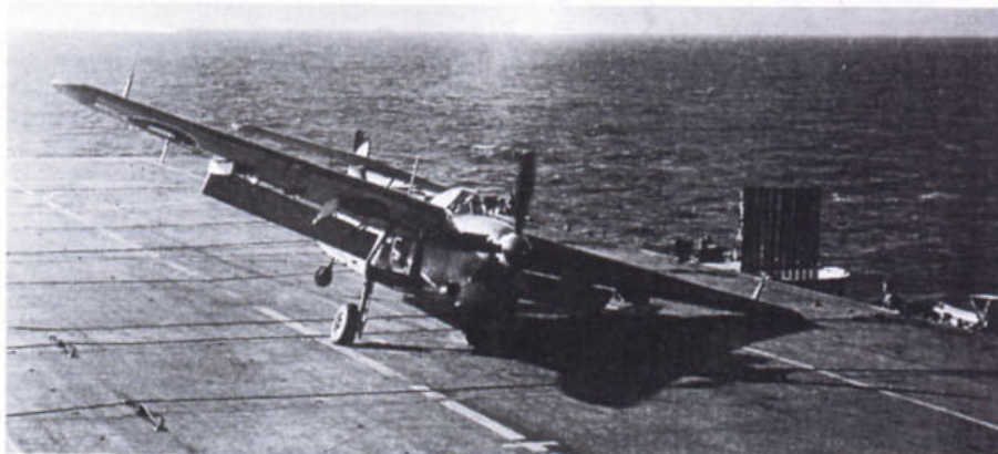
Above: Lt. (A) 'Mush' Taylor making a heavy landing which collapsed the port undercarriage leg of Barracuda II PM757 381: A landing aboard HMS Vengeance off Hong Kong 28 November 1945. The aircraft was a write off. (J. Dickson)
