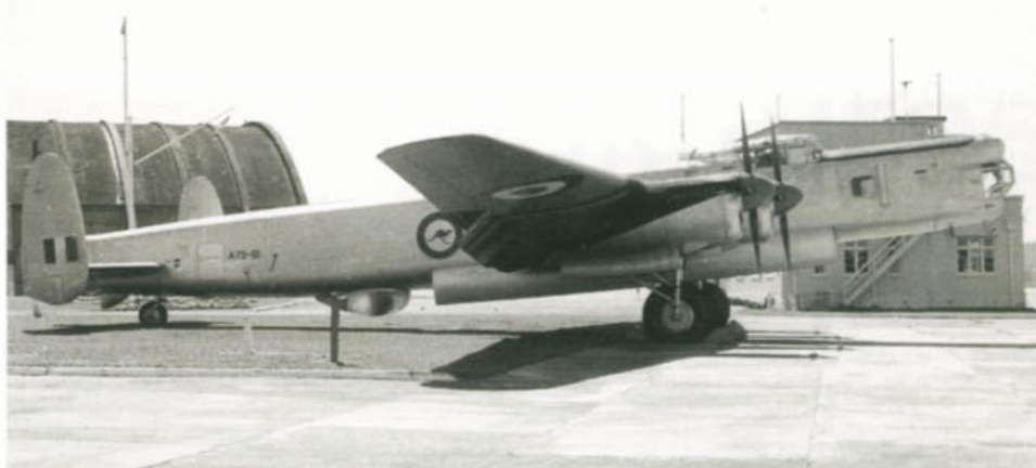
Above: The extended nose of the MR.Mk.31 helped the variant to do a fine job as a maritime aircraft, though it did nothing for the Lincoln's appearance. The view shows A73-62. Right: Side view of long-nose A73-61. Note the dark livery over the upper nacelles. (Alan Hall collection)
