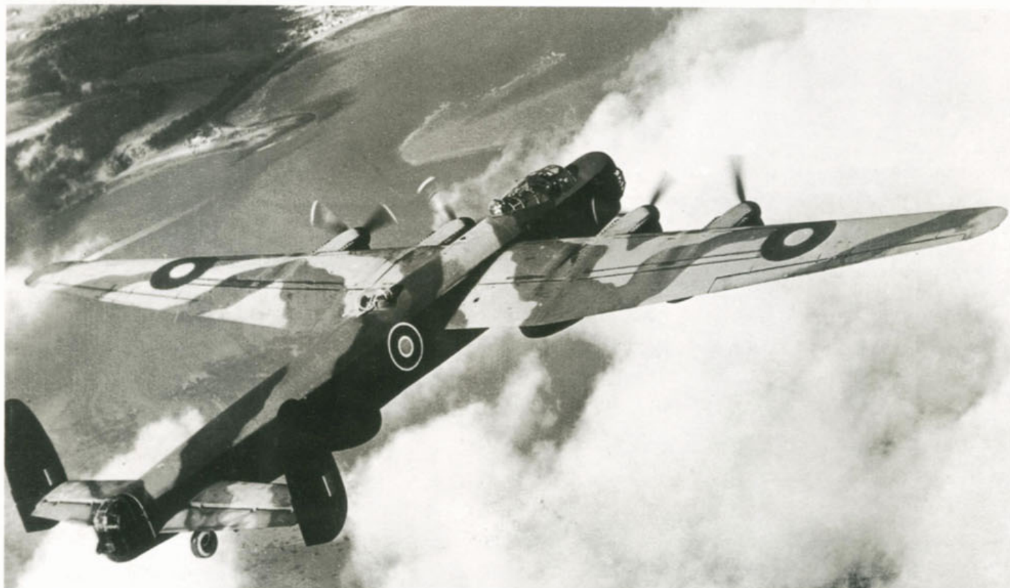
Above and below: Two contrasting pictures of second production prototype B.Mk.1 RE 228. This aircraft had an interesting career with Rolls Royce and at Boscombe Down. Interestingly both pictures show it without armament apart from the mid-upper turret. Three bladed propellers were still in evidence before the engines were changed.
