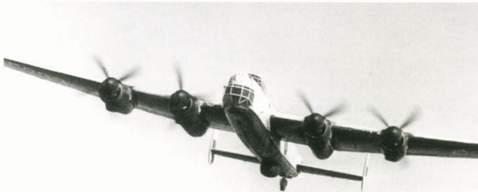
Above, below and bottom: Three views of Lincoln Mk.II RE290 in Rolls-Royce hands during the summers of 1945 or 1946. Fitted with Merlin 68s (note the dark cowlings) this aircraft became non-standard and as a 'Mk.I' passed to civilian hands in 1949 for use as a freighter during the Berlin Airlift. Note the ever-present exhaust stains on the wing upper surfaces. (Bill Harrison and Rolls-Royce)
