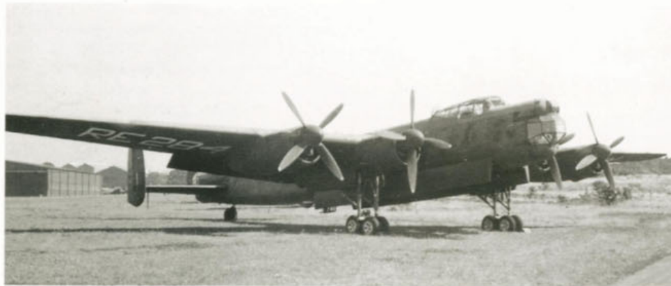
Left: B.Mk.I RE284 received a scaled-down model of the Brabazon airliner's Messier multi-wheel bogie undercarriage. It is seen on 10 September 1949 at Farnborough. (Peter Green) Lower left: RA716/G had Bristol Theseus turboprops in the outer nacelles. In April 1947 test pilot A.J. 'Bill' Pegg, flying at 120mph (193km/h), formed the aircraft on an Oxford for this photograph to be taken. Note that the inner Merlins are feathered. (Eric Myall)
