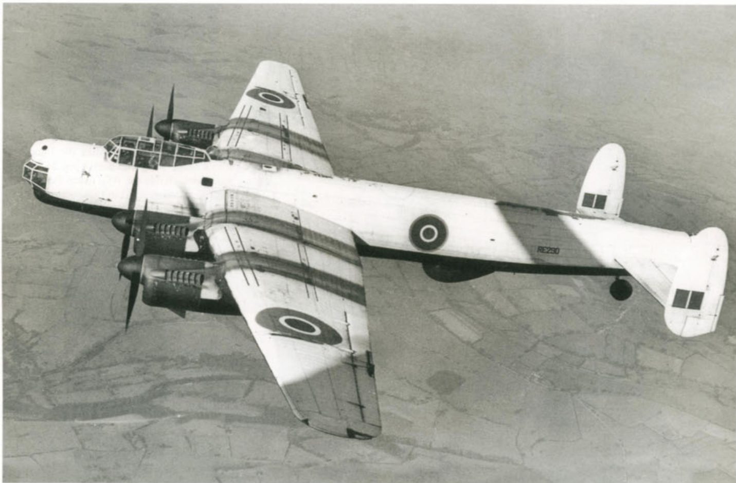
Above, below and bottom: Three views of Lincoln Mk.II RE290 in Rolls-Royce hands during the summers of 1945 or 1946. Fitted with Merlin 68s (note the dark cowlings) this aircraft became non-standard and as a 'Mk.I' passed to civilian hands in 1949 for use as a freighter during the Berlin Airlift. Note the ever-present exhaust stains on the wing upper surfaces. (Bill Harrison and Rolls-Royce)
