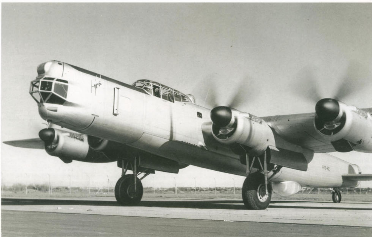
Above: The extended nose of the MR.Mk.31 helped the variant to do a fine job as a maritime aircraft, though it did nothing for the Lincoln's appearance. The view shows A73-62. Right: Side view of long-nose A73-61. Note the dark livery over the upper nacelles. (Alan Hall collection)
