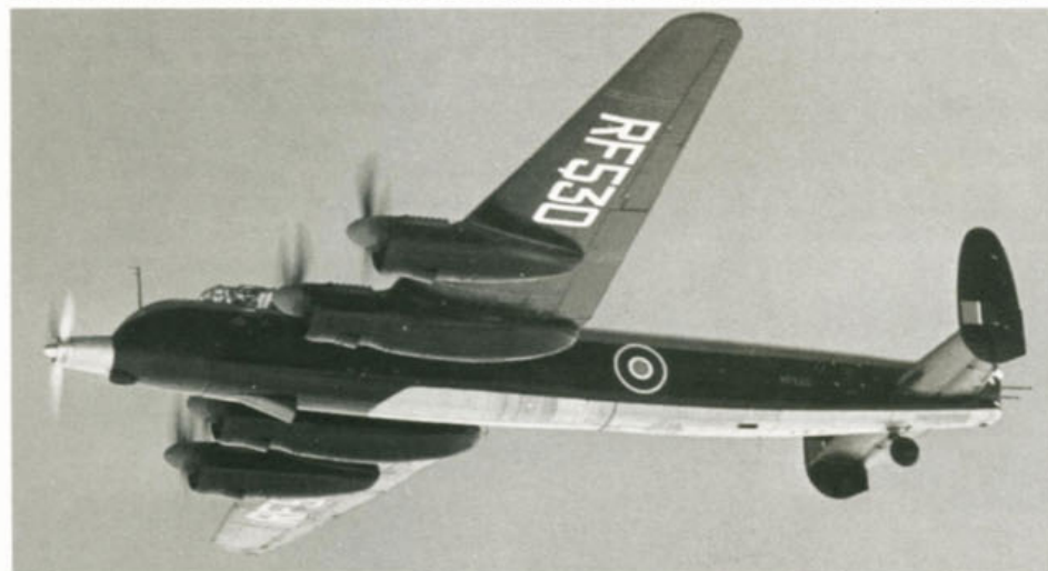
Above: Lincoln RF402's Nomad was removed later in its test programme but this view taken on 29 April 1953 shows an air intake protruding above the fuselage. (Avro Heritage) Below: RF530 had a Napier Naiad fitted in its nose in 1946. Note the jet pipe beneath the cockpit. (Alan Hall collection)
