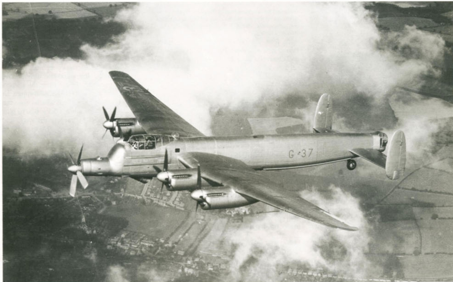
Above: Lincoln RF530 was refitted with a Rolls-Royce Tyne turboprop in its nose and flew in June 1956 registered as G-37-1. It retained its natural metal finish (Bill Harrison) Centre: Lincoln RF533 spent its entire career doing research and received a special nose designed to take all known air-interception radomes. It is seen here at Farnborough in July 1955. (Peter Green) Below: When its active experimental life was completed Lincoln RF533 ended its days with the Stansted Fire School. (Peter Green)
