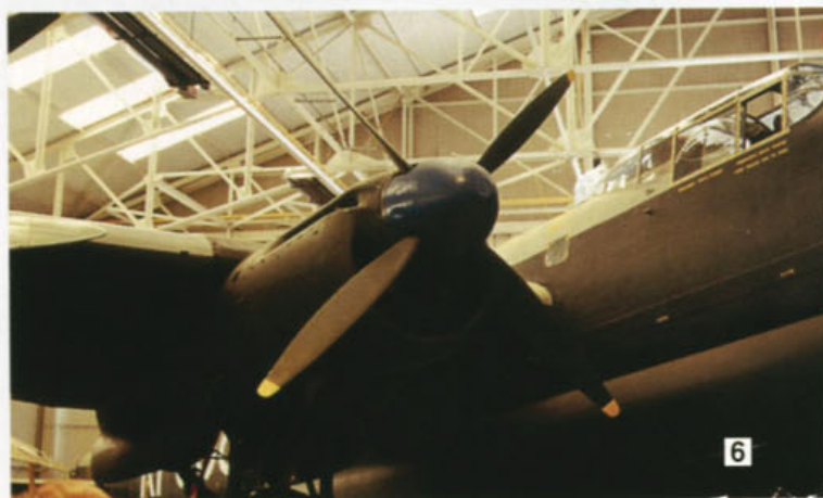
5. Looking directly under the nose of the bomb aiming position with optical flat panels and a seat for the bomb aimer as opposed to the Lancaster's prone position. 6. The starboard side of the fuselage showing the propeller feathered and the bomb doors open. Spinners were in blue and standard yellow tips appeared on the propellers. 7. Another view of the port side of the nose giving the placing of the pitot head on the mid-fuselage line and covered by a red warning tab.
