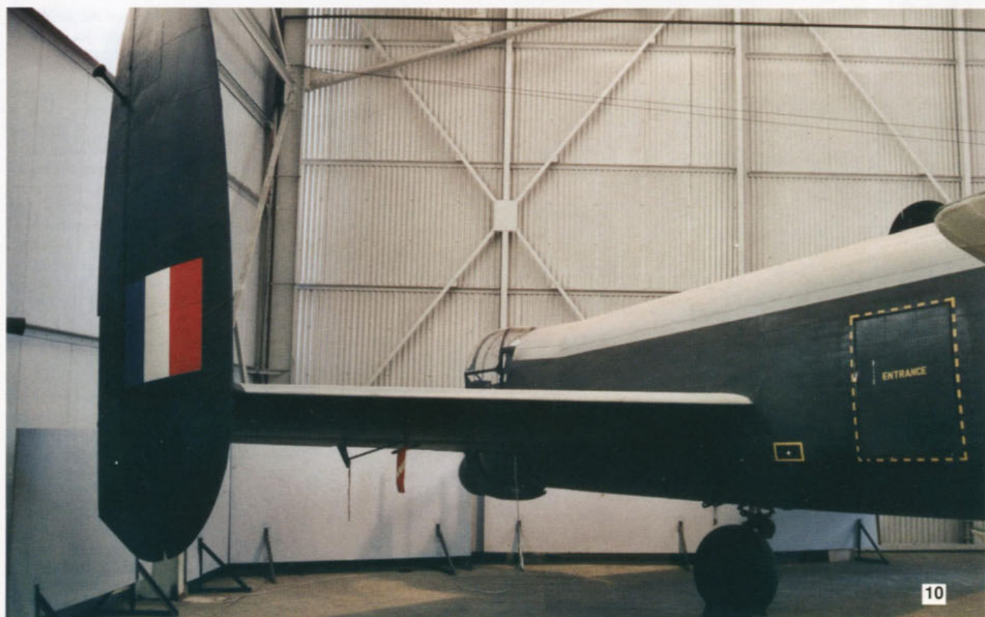
10. A useful view of the rear fuselage showing the differences in the Lincoln's tail fin compared to those of the Lancaster. The former had increased area and much larger trim tabs. Crew entrance, outlined in yellow, was also in the rear fuselage. The tail wheel did not retract. 11 and 12. Two views of the forward fuselage taken from port and starboard. The framing of the cockpit can be clearly seen and the armour plating behind the pilot's seat is also visible. All fuselage and wing stencil markings were in yellow.
