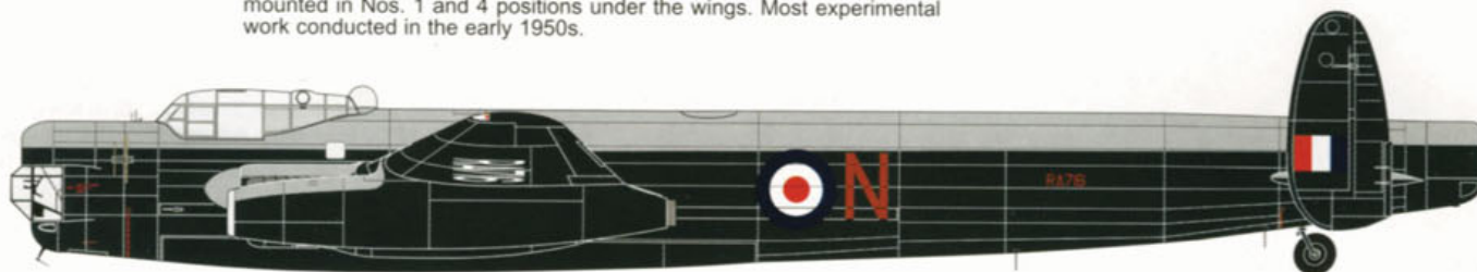
Avro Lincoln B.Mk.II RF402 later in its career was used by Napier Icing Research to evaluate the anti-icing system on the Blackburn Beverley's wing tip during 1956.
