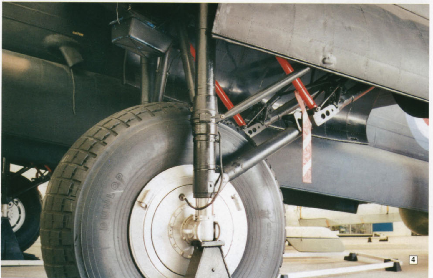
4. The main undercarriage which differed from that of the Lancaster. All main legs are in gloss black with the exception of the two retraction jacks in red and the lower part of the oleo leg in natural metal. Undercarriage locking pins are in position shown by the red tabs.
