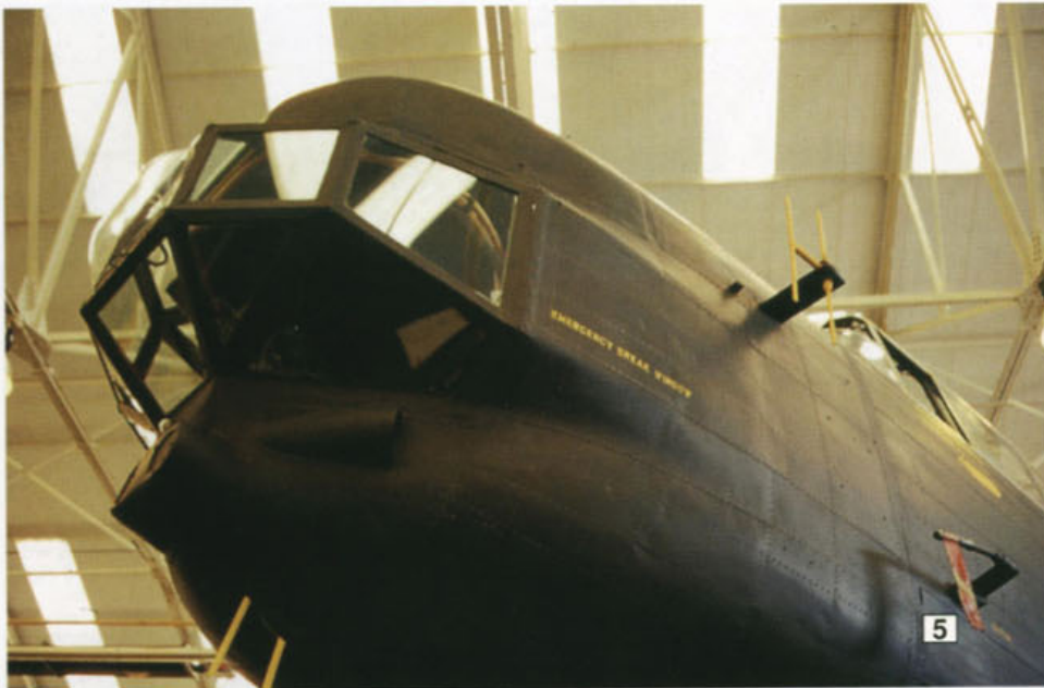
5. Looking directly under the nose of the bomb aiming position with optical flat panels and a seat for the bomb aimer as opposed to the Lancaster's prone position. 6. The starboard side of the fuselage showing the propeller feathered and the bomb doors open. Spinners were in blue and standard yellow tips appeared on the propellers. 7. Another view of the port side of the nose giving the placing of the pitot head on the mid-fuselage line and covered by a red warning tab.
