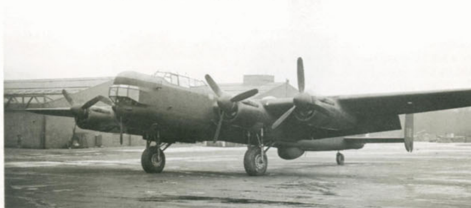
Above: RE228 the second production prototype flying with A&AEE between 27 March and 10 July 1945. The one inch (2.5cm) wide jacking positions are visible but it lacks the white underwing serials introduced to all military aircraft just after the war. Below: Official photograph taken in January 1945 of Avro-built B.Mk.I RE228, the second production aircraft with the larger rudders, three-blade props and no guns. The next month this aircraft went to Rolls-Royce at Hucknall and then in March to A&AEE for intensive flying trials (Crown Copyright/MoD)
