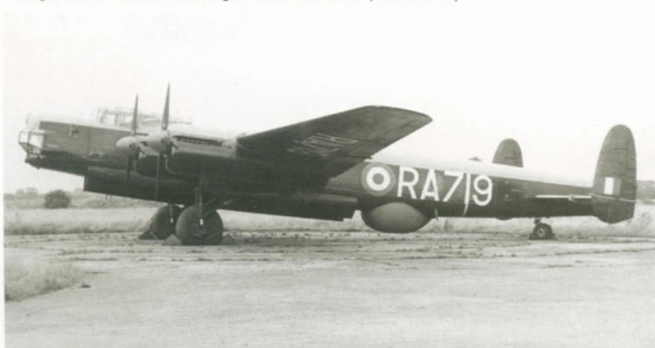
Above: Lincoln RE368 as SN:Q of No. 230 Operational Conversion Unit photographed at Middleton St. George in 1949. (MAP) Below: RA719 with the larger H2S Mk.IV A radome. Note the fuselage serial in large letters which were coming into use at the time. (Bill Harrison)
