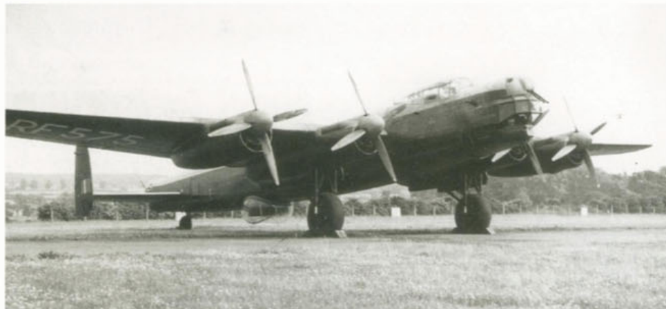
Left: New-built Lincoln Mk.II RF575 waiting delivery from Armstrong Whitworth Aircraft in 1947. Note the four-blade propellers, nose guns and the transparent H2S radome. (Eric Morgan) Lower left: Three No. 617 Squadron aircraft seen during their August 1947 visit to the USA. (Peter Green)
