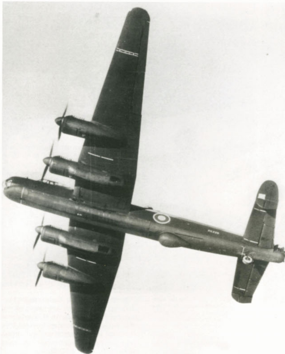
Above and below: Two contrasting pictures of second production prototype B.Mk.1 RE 228. This aircraft had an interesting career with Rolls Royce and at Boscombe Down. Interestingly both pictures show it without armament apart from the mid-upper turret. Three bladed propellers were still in evidence before the engines were changed.
