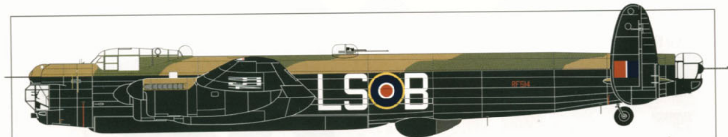
Avro Lincoln B.Mk.II RF514:LS-B of No. 15 Squadron, RAF Wyton late 1940s. This aircraft had the bulged bomb bay for either 12,000lb Tallboy or 22,000lb Grand Slam bomb trials.
