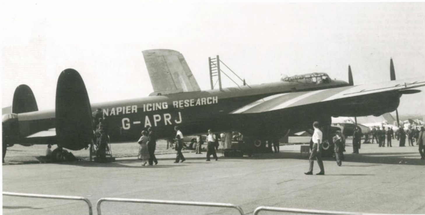
Above: As Napier's Icing Research aircraft, RF342 received civil registration G-APRJ and is seen at the September 1959 SBAC Farnborough Show complete with spray rig and test wing section above the rear fuselage. (Eric Morgan) Left: G-APRJ was later renumbered G-29-1 and then G-36-3 when it went to Cranfield in 1962. (APN)
