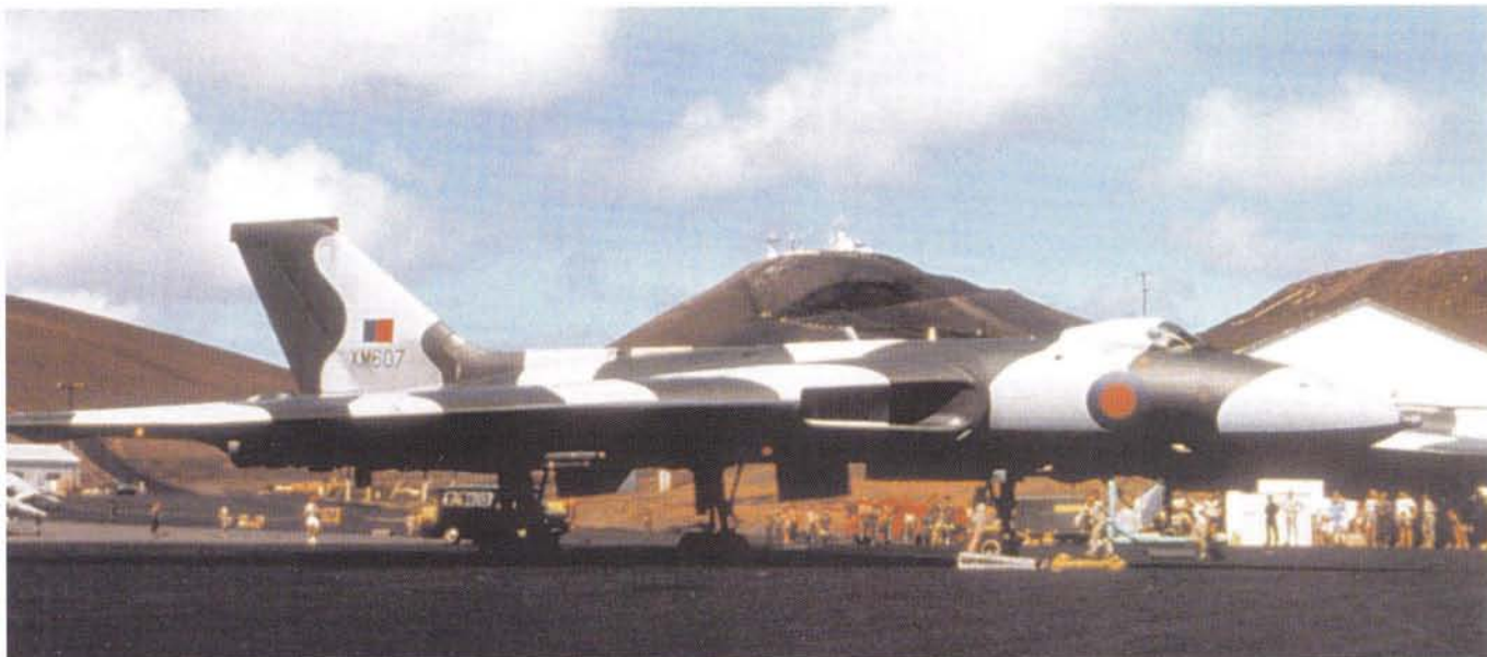
The celebrated Vulcan B.2, XM607, was one of the stalwarts of the Black Buck raids over the Falklands. It is seen here parked at Wideawake airfield complete with an ALQ-101 ECM pod under the starboard wing. Since retirement it has been the gate guard at RAF Waddington. (Mel James)
