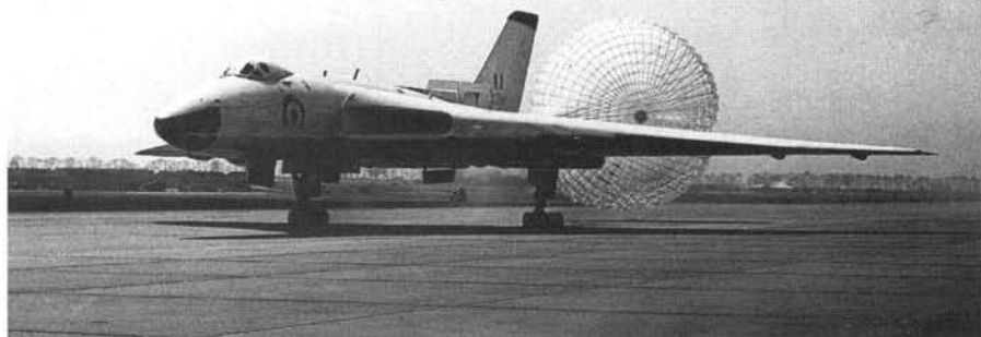
Above and below: These two pictures were taken at the Press open day at RAF Scampton when No. 83 Squadron was on show. A demonstration flight was accompanied by the use of the tail braking chute seen deployed above, and below, its release. Normally this would have been done at the very end of the runway to be collected by the Safety Equipment Section for repacking but, in full view of the cameras, it was released early as part of the demonstration. (Alan W.Hall)
