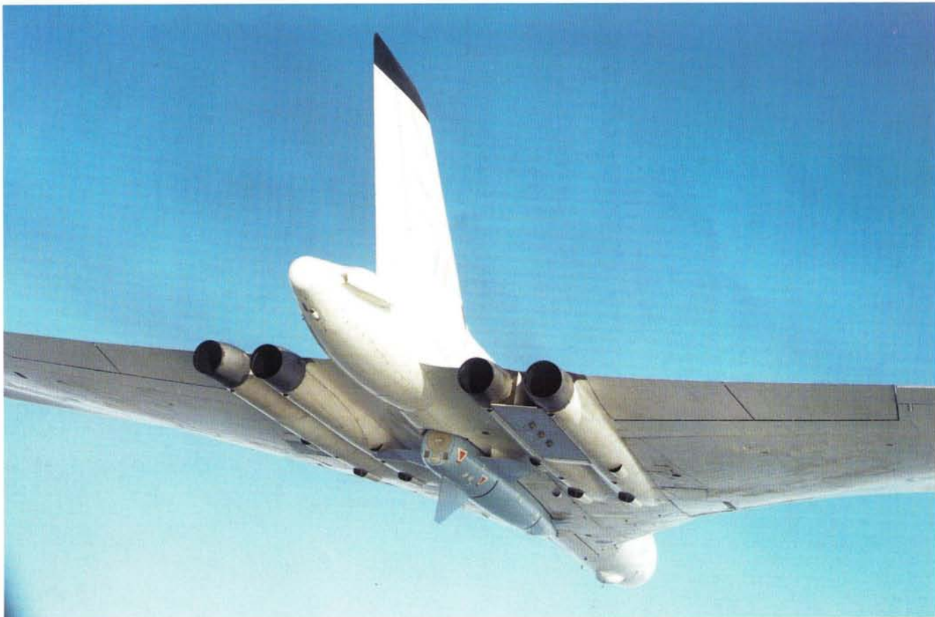
Above: This excellent rear view of Vulcan B.2, XL317, has the flashes of No. 617 Squadron on the fin. The Blue Steel round under the fuselage is a blue painted training weapon. This view shows to great advantage the angles of the jet pipes of the Olympus 201 engines. (Tony Buttler Collection) Right: Once airborne the lower fin on the Blue Steel was deployed. When approaching to land the fin was folded up to clear the ground. This view shows XL320 climbing to height, of note is the faded paintwork on this Vulcan. (Avro Heritage/ BBA Collection)
