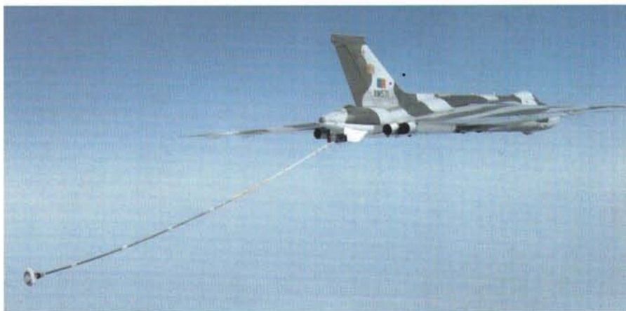
Above: Turbulence and heavy aircraft trials were carried out using Vulcan XH560 as the tanker with XL426 acting as the receiver, note the red photographic marks on the wing leading edge of the latter. Below: This rear on shot of XM571 reveals quite clearly the distinctive turn down and toe out of the jet pipe end caps. This was more noticeable on the Olympus 201 powered aircraft as the caps were longer and more slender whilst those of the more powerful Olympus 301 were more squat in nature. (Avro Heritage/BBA Collection)
