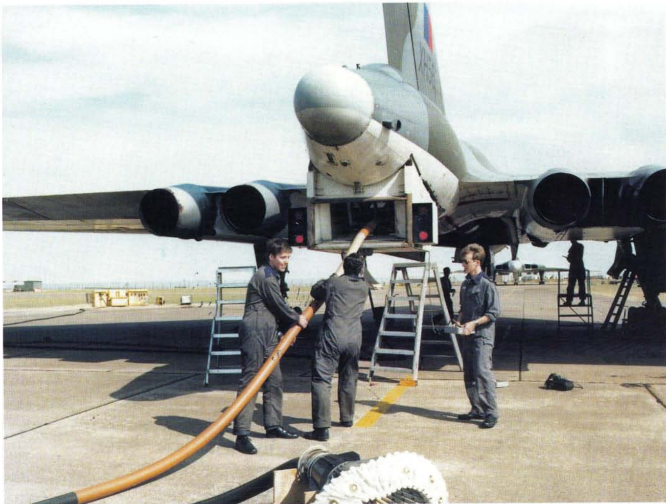
Part of the ground crew's job was to check the hose drogue unit after each sortie in case of damage. These three airmen have the hose almost fully extended to carry out the check.
