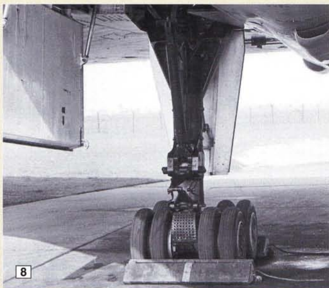
7. Another view of the Vulcan's crew entrance in front of the nose wheel assembly. Suspended from inside the undercarriage bay are the headphones used by the crew chief during start up and before taxi clearance. 8. Another view of the main undercarriage leg. Note the size of the main wheel door.
