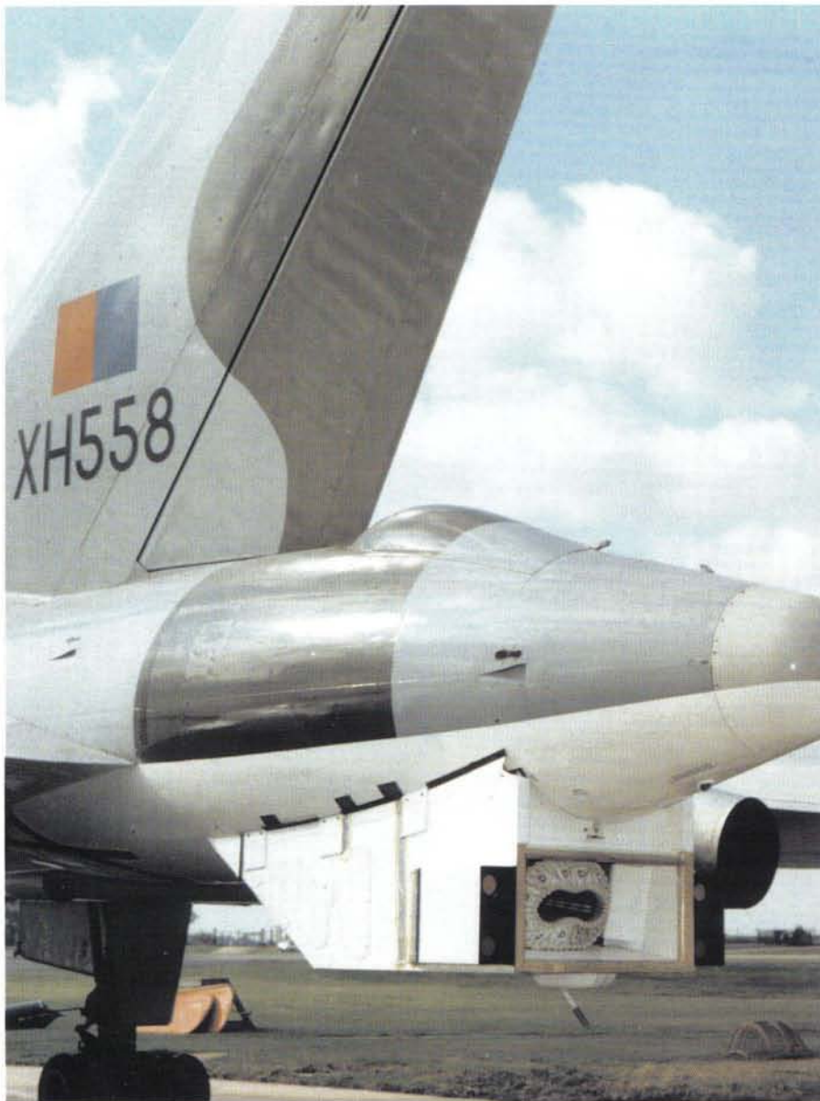
On the occasion of its roll out the now preserved Vulcan K.2, XH558 still wears the gloss finish it acquired whilst in service with No. 27 Squadron. The tanker basket can be seen under the rear fuselage with the drogue stowed inside the box. (Avro Heritage/BBA Collection)
