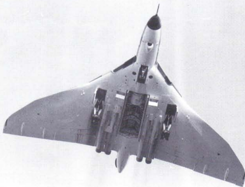
This undersurface picture of a Vulcan B.2 reveals much interesting detail. Close observation of the bomb bay reveals an 8,000 lbs fuel tank in the forward position. For those interested in 100 per cent accuracy, all the aerial covers surrounding the nose wheel bay are a faded brown in colour. (John Nickolls)
