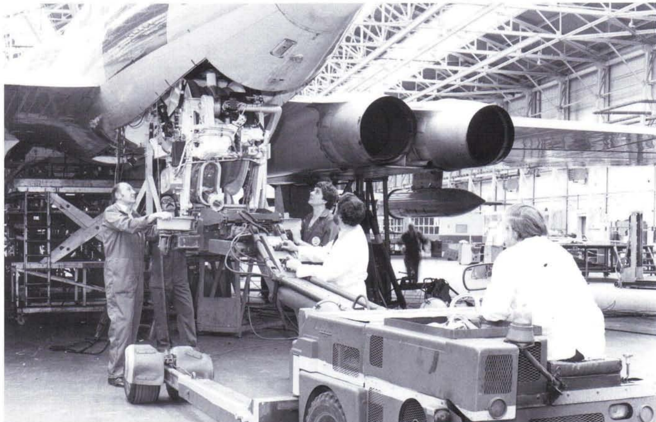
Gently does it as one part of the hose drogue unit is lifted into the rear fuselage of Vulcan XH560 which still carries the pods associated with its earlier role of B.2(MRR). (Avro Heritage/BBA Collection)
