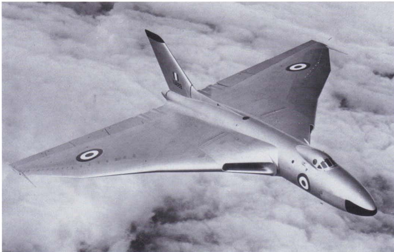
Above: Vulcan XA899 at a later stage in its life. By this time the modified wing leading edge plus vortex generators had been fitted thus improving the aircraft's performance. The machine achieved a measure of fame when it completed the world's first automatic, hands off, landing at RAE Bedford. (Avro Heritage/BBA Collection). Right: This early picture of the all-white first prototype reveals the underwing air brake, that was later deleted as superfluous, as well as an extra pitot head mounted on the tip of the all-metal nose. The badge at the top of the fin is that of Avro and note the absence of the bomb aimer's blister. (C.P.Russell Smith Collection)
