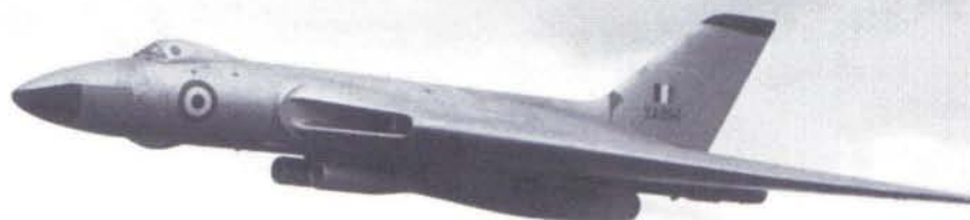
Above: Vulcan B.1, XA894, was used as a testbed throughout its short career. Here it sports the test installation required for the Gyron Junior engine. This aircraft was later used as a trials vehicle for the Olympus 22R engine destined for the TSR.2. It later burnt out on the ground during full power engine runs. (C.P.Russell Smith Collection). Below: The test installation for the forthcoming Tornado engine, the Turbo Union RB.199, seen under XA903 at the 1979 Farnborough air show, (RAE Farnborough)
