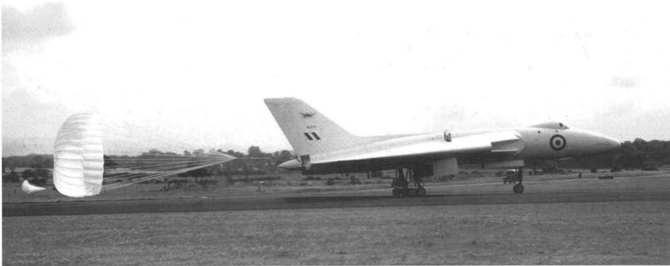
Above: By now named the Vulcan the second prototype is seen landing at Farnborough with its brake chute deployed. By this time many of the features of the production aircraft are now evident including the side mounted tail brake chute bay door. (C.P. Russel Smith)
