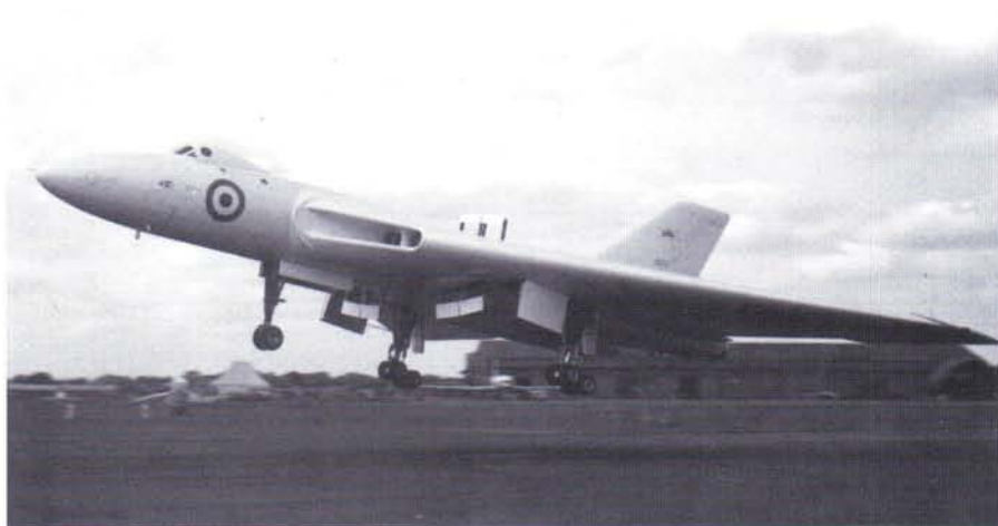
Above: Vulcan XA899 at a later stage in its life. By this time the modified wing leading edge plus vortex generators had been fitted thus improving the aircraft's performance. The machine achieved a measure of fame when it completed the world's first automatic, hands off, landing at RAE Bedford. (Avro Heritage/BBA Collection). Right: This early picture of the all-white first prototype reveals the underwing air brake, that was later deleted as superfluous, as well as an extra pitot head mounted on the tip of the all-metal nose. The badge at the top of the fin is that of Avro and note the absence of the bomb aimer's blister. (C.P.Russell Smith Collection)
