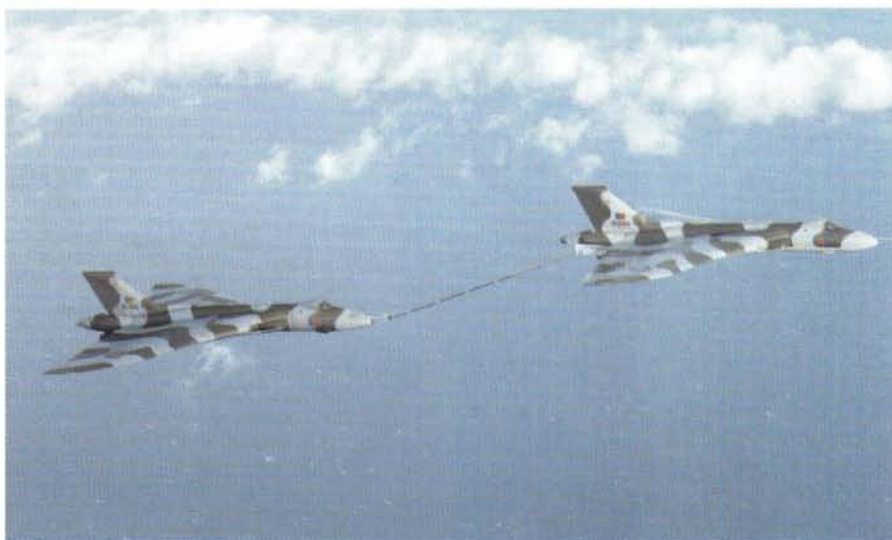
Above: Turbulence and heavy aircraft trials were carried out using Vulcan XH560 as the tanker with XL426 acting as the receiver, note the red photographic marks on the wing leading edge of the latter. Below: This rear on shot of XM571 reveals quite clearly the distinctive turn down and toe out of the jet pipe end caps. This was more noticeable on the Olympus 201 powered aircraft as the caps were longer and more slender whilst those of the more powerful Olympus 301 were more squat in nature. (Avro Heritage/BBA Collection)
