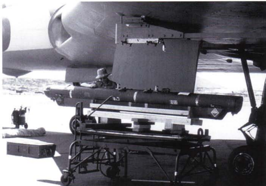
Above: Seen undergoing pre-fitment preparation is an ALQ-101 ECM pod. Such a unit was required as the internal fit in the Vulcan was tuned to the Soviet radar systems. Below: Heading for its parking slot on the Ascension Island airfield is XM598 complete with a different variation of deflector vanes on the nose. (Mel James)
