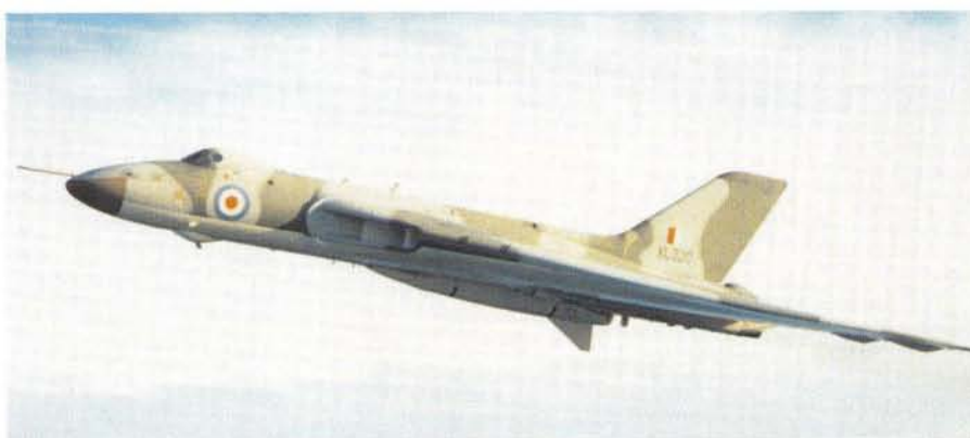
Above: This excellent rear view of Vulcan B.2, XL317, has the flashes of No. 617 Squadron on the fin. The Blue Steel round under the fuselage is a blue painted training weapon. This view shows to great advantage the angles of the jet pipes of the Olympus 201 engines. (Tony Buttler Collection) Right: Once airborne the lower fin on the Blue Steel was deployed. When approaching to land the fin was folded up to clear the ground. This view shows XL320 climbing to height, of note is the faded paintwork on this Vulcan. (Avro Heritage/ BBA Collection)
