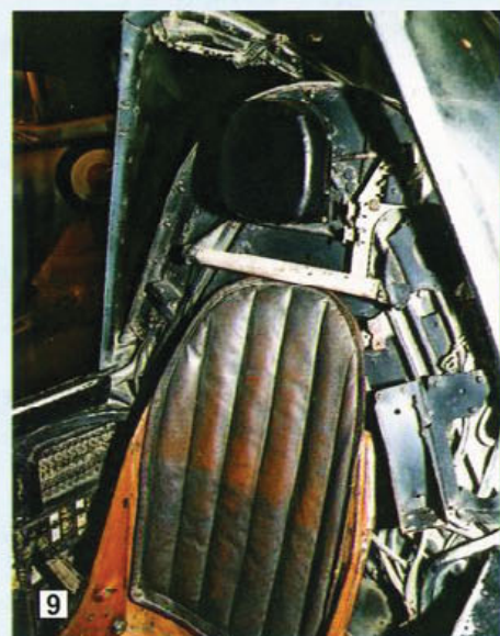
9. The cockpit of Firefly Mk.1 Z2033. The seat has a bucket shape for the parachute and a padded back in dark green. 10. The same cockpit looking at the starboard side.
