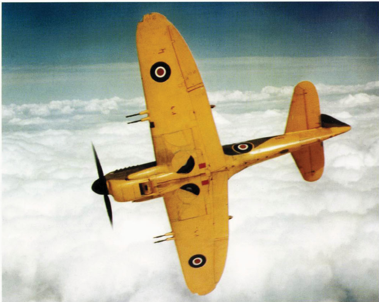
With yellow-painted undersurfaces, Firefly F.1 Z1832 shows that the original fabric covered ailerons have been replaced by metal covered ones. This Firefly was amongst the first aircraft to enter front line service with 1770 Squadron in October 1943. (RAF Museum)
