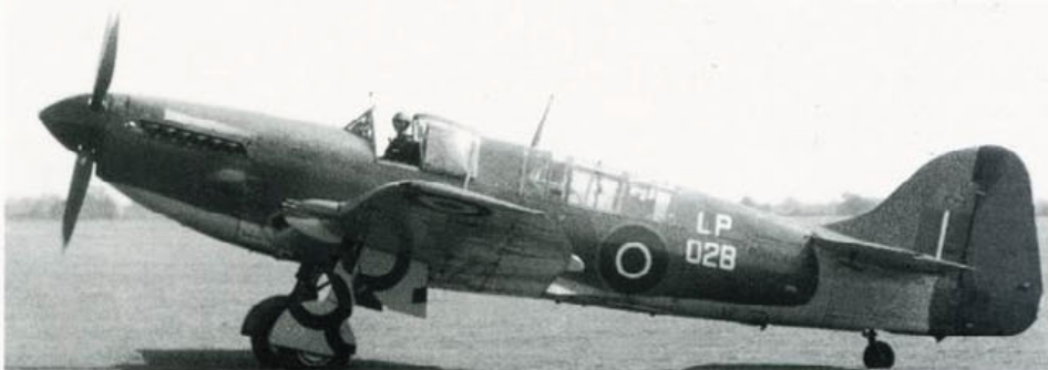
Above: Firefly Mk. 4 VG968 joined 778 Squadron at Lee-on-Solent to carry out intensive operational flight testing. The Service Trials Unit was amongst the first squadrons to receive new aircraft entering FAA service. The underwing nacelles were removed. Below: Firefly FR.4, VG980 of 737 Squadron featured the two-colour upper surface finish whilst another aircraft in the background had the new paint scheme. 737 Squadron was part of the Naval Anti-Submarine School based at Eglinton
