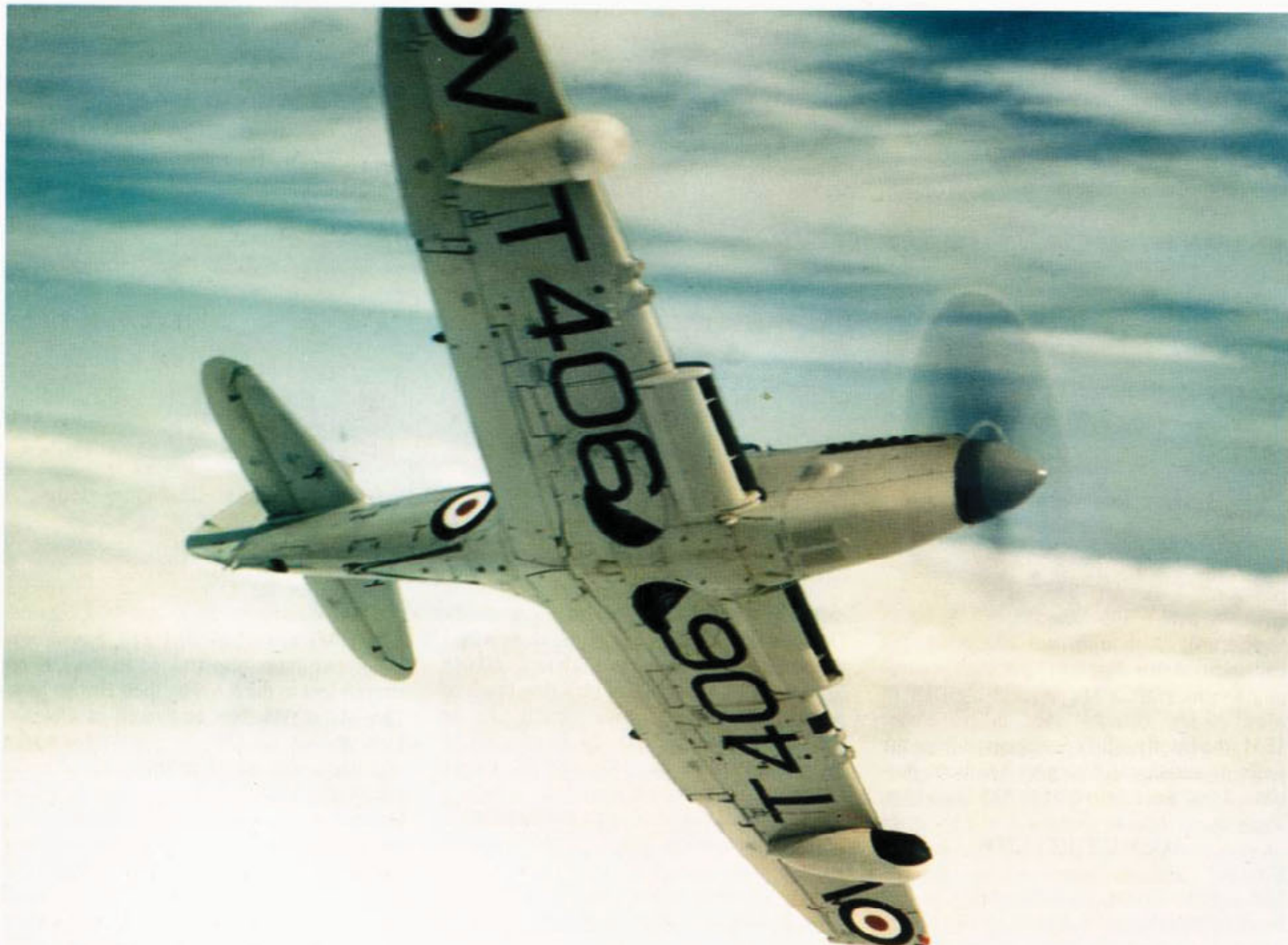
This picture of Firefly AS.5 VT406 clearly shows the arrester hook, the Youngman flaps and prominent leading edge radiator air intakes.
