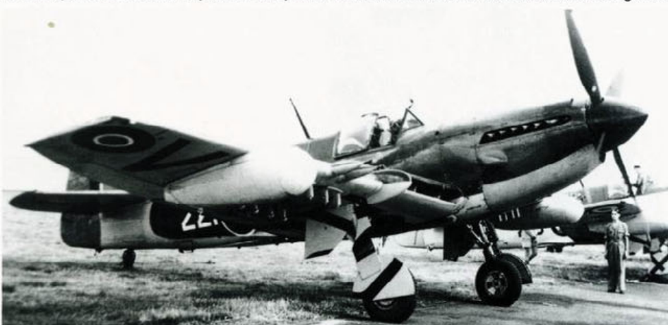
Above: Firefly Mk. 4 VG968 joined 778 Squadron at Lee-on-Solent to carry out intensive operational flight testing. The Service Trials Unit was amongst the first squadrons to receive new aircraft entering FAA service. The underwing nacelles were removed. Below: Firefly FR.4, VG980 of 737 Squadron featured the two-colour upper surface finish whilst another aircraft in the background had the new paint scheme. 737 Squadron was part of the Naval Anti-Submarine School based at Eglinton
