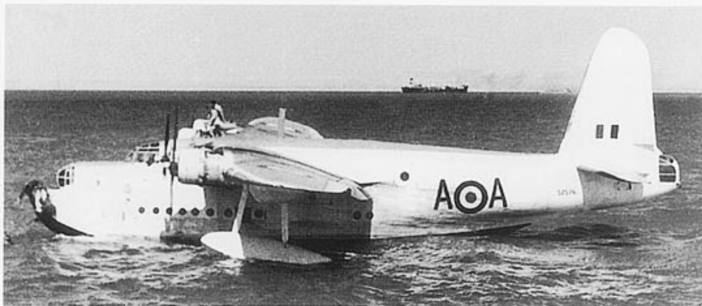
Mk.5 SZ576 A:A of No. 201 Squadron. Note the extended Gouge Flap. The picture was probably taken in the Mediterranean as the three crew members on top of the fuselage are scantily clad. (MAP)
