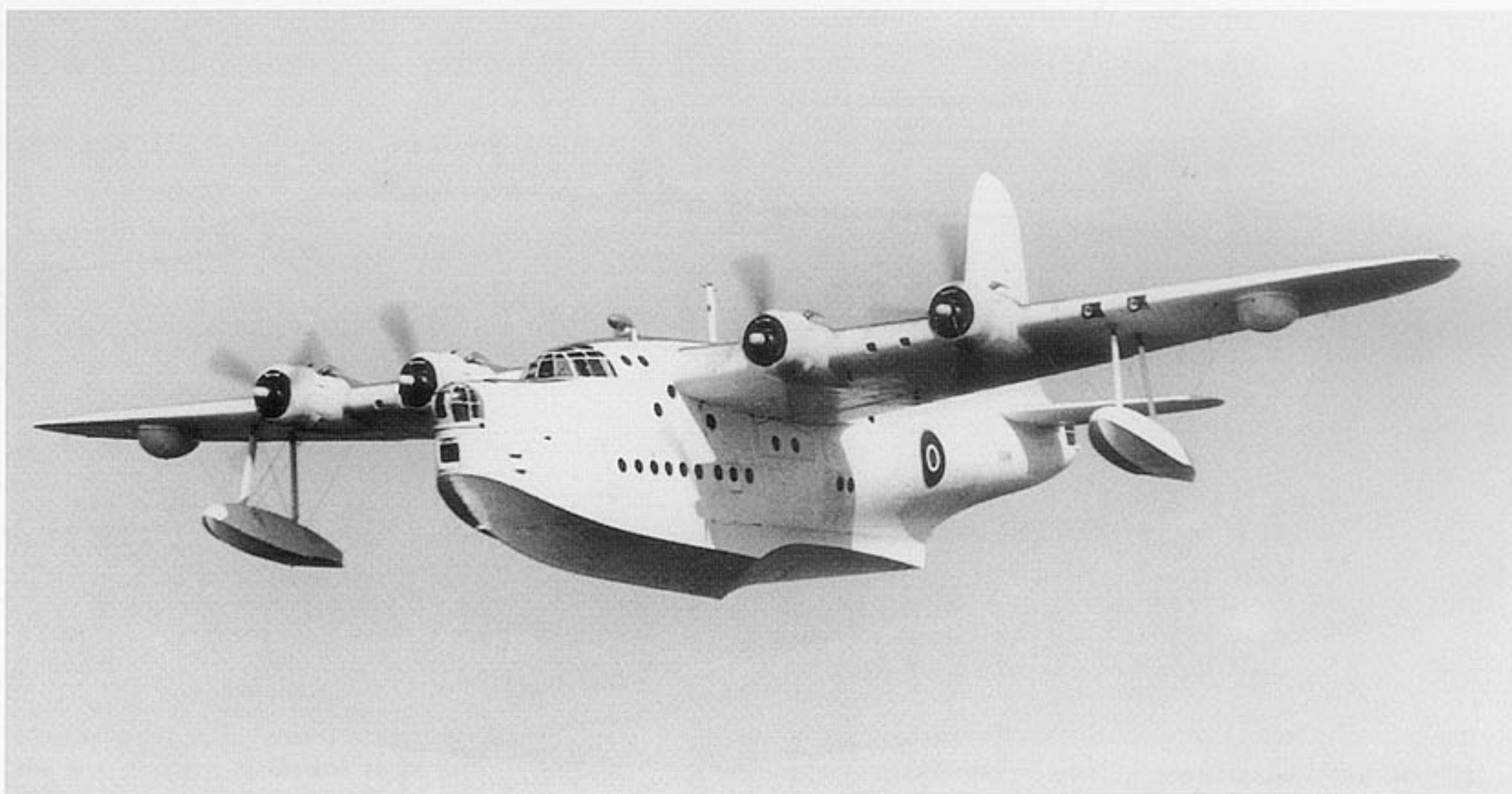
The final Sunderland variant was the Mk.V. This view shows how the design has evolved with Pratt & Whitney engines and enclosed underwing radar scanners now fitted. (Short Bros.)
