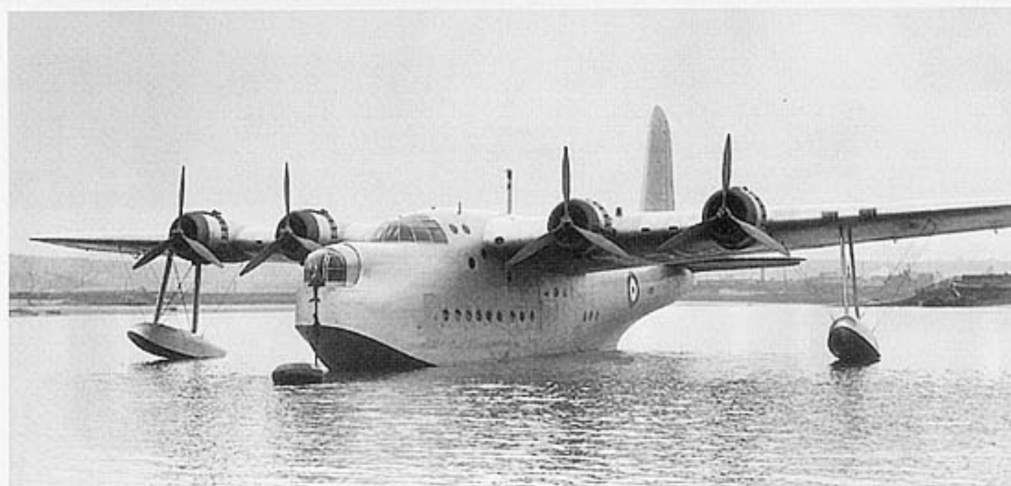
Above: Another view of K4774, this time pictured at MAEE Felixstowe in about August 1938. It now has the swept wing which featured on every other Sunderland, a repositioned main step on the planing bottom and Pegasus XXII engines. The double-wheel beaching chassis and tail trolley are shown to good effect. (MoD) Left: The first Mk.I Sunderland was L2158 seen here on the River Medway in May 1938. From the side one can see how the outer engines have moved slightly behind the inner units, an effect of sweeping the wing, and how the nose turret retracts backwards to facilitate mooring. This aircraft went to MAEE Felixstowe on 2 June. (Eric Morgan)
