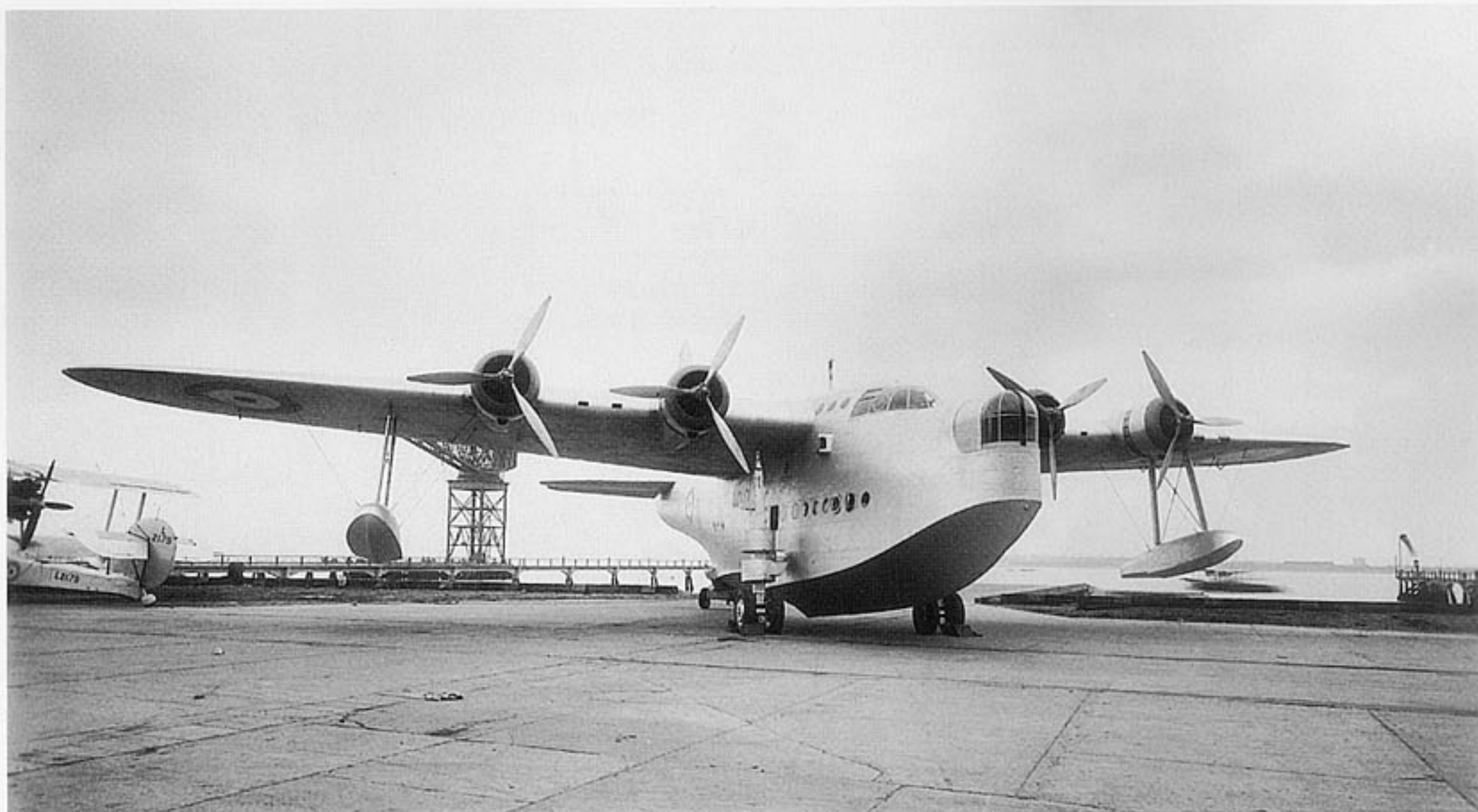
Above: Another view of K4774, this time pictured at MAEE Felixstowe in about August 1938. It now has the swept wing which featured on every other Sunderland, a repositioned main step on the planing bottom and Pegasus XXII engines. The double-wheel beaching chassis and tail trolley are shown to good effect. (MoD) Left: The first Mk.I Sunderland was L2158 seen here on the River Medway in May 1938. From the side one can see how the outer engines have moved slightly behind the inner units, an effect of sweeping the wing, and how the nose turret retracts backwards to facilitate mooring. This aircraft went to MAEE Felixstowe on 2 June. (Eric Morgan)
