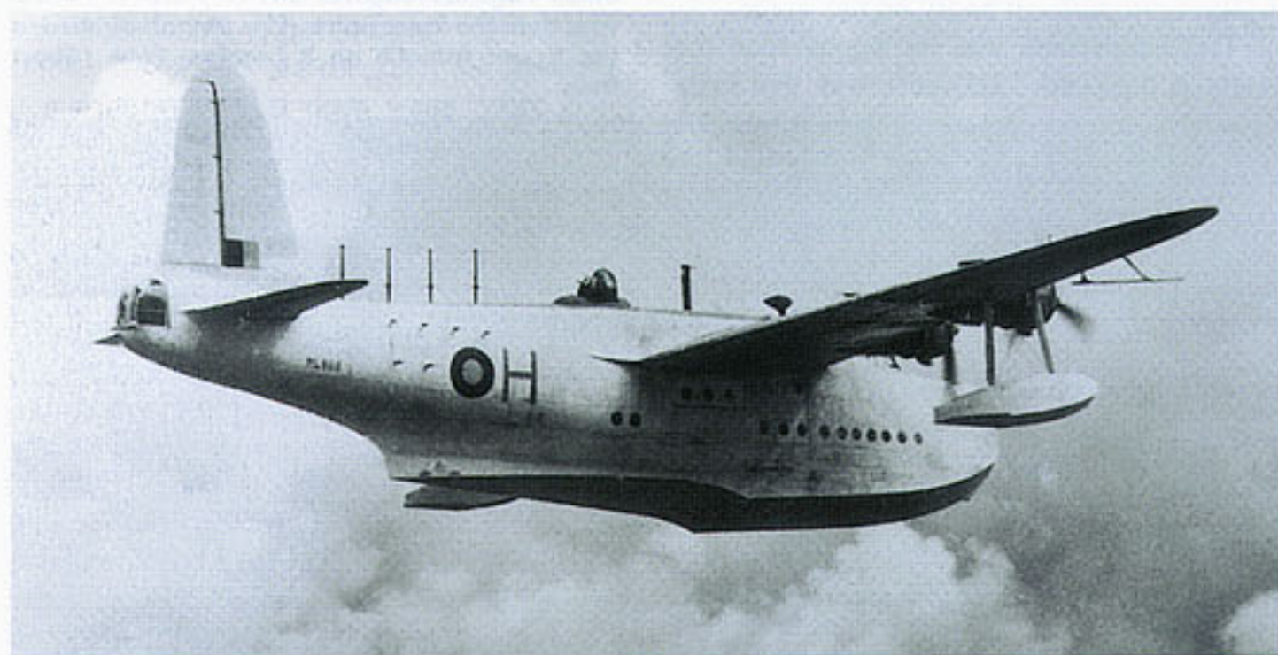
Sunderland ML868:H, a Mk.III built by Blackburn at Dumbarton, in service with No. 230 Squadron flying over Lake Koggala in Ceylon in 1944-45. It shows the new planing bottom. (MAP)
