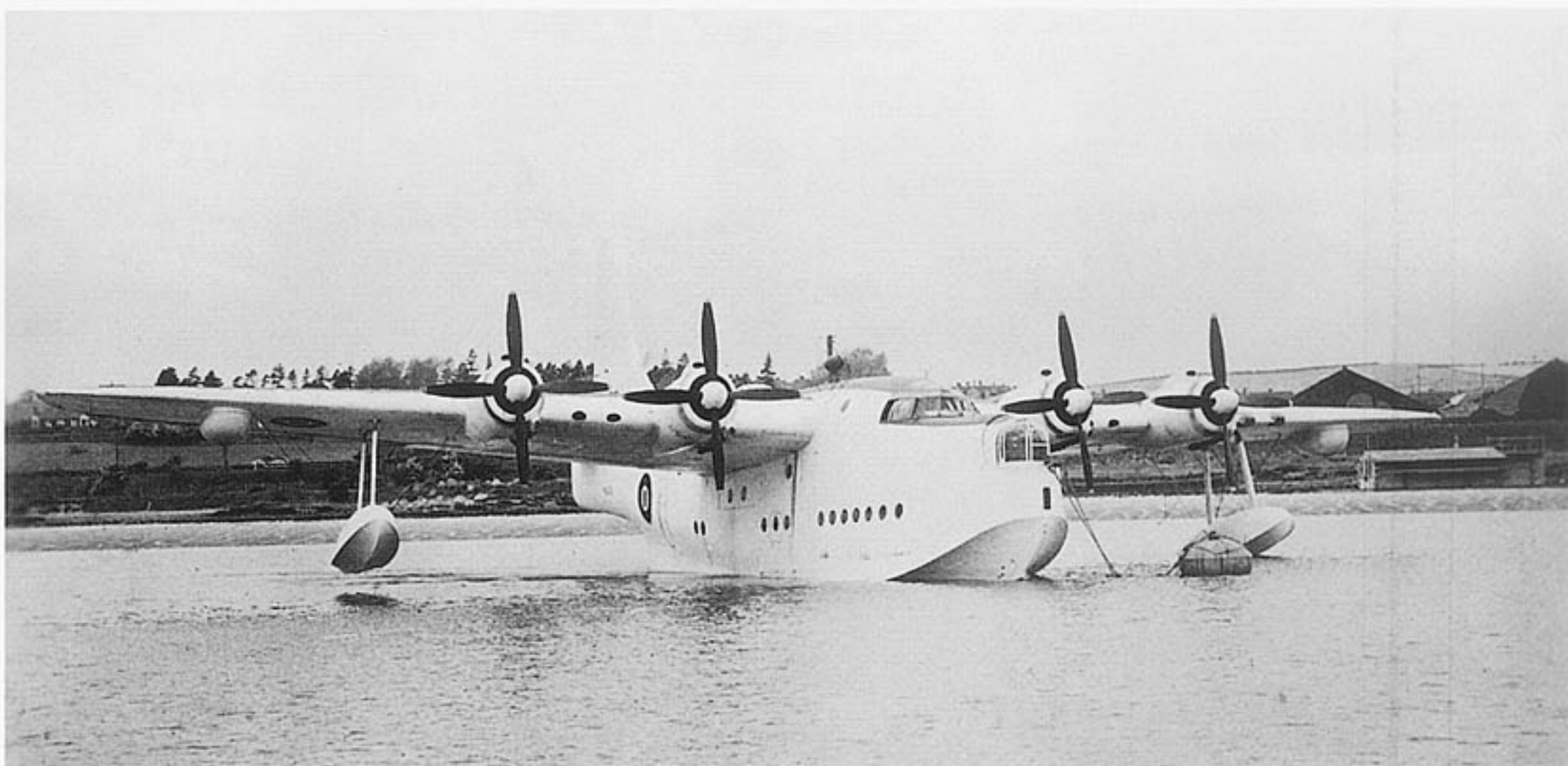
The first prototype Sunderland Mk.IV (later Seaford Mk.I) MZ269 with four Hercules XIXs. The picture was taken in April 1945. (MoAP)
