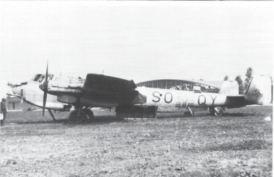
Top right: A Do 217J-1 bearing the 'Englandblitz' badge of the Nachtjagd undergoing armament maintenance and exhibiting the blast tubes for the 20-mm MG FF cannon mounted below the masts for the radar aerials. Right: Found by Allied troops at Straubing, Germany in May 1945 this Do 217N-1 bears radio call letters rather than operational codes - which does not necessarily indicate a second line machine. With their backs to the wall the Germans then had more pressing priorities than painting unit identity on aircraft. Note the open bomb bay, fuselage hatch and sprung Zeus fasteners holding the machine gun ammunition access doors in place. (J. V. Crow)
