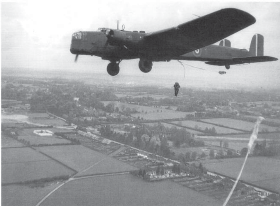
A training jump from a Whitley Mk.III. The troops are exiting the aircraft from the space made available by the removal of the FN 17 turret under the fuselage. (IWM)
