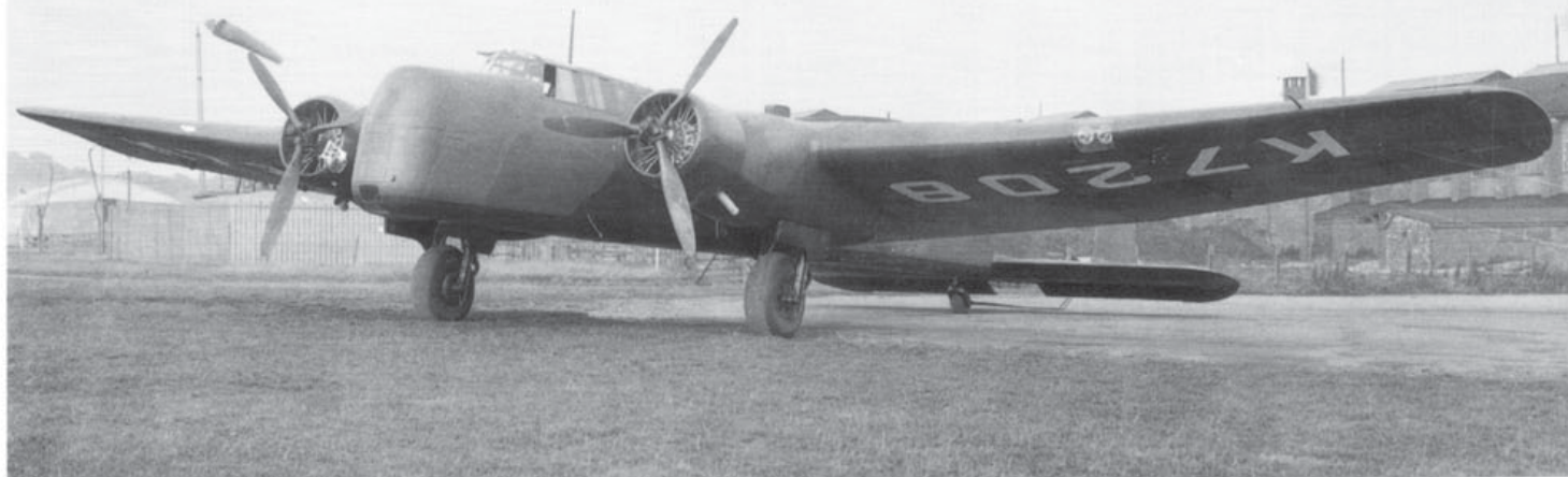
Above and left: Whitley Mk.I K7208, after its arrival at Rolls Royce, Hucknall, in late 1937 where two Armstrong Siddeley Tiger IX radials were replaced by Rolls Royce Merlin IIs. The nose and tail turrets have been superseded by fairings, a legacy of earlier modifications to permit a gross operating weight of 33,000 lbs. (Rolls Royce)
