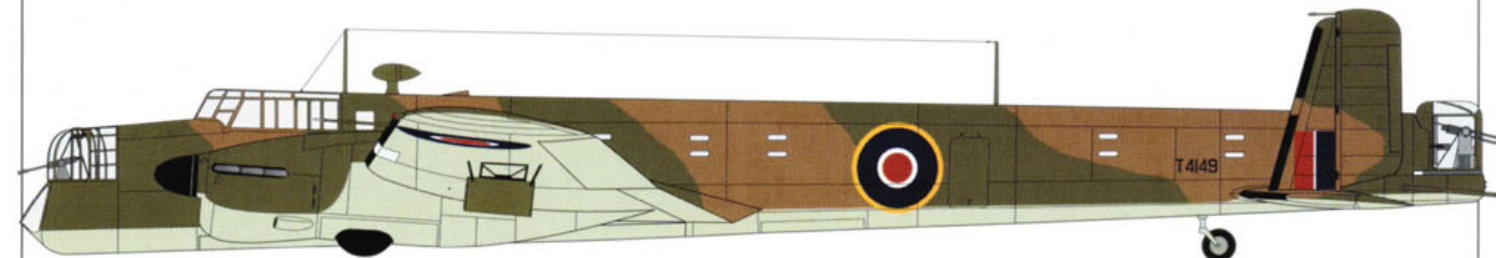
Armstrong Whitworth Whitley Mk.V T4149, A&AEE Boscombe Down, 1943. Used for rocket assisted take-off trials, note underwing cannisters.
