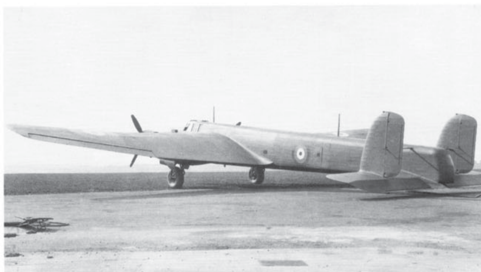
Above and left: Whitley Mk.I K7208, after its arrival at Rolls Royce, Hucknall, in late 1937 where two Armstrong Siddeley Tiger IX radials were replaced by Rolls Royce Merlin IIs. The nose and tail turrets have been superseded by fairings, a legacy of earlier modifications to permit a gross operating weight of 33,000 lbs. (Rolls Royce)
