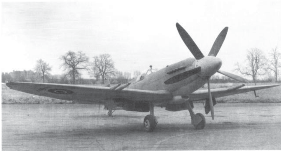
Left and lower left: Two views of the Seafire F.Mk.45 which was basically a navalised Spitfire F.21 with a hook, slinging points and a naval radio. Strengthened wings allowed the installation of four 20-mm Hispano cannon. It had a top speed of 443 mph powered by a Griffon 61 engine. The aircraft lower left is LA443 seen at Boscombe Down. (IWM and DERA)
