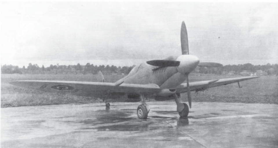
One of the early production Seafire F.XVIIIs seen at Yeovil where they were built. Bomb shackles appear under the wings as well as distinctive trestle markings. (MoAP)
