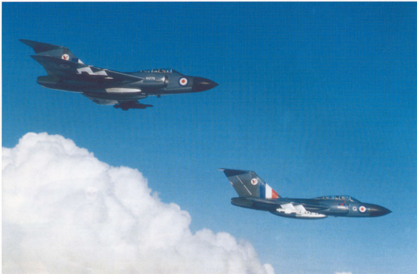
Two of No. 23 Squadrons Javelin FAW.Mk.7s in formation. Both are armed with Firestreak missiles with the upper left aircraft having black painted ones which probably means that they are dummy rounds. (MoD)
