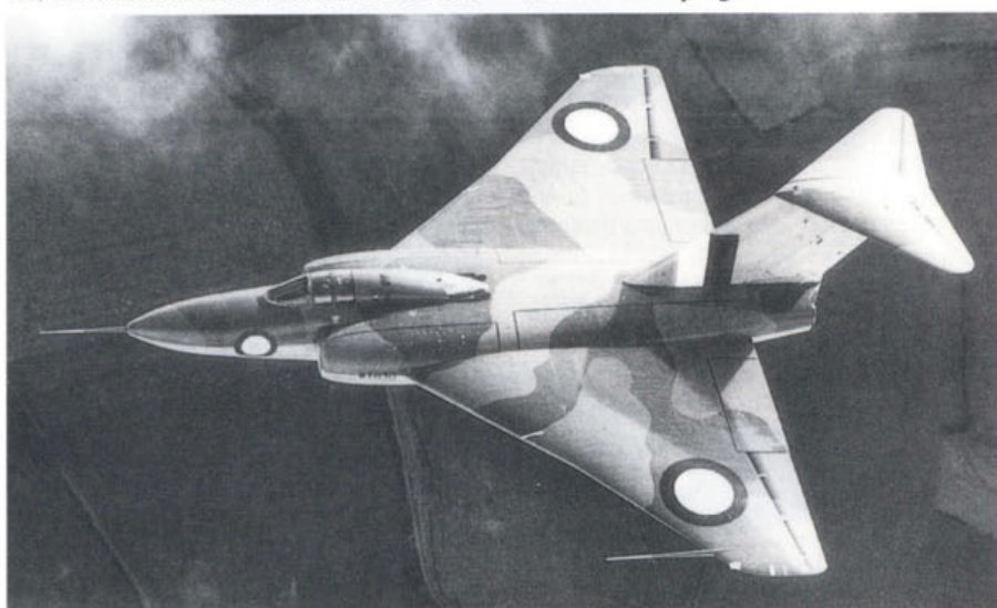
The fourth prototype WT830 shows the modified kinked wing leading edges. As with some of the other prototypes the rear of the cockpit is faired over. This aircraft ended its days as an instructional airframe at RAF Halton, serialised 7485M.
