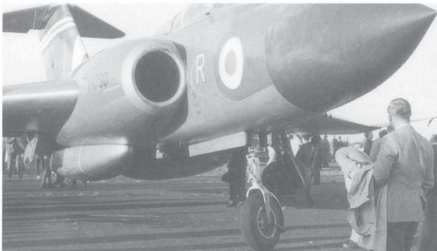
Above: Front view showing fully extended nose wheel. (Author) Below: Reheat extension on jet exhaust of a Javelin FAW Mk.9. (A.W.Hall)
