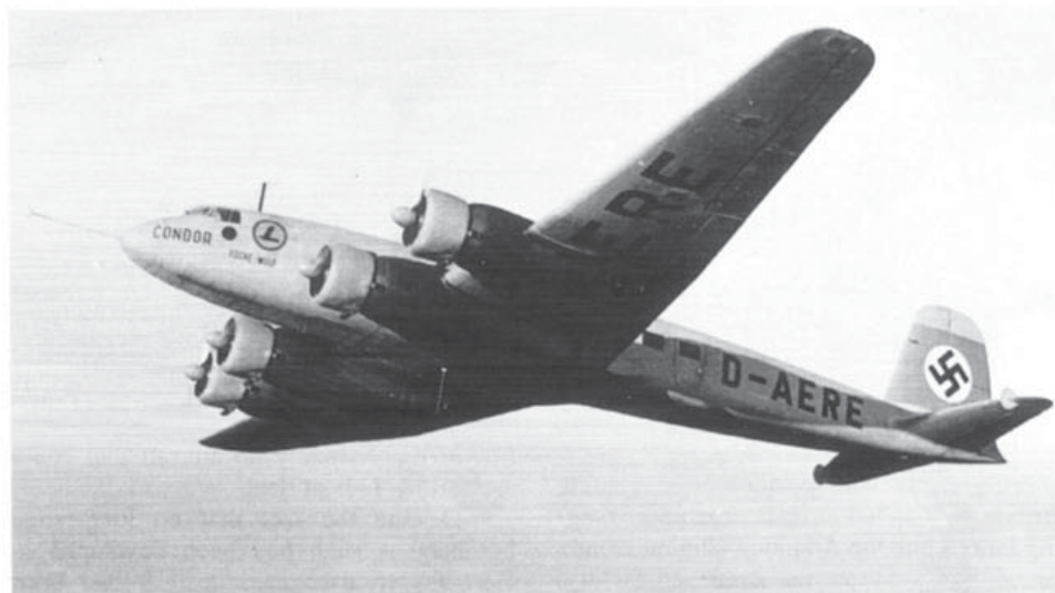
Marked with its civil registration and swastika tail band, the first Condor carries a nose probe for instrumentation and has the early curved rudder trailing edge (Denes Bernad)
