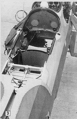
1. Loading a torpedo onto a Swordfish. Note the two cradles to which it will be attached. 2. The enclosed cockpit on Swordfish IV HS553. 3. The Observer's cockpit without instrumentation. 4. Swordfish II rear cockpit with instruments, radio and Vickers gun in place. 5. Swordfish II V4689, pilot's cockpit.
