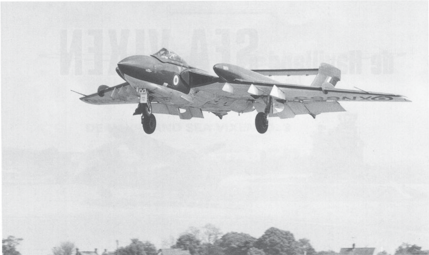
One of the Sea Vixen FAW. 2s used by RAE Bedford was XN653, which had previously served with 892 Squadron. It flew from Bedford throughout the 1970s devoid of naval markings and with a raked fin flash applied, and never fitted with the bulged, frangible observer's hatch. (A.W.Hall)
