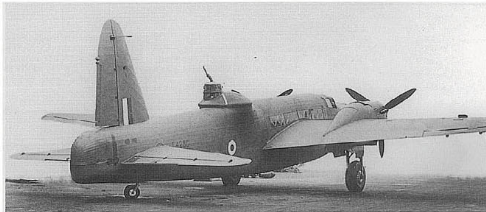
Wellington Mk. II L4250 was modified to have a single Vickers 40-mm cannon fitted on the rear fuselage. This view shows it with the original single fin and rudder.
