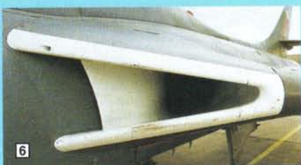
6. Port jet intake unusually painted white. 7. A view of the jet orifice. The doors above house the braking parachute.
