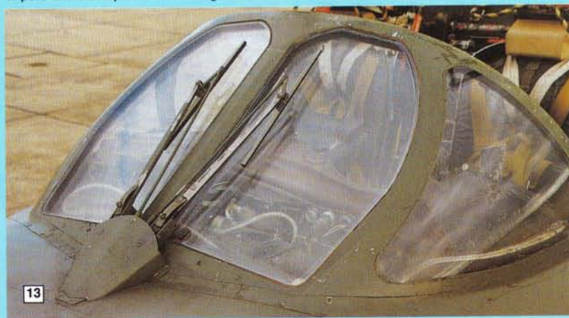
11. The inner undercarriage door port side. Note the actuating jack. 12. The port inner stores pylon. Note its location in relation to the saw tooth wing leading edge and main undercarriage leg. 13. Close-up of the windscreen of the T.8C showing the housing for the windscreen wipers and the top of the coaming inside.
