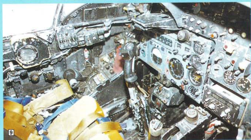
8 and 9. Cockpit interior and instrument panel. Colours predominantly black but well worn and scuffed. 10. Starboard view of the air brake in the closed position.
