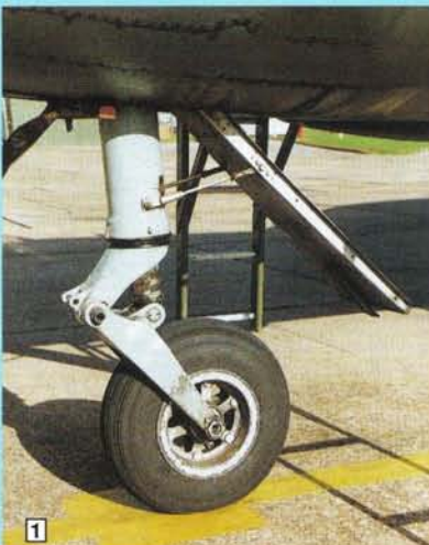
1. Nose undercarriage leg and rear door. 2. Starboard main undercarriage leg. 3. Signs of previous FAA ownership. The arrester hook fairing with the hook removed.
