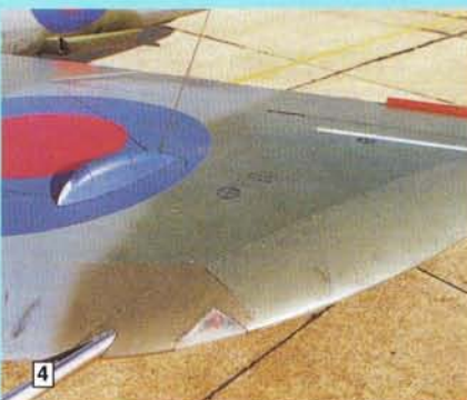
4. Upper port wing detail shows the navigation light, pitot tube and tear-shaped ejector fairing.
