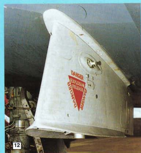
11. The inner undercarriage door port side. Note the actuating jack. 12. The port inner stores pylon. Note its location in relation to the saw tooth wing leading edge and main undercarriage leg. 13. Close-up of the windscreen of the T.8C showing the housing for the windscreen wipers and the top of the coaming inside.
