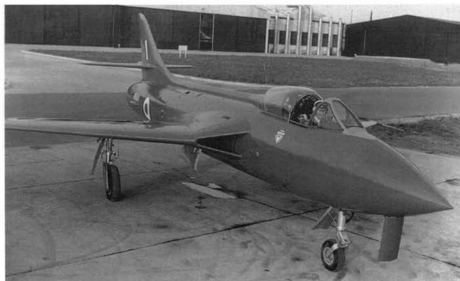
Right: Compare this picture of the Hunter F.3 with that on the previous page and it will be seen that it was taken before the forward part of the canopy was modified.
