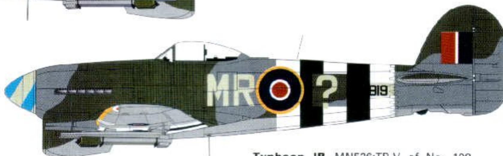
Typhoon IB MN526:TP-V of No. 198 Squadron, at B.10 Plumetot in July 1944. AEAF bands on undersurfaces only. Code letters 'TP' in Medium Sea Grey and repeated in small white letters on the nose. Sky 'V' repeated in white on the fin. Tempest tailplane. RP Mk.1 rocket rails.
