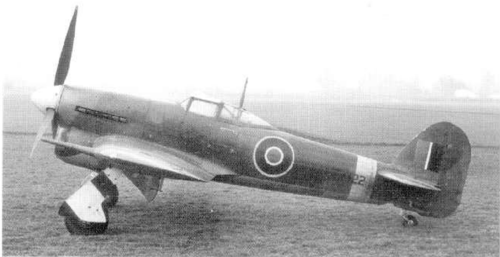
This aircraft EK122, shows the production standard in the Spring of 1943. The cannon barrels are now faired, a rear view mirror is housed in a small blister on the canopy and the external rudder balance has been replaced by an internal one. EK122 was retained by Hawkers for trials into high speed dives during the investigation into tail failures. It was later used by Napiers for engine development. (BAe)
