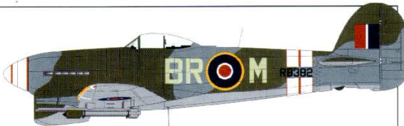
Typhoon IB RB382:BR-M of No. 184 Squadron, August 1945. Spinner and fuselage bands red and white. Tempest tailplane, RP, Mk. 3 rocket rails.
