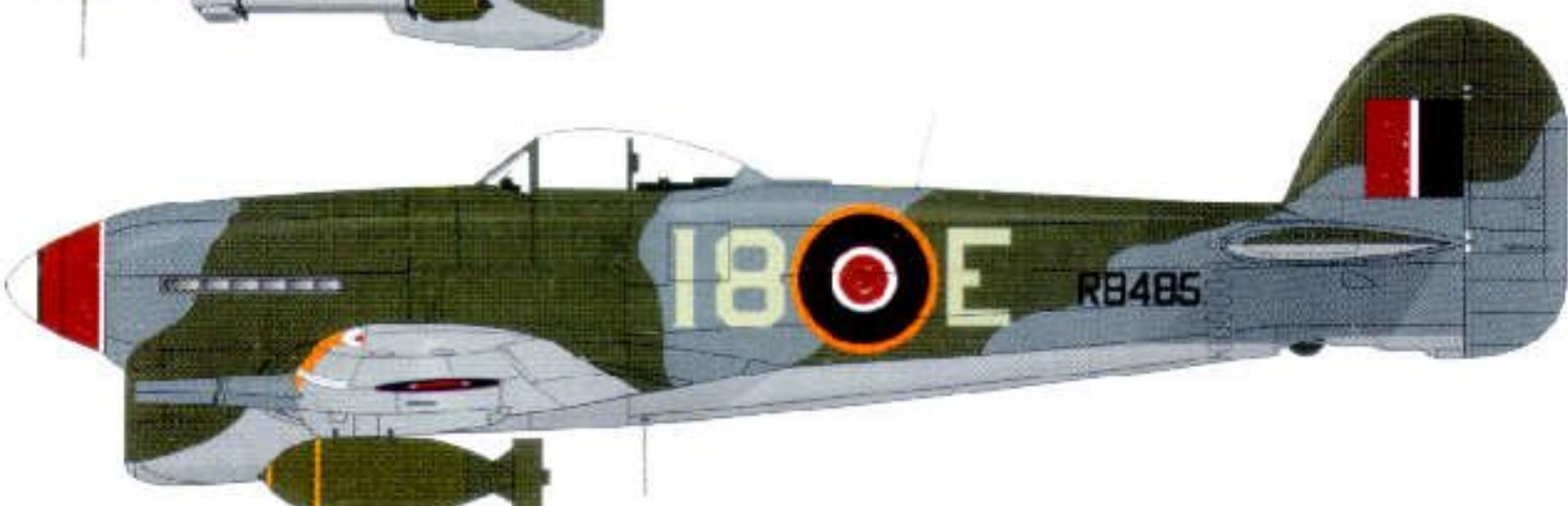
Typhoon IB RB485:IB-E of No. 440 Squadron, Flensburg 1945. Spinner red, tip white, red and white backplate. Tempest tailplane. Bombs only.
