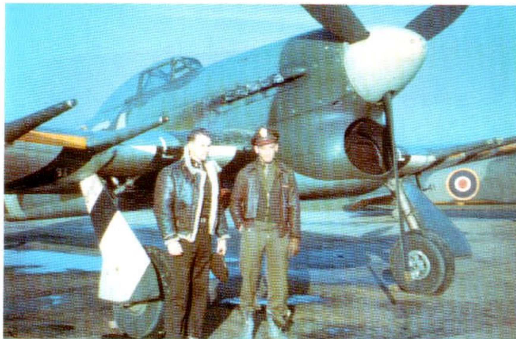
Left: Two USAAF pilots seen with visiting Typhoon JP488 SA-L of No. 486 Squadron RNZAF at Raydon, January 1944. Clearly visible is the exhaust fairing which featured on Typhoons delivered in late 1943. (Harvey Mace)
