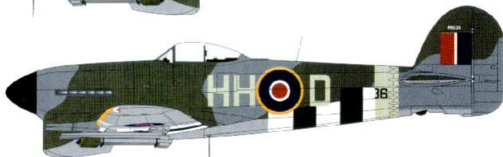
Typhoon IB MN536:HH-D of No. 175 Squadron, July 1944. Serial repeated in small white letters above fin flash. AEAF stripes on lower surfaces only. RP Mk.1 rocket rails.
