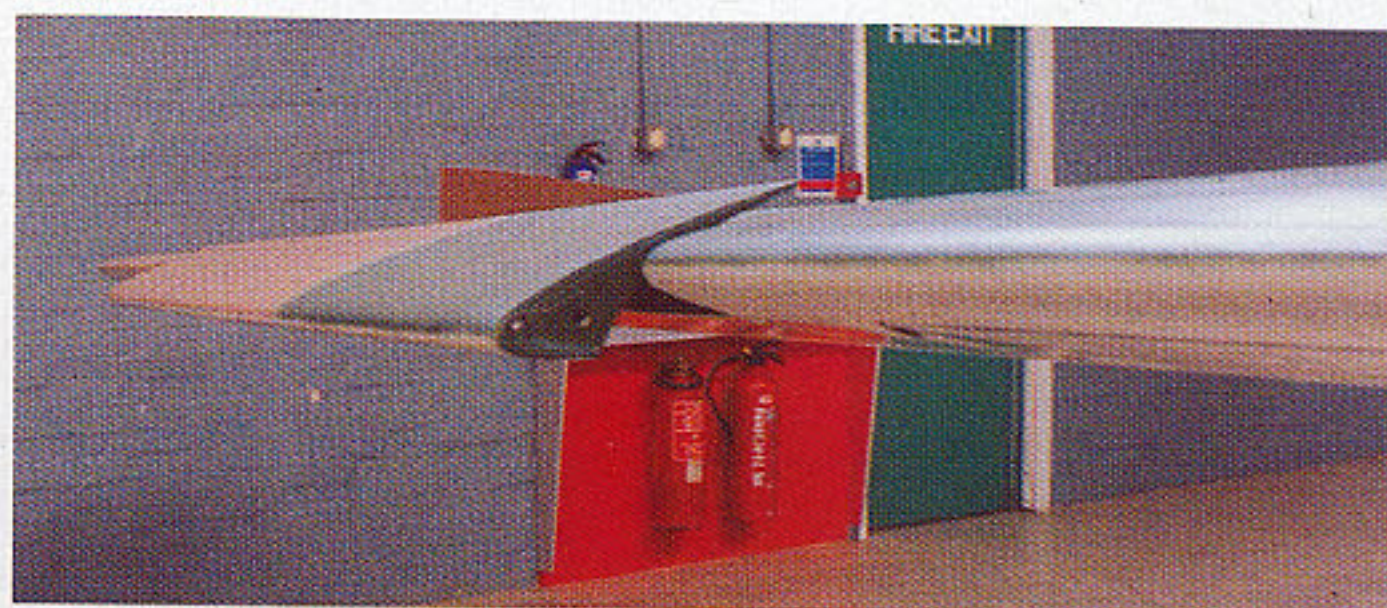
Above: The leading edge slats on the starboard wing. Left: One of the wing fences typical of later versions of the F-100D.
