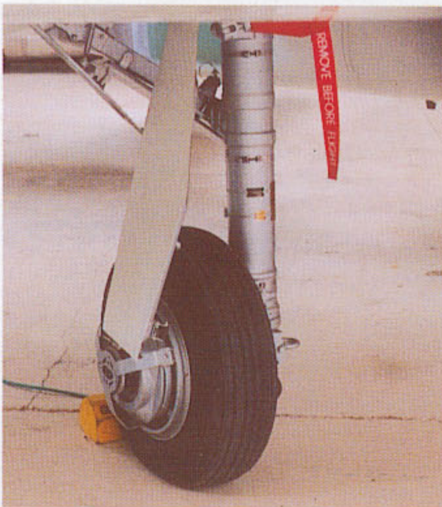
Main undercarriage leg, starboard side. 'Remove before Flight' tags were always inserted when the aircraft was parked.
