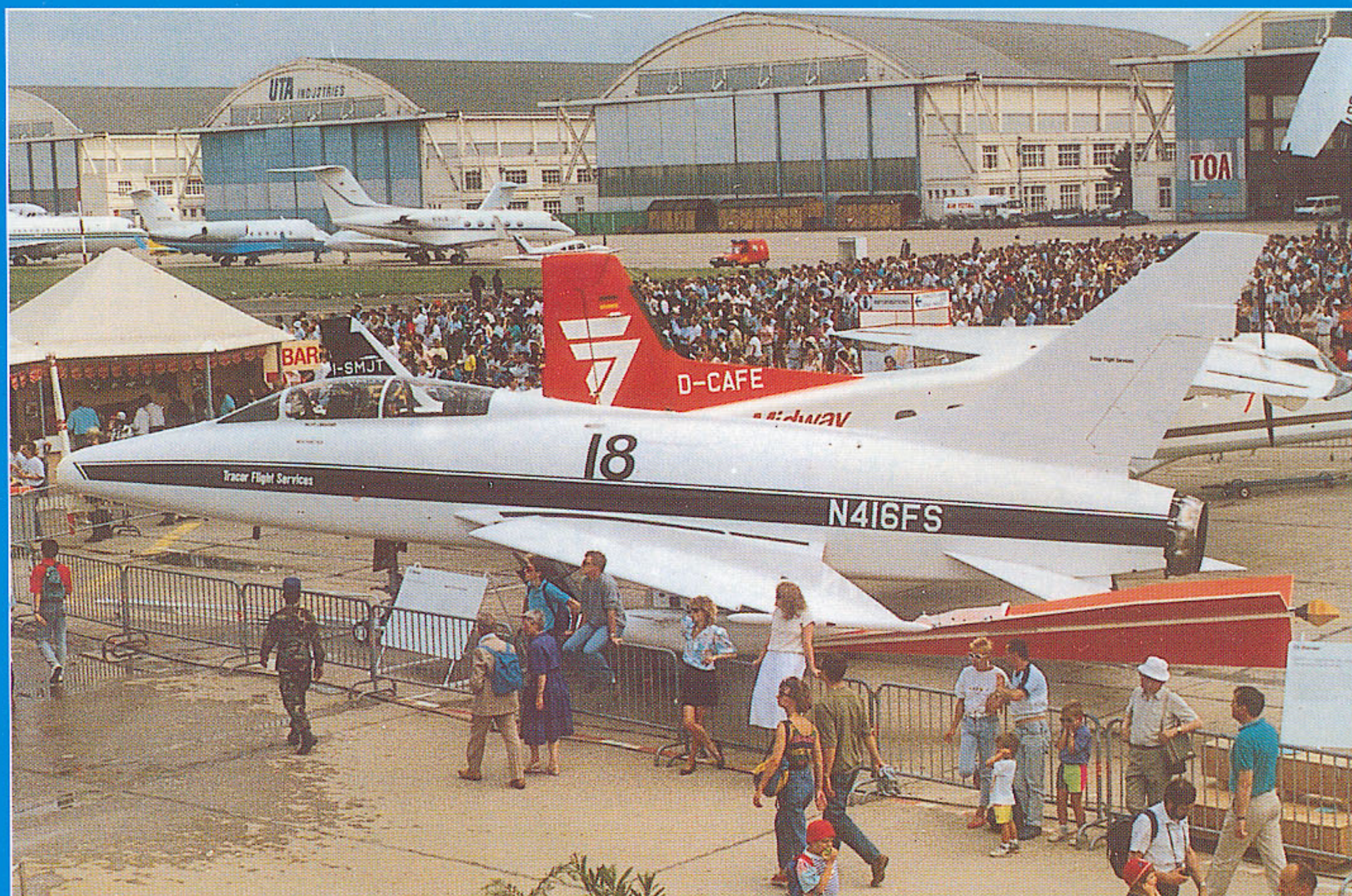
Above: A number of F-100Ds and Fs were converted for civil duties by two US-based companies, Flight Systems inc. and Tracor Flight Services. They were used for target towing duties. A total of 13 aircraft were given civil registrations including N416FS of Flight
