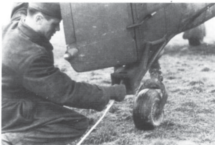
The Junkers Ju 87 was readily adapted for glider towing and as seen in the top view when used with a DFS 230A operationally or as a training glider. The Ju 87R-2 variant was favoured for this task because of its longer range, particularly useful when flying over the Mediterranean. Above: The glider towing attachment for the Ju 87 was dismantable and consisted of a simple box-like attachment that fitted to the aft bulkhead and could be quickly and easily installed under field conditions. This view shows a ground crewman fitting the towing cable in preparation for a launch. (Bundesarchiv)
