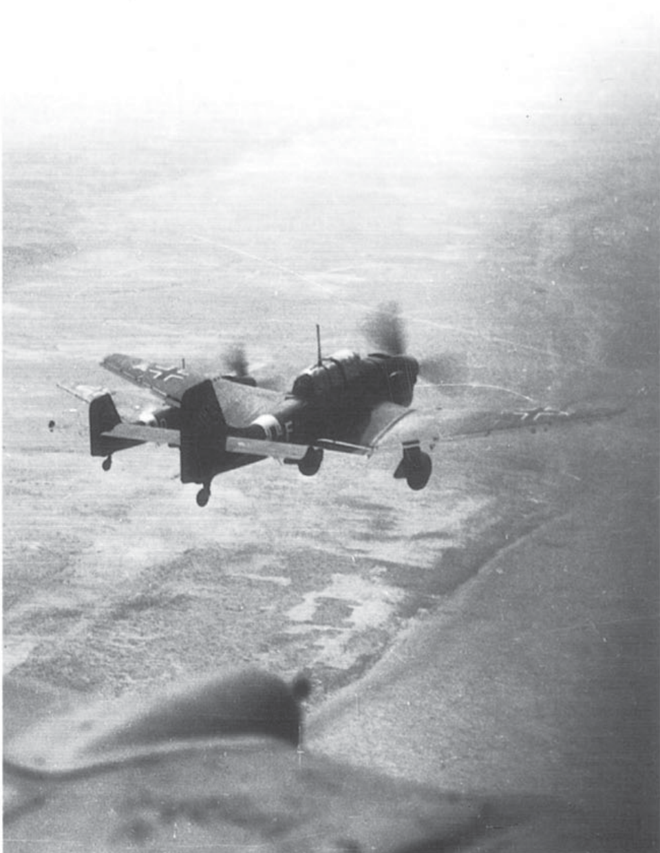
This interesting picture of a Junkers Ju 87D-1 of St.G 1 shows the trapeze bomb release under fuselage hanging down. The spinner appears to be painted in RLM 70, yellow, white and RLM 70 while the individual aircraft letter is repeated on the front of both spats. (Bundesarchiv)
