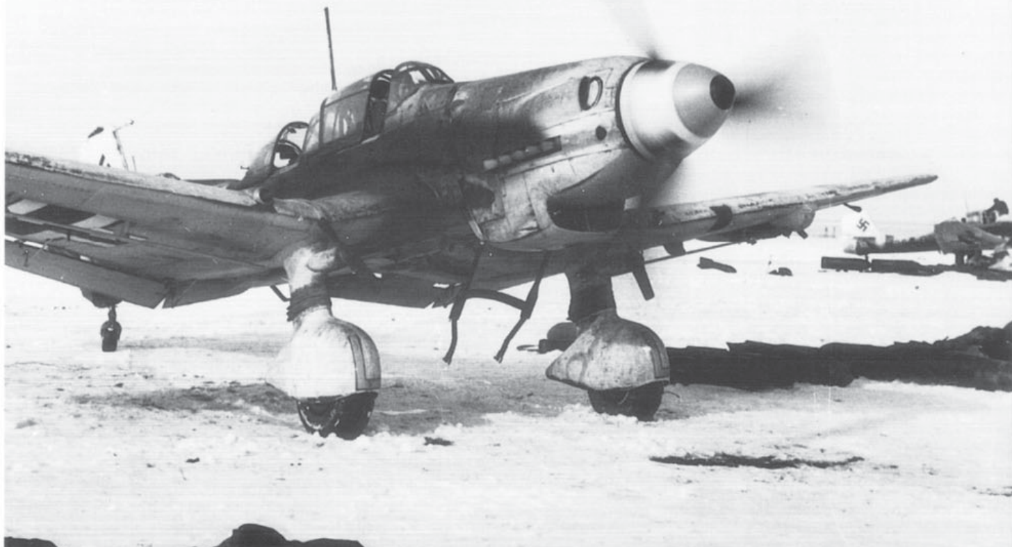
This interesting picture of a Junkers Ju 87D-1 of St.G 1 shows the trapeze bomb release under fuselage hanging down. The spinner appears to be painted in RLM 70, yellow, white and RLM 70 while the individual aircraft letter is repeated on the front of both spats. (Bundesarchiv)
