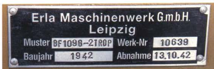
The aircraft nameplate, stating: Manufacturing Plant - Erla Machineworks of Leipzig; Model No. BF109G-2TROP (Tropical); Work No. 10639; Year Built - 1942; Factory Release Date - 13 October 1942.
