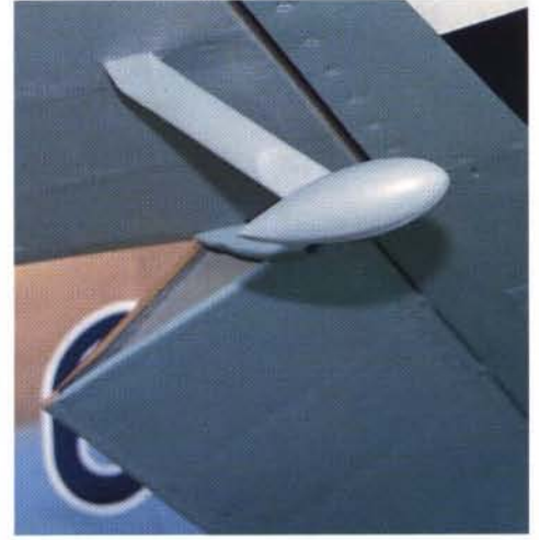
Starboard side mass balance located under the aileron.
