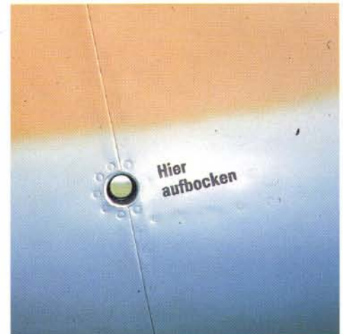
A tube could be inserted through this hole and used to lift the tail off the ground. "Hier aufbocken" translates to "Lift here". Circular hatch allows access inside the rear fuselage.
