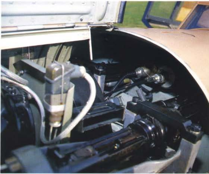
View of the MG17's 7.92mm with 500 rounds each.
