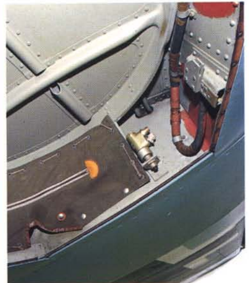
Port side view shows the zippered canvas dust cover. The hose is the radiator/flap shutter hydraulic line.
