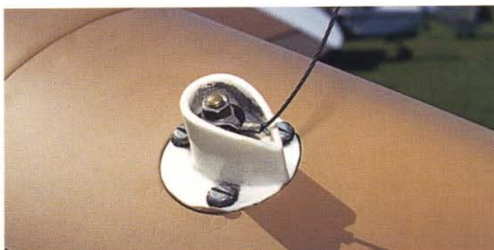
Aerial lead-in, offset to the port side located at the 5th bulkhead.
