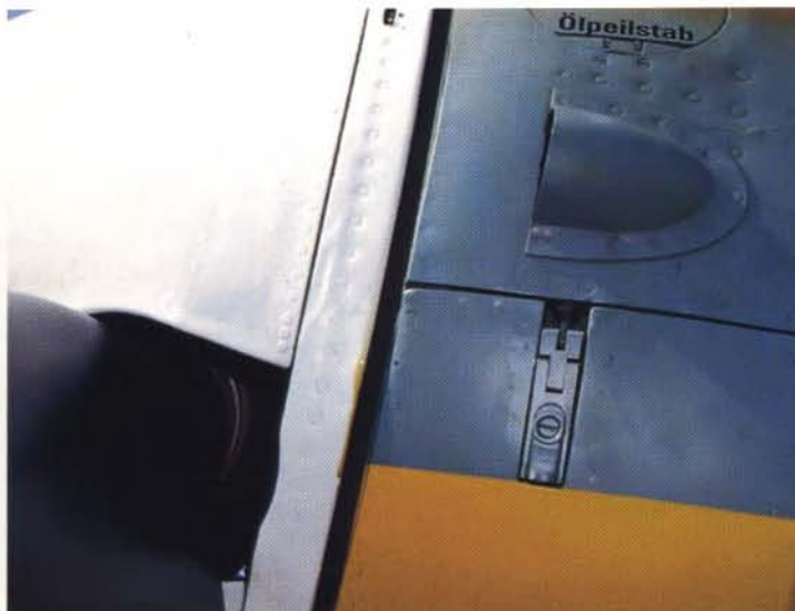
Closeup of the opening in the spinner. The prop on the Bf109G-2 is the VDM9-12087. On the cowling are the "Zu" fastener, engine cooling intake and oil filler hatch. "Ölpeilstab" translates to oil level indicator.
