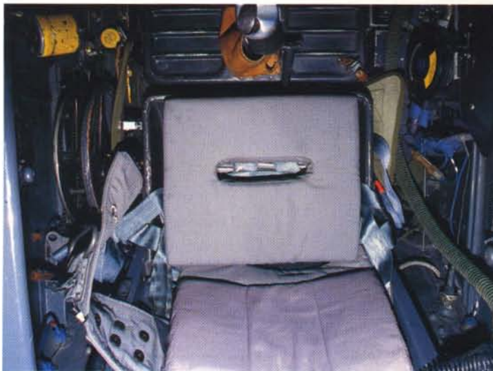
Pilot's seat. On the left are the landing flap control handwheel and to the right is the tailplane adjustment control wheel. Large yellow knob is the throttle lever; small yellow knob is the engine starter hand pump. On the right, in blue, are oxygen controls, hose and pressure gauge. The two small grey knobs on either side are the cockpit fresh air vents. Note they are staggered, starboard side slightly aft.
