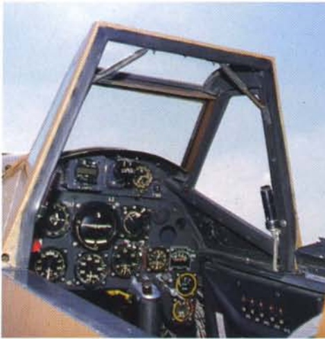
The colored rings around critical gauges give the pilot quick glance location.
