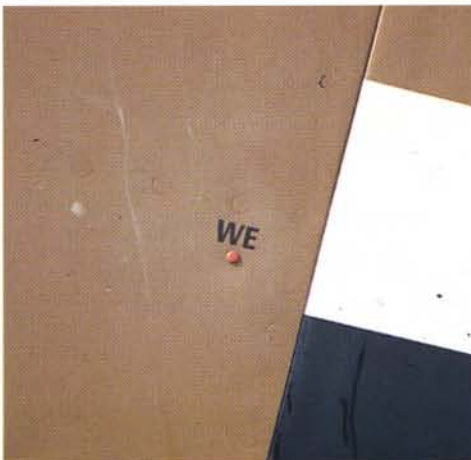
The marking "WE" is the fuselage horizontal datum. "WE" stands for "Waagerecht Einstellung". These are placed in five positions on the port side. They are used to line up the airframe in the "in-flight" attitude on the ground.
