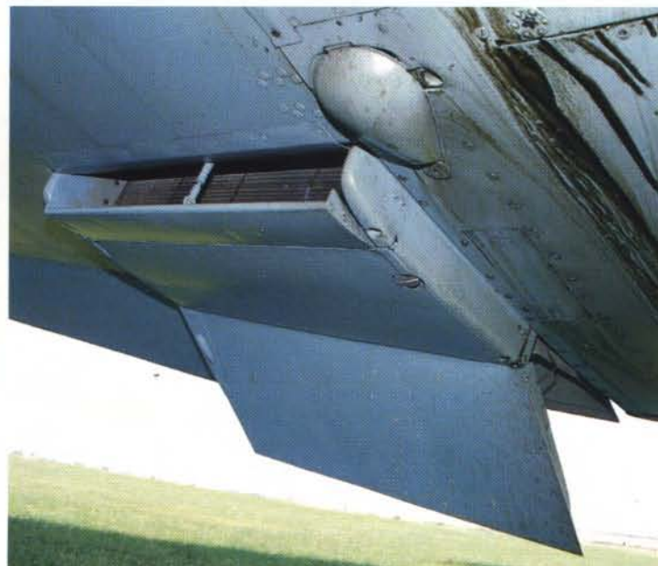
View of the radiator. The bulge covers the wing to fuselage attachment bolt. Note the oil streaks present on this meticulously maintained machine.
