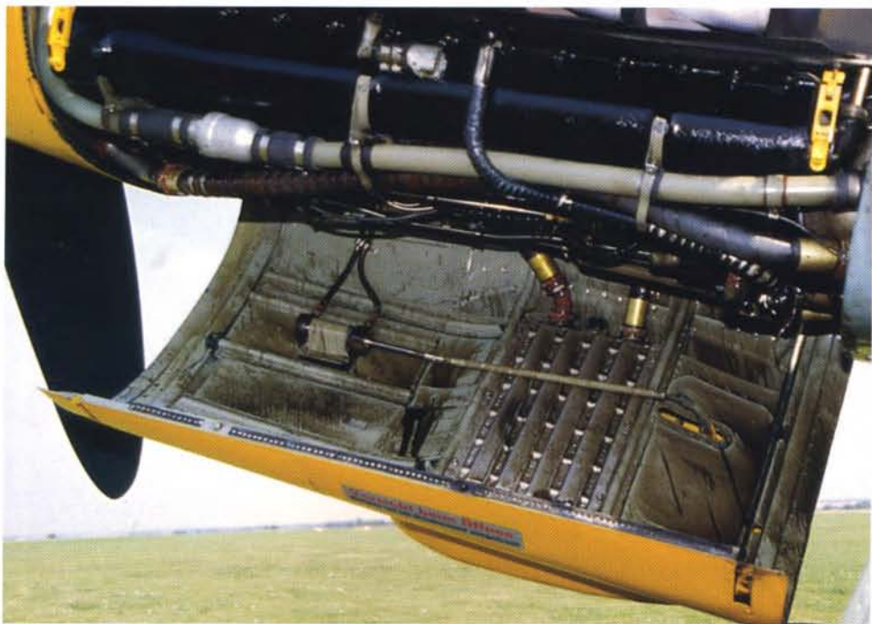
Locations of coolant hoses. On the lower panel are the hydraulic cylinder and actuating arm for the oil cooler shutter.
