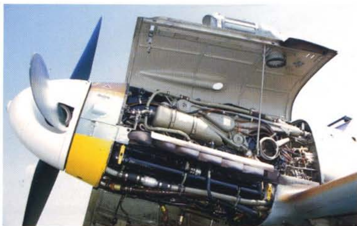
Locations of coolant hoses. On the lower panel are the hydraulic cylinder and actuating arm for the oil cooler shutter.
