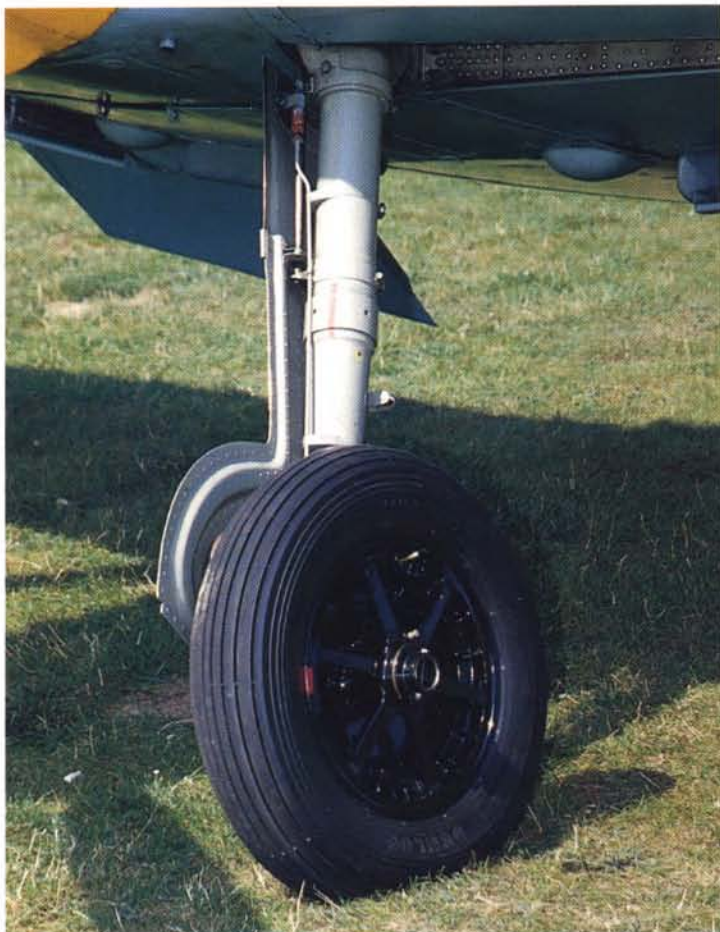
Port side landing gear showing brakeline. Main wheels are 660x160mm. Red mark is a wheel/tire slip indicator. Small tube is the coolant drain (both sides). The wheels are cast; later models had wider and machined wheels.
