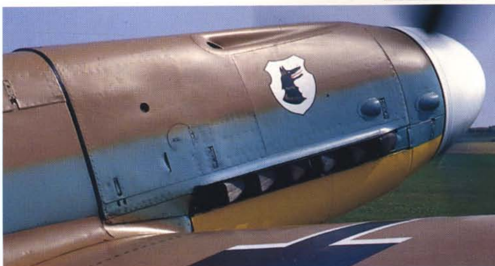
Here the engine crank is in position; below it the engine inspection hatch is visible. The starboard gun trough is for the MG17. Note the thick rubber gasket between the cowling and main frame.
