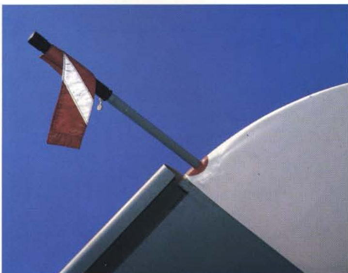
Closeup view of the pitot tube complete with protective boot and "don't bump your head" flag!
