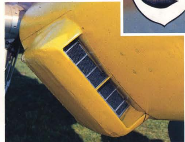
View inside the oil cooler.
