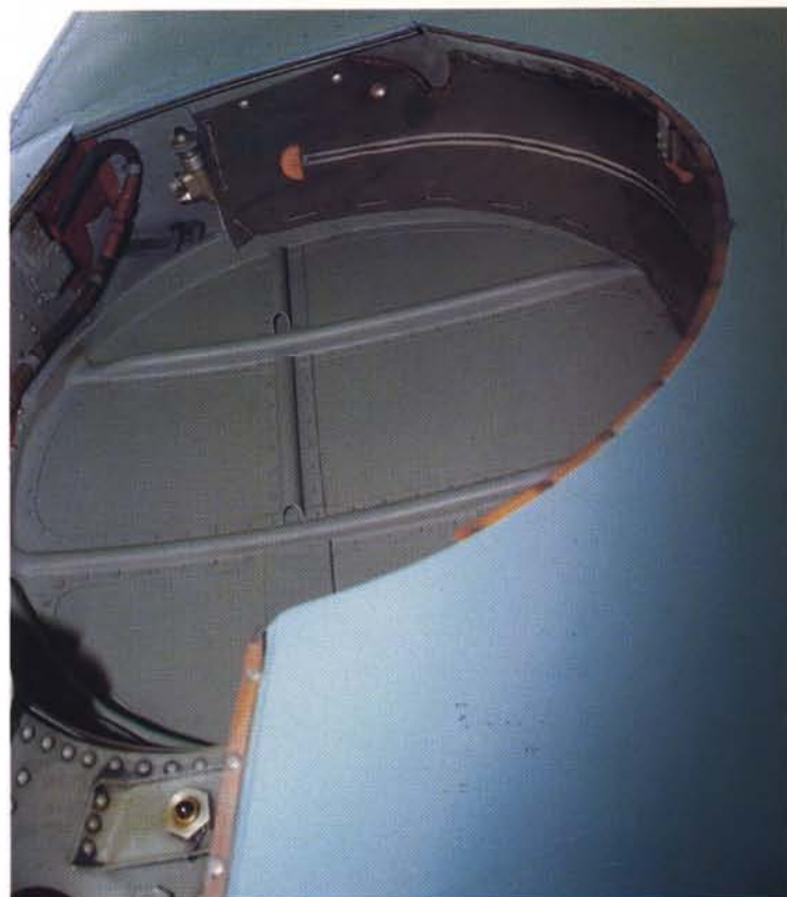
Port side landing gear showing brakeline. Main wheels are 660x160mm. Red mark is a wheel/tire slip indicator. Small tube is the coolant drain (both sides). The wheels are cast; later models had wider and machined wheels.
