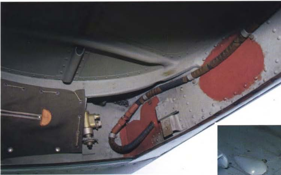
Closeup view of the radiator/flap hydraulic line. Note the oil and grease buildup around rivets even on this well-maintained machine.
