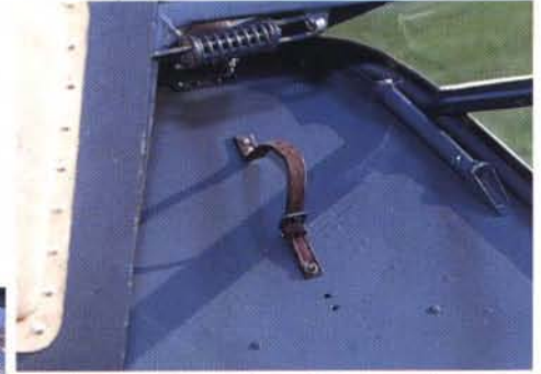
Canopy's spring-stop - pulling the leather strap accesses the personal storage bin.
