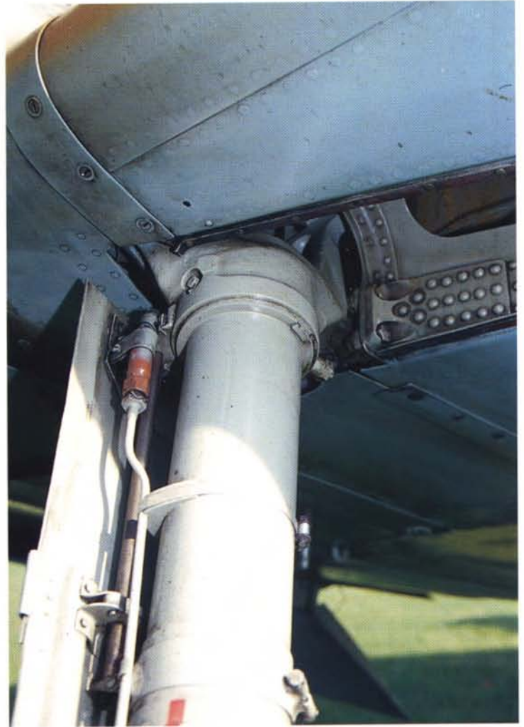
Port side landing gear attachment. The brake line and leather weather stripping are both visible. Note despite the fact this plane is in extremely clean restored flying condition, it has a fair amount of weathering around panel joints and rivets. This can be simulated with a wash of Raw Umber.
