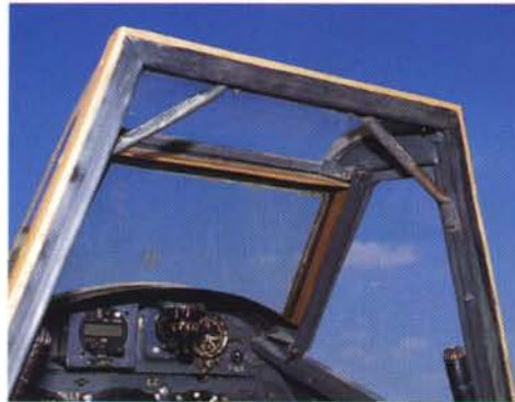
Above : The two angle bars are handholds. The front windscreen is 90mm thick bulletproof glass. Alongside the inside frames are the map reading lights.
