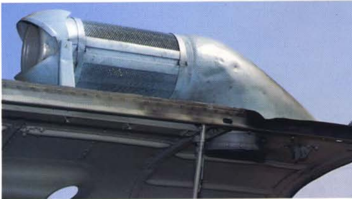
Nice view of the inside of how the supercharger intake seats onto the super charger. Note scorching from exhaust on the edge of the panel.
