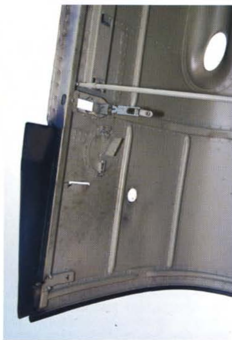
Inside view of port side cowl panel.
