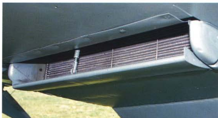
Radiators are set partially inside the wing to lower their profile. Actuating rod for the intake shutter can be seen. Circular hatch allows access to the radiator.
