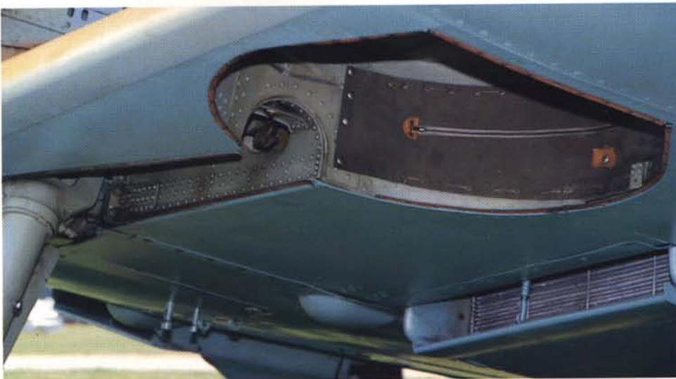
Port side landing gear wheel well, complete with canvas dust cover and leather weather stripping. Radiator can be seen with its raising and lowering aperture. The bulge beside it covers the wing fixing bolt. The two pipes are the fuel feed lines which connect the 300-liter drop tank.
