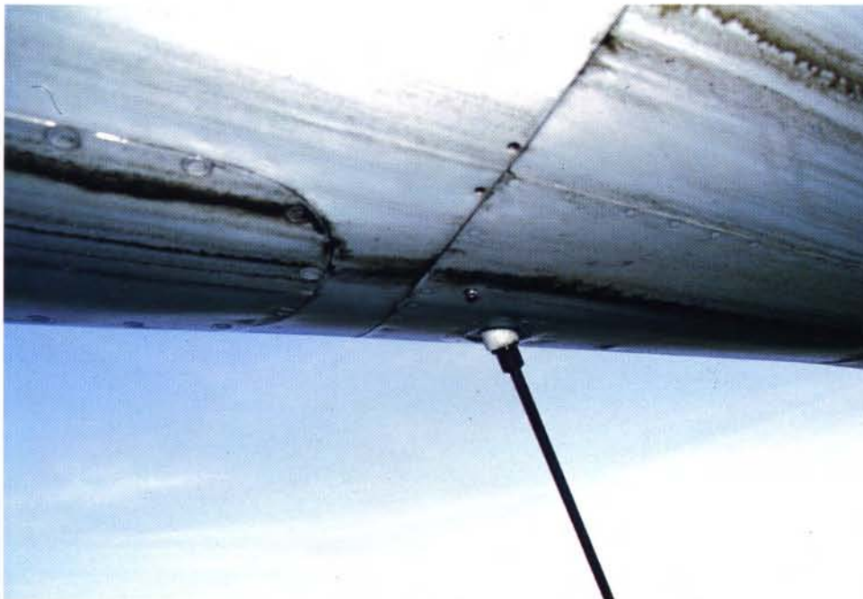
Closeup of the trailing antenna for the FuG25 IFF and the hatch to access the FuG IFF radio. Note how far the oil streaks traveled.
