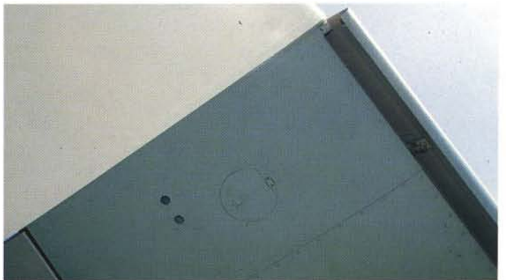
Starboard wingtip circular utility hatch. Note the Handley-Page gravity operated wing slats in the extended position.
