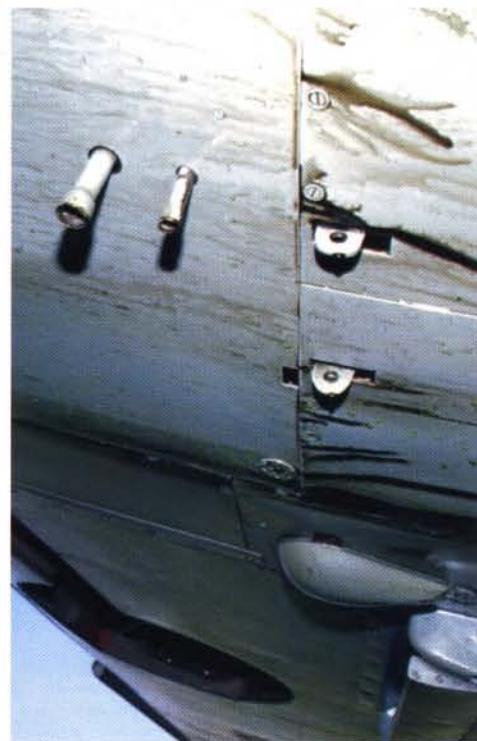
Closeup of the 300-liter drop tank fuel lead-in tubes. The attachment hooks for the ETC 500 rack are visible.
