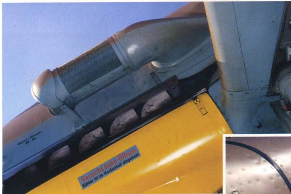
Here is an excellent view of the early mesh type tropical filter. Note the weld seams on the exhaust pipes. The text on the lower cowling reads (top line in red) "Caution Upon Opening"; the lower black line reads "Cooler is built into cowling section".
