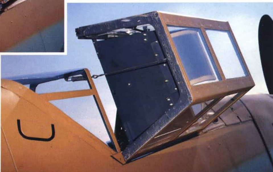
The frontal windscreen boasts 90mm bulletproof glass.
