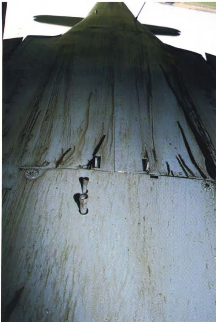
Underside view showing the two tubes which connect the 300-liter drop tank. Note the oil streaks that traveled in the slipstream, a fair amount of weathering especially for a well maintained airplane. Imagine a late war aircraft when cleaning and appearance were not a priority!
