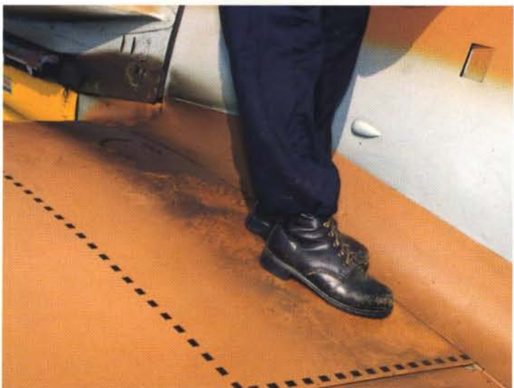
The dashed lines, sometimes in red, indicate areas where walking is allowed. The hatch behind the crewchief's feet is the ammunition supply hatch for the 20mm coaxial MG151/20 cannon.
