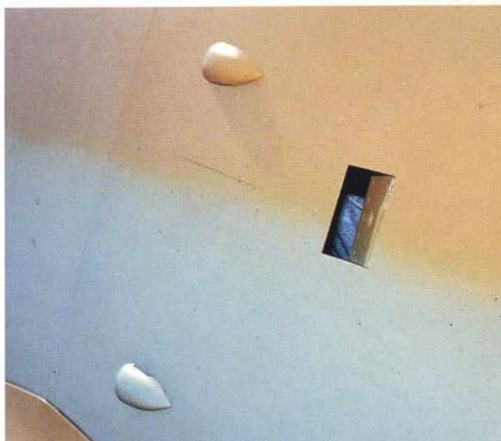
The two teardrop shapes are the parasol mounts found on tropical versions. The small door is a fresh air inlet for the cockpit port and starboard, sometimes port only, sometimes none at all.
