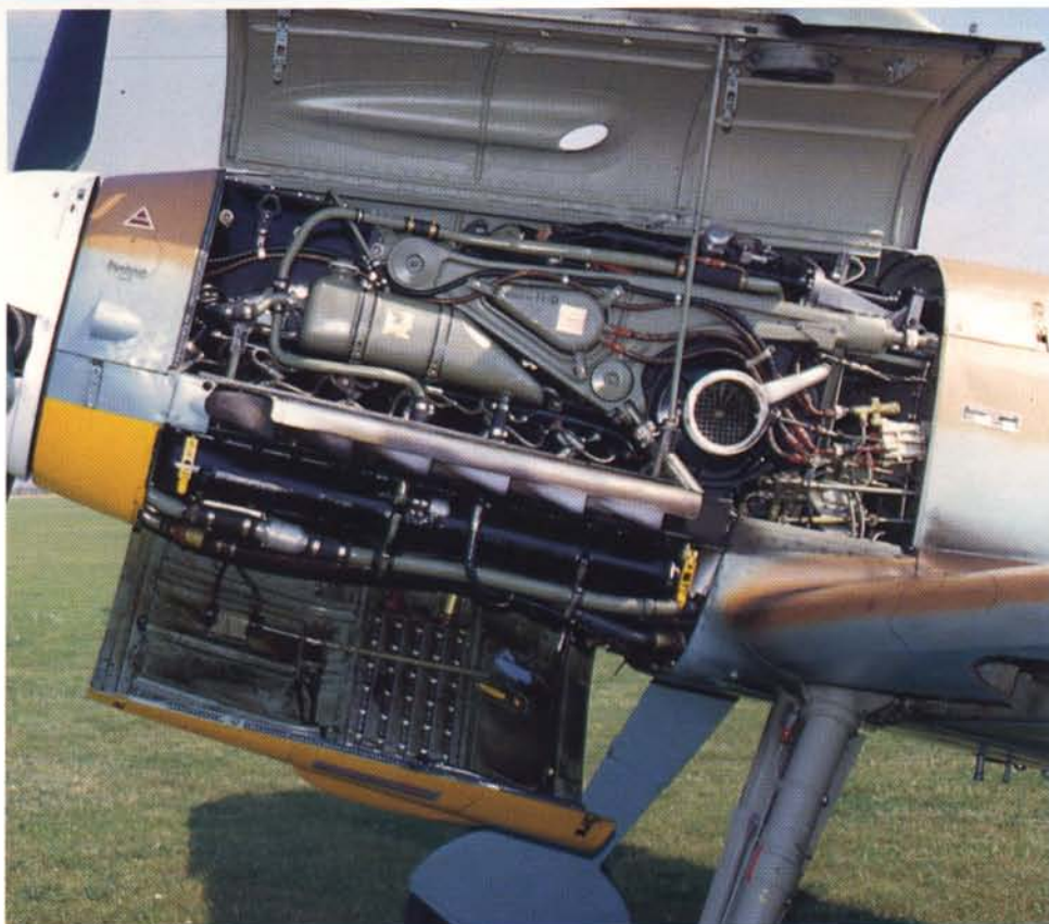
A handy resource for modelers on the location of hoses and wires. Note the oil-covered lower cowl panel.
