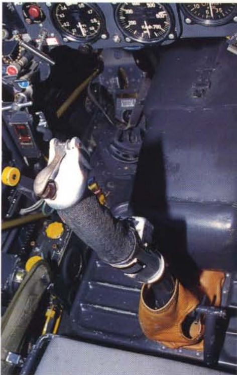
Closeup of the control column shows the trigger for the coaxial MG 151/20 on top of the grip. Cockpits were painted in RLM 66 Schwarzgrau.
