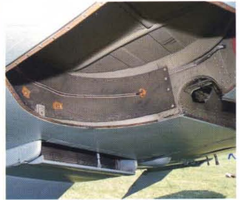
Closeup of the starboard wheel well with the canvas dust cover and leather weather stripping. The intake doors of the radiator are shown in the lower position for maximum airflow. The two circular hatches access the radiator for maintenance.
