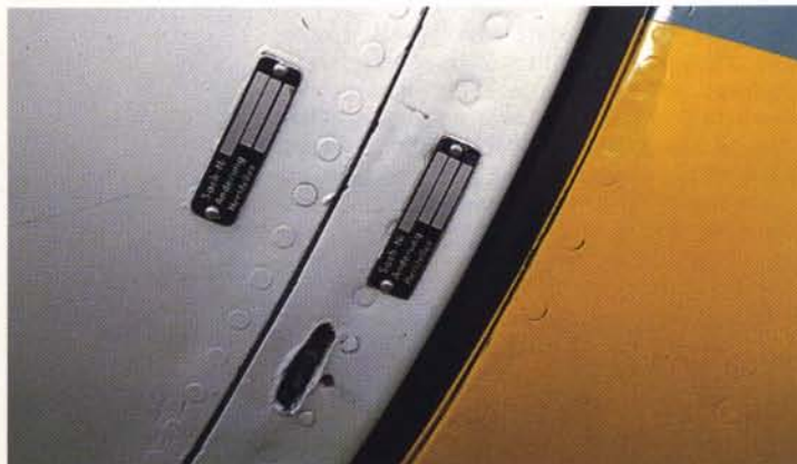
Closeup of nomenclature tags on the front and back plate of the spinner. Note the flush rivets that give Messerschmitts their sleek skin. Closeup also shows one of the cowl's "Zu" fasteners.
