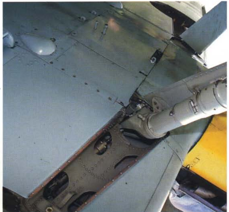
Here the two large bulges cover the bolts which connect the wings to the fuselage. Visible in the landing gear troughs are the hydraulic cylinders that raise and lower the landing gear. The two pipes in the middle are the fuel feed and fuel vent lines which connect the 300-liter drop tank. Behind them are the attachment points for the ETC 500 rack.
