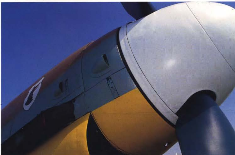
Closeup of one of the four scoops added to the G-series in order to help cool the engine. Mismarked on this example the red and white triangle should indicate "Oil Filler"; instead, it shows a water methanol filler marker.
