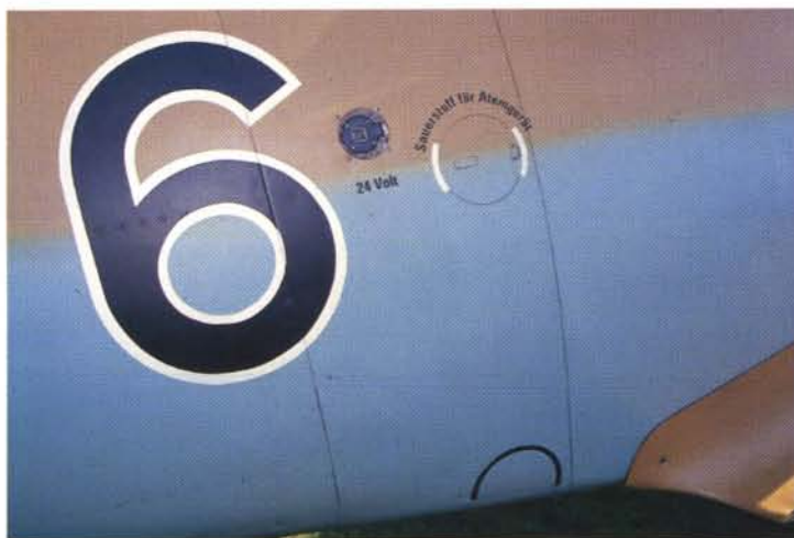
Starboard side: Half-moon is a hinged footstep. The large circular hatch marked "Sauerstoff für Atemgerät" translates "Oxygen for Breathing Apparatus". Sometimes also printed underneath was "Vor Anschluß ab ol u Fett", translated "Before connecting remove oil and grease". The hatch is sometimes painted blue and white. Behind the smaller hatch is the power socket, normally painted in red and marked 24 volts.
