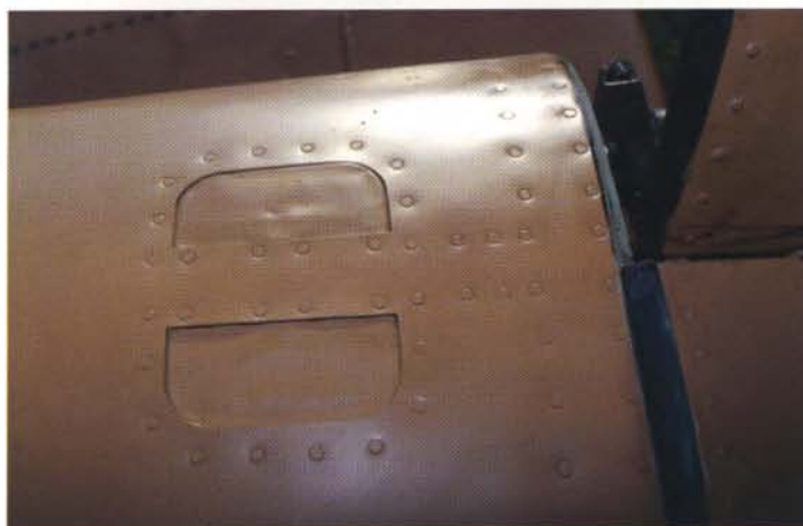
Located on the top of the fuselage, just ahead of the windscreen, are the hinged handholds for hoisting one-self up.
