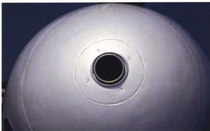
Closeup of spinner: In the center, you have the business end of the coaxial 20mm MG151/20 cannon that fires through the center of the crankcase in the engine.
