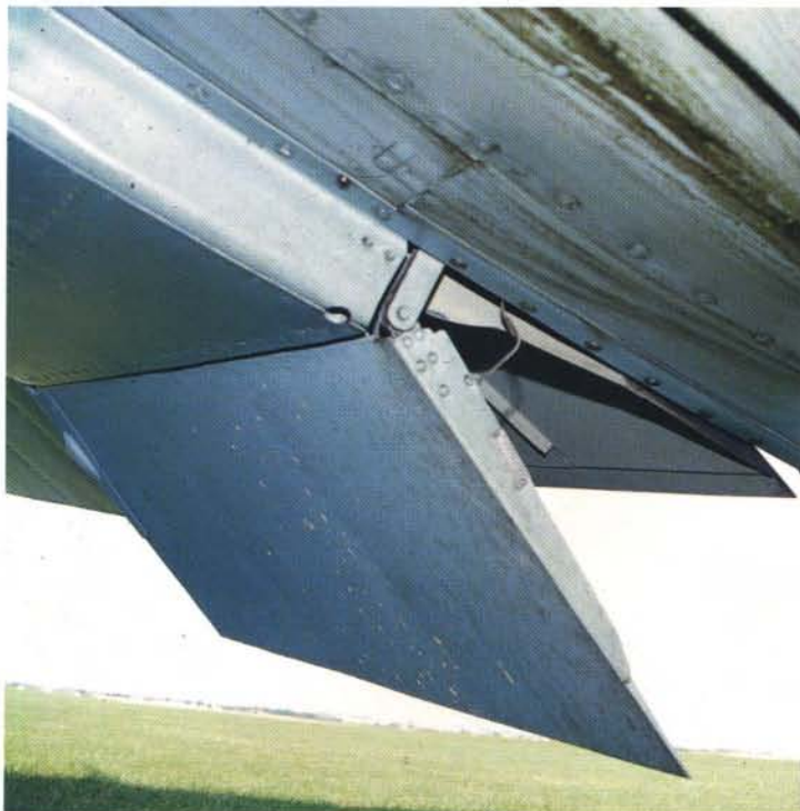
Closeup of the radiator/flap shutters. Note the oil streak dragged to the rear of the plane by the slipstream.
