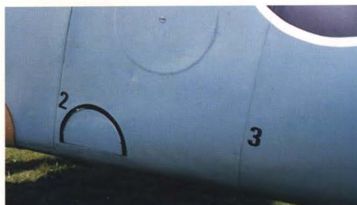
Port side, rear wing root and fuselage: The half-moon hinged panel is sometimes marked "Einstiegklappe", translated "step-board". The black numbers mark fuselage frames. The circular hatch accesses the master compass.
