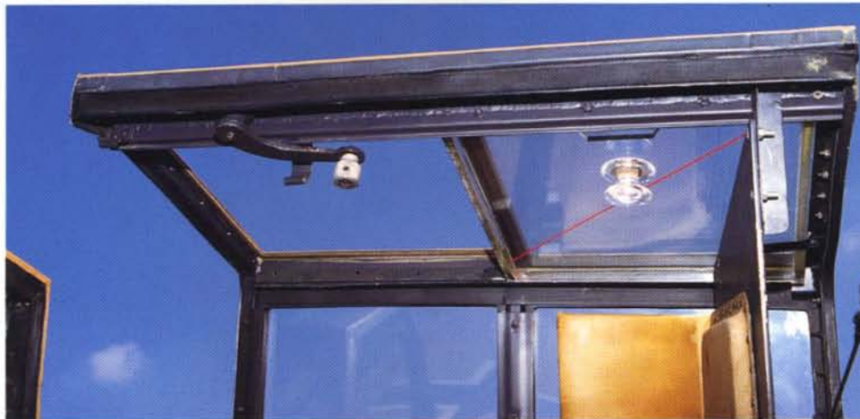
Canopy release lever, armored headrest attachment and sliding glass panes.
