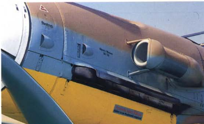
The cowling was space efficient and wrapped tightly around the engine.
