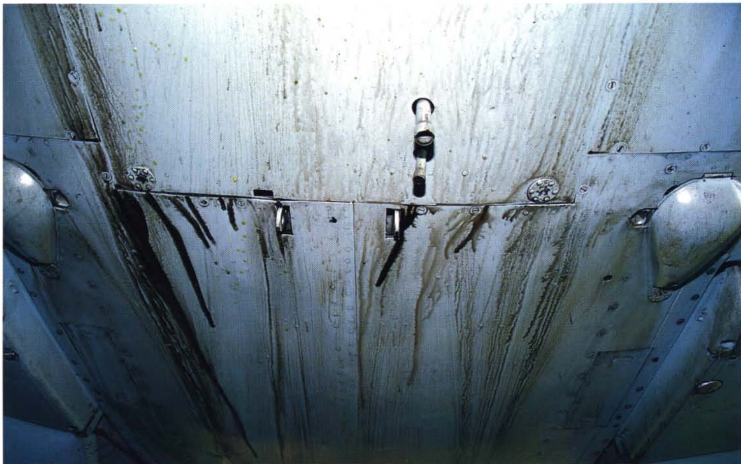
Pipes for the 300-liter drop tank and two hooks to attach the drop tank rack. The two large bulges cover the wing to fuselage bolts. Note the oil streaks.
