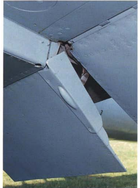
Radiator shutter hinge points.
