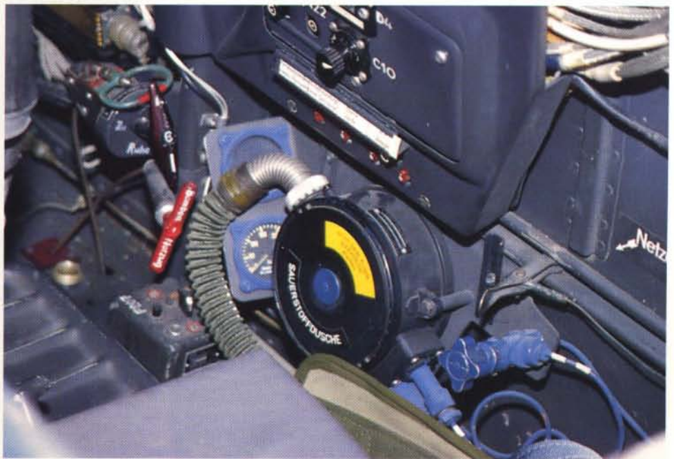
Closeup of the oxygen system: hose, (top gauge) oxygen control indicator, (bottom gauge) oxygen pressure indicator. Blue knob is the oxygen cut-off valve. Note blue tubing indicates oxygen lines. The small lever above the cut-off valve is the "Netzeinschaltung", translated "Main power switch". Red handle is the radiator flap lever; below is the radiator cut-out handle. Below the red handles on the floor is the frequency selector for the FuG 16 radio. Above the oxygen system is the control panel for the FuG 25 IFF.
