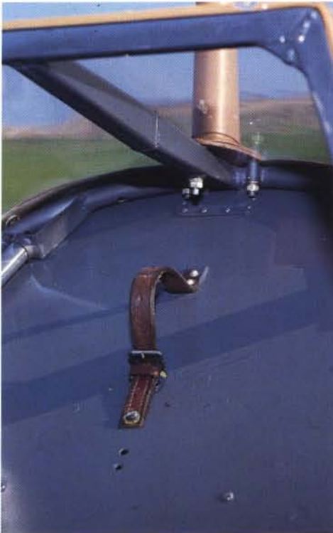
Closeup of the antenna mount, spring-loaded catch and leather strap to access the storage compartment.
