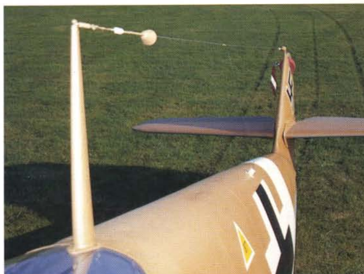
Antenna mast for the FuG16 radio. Tail fin is airfoil shaped in cross-section with the port side rounded and starboard flat.
