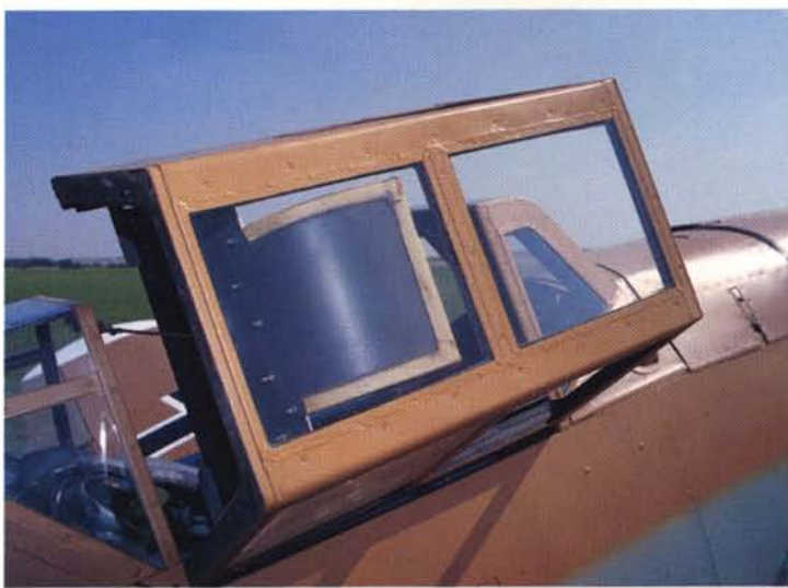
Top view of the canopy. Note the crude weld seams.
