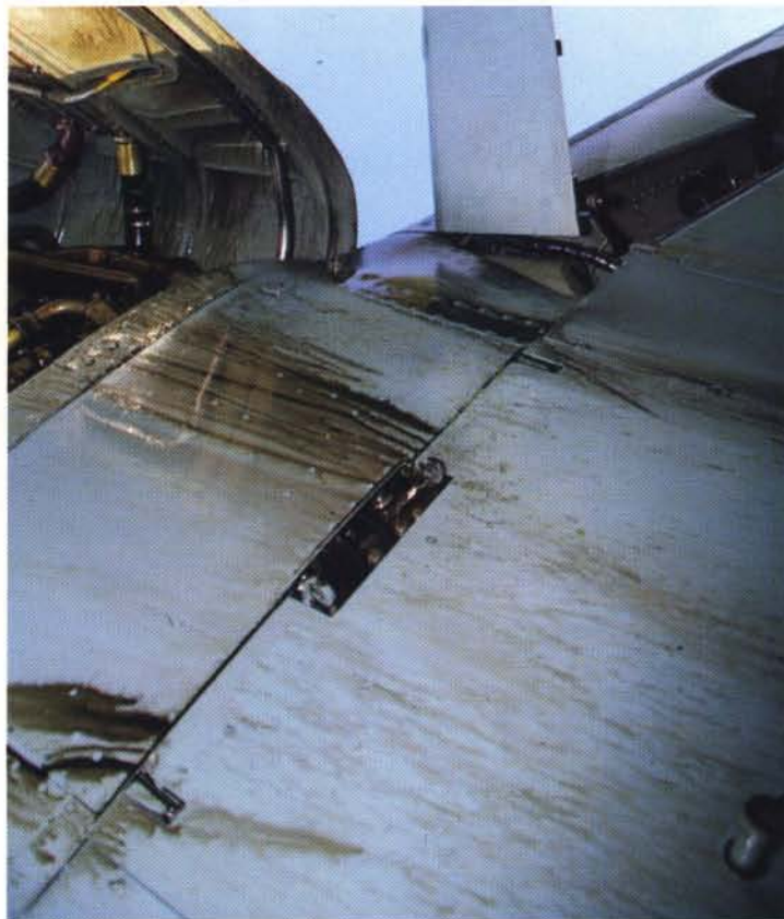
Messerschmitts from early on were notorious for their oil leaks and this pristine example is no exception.
