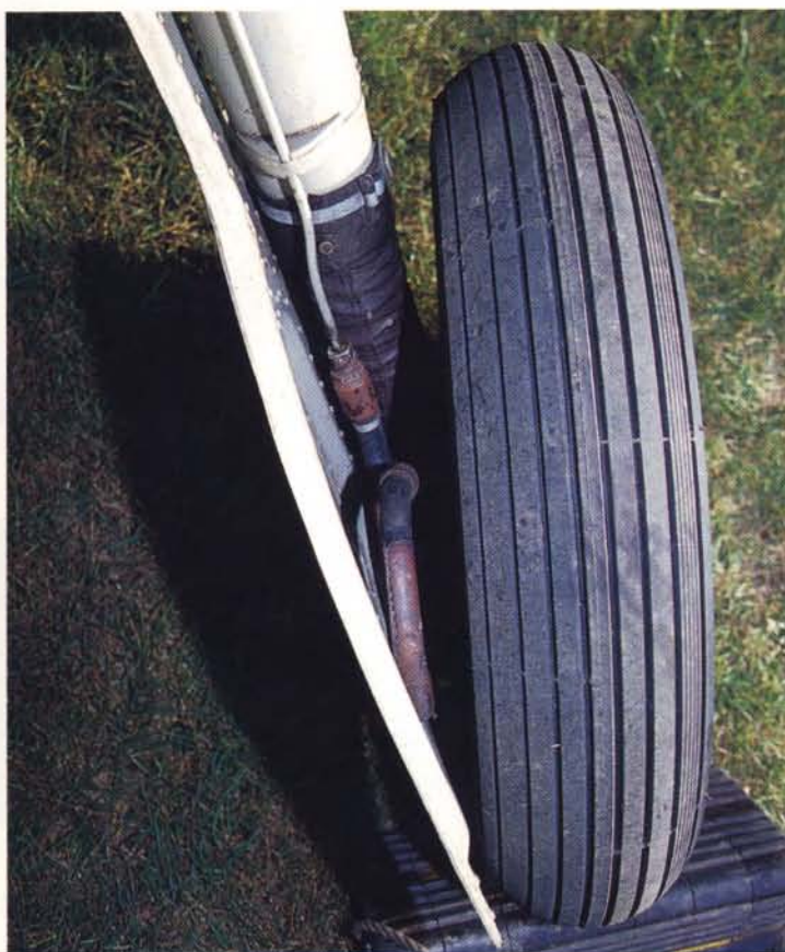
Top view of the tire. Note the leather-covered brake line and rubber sleeve covering the oleo.
