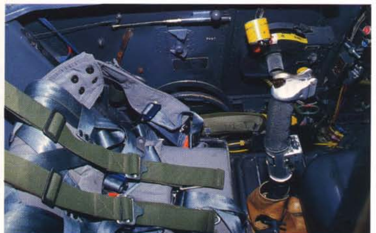
Port side view from the top is the tailwheel lock mechanism, fresh air inlet, engine throttle (yellow knob) and flap and trim wheels.
