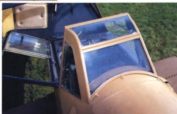
The frontal windscreen boasts 90mm bulletproof glass.
