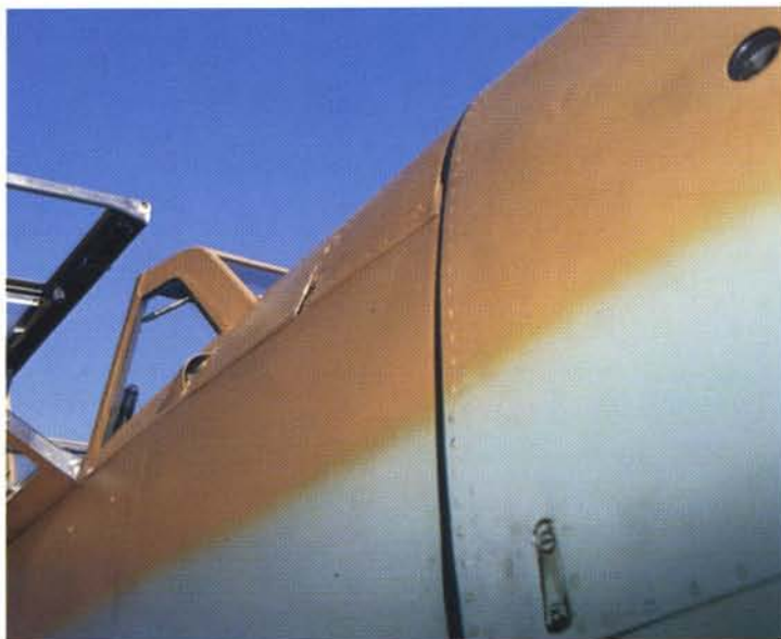
Insertion hole for engine starter crank; below it is a cowling latch. Below the front windscreen is the cockpit air intake.
