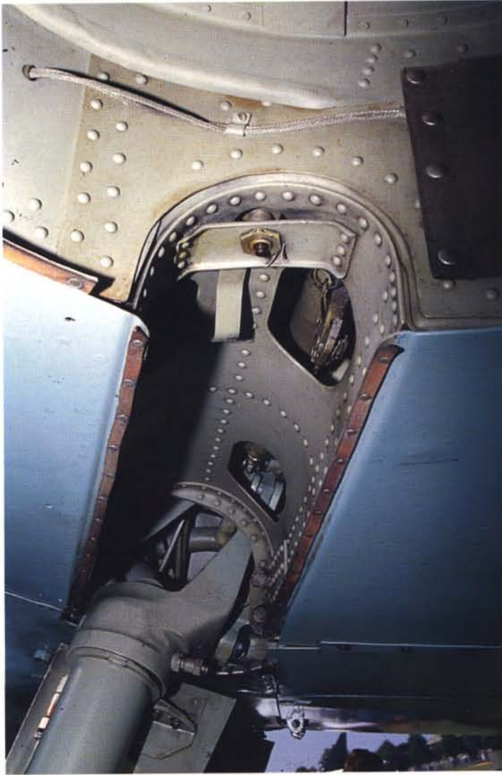
Port side landing gear attachments: locking mechanism, brake line, leather weather stripping are all visible. The pitot tube wires are visible.
