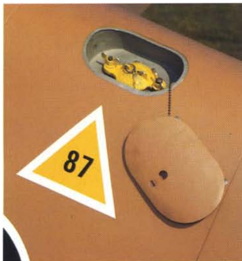
Filler hatch for the fuselage tank (400 liter). The yellow triangle indicates octane and grade: 87 octane and "B4" fuel type.
