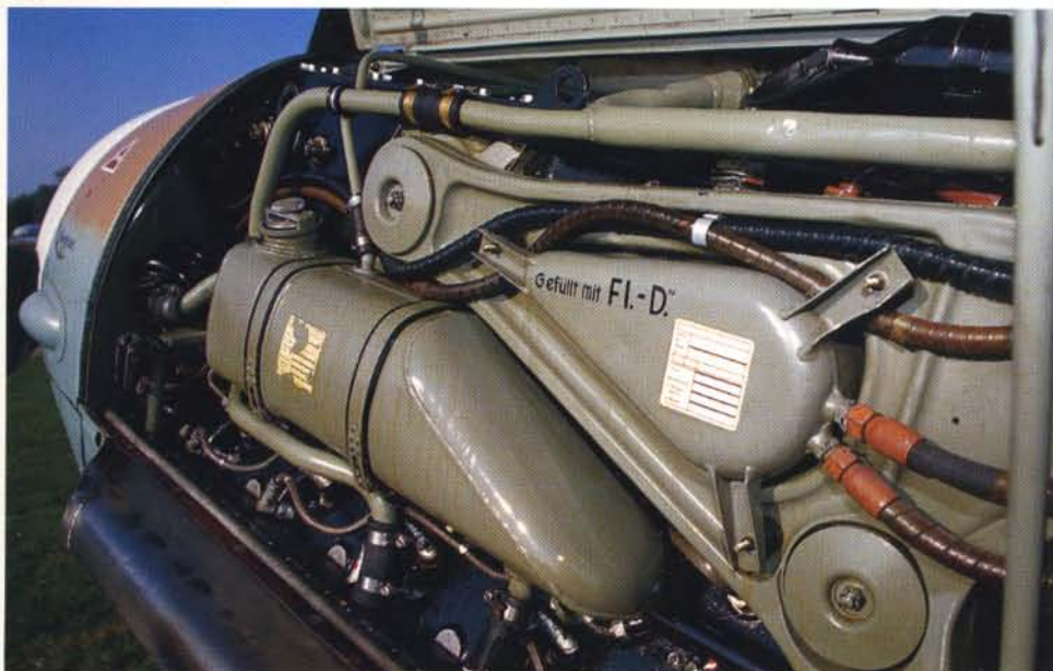
Closeup of the hydraulic reservoir and coolant reservoir. Barely visible at the extreme front inside is the 36-liter oil tank. At the bottom, the ignition wires are visible.
