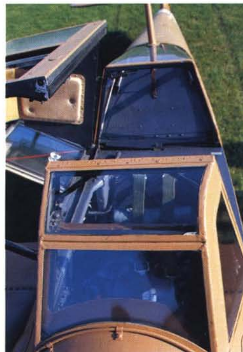
The small tube running the radius of the windscreen dispenses washing fluid.
