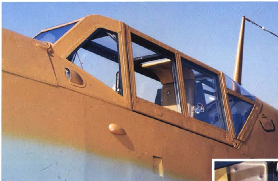
The "G" series introduced heavier canopy framing.
