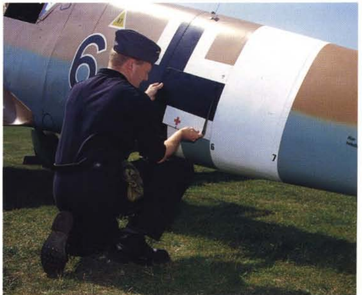
The "Blackman" removes the fuselage panel which accesses the radio and compass. Survival gear and Kar98k rifle are also commonly stored on tropical aircraft in, case of emergency landing in the barrens. The red cross denotes storage of a medical kit.
