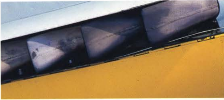
Closeup of piano hinge that attaches lower cowl.
