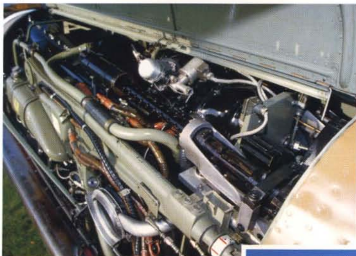
Locations of coolant hoses. On the lower panel are the hydraulic cylinder and actuating arm for the oil cooler shutter.
