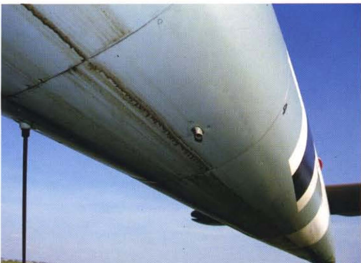
On the #3 bulkhead, the fuel vent is on the port side. On the starboard side, the FuG25 IFF antenna. Note how far the oil streaks reach!
