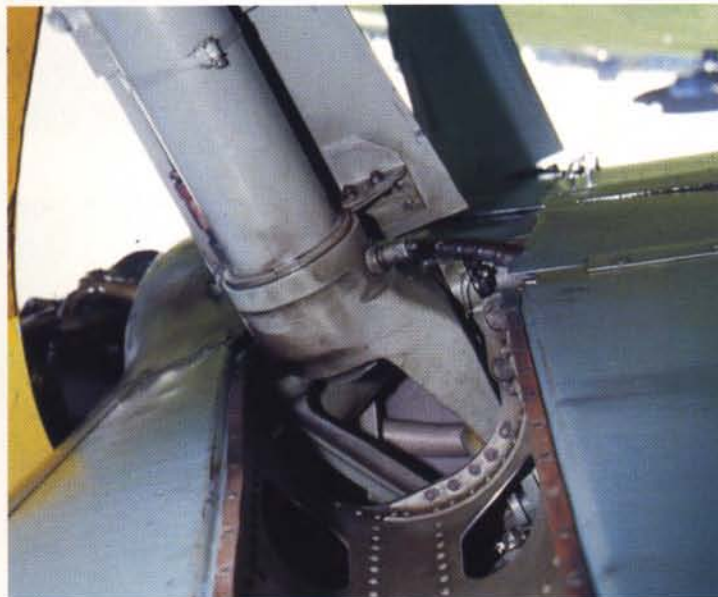
Above : Starboard landing gear attachment point. Brake line is visible. Note the leather weather stripping along the sides.
