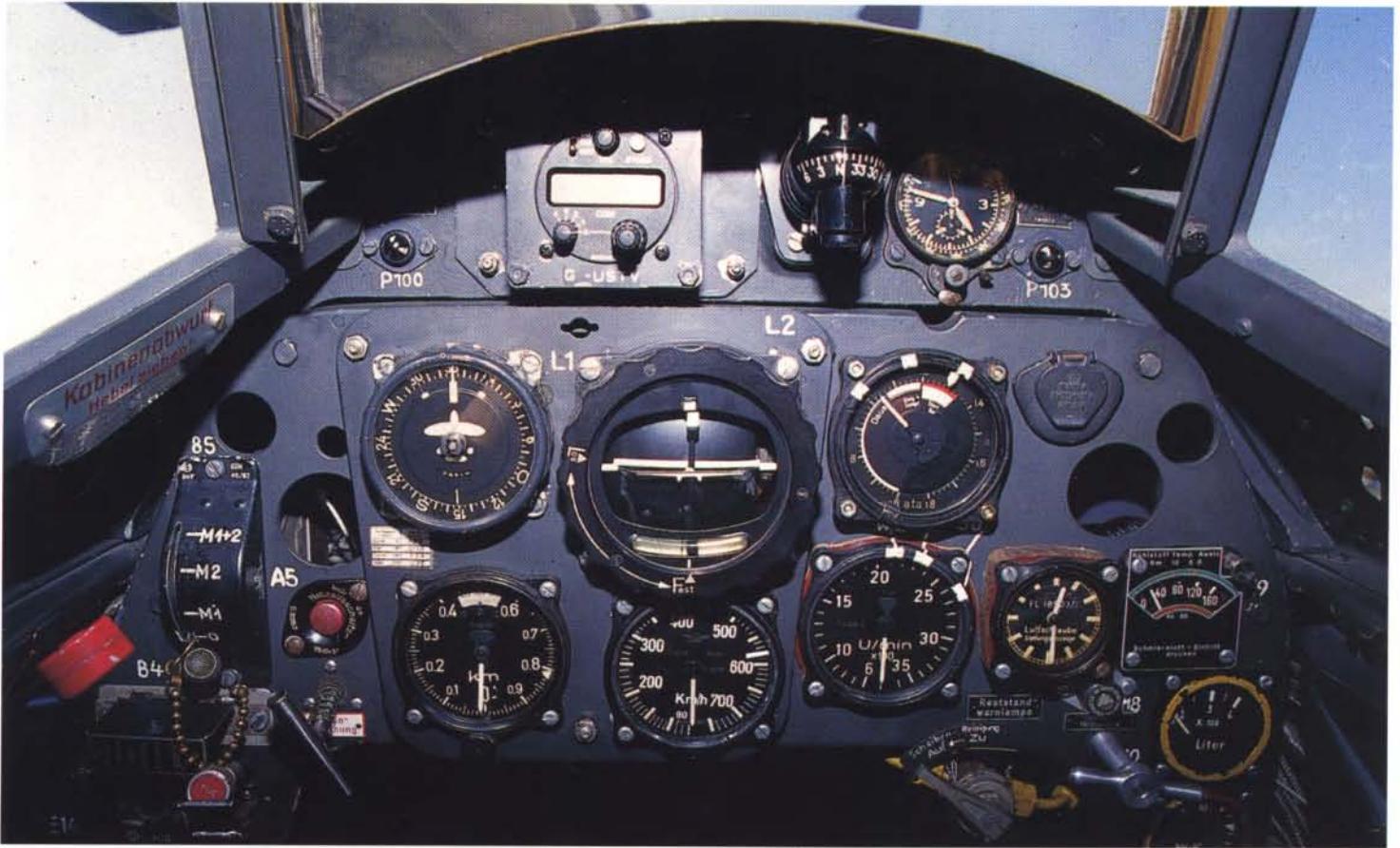
Instrument panel (from top left to right): modern instrument in place of ammunition counter; modern compass in place of Revolver 16B gunsight; aviation clock; (middle) compass; artificial horizon; tachometer; (bottom) magneto switch, circuit breaker, airspeed indicator, altimeter, super charger pressure gauge, propeller pitch indicator, fuel and oil temperature indicator, fuel gauge, fuel & oil pressure gauge.
