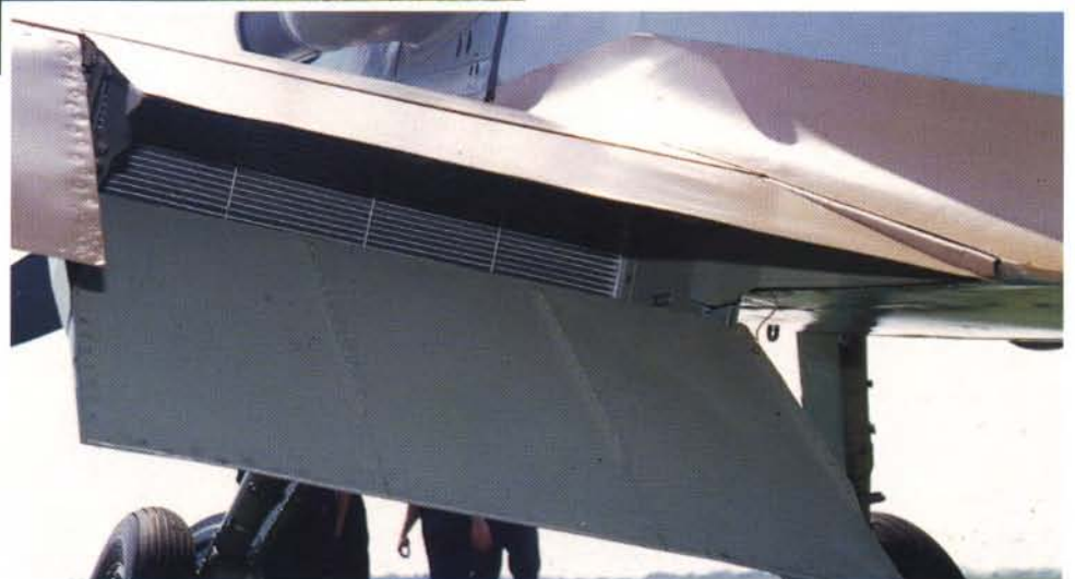
Radiator shutter hinge points.
