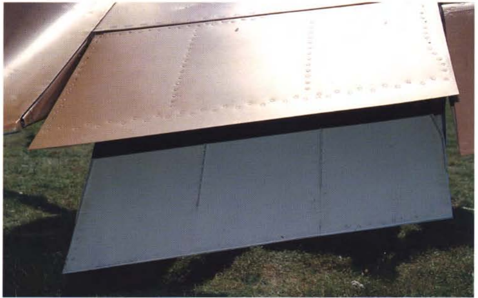
The split flaps that function as radiator shutters and supplemental landing flaps.
