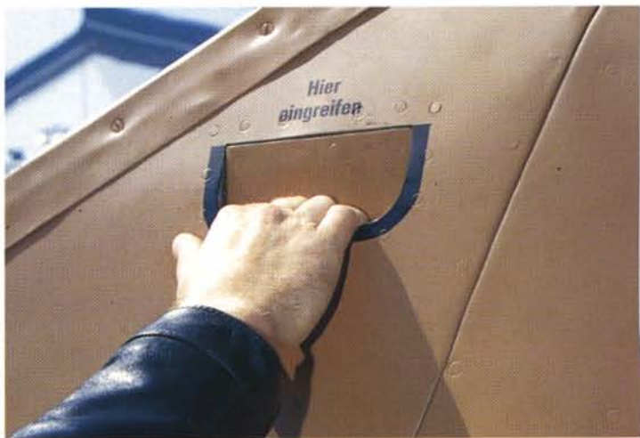
Hinged handhold to climb aboard both port and starboard. "Hier Eingreifen" translates "Grip Here". Note the 'flush rivet' surface.
