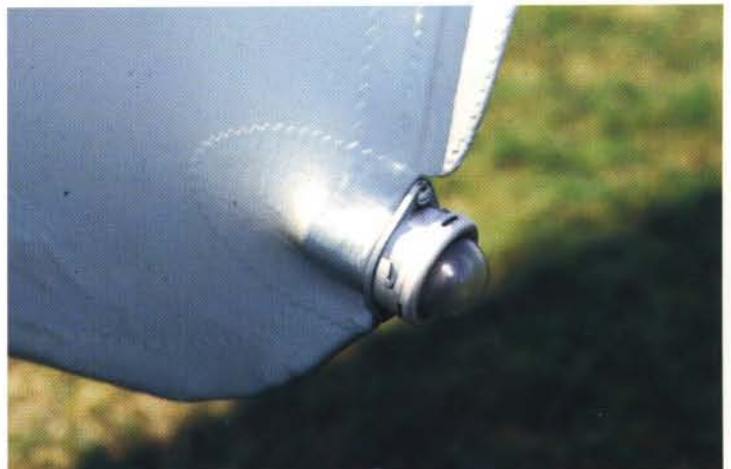
The tail light. Modeler's note: This can be replicated with a small droplet of clear 5-minute epoxy glue.
