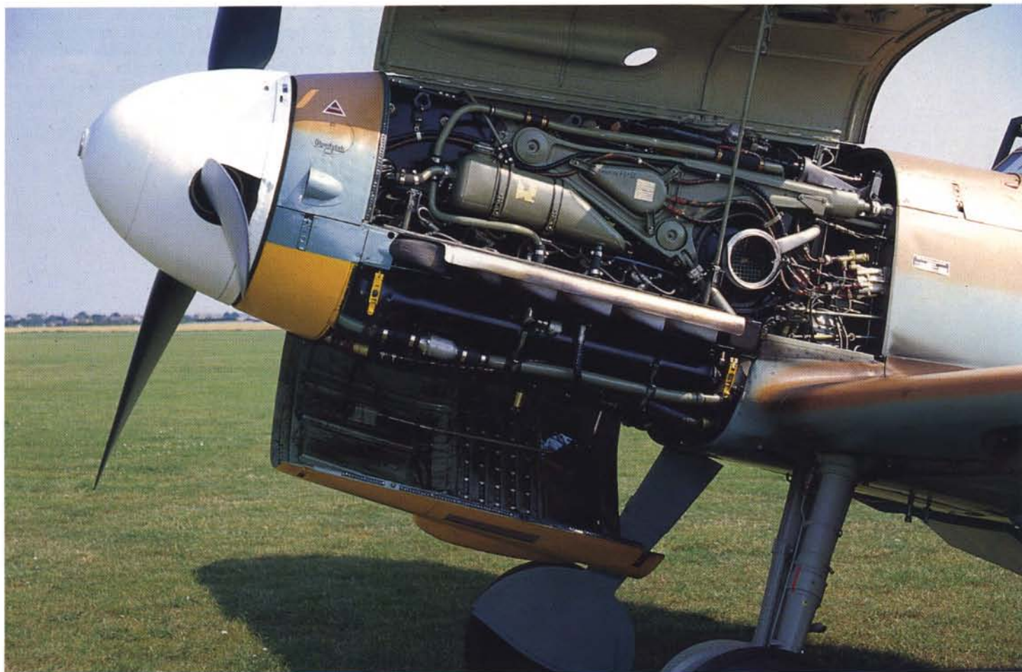
The powerful Daimler-Benz DB605A engine nestled in its cramped, space-efficient cowling.
