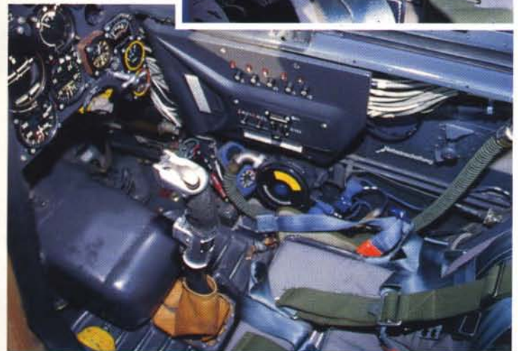
Circuit panel located on the starboard wall with the oxygen regulator below it. In the center are the coaxial 20mm MG151/20 breech cover and the control stick.
