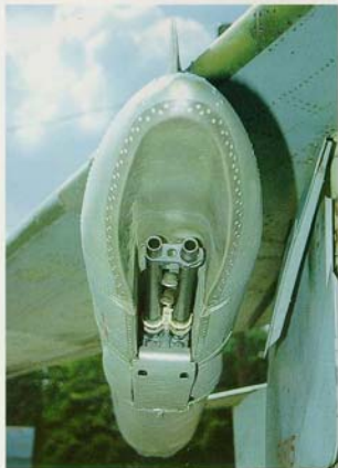
(Above) Rear view of the UB-32A launcher attached to the standard BD3-57MT pylon on wing station N°6.
