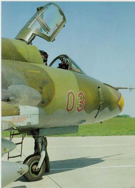
The auxiliary air intake can be seen in almost any position on parked aircraft. Usually, the upper ones open inward and the lower ones slightly outward because of gravity. Note the wing leading edge and pylon close to the muzzle is protected by heat resistant steel plates.
