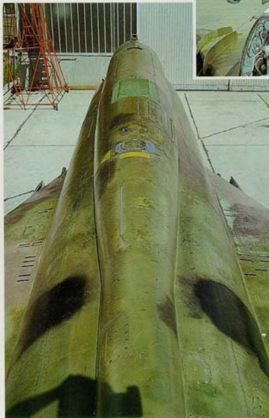
(Right) Visible details of the aft spine are the rectangular dielectric fairing of the ARK-15M aerial, the twin KDS-23 dispenser on starboard side and the central refueling point with control panel. Internal fuel capacity is 4900l in five fuselage and two wing tanks. With the additional 850l underfuselage tanks and two 1150l underwing drop tanks, total fuel capacity exceeds 8900l.
