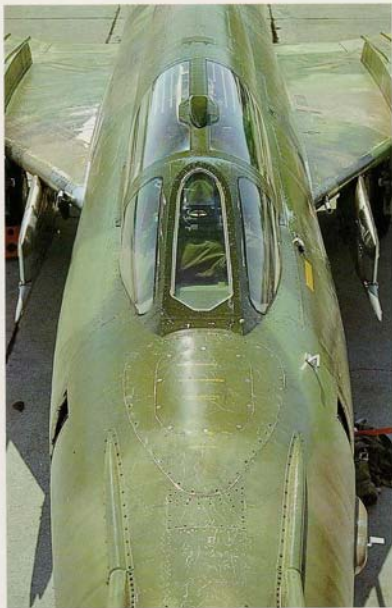
(Above) The center section of the windscreen is made of 40mm thick armored glass, electrically heated for defogging. Additional protection is given by a 22mm armorplate attached to bulkhead N°4, forming the forward cockpit wall. The avionics bay ahead of the windshield houses gunsight related electronics among others. The canopy latch, temperature probe and angle of attack sensor are located on the port side.
