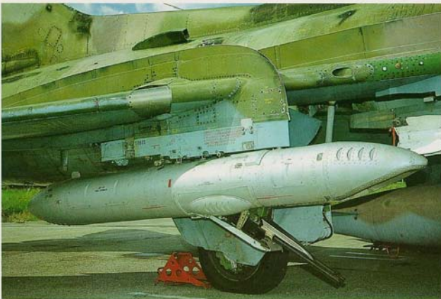
The huge S-25-OFME unguided air to ground missile is stored inside the O-25-L/E launcher. It is attached to the outer wing pylons and has a total length of 3575 mm (launcher 2860mm) with 370mm width and 460mm height.
