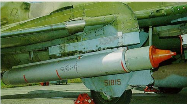
The huge S-25-OFME unguided air to ground missile is stored inside the O-25-L/E launcher. It is attached to the outer wing pylons and has a total length of 3575 mm (launcher 2860mm) with 370mm width and 460mm height.
