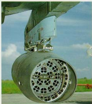
(Above) Rear view of the UB-32A launcher attached to the standard BD3-57MT pylon on wing station N°6.
