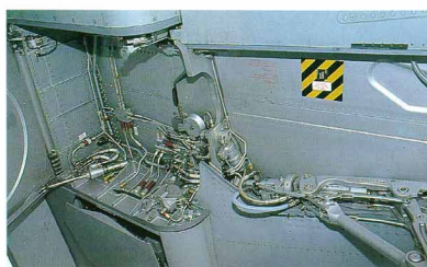
Because of a narrow wing cross section ample space is available for the main gear and its retraction mechanism as shown in top and bottom photo.
