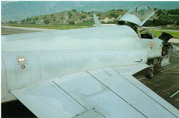
Spine and upper wing root detail clearly showing the forward LERX (or extended root fillet) for improved flight characteristics during high G-maneuvers and low speed handling. The red & white triangle marks the position of the flight system hydraulic tank. Note the black walkway demarcation on the wing.
