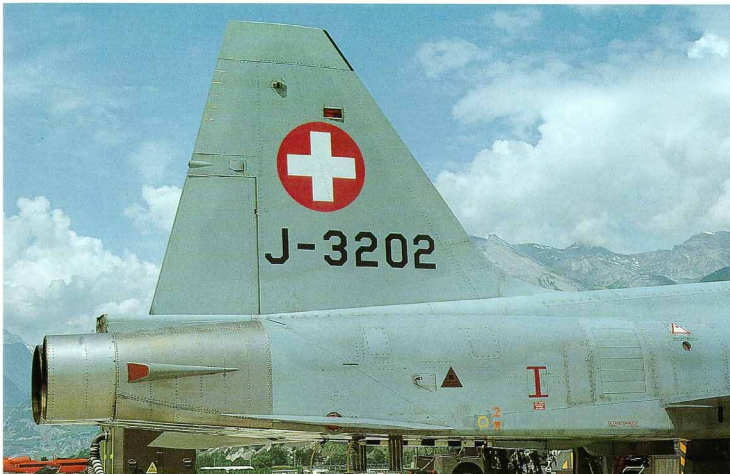
TIGER tail detail with fin tip leading edge UHF aerial, white TACAN/IFF bands at the trailing edge, fuel vent and VHF communications antenna immediately above the rudder. Note the all-flying horizontal tailplane and its fuselage hinge point.
