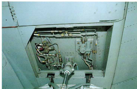
The airbrake manifold and control valve are roof-mounted inside the shallow housing.
