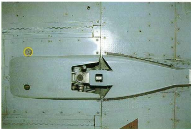
Important detail is the arresting hook fuselage attachment (above) and the two small rectangular hatches on either side of the hook to reach the engine oil reservoirs and from which mechanics retrieve small bottles of unburned fuel from the combustion chambers. Port panel also has engine starter hose hook-up.
