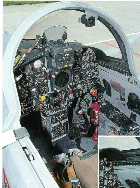
Looking down to the cockpit floor and the ejection seat survival kit with seat cushion. Note the tight fit of the seat between the side consoles and the small cushion to the back for supporting the pilot's parachute.
