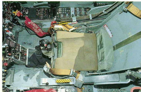
Looking down to the cockpit floor and the ejection seat survival kit with seat cushion. Note the tight fit of the seat between the side consoles and the small cushion to the back for supporting the pilot's parachute.
