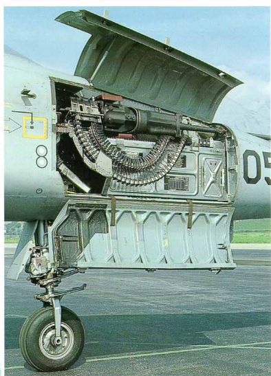
(Above) Installation of the 20mm Pontiac M39A2 cannons revealed, each able to fire 280 rounds of which 246 are stowed inside the ammo box below the gun. In peacetime, empty shells are retrieved in the black (mastic covered) box behind the gun (bottom right picture). Ammo speed is 1500 rounds per minute.
