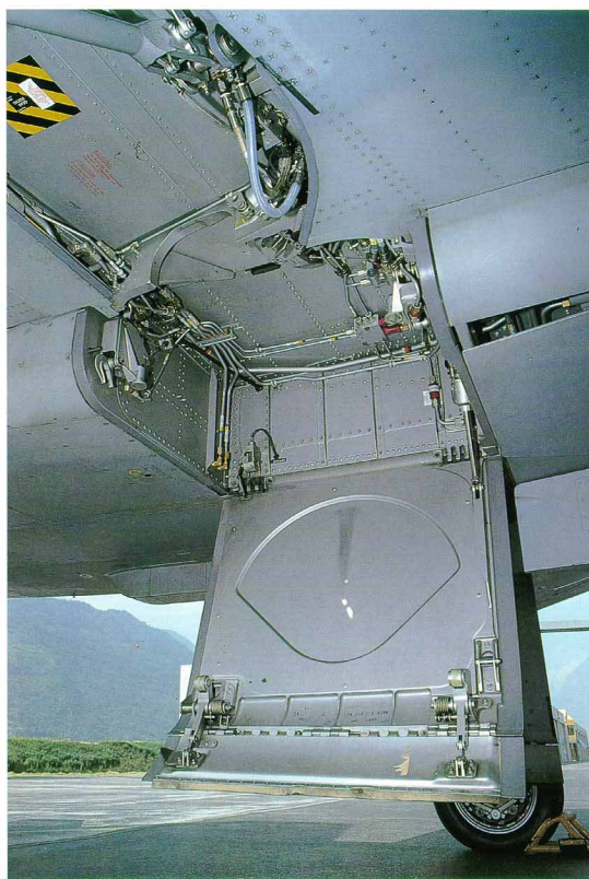
Wide-angle view of the immaculate starboard side main wheel well with split main gear door and dual locking mechanism. Note the retraction actuator at front.
