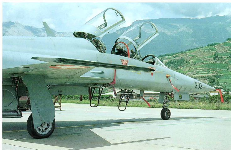
The sleek lines of the F-5F are very apparent in this quarter rear view of the nose section, clearly demonstrating its relation to the T-38 Talon, built by the same manufacturer. Note the bright red color of the cockpit center frame and the position of the low voltage formation light strip on the canopy instead of the fuselage as with the F-5E. Also note Sidewinder launch rail inner detail.
