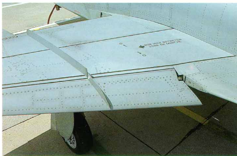
An improvement over the initial F-5A (F-5F wing shown) design was the installation of electrically operated leading edge flaps.
