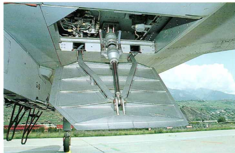
Inner detail of the magnesium construction ventral airbrake, the inboard edge cut for belly storage clearance, and its actuating rod.
