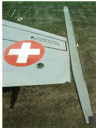
The Sidewinder missile launch rail on the F-5E is not much different than with other aircraft except for the incorporation of an outboard formation light at the rear.
