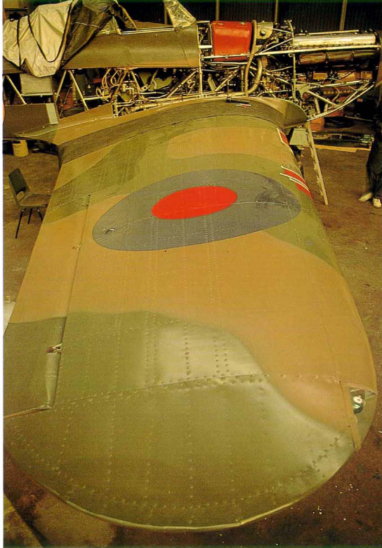
General view of the right wing upper surface with large two tone roundel. In the background can be seen the partially stripped fuselage and engine compartment. Contrary to the fuselage, the wing is an all-metal construction.
