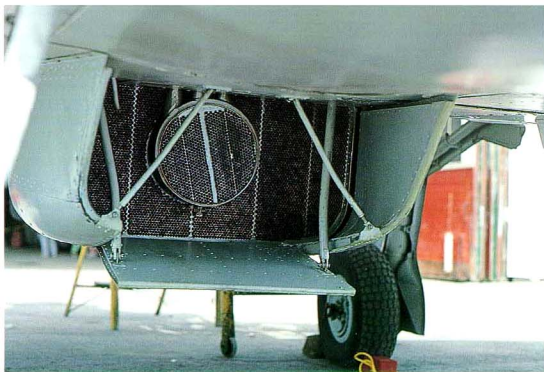
Front and rear view of the ventral oil and coolant radiator. The radiator fairing flap was generally open on parked aircraft.
