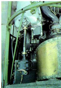
Engine coolant header tank with tubing and supply hoses (see also previous page) together with other engine related accessories and connectors.
