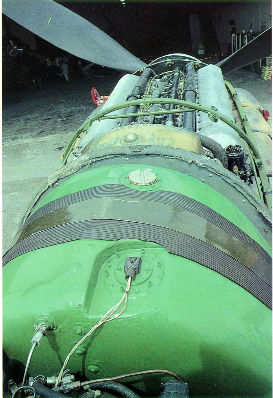
A view of the fuel tank and coolant reservoir from the rear. Capacity of the fuel tank was 28 Imperial gallons and served primarily as a reserve tank.
