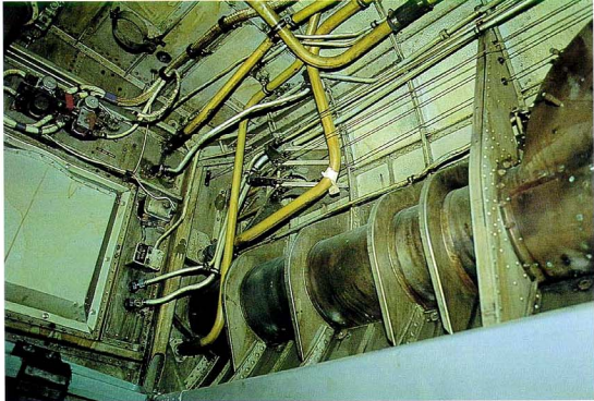
A firewall separates engine compartment and wheel well. Small bulkheads hold the exhaust pipe in position against the sidewall. Note the concentration of tubing in this area and also the control cables at the top.
