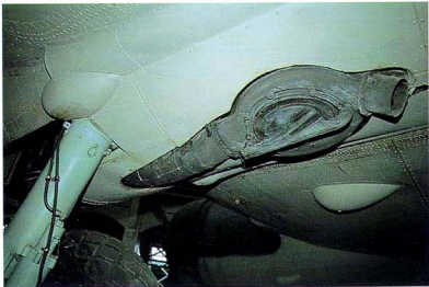
The below-nacelle supercharger with cooling intakes. The outlet at the rear of the supercharger is a waste gate.
