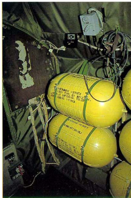
The area behind the seats is taken by more oxygen bottles and emergency back-up systems. Even a portable oxygen bottle is racked within arms reach for emergency situations. Note the crewmember's seats are mounted on solid beams rather than on platforms, providing stowage room below the seats.
