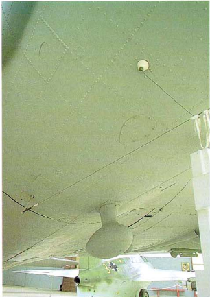
Close up of the loop antenna under the B-17 belly just in front of the bomb bay doors. Below can be seen the main gear strut wing attachment.
