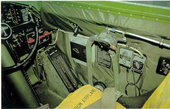
Further aft are the interphone jackbox and oxygen regulator. Note the neat fuselage lining.
