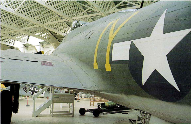
A good view on the wing/fuselage joint and upper wing detail with various exhaust louvers. On top of the fuselage can be seen part of the Sperry upper turret with twin .50 cal Browning machine guns.
