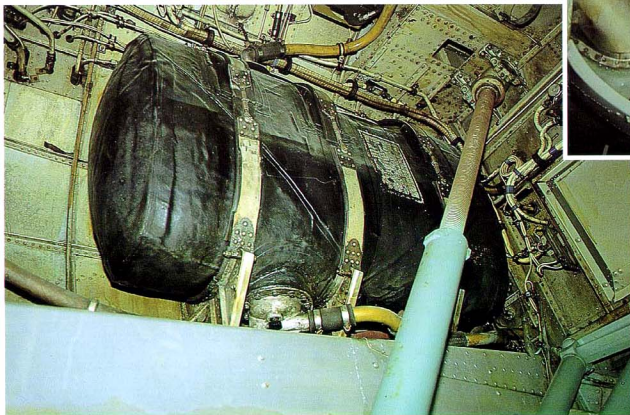
The main gear wheel well on starboard side looking up and aft. The hole at bottom right houses the main gear strut. The pressure duct to the roof connects to the intercooler behind the rear wall. The duct at bottom left connects to the supercharger. Tightly strapped against the nacelle wall can be seen the 37 US gal oil tank (30.7 Imp. Gal/140Liter). Note the forward retracting rod attached to the roof.
