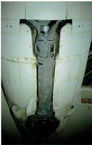
More belly and underwing detail is revealed in these photos whereas the bottom left photo focusses on the front of the supercharger where it emerges the engine nacelle.
