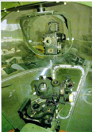
Just forward of the navigator's station and to the fuselage side is a control box operated by the bombardier. Note the red securing cover over the electric bomb release switch to the right of the box. The port cheek gun (operated by the navigator) can be seen hanging from the roof.
