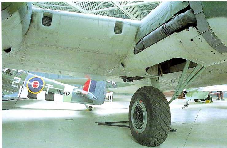
A firewall separates engine compartment and wheel well. Small bulkheads hold the exhaust pipe in position against the sidewall. Note the concentration of tubing in this area and also the control cables at the top.
