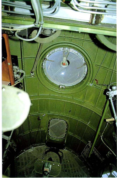
The Astrodome with compass viewed from below. Two locking side levers secure the hinged dome. Note the gun cable reels aside the dome and the forward upper observer window.
