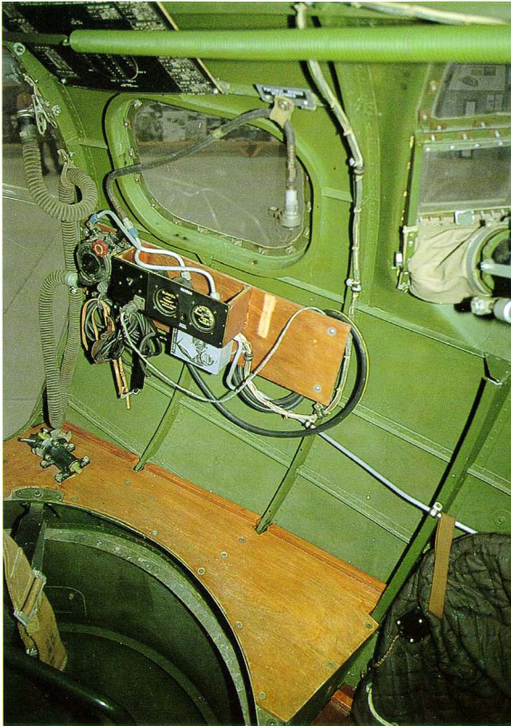
To the right of the bombardier's station is a bombardier's loading panel and oxygen flow regulator. Note the bombardier is seated on top of the open chin turret, overlooking the twin .50 cal guns (dummy's installed here).
