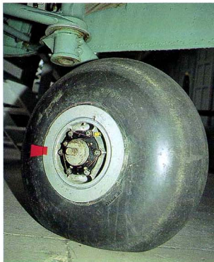
The fully retractable tail wheel (contrary to the partially retracted main wheels) features a single side yoke and big Good Year balloon tires, suitable for rough grass field from which most B-17's operated.
