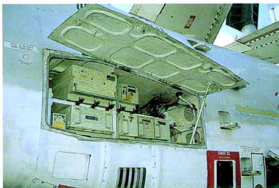
The Viking has two avionics bays in the aft top fuselage section, the starboard bay holds some avionics mounted in racks. Note the arrestor hook manual retraction pushbutton aft of the bay.
