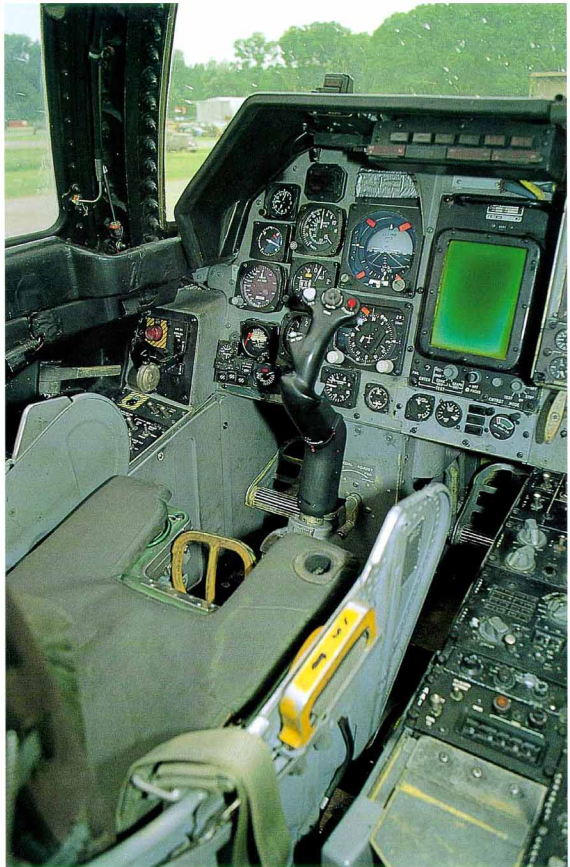
Pilot's console with central control column and major flight instruments. Note two rear view mirrors are attached to the cockpit side frame and the many scratches in the cockpit glass.
