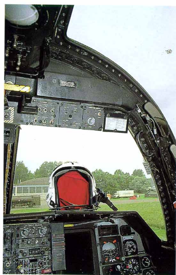
Co-pilot's station with most of the same flight instruments as on the pilot's panel but with fairly larger display screen and additional caution panel. Note the radar operation control panel at the bottom of the extreme right side of the console. Also note the pedal adjustment handle behind the control stick.
