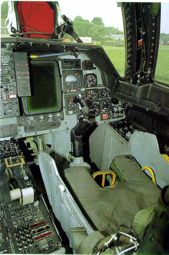
Co-pilot's station with most of the same flight instruments as on the pilot's panel but with fairly larger display screen and additional caution panel. Note the radar operation control panel at the bottom of the extreme right side of the console. Also note the pedal adjustment handle behind the control stick.
