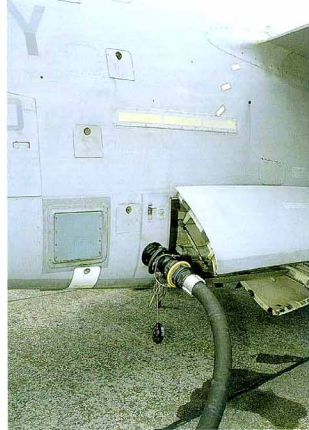
The Viking's single point refueling connector is located just aft of the starboard main gear housing.
