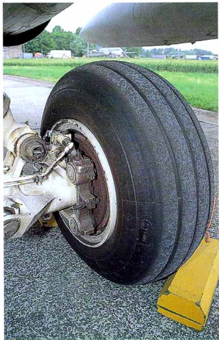
Apparently visible in the bottom right photo is the inboard heavy-duty disc brake and connecting brake fluid lines.
