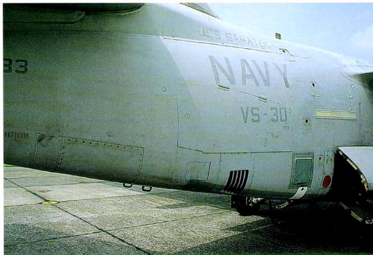
The small gray rectangular hatch aft of the single point refueling connector houses an ECM panel, covered here but clearly visible in the large photo on the next page, also showing the foldable steps on the aft fuselage. Note the low-voltage formation light strip and the flap deflector indicators.
