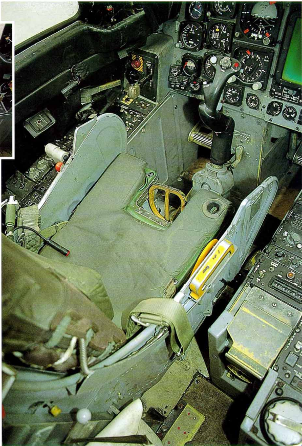
Pilot's side console with mostly lighting control panels and auto-pilot control panel. Note two small console lights on the side wall and one larger instrument panel light on the window sill.
