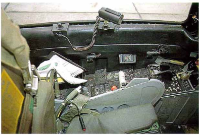
Pilot's side console with mostly lighting control panels and auto-pilot control panel. Note two small console lights on the side wall and one larger instrument panel light on the window sill.
