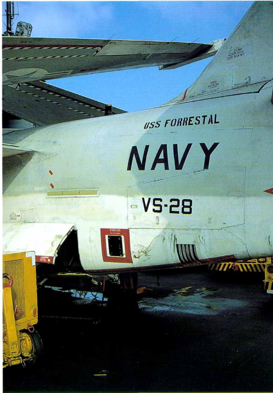
Close-up of the rear fuselage area on the port side clearly showing the shape of the avionics bay hatch and the exhaust louvers just below it. The bay on this side is used to stow engine covers and related equipment. Note the black and white walkway markings on the folded wings.
