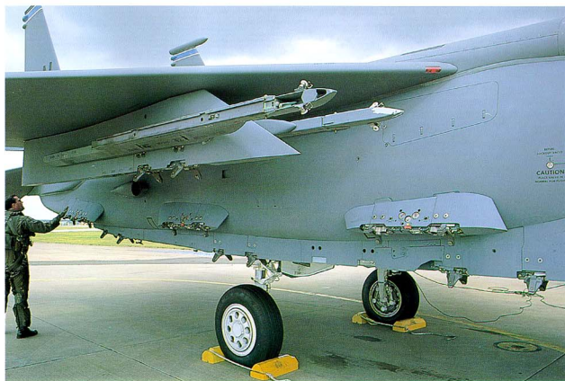
Detail of inboard SUU-59C/A wing pylon with missile launcher rails on both sides (above & below).
