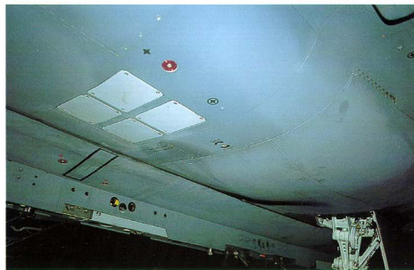
Bottom detail of the F-15E clearly showing the bulky main landing gear doors providing additional space for the wider main wheel tires.
