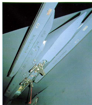
Detail of inboard SUU-59C/A wing pylon with missile launcher rails on both sides (above & below).
