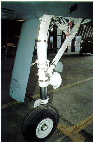
The F-15E nose landing gear differs slightly from the one used on previous F-15 models.
