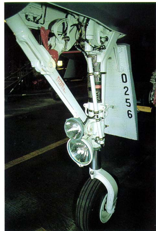
The F-15E nose landing gear differs slightly from the one used on previous F-15 models.
