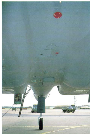
Bottom detail of the F-15E clearly showing the bulky main landing gear doors providing additional space for the wider main wheel tires.
