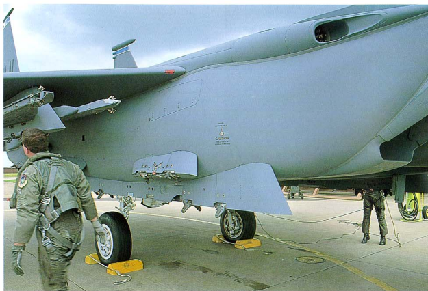
Detail of inboard SUU-59C/A wing pylon with missile launcher rails on both sides (above & below).
