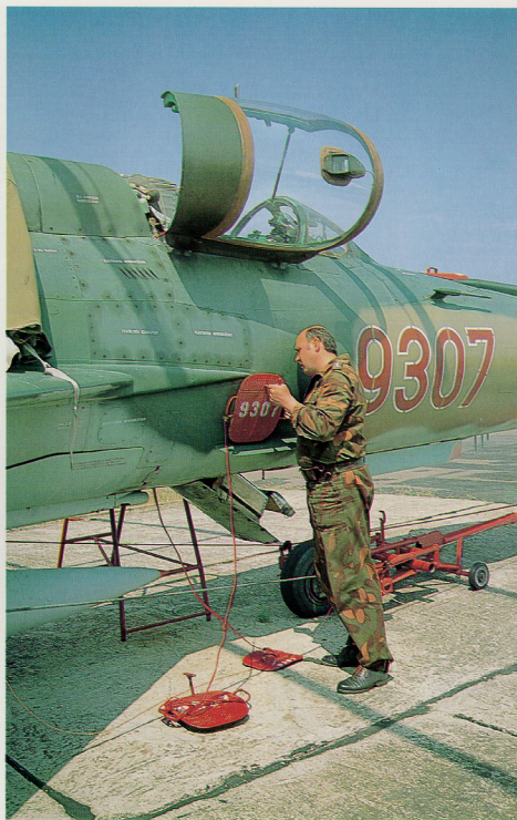
RSM János Szél installing the cover grid over the starboard suction relief door as part of the pre-flight activities. The grids protect against FOD (foreign objects) during engine runups. The accumulator batteries are yet to be installed as can be notified from the open battery bay aft of the nose landing gear.
