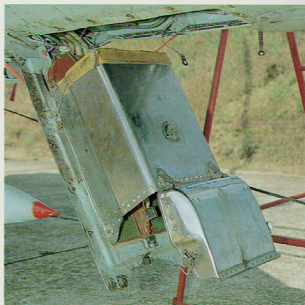
The heat resistant housing of the two 15-SCS-45 accumulator batteries. These batteries are installed before the first flight of the day and are only removed after the last mission of the day is completed, to be recharged overnight (except for aircraft on alert). These units, with 45Ah capacity, can supply the vital systems for a 15 minute period in case of a generator malfunction.
