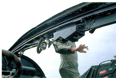
Important detail for modelers, seldom shown so clearly, is the overhead control column.
