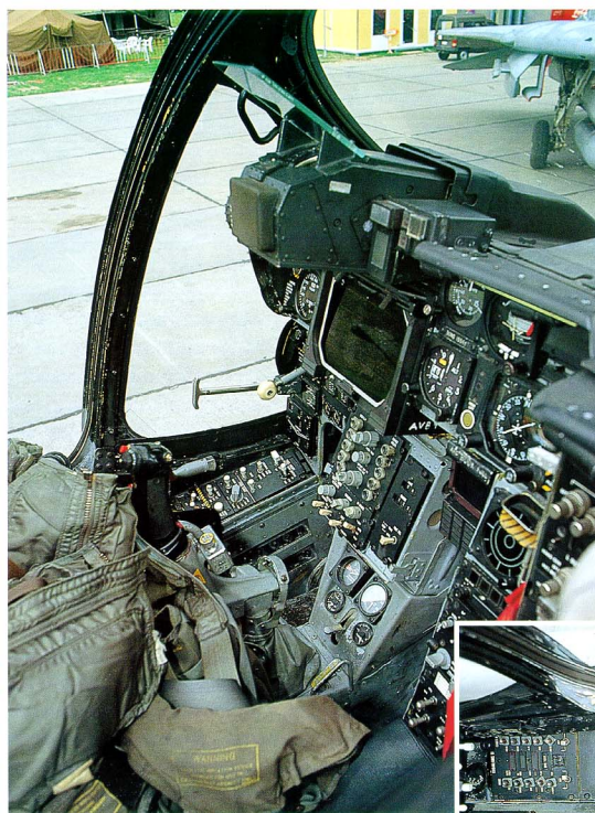
Again the pilot's station, this time viewed from the B/N seat. Clearly visible at the far end is the landing gear actuating handle and the emergency brake selector handle. The protective face cushion over the radar screen is used by Lt John "Frito" FREDAS to stow his oxygen mask.
