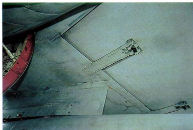
Underwing detail of the trailing edge travel guide, also showing the position of the underwing pylon in regard to the wing trailing edge.
