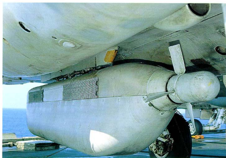
An AN/ALQ-99(V) jamming pod carried on the centerline belly pylon with the rear end of the pod open to allow coolant air to escape (see also top middle photo). Note the different location of the chaff/flare dispenser cages and blade antenna on the Prowler (top right photo).
