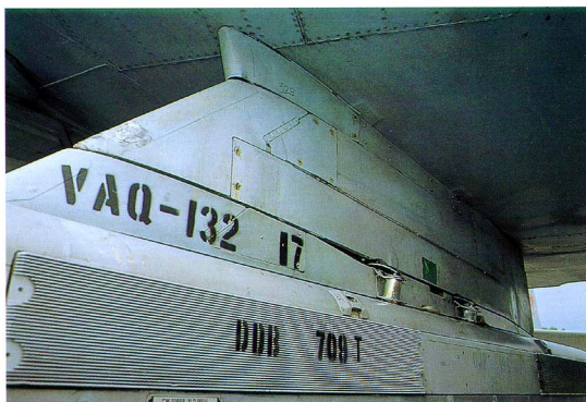
Close-up of the outboard pylon and sub-pylon holding the jamming pod. Barely visible at the bottom of the photo is the jamming pod ID marking, reading CW-1089B/ALQ-99(V).
