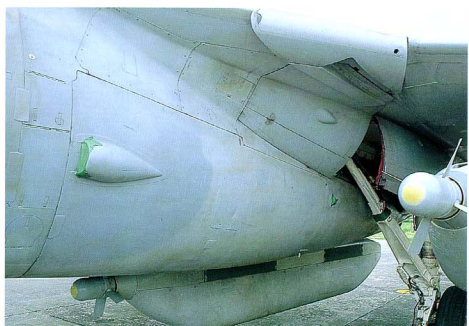
An excellent view on the wing glove main wheel door which is shown closed, as is common on parked aircraft. Note the recess in the bottom wing fillet. Noteworthy at far left are the two small panels being blocked by the retractable boarding step.
