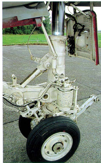
Left an right rear view on the nose gear strut which is similar to the A6-E nose gear. Unlike other aircraft which have the oleo at the bottom of the strut, Intruder and Prowler have the oleo on the top, behind the small gear door. At front is the launch shuttle engaging bar.
