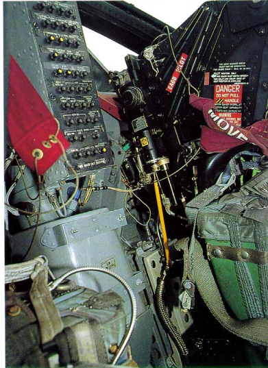
The upright console between the seats is used to store the forward main circuit breaker panel with a first aid kit container below. Note that the canopy defogging pipe does not run behind the pilot's seat but stops at the port side canopy hook-up. One can spot the rear of the ECMO-3 instruments in the distance.
