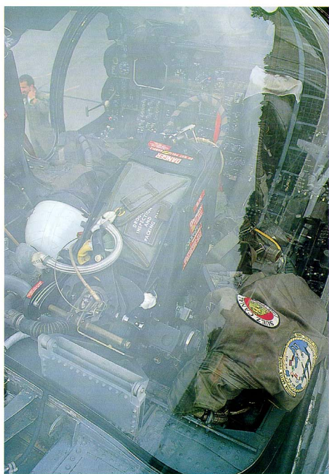
An almost similar view on the bombardier/navigator's seat. Note the safety pins are also installed on the left side of the seat headrest, hard to reach from this side of the aircraft. When the ejection handle (face curtain handle at front in the seat headrest or the handle between the crewman's legs) is actuated, the seat is simply blasted through the canopy.
