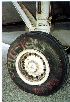
Outer wheel detail with partially faded sticker on the wheel hub, reading "ANTI-SKID GENERATOR". Note the painted markings on the rubber tires.
