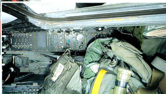
Again the pilot's station, this time viewed from the B/N seat. Clearly visible at the far end is the landing gear actuating handle and the emergency brake selector handle. The protective face cushion over the radar screen is used by Lt John "Frito" FREDAS to stow his oxygen mask.
