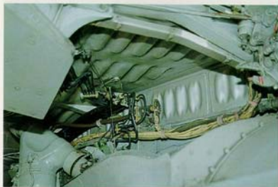
Angled main gear hinge point and shallow leg housing area. The piping of different systems can be recognized as follows: black- pressurized air, yellow- fuel system, grey/bare metal- hydraulics, blue- oxygen, brown- oil system.
