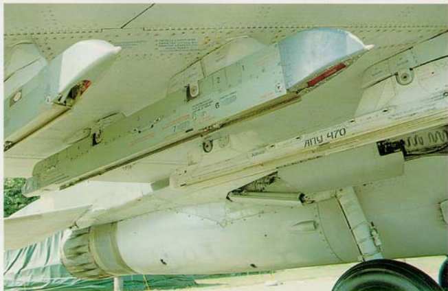
The inboard wing pylon is capable of holding missile launcher pylons (shown here) or 800 liter external fuel tanks (with heavier pylons). The latter remain attached to the fuel tanks during removal and transport.
