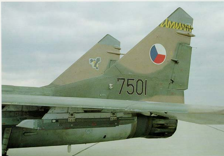
The tail area of "7501" from the left with colorful markings on the inside of the right vertical tailplane. Two ram air intake probes can be distinguished just in front of the tailcode. Note the mirror image of the national insignia (compare with page 16).
