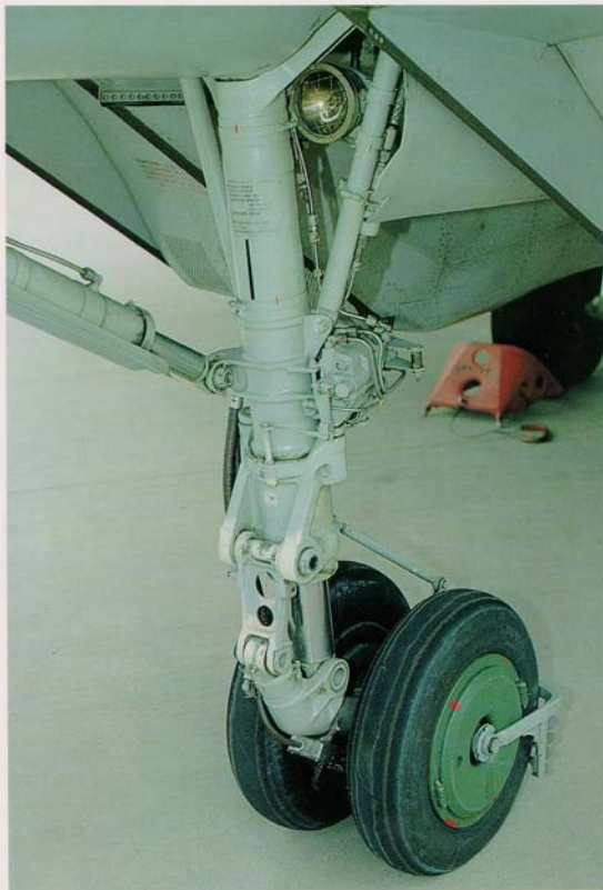
Noteworthy in this view is the single landing light mounted to the left upper side of the strut and both anti-sway struts. A small strut aft of the leg serves mudguard movement according to gear position.
