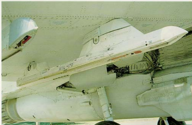
The inboard wing pylon is capable of holding missile launcher pylons (shown here) or 800 liter external fuel tanks (with heavier pylons). The latter remain attached to the fuel tanks during removal and transport.
