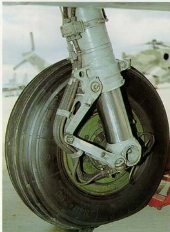
Inside detail of the left main wheel hub with scissor linkage and hydraulic pressure hoses for the brakes.
