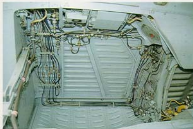
Left main gear well only differs in detail from the right side well as described on page 10 & 11, mainly in components attached to the outside upper wall. Wiring is almost identical.
