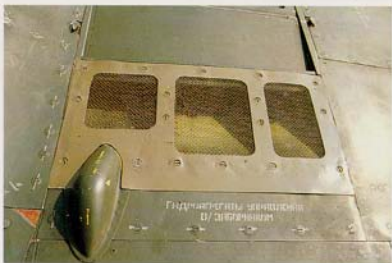
A screen cover spans the boundary layer bleed air vents aft of the auxiliary air intakes. Again note the Cyrillic inscriptions.
