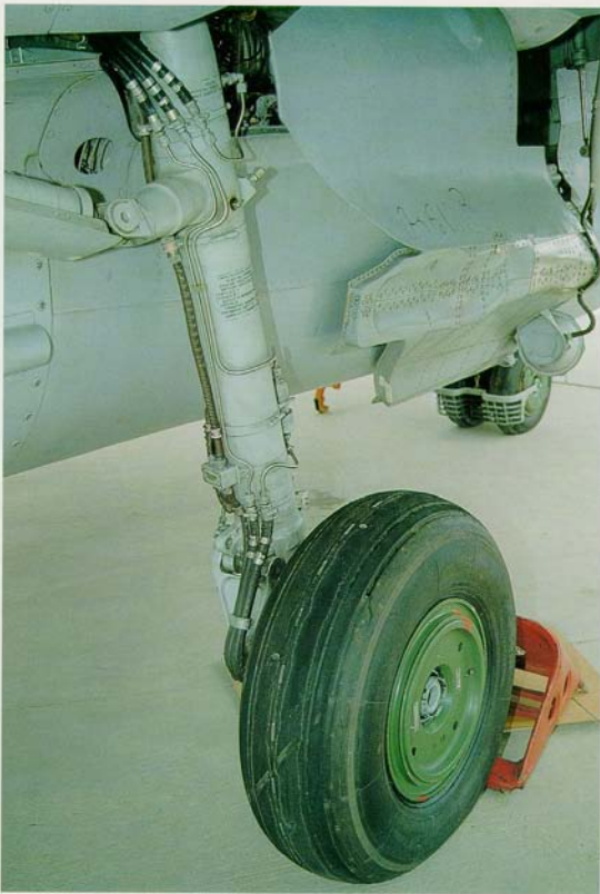
The main gear strut and door from behind revealing main gear detail and the pushbeam connecting strut protruding from the main leg. Note the shape of the outboard wheel well cover.
