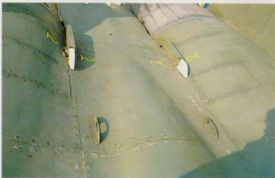
Speedbrake actuators which are located inside of each engine nacelle (above and below). Noteworthy is the tapering of the spine into the speed brake and the lifting eyes closest to the camera.
