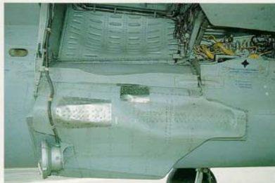
No differences here with a second landing light and reinforcement plates to the gear door inside surfaces.
