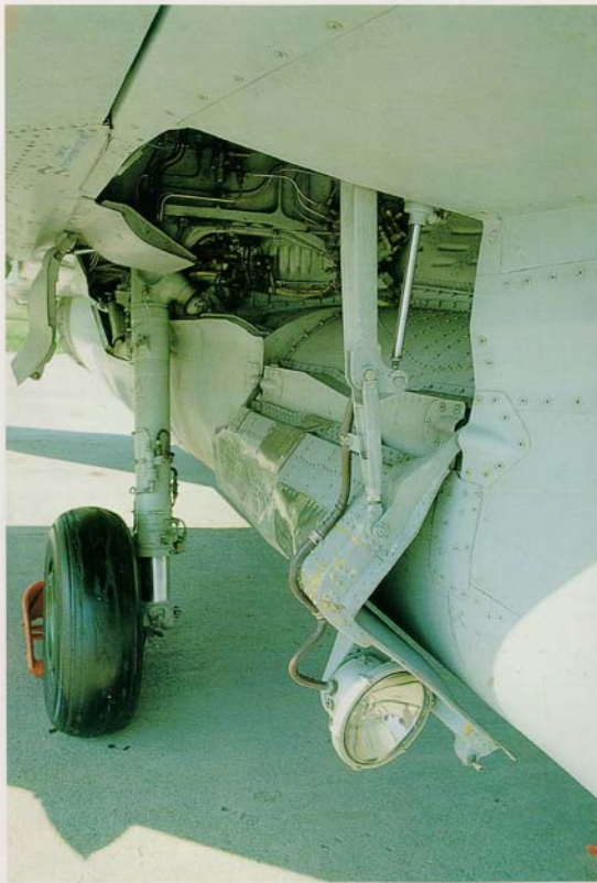
The right side main gear door looking aft with the forward mounted retracting arm and actuating ram. The door also serves as a mounting platform for the landing light, served by an oversized electrical feed line.
