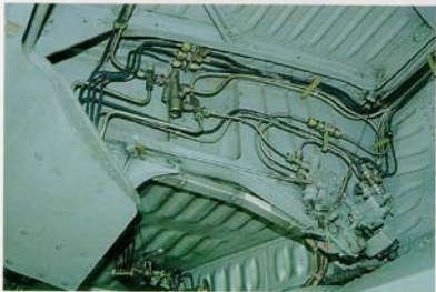
A view on the center spar of the main gear well also serving as a platform to mount feed lines and pressure control devices.
