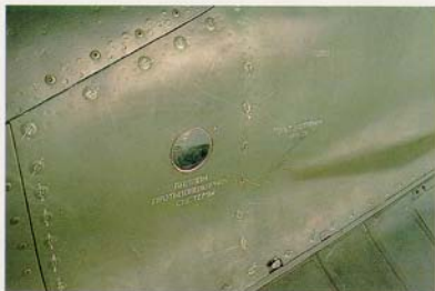
Upper fuselage detail includes small circular inspection glass in the slope of the spine, next to the right side auxiliary intake doors.
