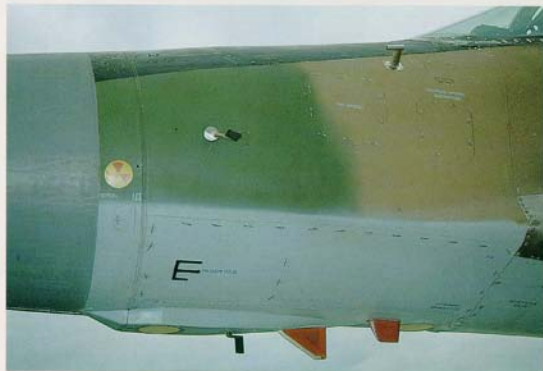
One more AOA vane and static sensor probe can be found on the left side nose area. Note the camouflage demarcation line.
