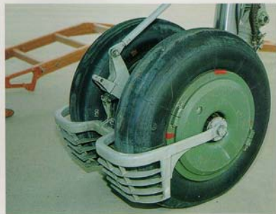
Noteworthy in this view is the single landing light mounted to the left upper side of the strut and both anti-sway struts. A small strut aft of the leg serves mudguard movement according to gear position.
