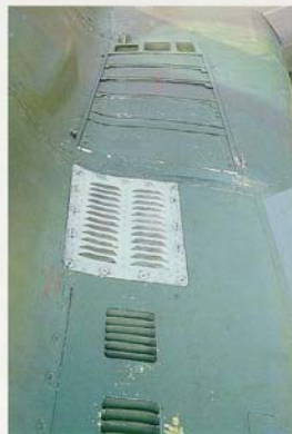
(Top right and below) When the intake FOD screen is lowered with engine cranked, the spring-loaded ventral auxiliary air intakes automatically open to maintain a constant airflow to the engines.
