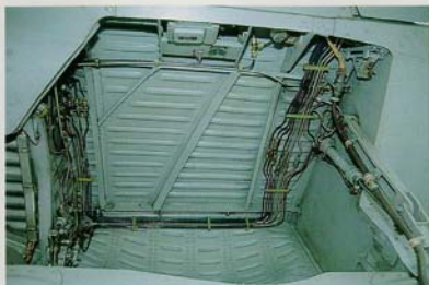
The main wheel bay roof features embossed panels and structural strengtheners, surrounded by feed/hydraulic lines mainly serving gear and gear door retraction. The small pressure gauge and box counts engine operation time.
