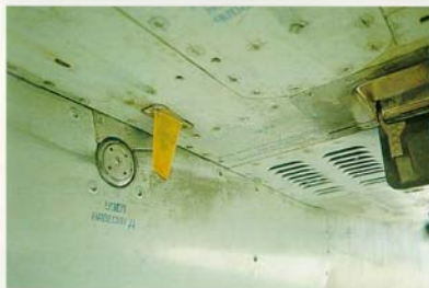
(Above & right) Halfway down the tunnel between the engine nacelles is an auxiliary power unit outlet door and exhaust vents. Centerline fuel tank connectors and hook-ups are also apparent.
