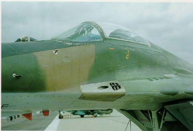
Forward left side nose area with bare metal gun exhaust muzzle in the center of the picture. Just aft of the gun opening is a two-rib blast suppression duct shown in detail in the top left picture. On top are four vented slots to remove gun gases from the gun compartment.
