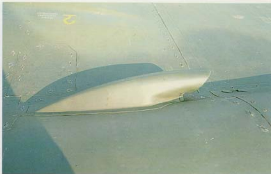
The APU air intake scoop mentioned earlier is located just on top of the GTDE-117 gas turbine auxiliary power unit. The APU is used not only to start the engines but for cranking cold engines during maintenance and to provide power for all systems during ground operations.
