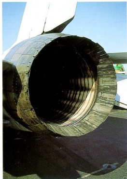
Partially dilated (left) and fully dilated (right & below) exhaust nozzle of the Pratt & Whitney TF30-PW-414 turbofan engine.
