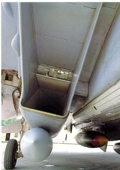
(Left) The air intake nacelle is installed some distance from the fuselage which is very clear in this view. Also, the N°1 and N°2 air intake ramp can be seen at the intake roof.
