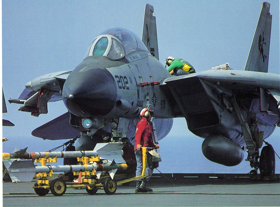
The "Mighty Tomcat" of the "Tomcatters" tied to the front deck elevator, its tail and exhaust nozzles well over the side. Sunlight reflection clearly shows the tinted glass of the TCS and the front windscreen annex HUD. On top, a green-shirted ordnance men is replacing some malfunctioning avionics while red-shirted weapon specialists are awaiting the arrival of the "Sidewinder trolley". Note the ECM fairing on the wingroot/air intake nacelle and the radome/anti-glare panel demarkation.
