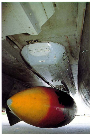
Three photos to conclude the external walkaround of the F-14B Tomcat with a final view on the solid tail hook fairing and the rear of the travel pod.
