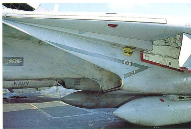
A lot of time and effort was spent designing the variable-geometry air intake with rectangular cross section and highly raked intake lips. Various probes and sensors provide data for the Air Inlet Control System (AICS) which independently controls actuators and hydraulic power systems of right and left intake. Note the lower lip of the inlet duct is bare metal.
