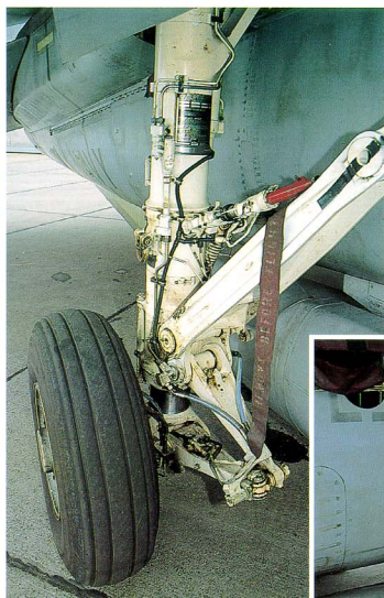
Massive main landing gear strut of conventional concept located aside the engine nacelles, designed to take the heavy punishment of deck landings. Note bottom left detail shot of the main gear locking bracket in the lower nacelle edge.
