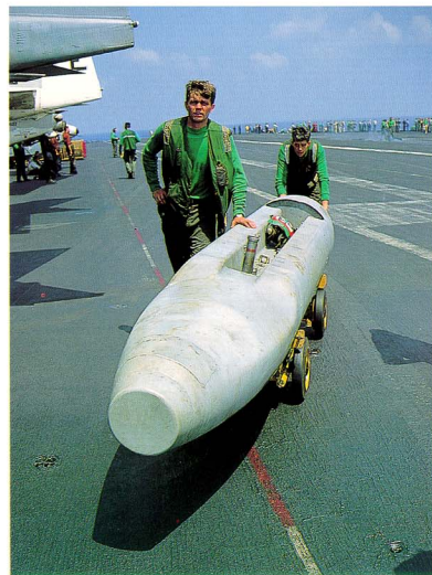
(Below) Rare view of slot at top of the nacelle drop tank. Support pylon recessment is dictated by minimal ground clearance of tank below nacelle.
