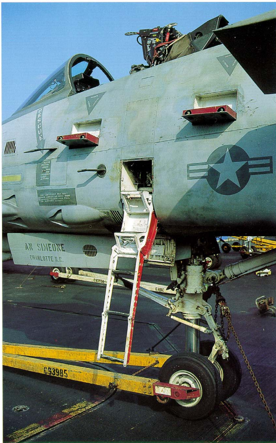
A lot of time and effort was spent designing the variable-geometry air intake with rectangular cross section and highly raked intake lips. Various probes and sensors provide data for the Air Inlet Control System (AICS) which independently controls actuators and hydraulic power systems of right and left intake. Note the lower lip of the inlet duct is bare metal.
