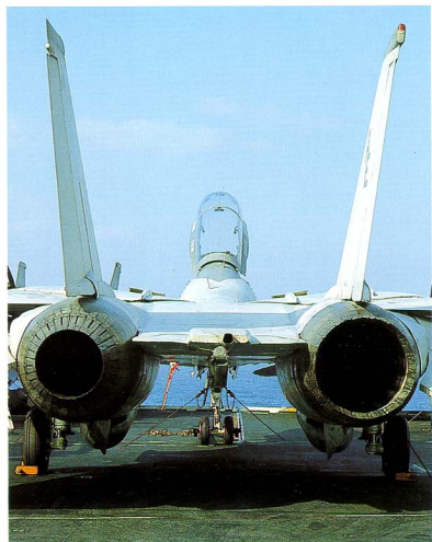
Partially dilated (left) and fully dilated (right & below) exhaust nozzle of the Pratt & Whitney TF30-PW-414 turbofan engine.
