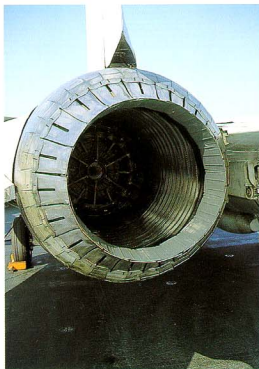
Partially dilated (left) and fully dilated (right & below) exhaust nozzle of the Pratt & Whitney TF30-PW-414 turbofan engine.
