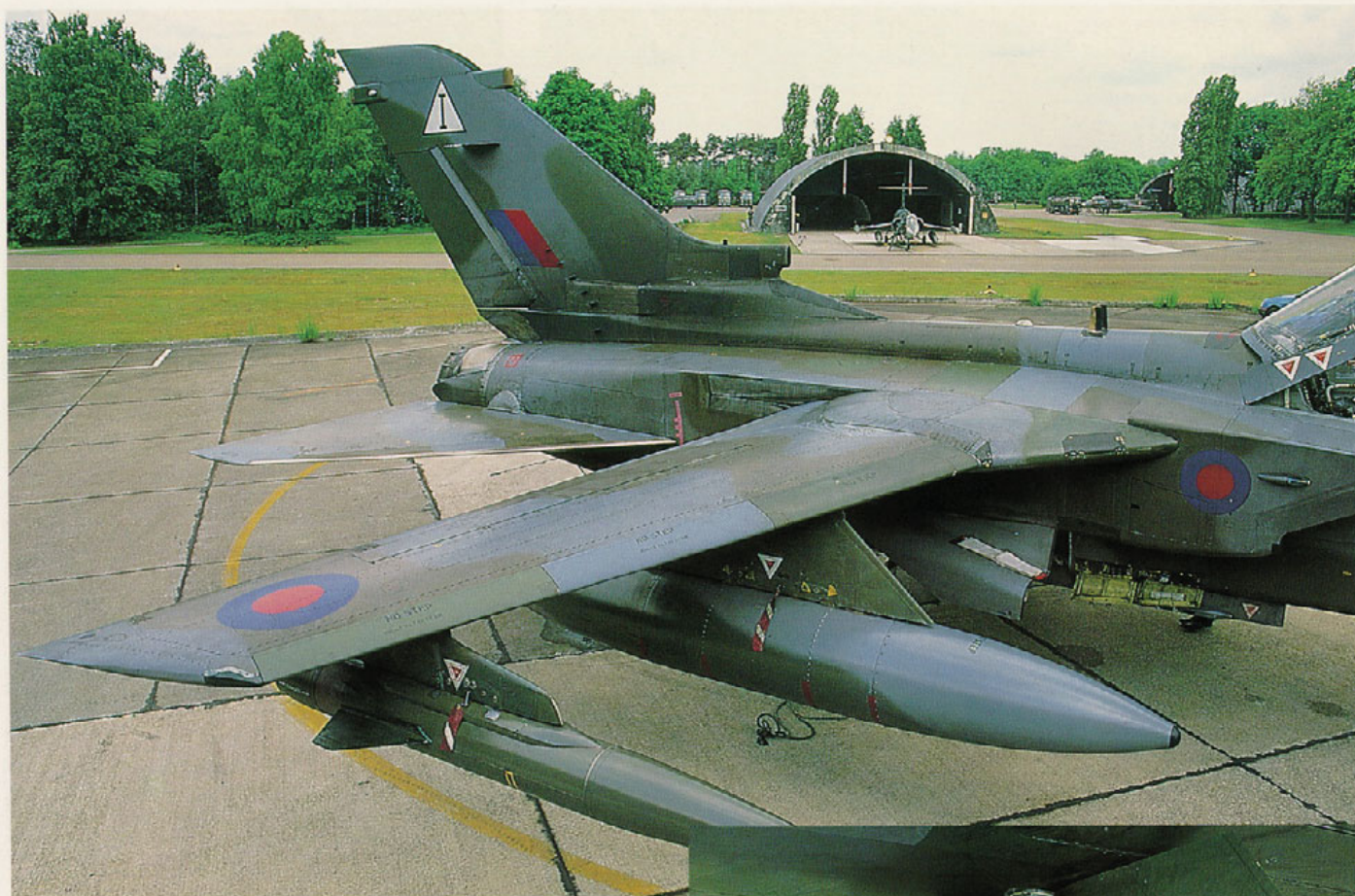
The wing and tail section showing the same discoloration of various panels. The wing, holding a BOZ 107 Chaff/Flare pod on the outboard pylon and a 330 Imp gallon ( 1500 liter) external fuel tank on the inboard hardpoint, is locked in the full-forward position. Note the difference in "NO STEP" markings on the leading edge slats.
