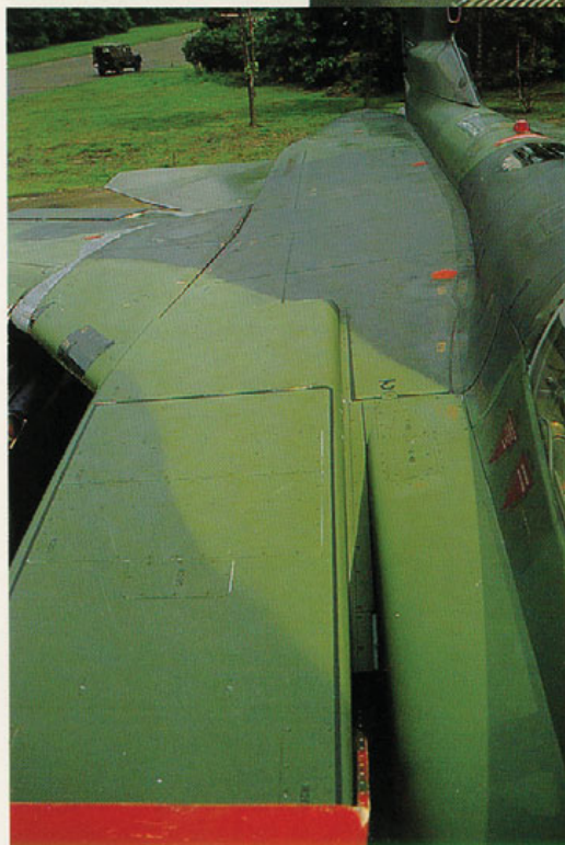
Top :Looking down the spine showing the replacement of the dorsal UHF antennas with a glossy disc antenna. Note the black walkway markings.
