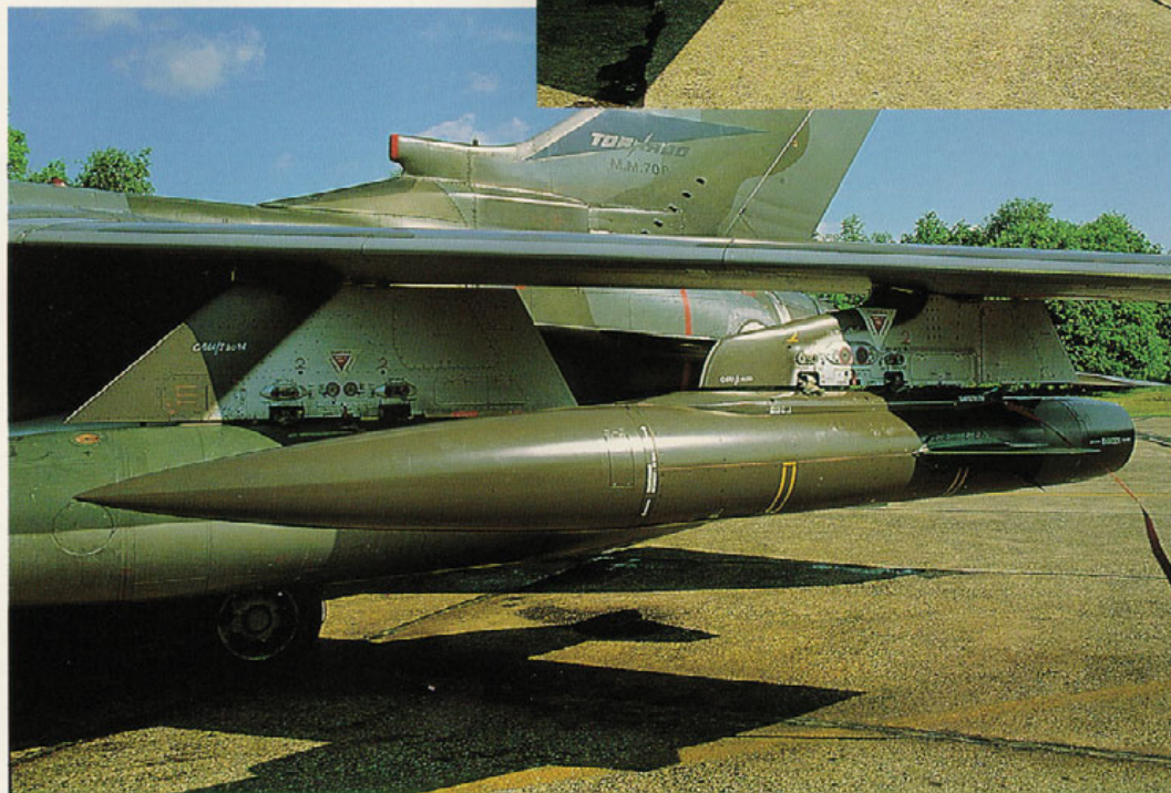
Pylon detail and colors on the same aircraft with the same BOZ 107 Chaff/Flare dispenser shown on page 6. The external fuel tank has forest green upper and silvergray lower surfaces.
