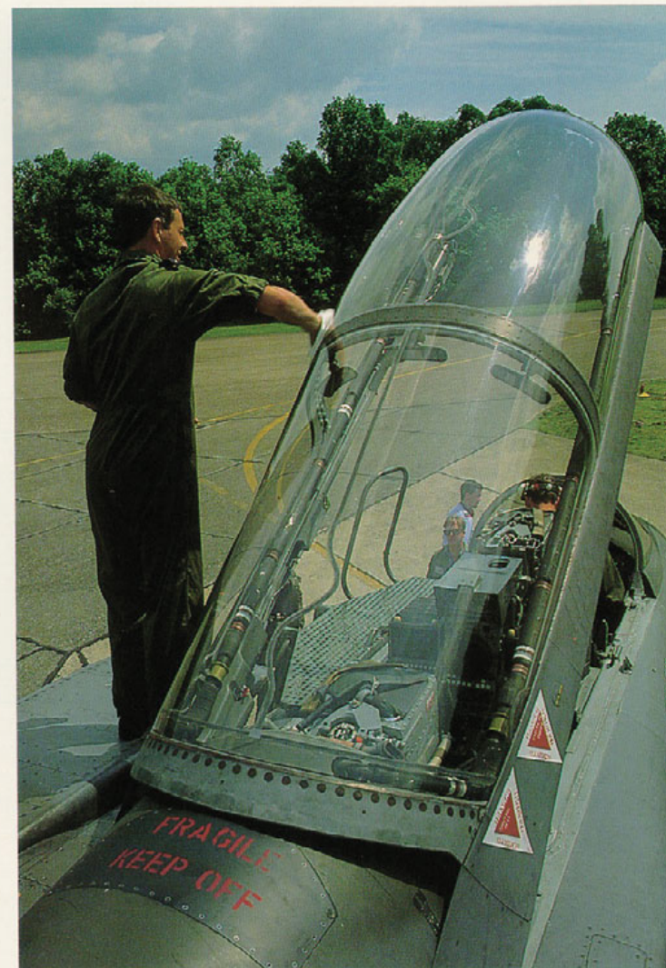
Above: Like most modern planes the Tornado features a single piece perspex hood to cover both canopies. As shown here the hood is kept spotless at all times by groundcrew. In case of emergency the hood can be jettisoned or, if this should fail, fragmented.
