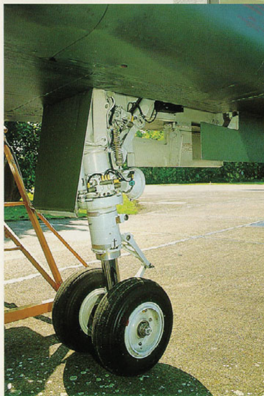
Left: Right rear view of the nose landing gear in overall white finish. Note the spring just above the landing light.
