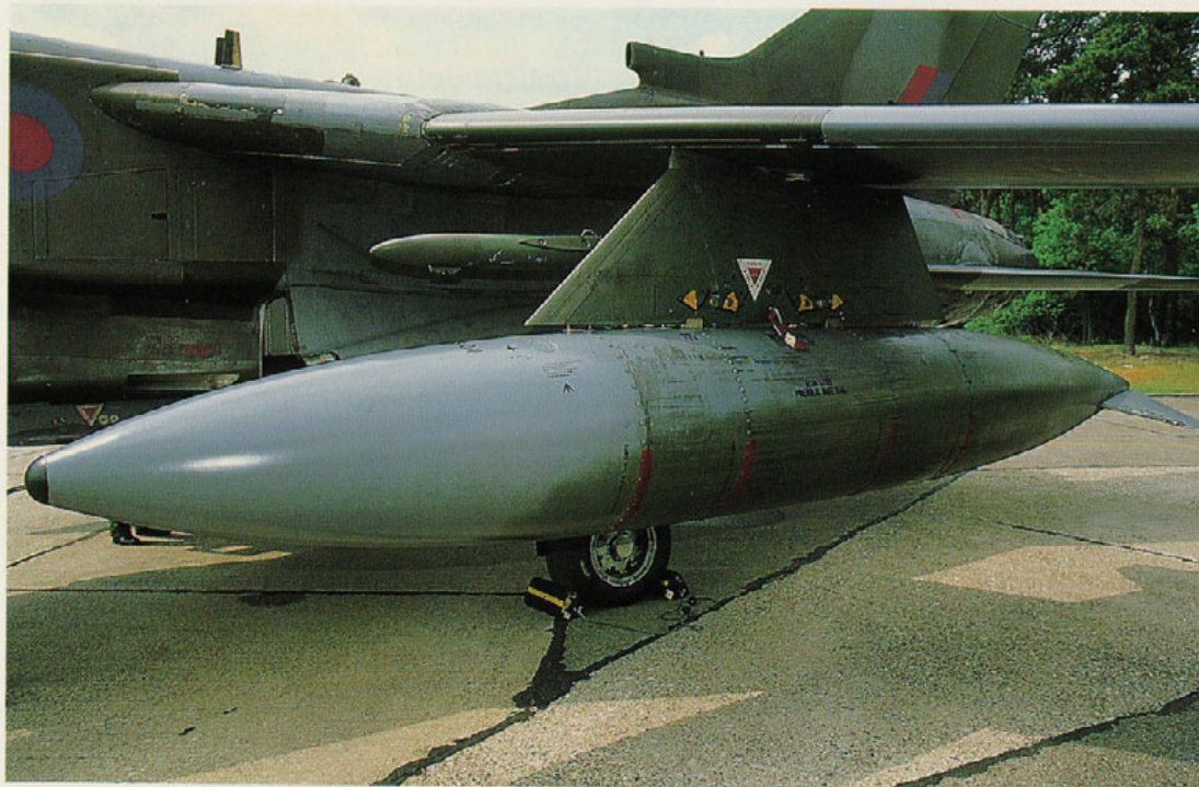
The 330 gallon fuel tank on the inboard swiveling pylon with a black stencilling stating "Asbestos Phenolic Material". Note the clean appearance of the front part of the tank compared to the remainder. The leading edge of the pylon has a different color.
