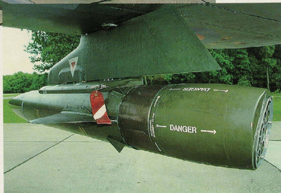
The wing and tail section showing the same discoloration of various panels. The wing, holding a BOZ 107 Chaff/Flare pod on the outboard pylon and a 330 Imp gallon ( 1500 liter) external fuel tank on the inboard hardpoint, is locked in the full-forward position. Note the difference in "NO STEP" markings on the leading edge slats.
