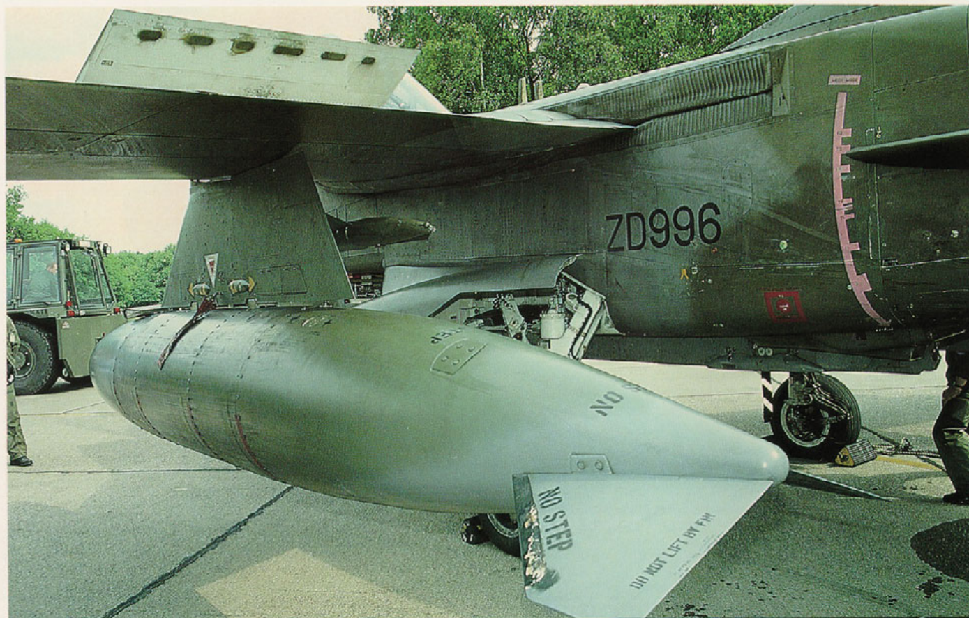
Close view on the aft part of the external fuel tank and stabilizer fins. "NO STEP" markings can be found all over the aft part of the tank. Two more stabilizer fins can be mounted on top of the tank at either side of the centerline. Note the black aircraft serial number below the flexible wing seal and the pink tailplane incidence marking on the right.
