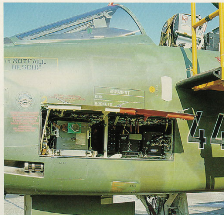
Left: Luftwaffe version of the battery compartment and adjacent markings. Note the armament panel above the compartment.
