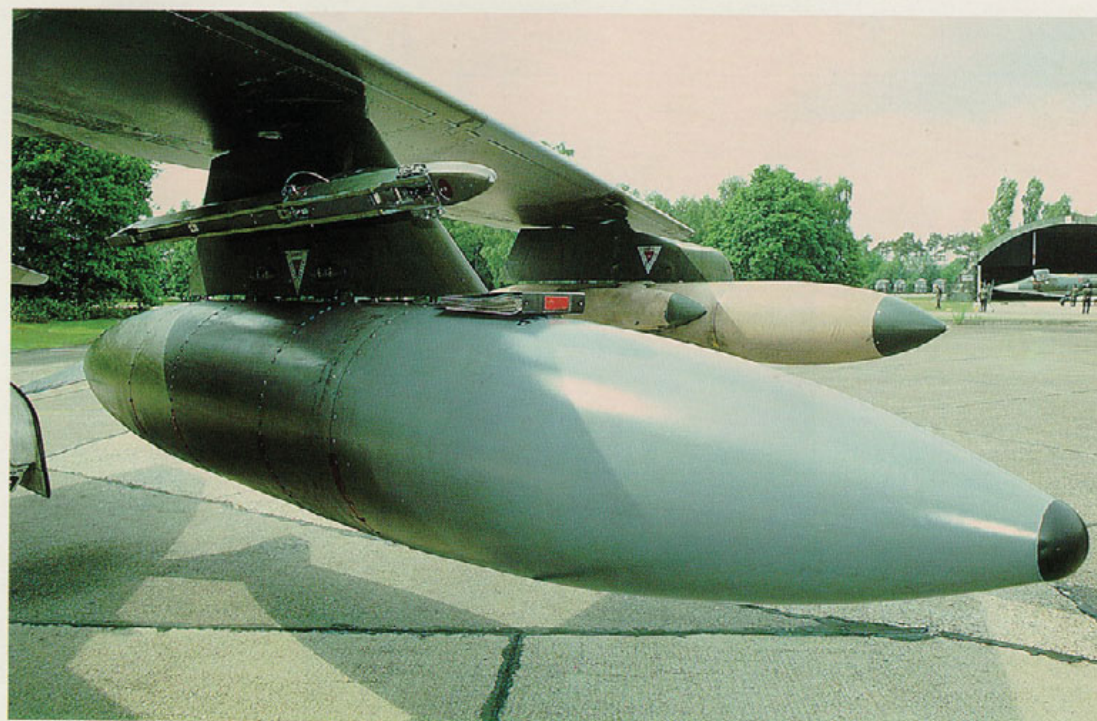
Sidewinder air-to-air missiles can be fired from launching rails mounted inboard of the pylon. Note the aircraft maintenance registration manual on top of the tank and inboard detail of the Sky Shadow ECM pod.
