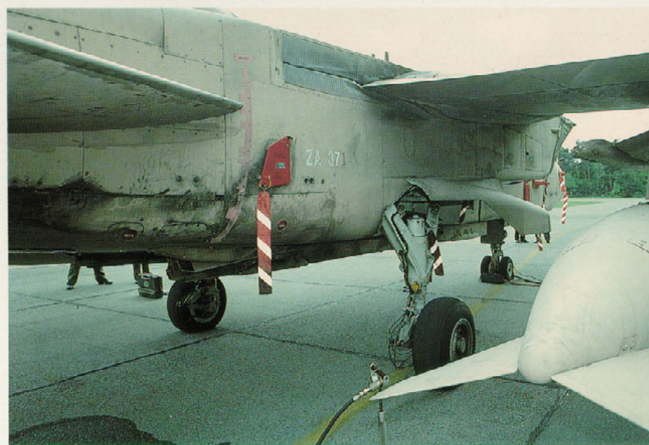
Heavily weathered rear of ZA371 showing the panel lines in this area. Clearly visible is the high ground clearance of the Tornado reducing the risk of engine flameout caused by FOD (Foreign Object Damage) both on concrete and unprepared runways.
