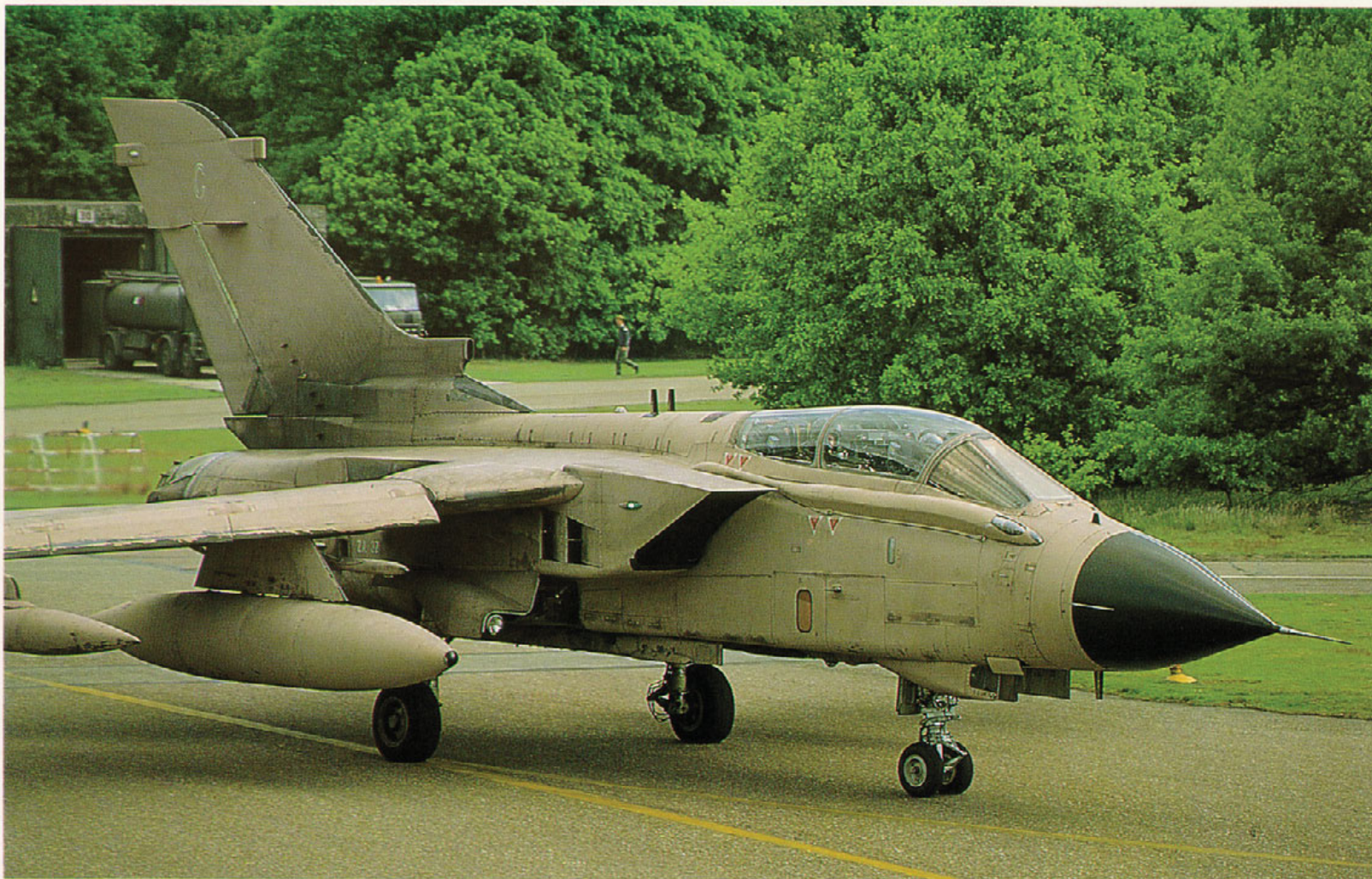
Photographed only weeks after its return from the Gulf, this Tornado ZA 371/C is heading for the runway. Note the panel in front of the air intake which has an oval window, a remainder of its operation over Iraq. It is part of the aircraft's reconnaissance equipment and covers sideways looking thermal imaging sensors. A similar window is on the opposite side. The intake suction relief doors are open while the aircraft is taxiing.
