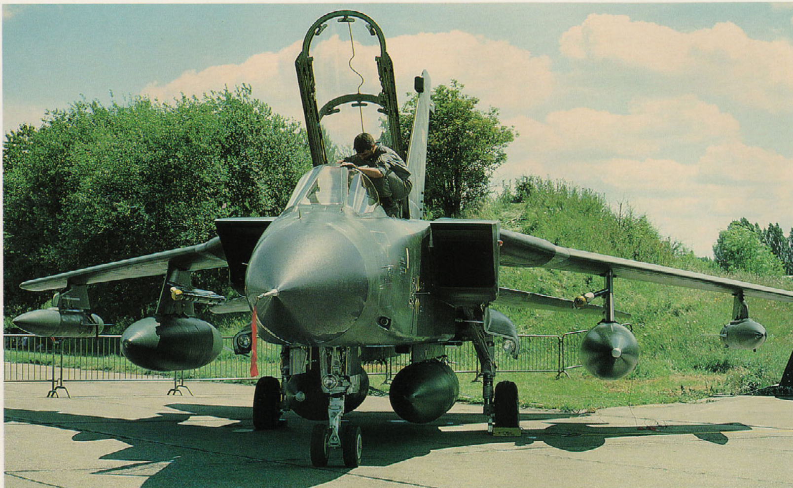
German Tornado with a full load of four external fuel tanks, one each on the inboard pylon and one on the outer fuselage shoulder pylons. Dummy practice missiles are mounted on the inboard Sidewinder launching rails while chaff/flare dispensers are attached on the outermost pylons.
