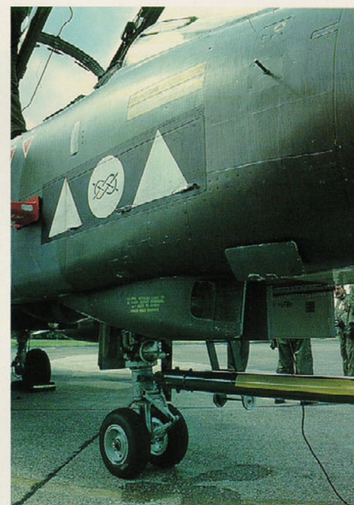
Close up of the LRMTS or Laser Range-finder and Marked-Target Seeker located on the right and in front of the nose gear door. When illuminated by the crew it provides a laser beam to guide homing weapons to the target. Note the auxiliary power receptacle just above the LRMTS and the angle of attack probe just aft of the radome.
