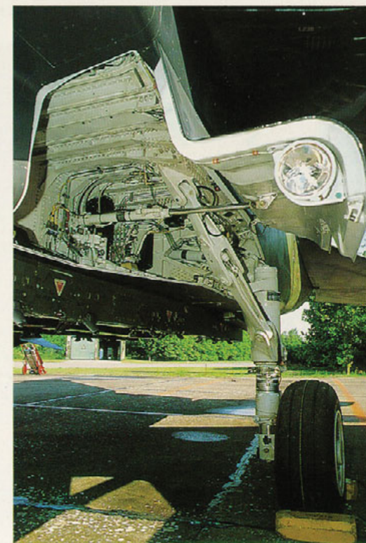
Left: Right rear view of the nose landing gear in overall white finish. Note the spring just above the landing light.
