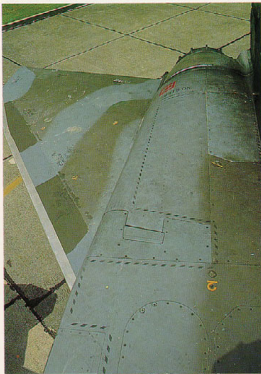
Overhead view of the starboard tailplane and airbrake. Note the bare metal leading edge of the tailplane and the hoisting point marking in the bottom right of the picture. Again note how various panels have been replaced, indicated by the difference in color.
