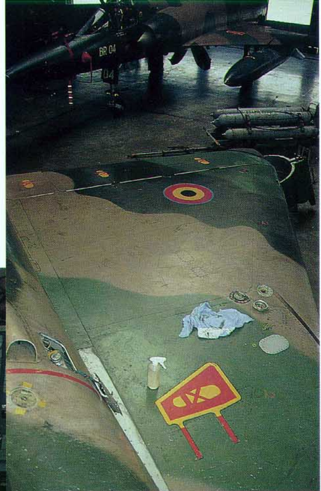
(Right) Upper wing detail on the left side. The wing root fuel tank cover can be seen next to the dog tooth on the right.
