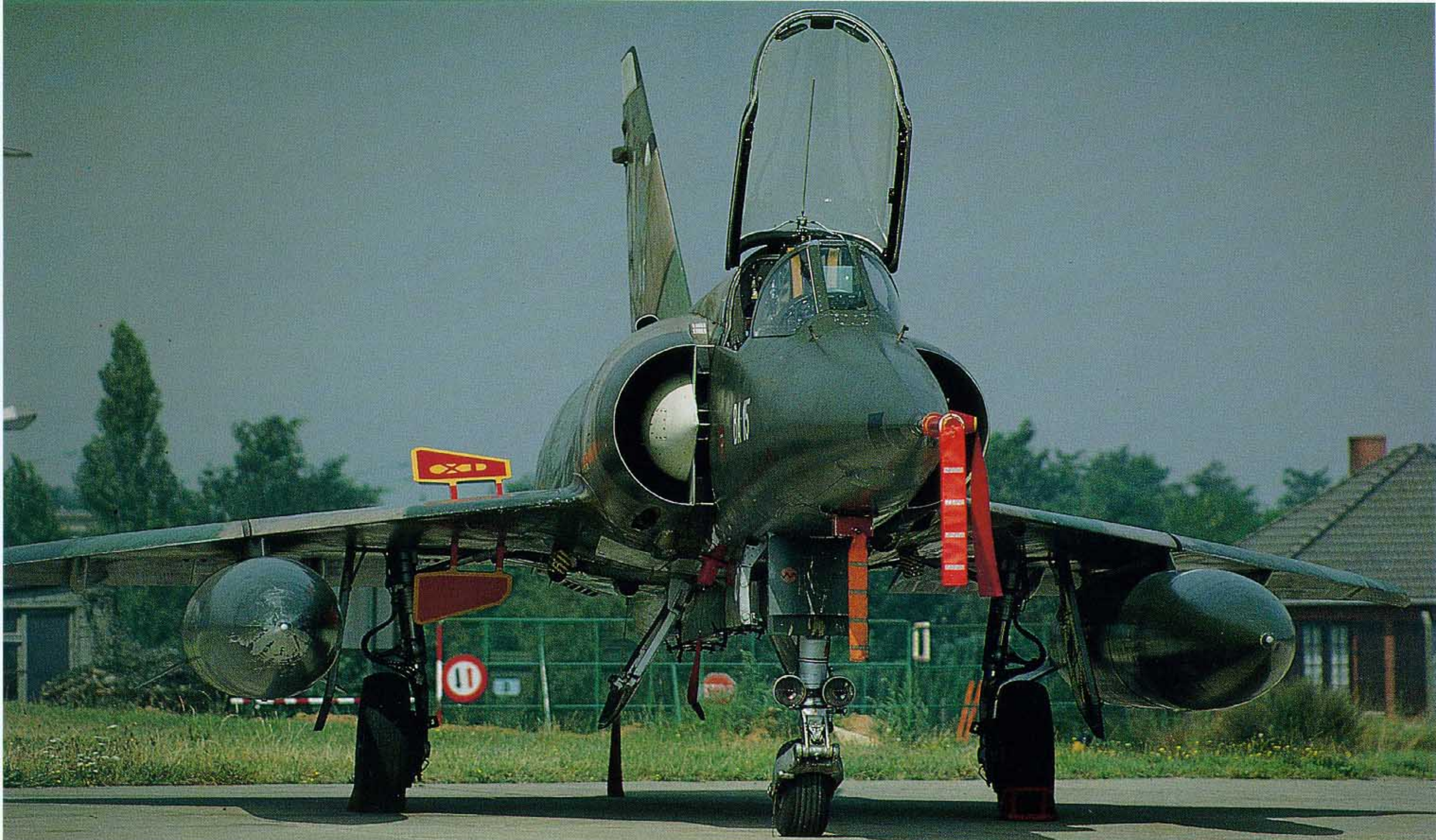
(Top) Belgian Air Force MIRAGE V (BA15) parked on the outskirts of Bierset Air Base showing to good advantage the dual speedbrakes and the distinctive "NO STEP" marking on the upper speedbrake. The sleek lines of this DASSAULT design stand out very clearly when viewed from this angle.
