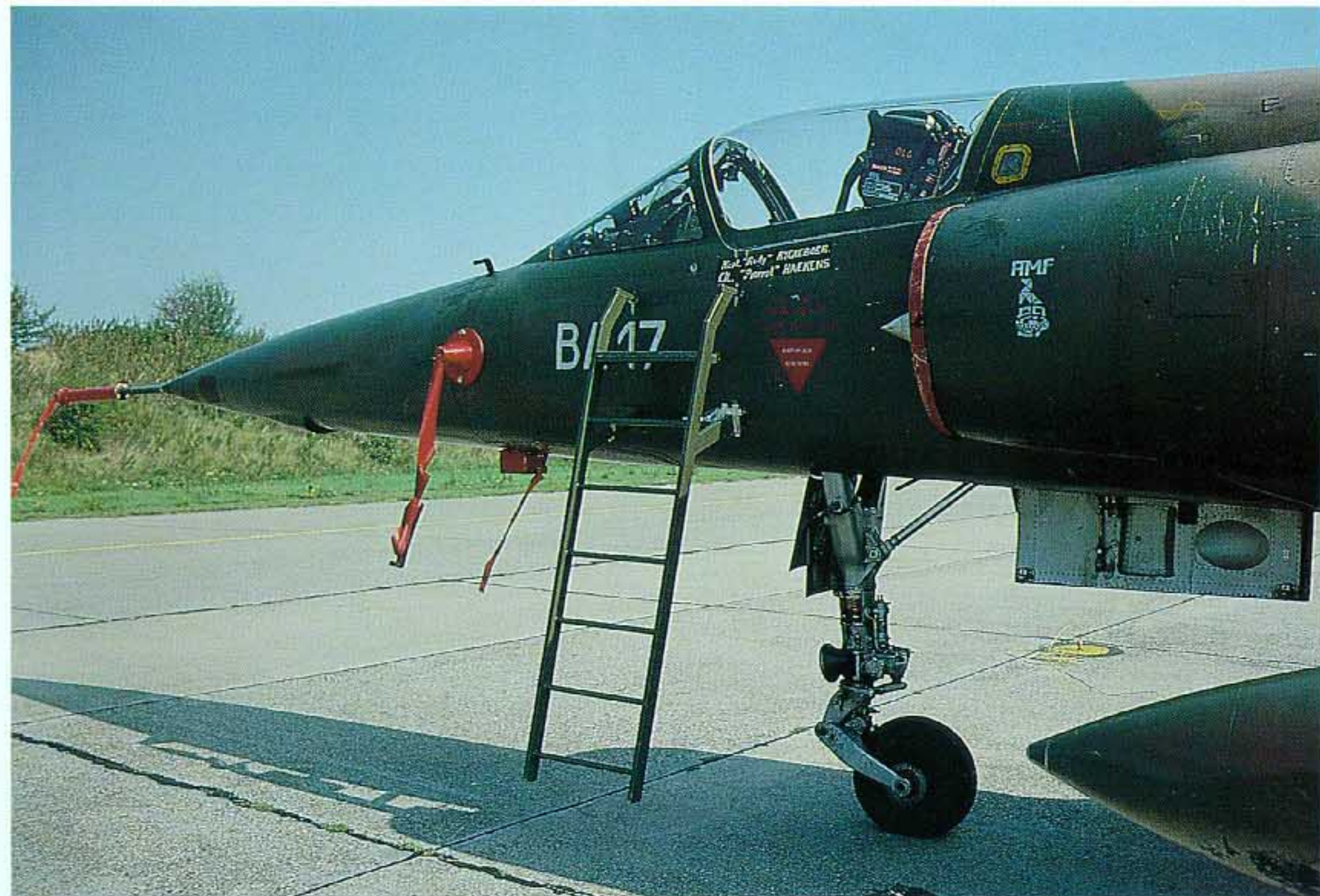
A small ladder can be attached to the left fuselage side slightly in front of the canopy. Note the cover over the static port (aside) and the lower DOPPLER antenna (bottom) on the nose. Also note the small emergency rescue window (marked in yellow) just aft of the canopy.
