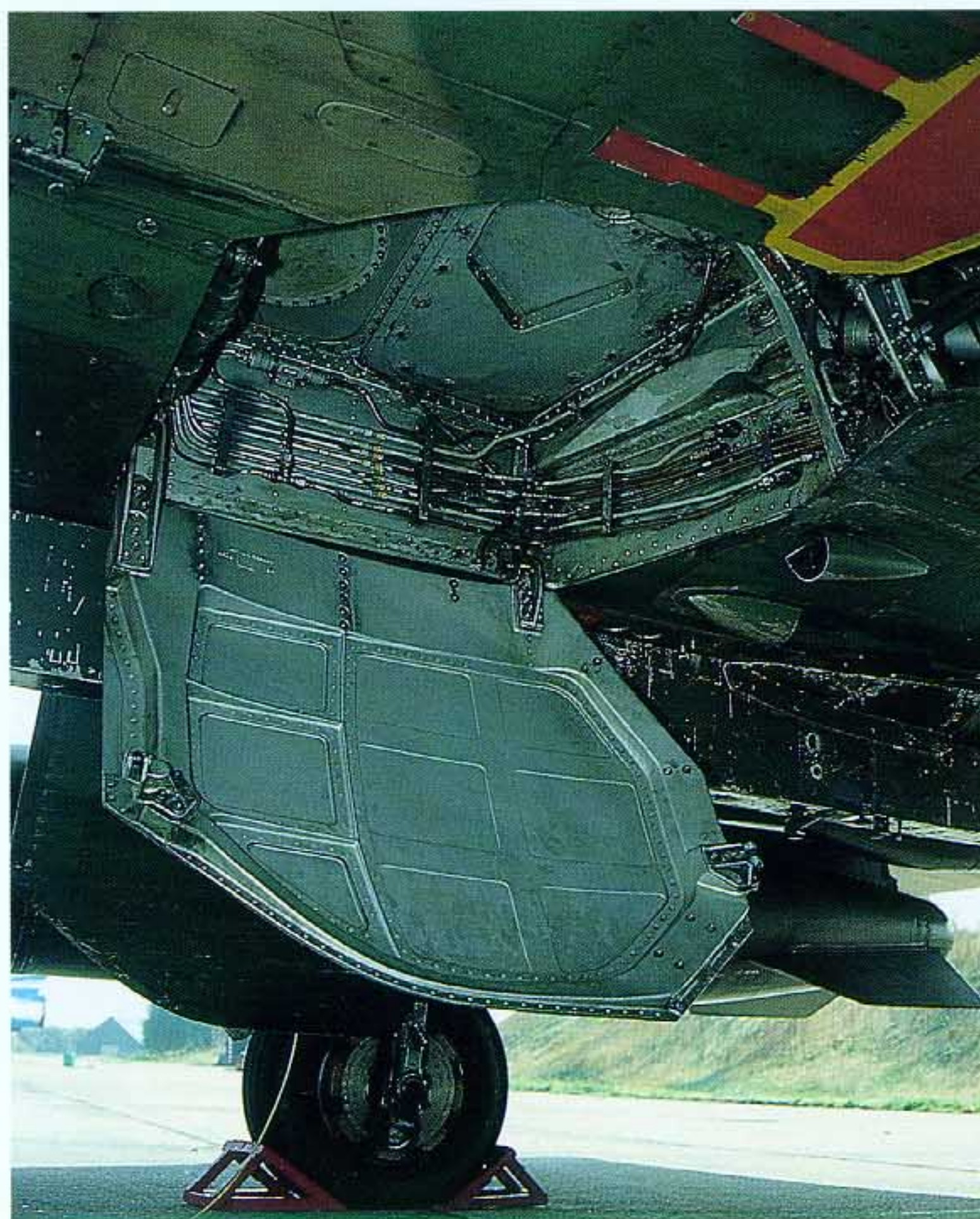
(Top left) Bottom detail of the area between the main wheel wells with a close view on the rear of the center pylon. Note the white TACAN antenna at the top of the picture.
