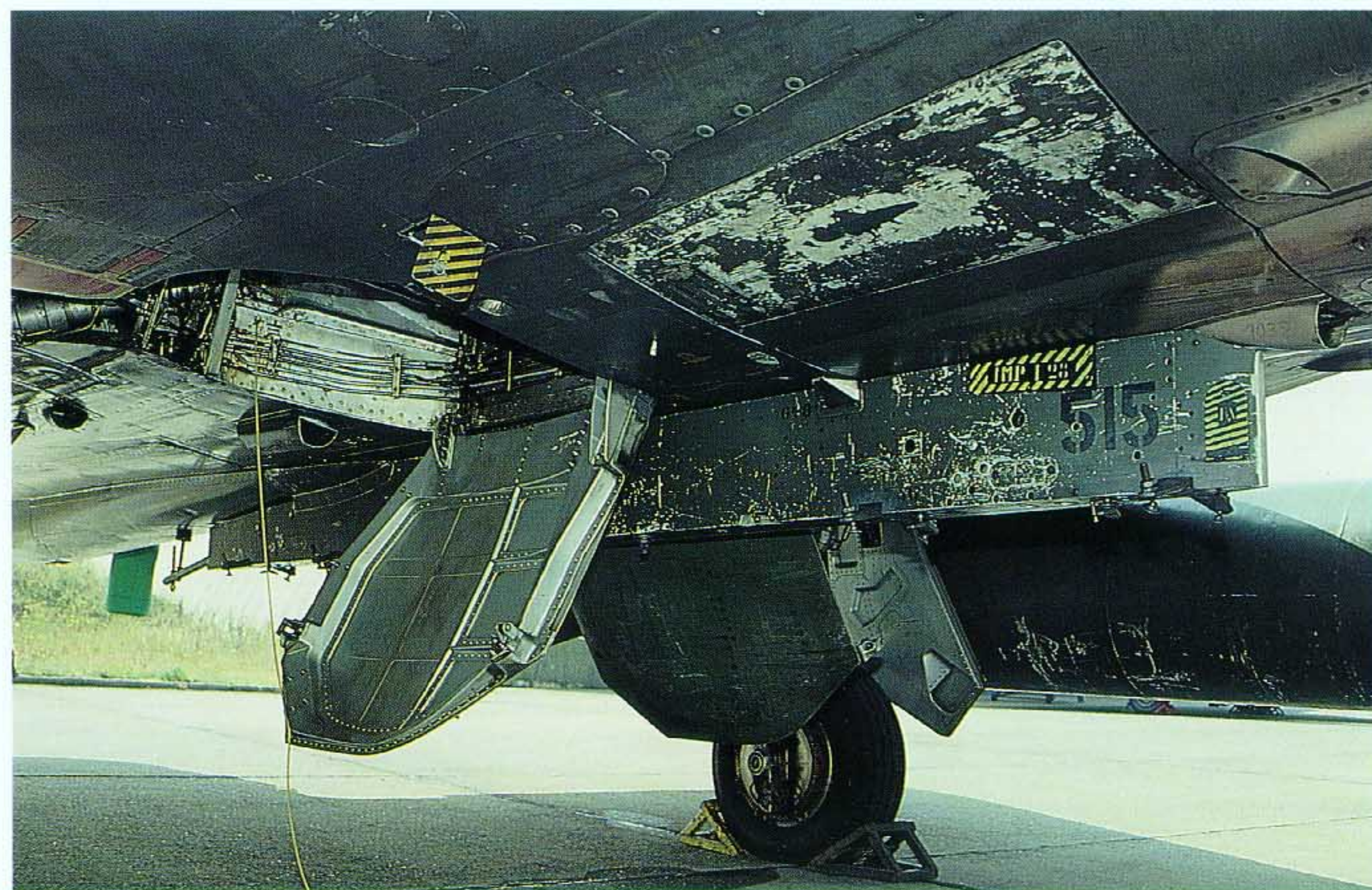
(Right) A severely weathered center pylon which runs all the way through to the ventral spine on the aft side of the fuselage. The chipped-off panel aside the front of the pylon gives access to the gun (one on each side) and is part of a gun pack which can be seen on the next page. Inside detail of the bare aluminum main gear door is also clear.
