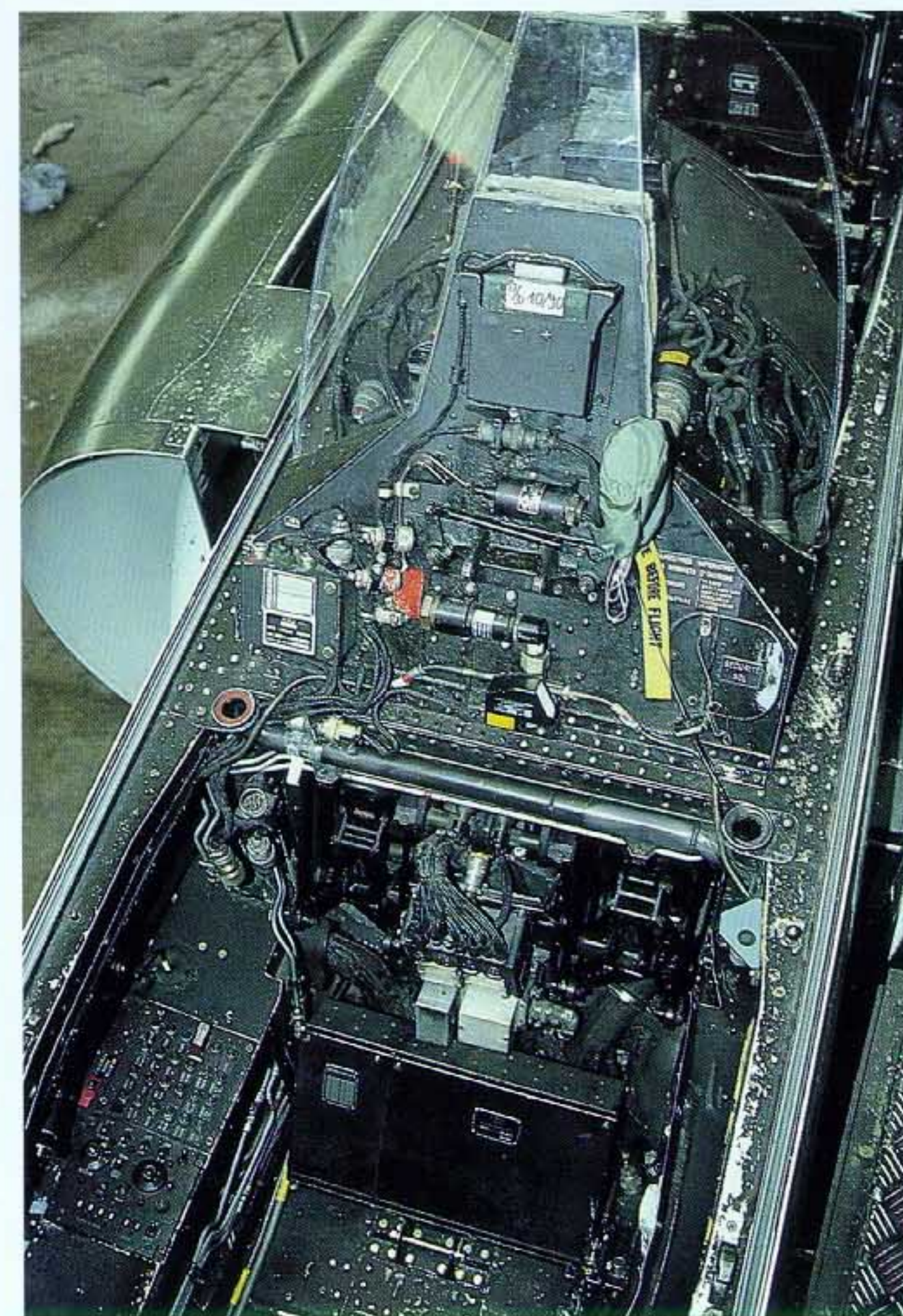
(Above) A photo to show the twin seat Mirage has the same front cockpit as the single seat variant. Of special interest is the small placard holding radio call signs just in front of the canopy frame on the right and the area underneath the ejection seat revealed in this view.
