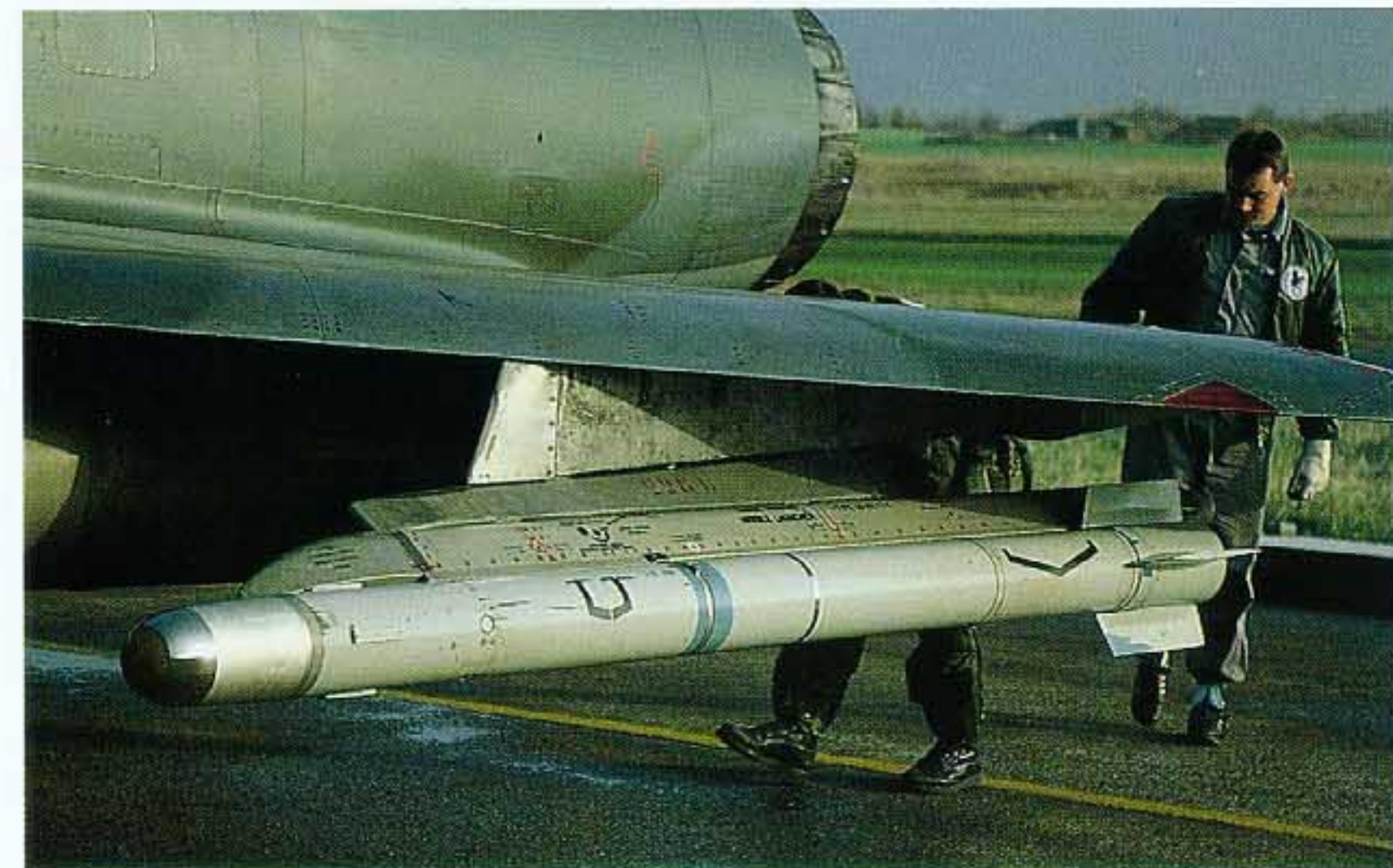
The limited number of external stores had the French looking for additional hardpoints such as the ones on the inner pylon fuel tank. A side-mounted launching rail on the outer wing pylon was designed to use the deadly "Matra Magic" missile. (All photos by Marck De Boeck)
