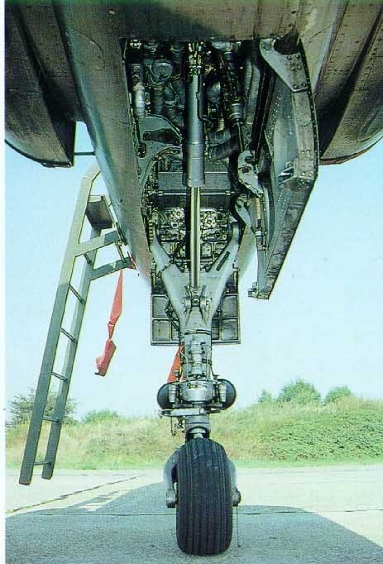
(Top) A single strut retracts the nose gear into the nose gear well which has a bare aluminum color. Note the distance between the air intakes and the fuselage.
