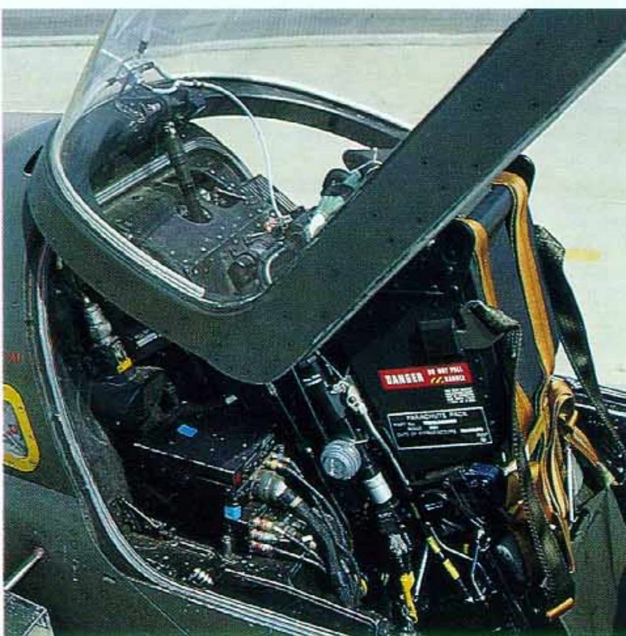
The installation of the new Mk10 seat was combined with the installation of a detonation cord inside the canopy glass.
