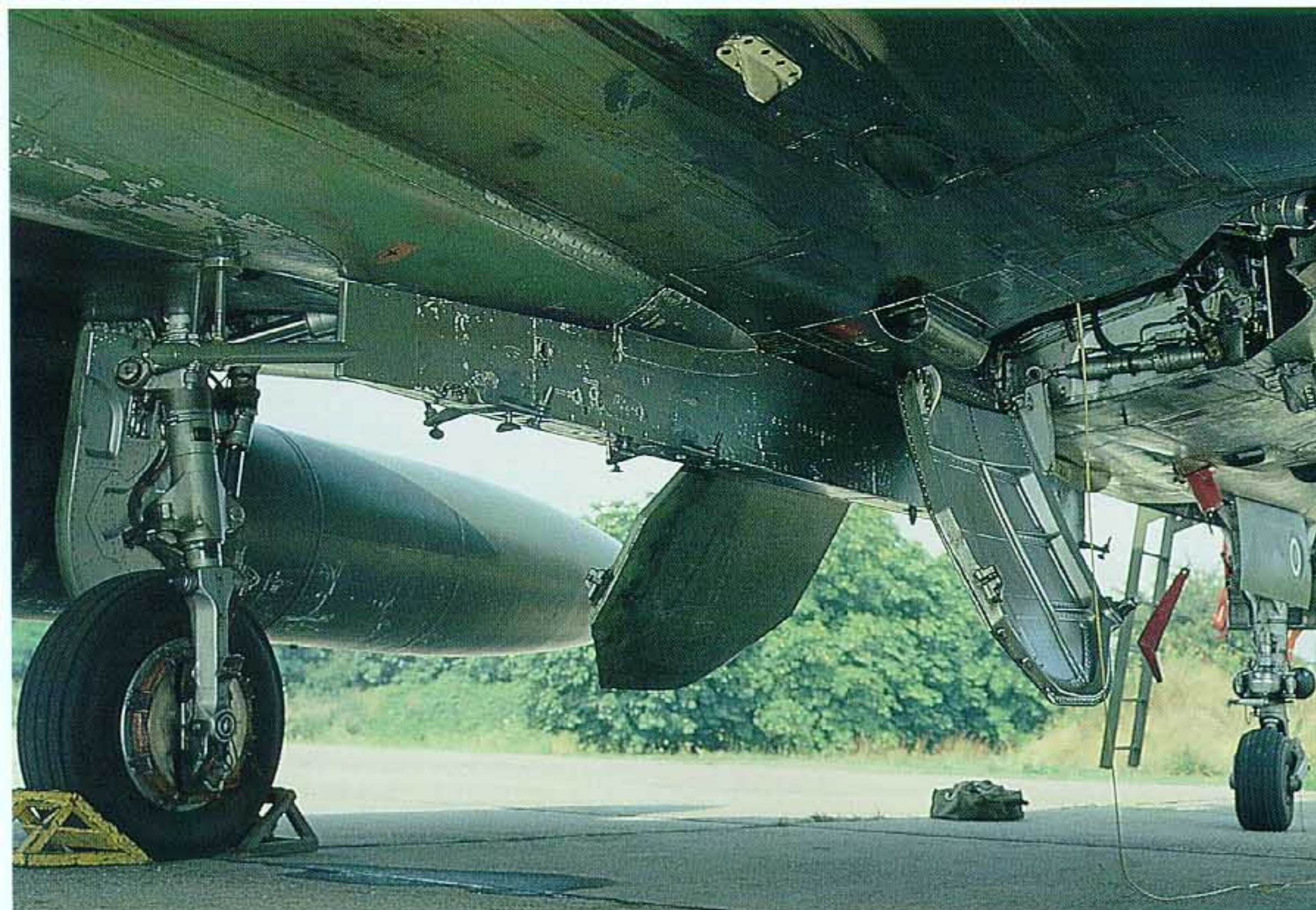
(Top left) Bottom detail of the area between the main wheel wells with a close view on the rear of the center pylon. Note the white TACAN antenna at the top of the picture.
