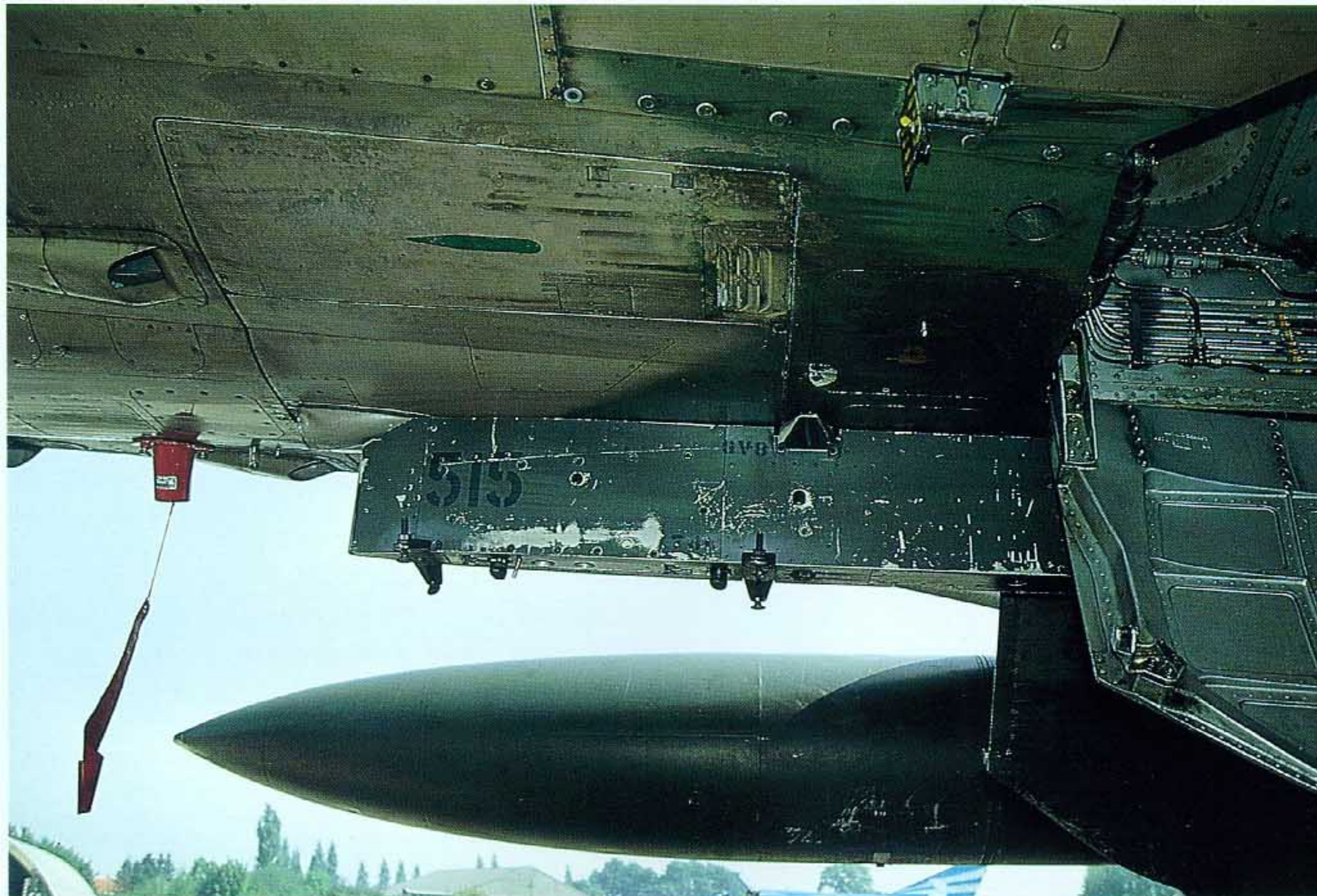
The opposite side of the center pylon with the left side gun door in the center of the picture. Extensive use of the aircraft leaves a lot of scratches and chipped-off panels which will be replaced or overpainted when major overhaul is executed.
