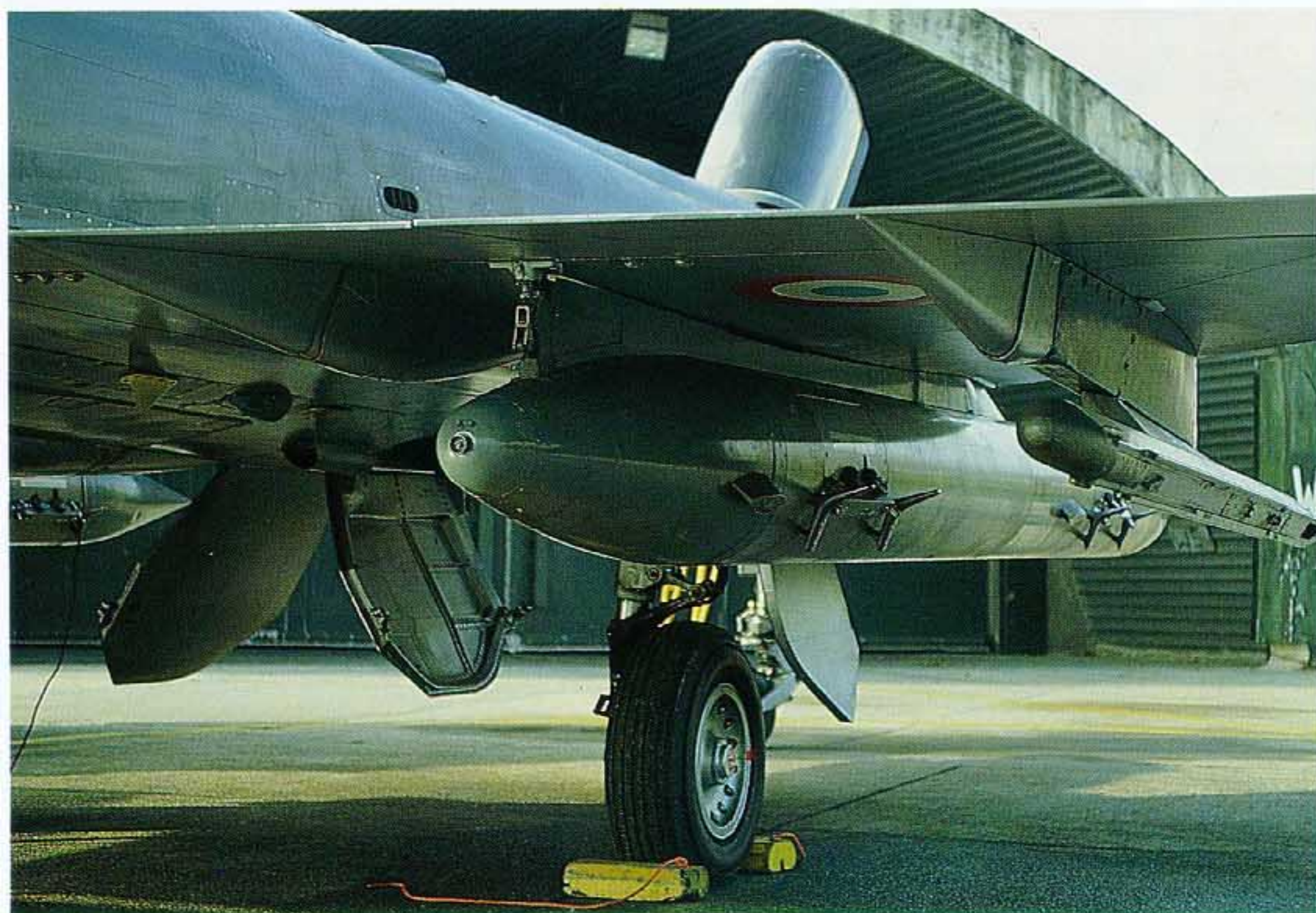
The limited number of external stores had the French looking for additional hardpoints such as the ones on the inner pylon fuel tank. A side-mounted launching rail on the outer wing pylon was designed to use the deadly "Matra Magic" missile. (All photos by Marck De Boeck)
