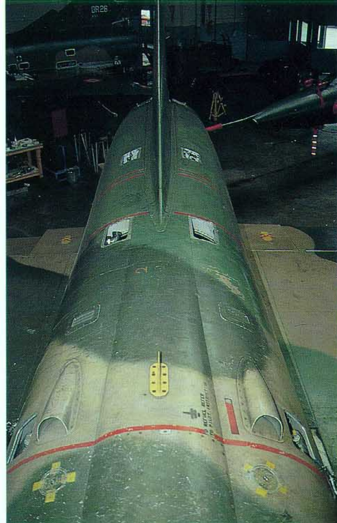
A view of the upper spine looking aft. The red band marks the front end of the engine. The upper TACAN antenna and the auxiliary air intakes can be seen just aft of it. The two small round access panels in front give way to the hydraulic reservoirs.
