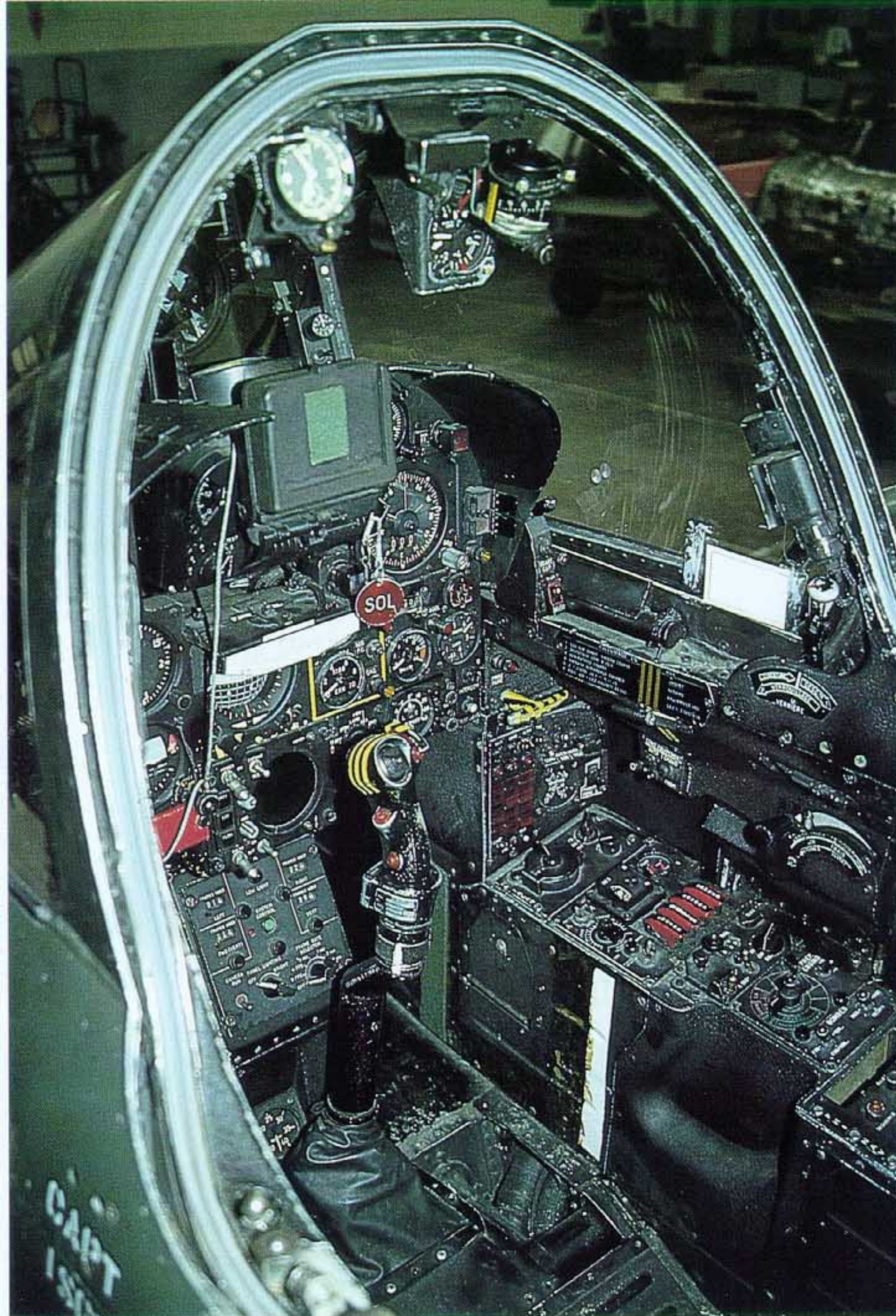
(Above) A photo to show the twin seat Mirage has the same front cockpit as the single seat variant. Of special interest is the small placard holding radio call signs just in front of the canopy frame on the right and the area underneath the ejection seat revealed in this view.
