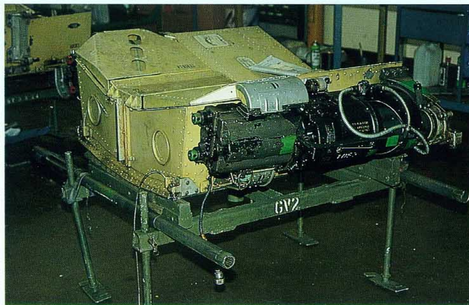
Two 30mm DEFA cannons are side-mounted to a removable ammo pack which weighs 356 K's. The 80 k's heavy guns are interchangeable and are powered by a 24 volts electrical current. The two gun barrels can be seen in front of the pack.
