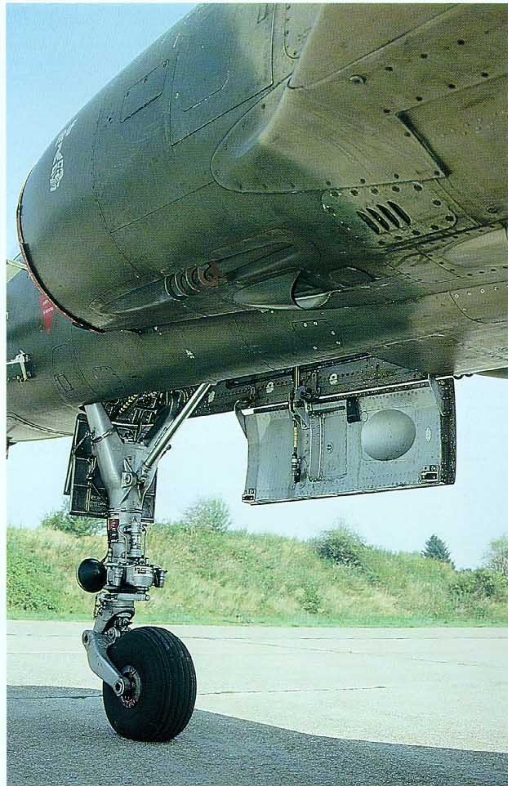
The lower side of the left air intake with a good view on the wing root housing. Just below it can be seen the gas exhaust vent of the gun. Note the inside detail of the nose gear door.
