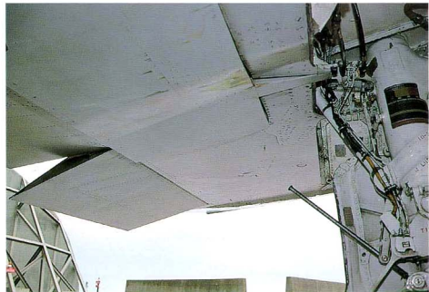
The bottom speed brake just aft of the main gear well. Part of the latter can be seen at far right.
