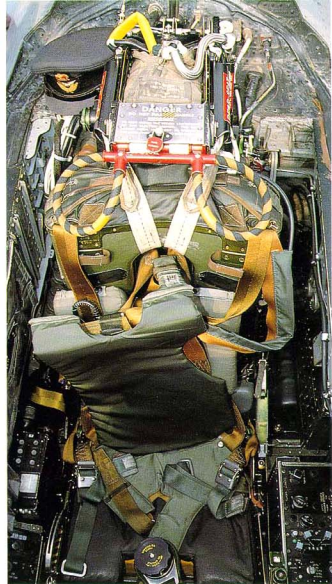
(Top) An overall top view of the rear ejection seat with the combine harness and the parachute lift webs (orange straps) clearly visible. The actual parachute is packed inside the pack just below the headrest. Also note the light gray back pad behind the combine harness. Rear cockpit detail is also visible.
