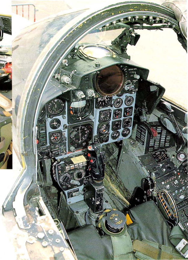
The front office of an FGR.2 in detail and part of the area behind the seat. Note the multitude of colors and the new style pilot helmet on top of the seat headrest.
