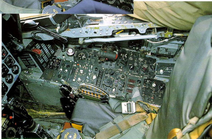
(Left) The left side console of the front cockpit. Layout is different than of its US counterparts as a close study will reveal. Part of the cockpit defogging system can be seen behind the yellow cockpit jettison handle. The red panel below the landing gear actuating handle is a safety pin stowage and control panel. At the right front of the dual throttle levers can be seen the Bullpup control knob. Also note the sidewinder launch control panel on the far end of the side console.
