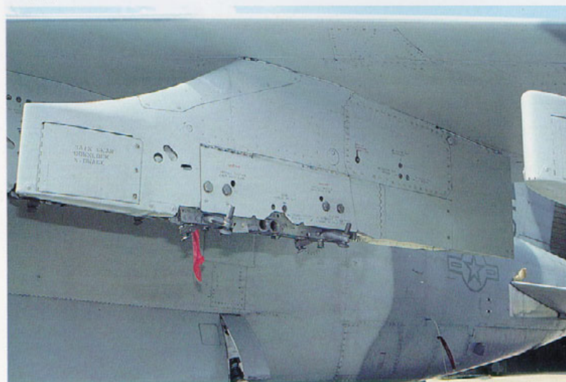
Surface detail of the center wing pylon with the main gear downlock stowage housing in the pylon leading edge. The downlock device is shown on page 6, bottom left picture.
