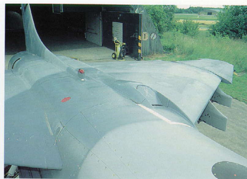
The upper fuselage with the upper TACAN antenna (far right), the inflight refueling receptacle (air force A-7 location, replacing the navy's side-mounted nose probe), and the upper anticollision light. The white light just in front of the latter is a formation light.
