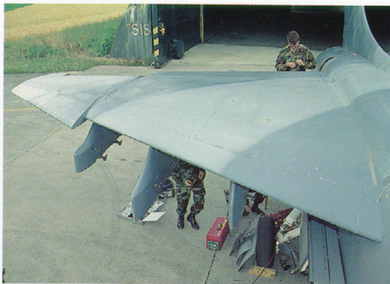
The upper surfaces of the starboard wing show little detail. The camouflage pattern can however be distinguished. Note the perfect integration of the leading edge slat in the wing.
