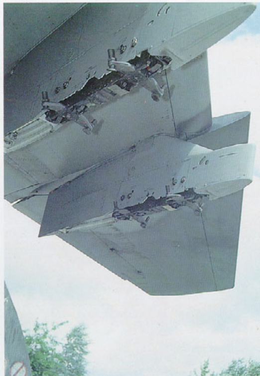
The center and outer wing pylon viewed from the same spot. Note the "dog tooth" in the wing leading edge.
