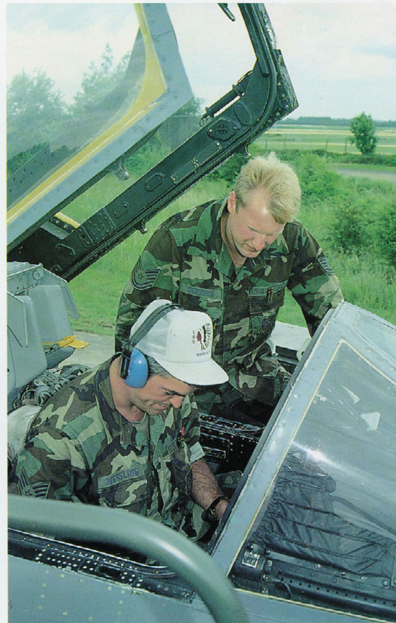
Sgt Wessling and Sfc Schreck conducting tests on the aircraft's navigation system. Most interesting in this view is the canopy inner frame and the canopy piercing knife mounted on the frame. When looking through the perspex windscreen on can see the pouches mentioned earlier from above. Note the yellowish canopy seal.
