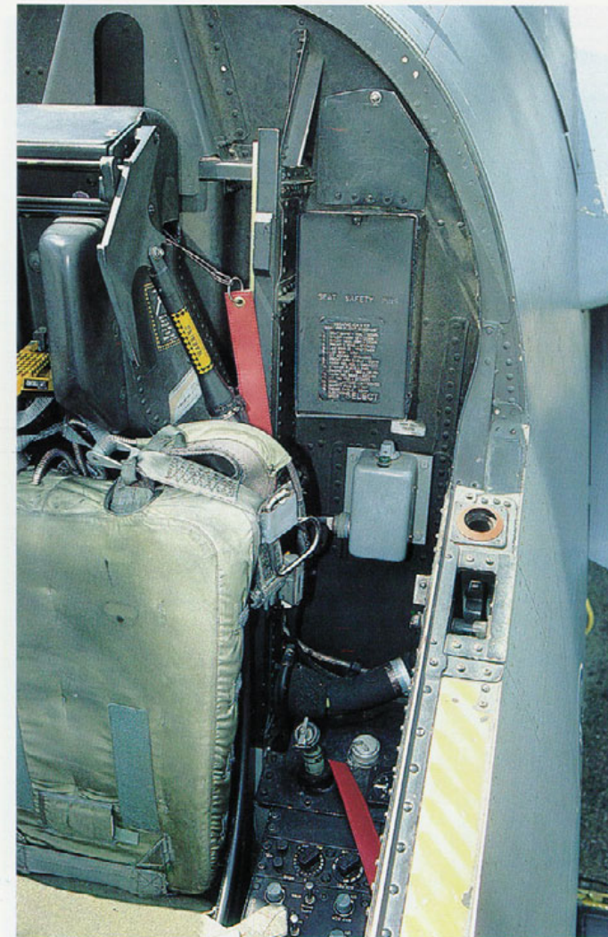
(Below) Left of the rear cockpit seat is seat safety pin stowage box which features a seat pre-flight checklist. Note the various safety pins installed to the seat and to the rest of the cockpit.
