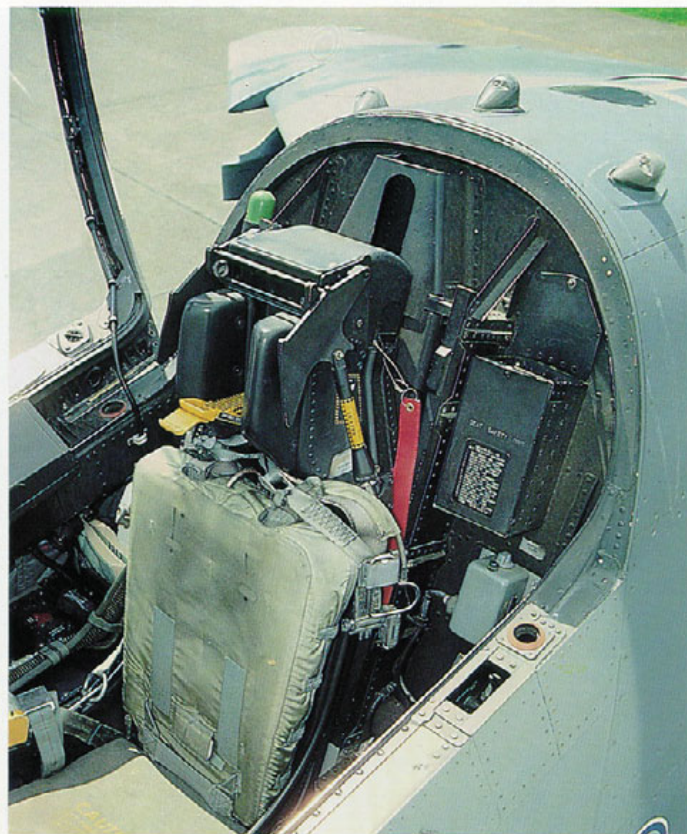
(Left) The seat viewed from the right side of the aircraft. This time it is an 1C-5 ESCAPAC which was developed to fit in the rear cockpit. The position of the three refueling floodlights can be determined.
