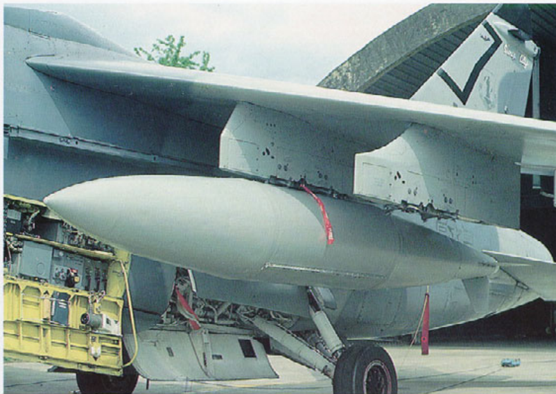
The 300 gallon fuel tank features only three stabilizing fins, lacking one on top. Note the reinforcement/hinge at the lower part of the tank.
