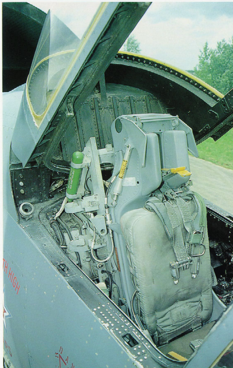
An overall view of the ESCAPAC 1C-2 ejection seat and the area behind the seat. The oxygen hose and voice connector cable can be seen aside the ejection seat launching assembly. The rubber-covered outlet on the aft cockpit framing is part of the canopy climatization and defogging system. Note the aft inner bulkhead of the raised canopy and the canopy seal.
