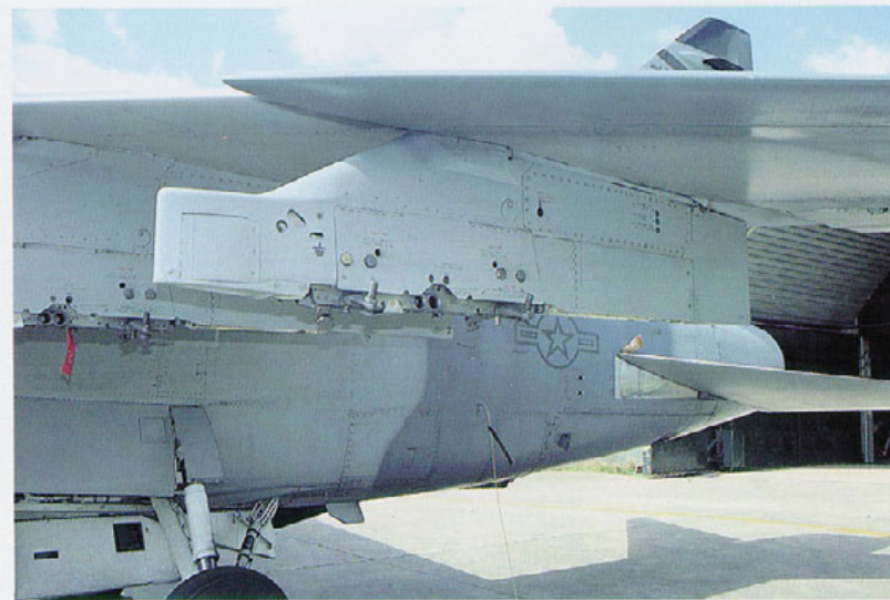
Panel detail of the most outboard wing pylon. Note the different shapes of the pylon's leading edges. Nevertheless, they all feature the same attachment racks.
