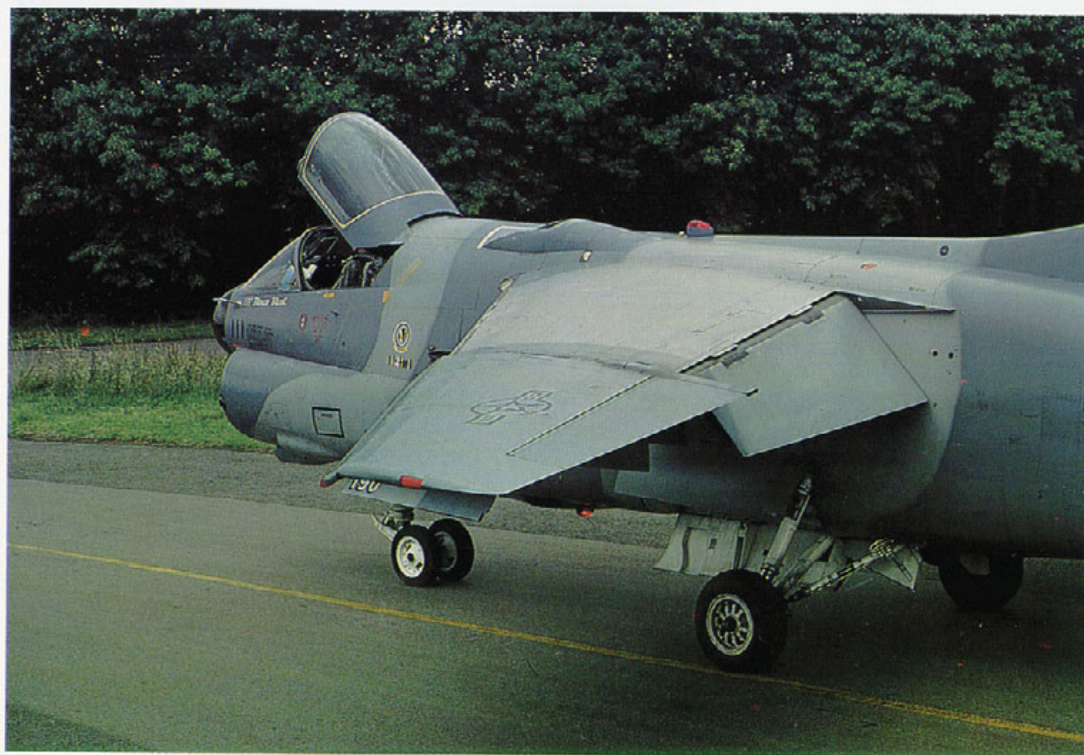
An A-7D (72-190) seen taxiing towards its shelter after an uneventful cross-country flight. An interesting photo because it shows the landing flaps and the leading edge slats in the down position, as well as the other side of the inflight refueling receptacle. Note the through-the-wing spoiler just in front of the lowered flap.
