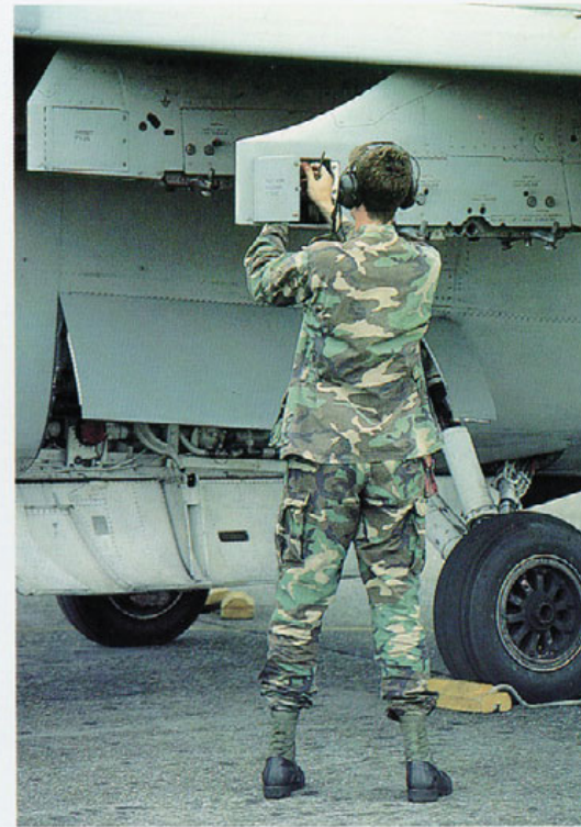
Safety pins are stowed in the front housing of the pylons as demonstrated by this ANG crewmember.
