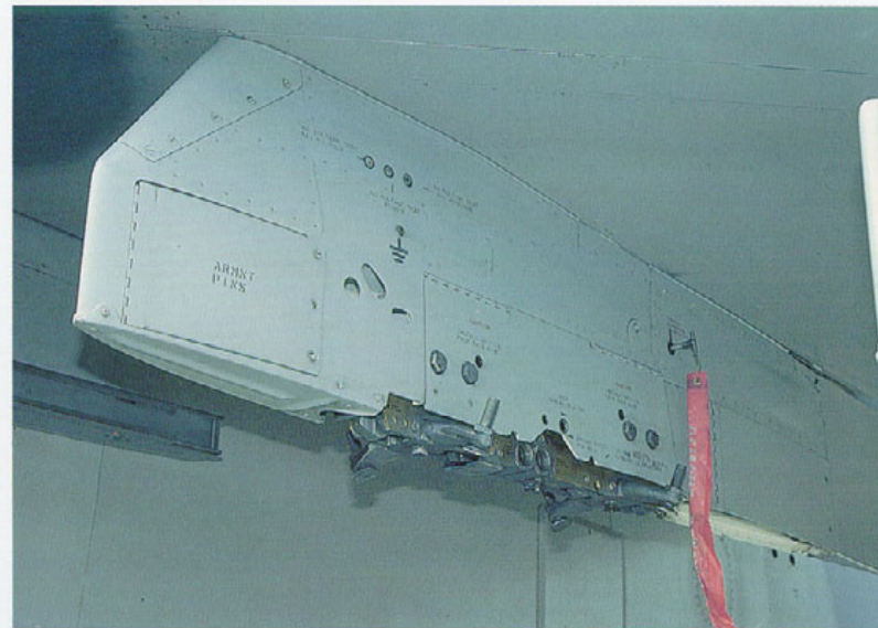
Obscured when viewed from aside, the inboard pylon itself has some detail worth showing. Note the A-7 pylons are firmly attached to the lower wing surface, leaving no gaps at all.
