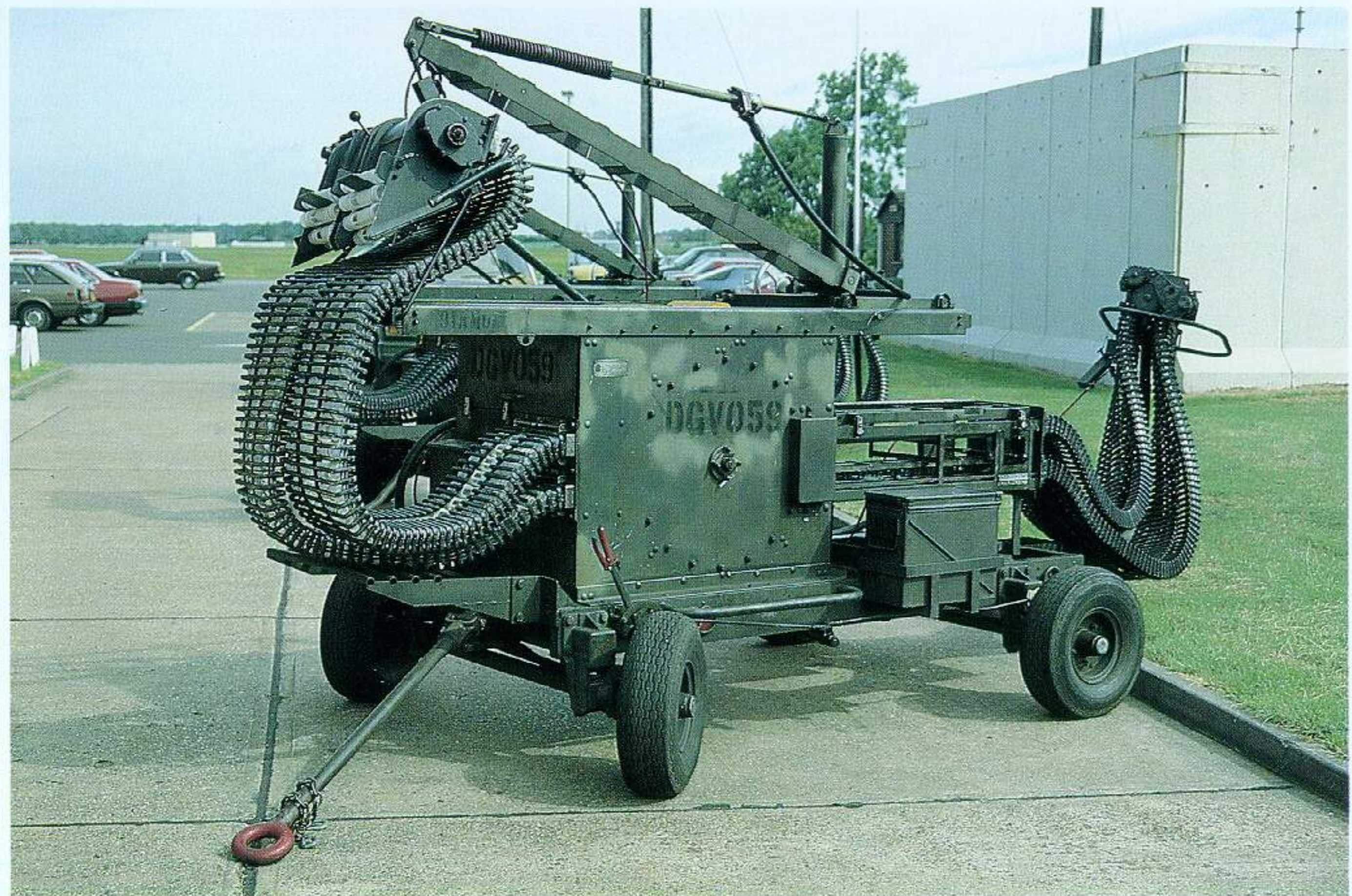
Loading the linkless A-10 ammo is done with this special piece of equipment, the Ammunition Loading System (ALS) platform. The principle is the same as that of the GAU-8/A gun itself. It loads rounds on one side and extracts empty cases simultaneously. A full load of 4,200 rounds can be changed in less than 12 minutes under forced loading conditions.
