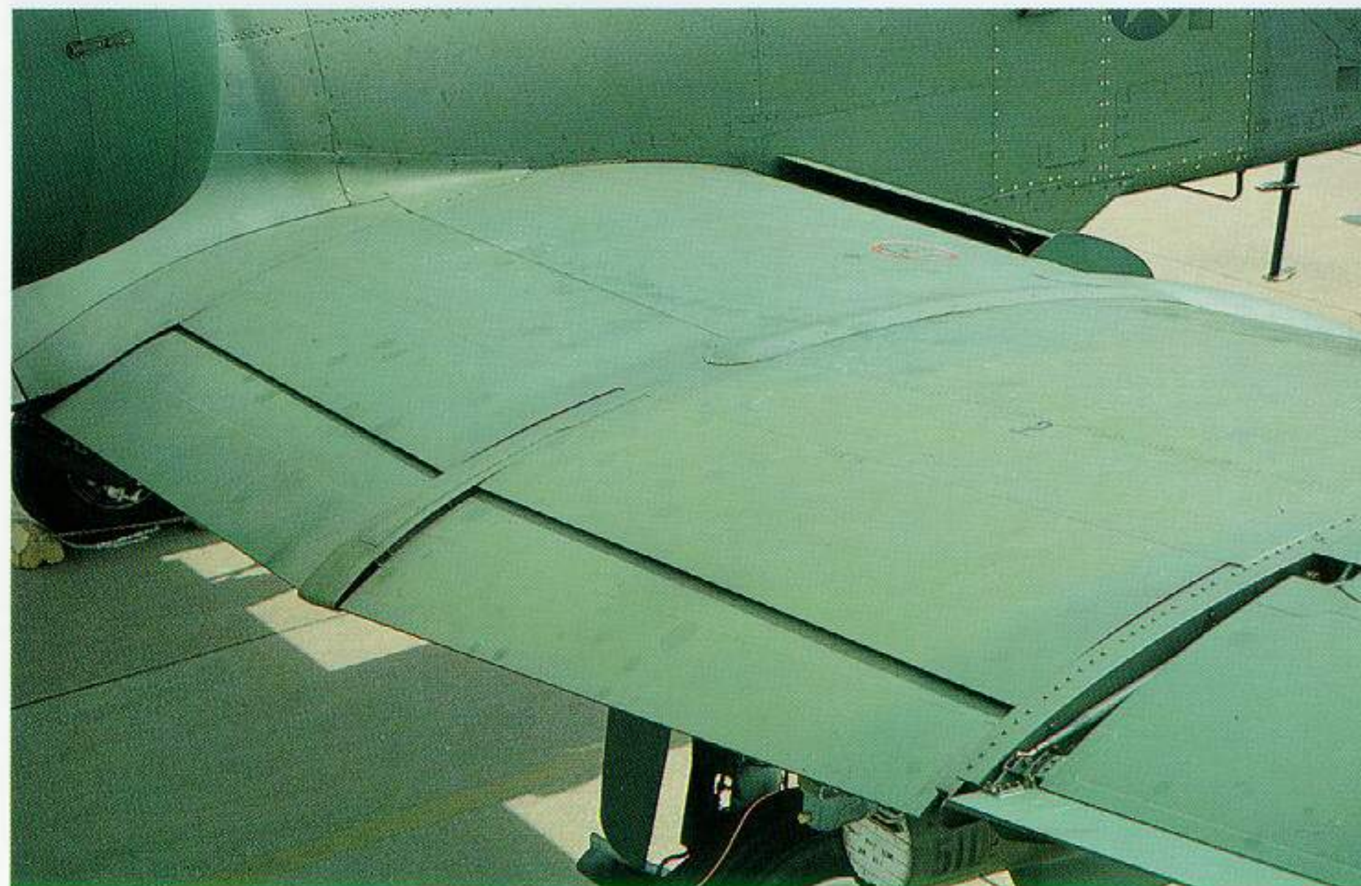
A different look at the underwing stores. Note the aileron actuating rod protruding from the rear of pylon 11, making the rear end of this pylon much wider than pylons 9 and 10. The picture at right shows the covered flare dispenser and wingtip navigation light. Part of the wingtip pitot-static boom can still be seen at right. Both bottom pictures show the right upper wing from above. Note the aileron trailing edge pitchup and the drooped wingtip.
