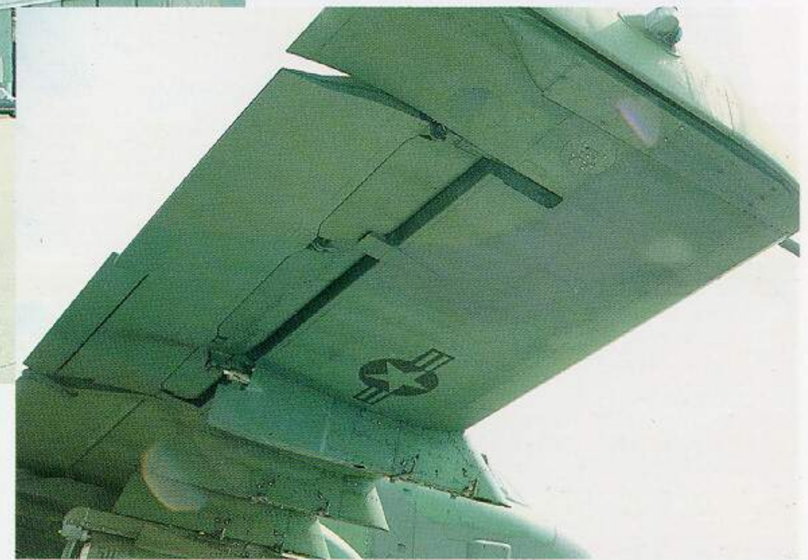
A different look at the underwing stores. Note the aileron actuating rod protruding from the rear of pylon 11, making the rear end of this pylon much wider than pylons 9 and 10. The picture at right shows the covered flare dispenser and wingtip navigation light. Part of the wingtip pitot-static boom can still be seen at right. Both bottom pictures show the right upper wing from above. Note the aileron trailing edge pitchup and the drooped wingtip.
