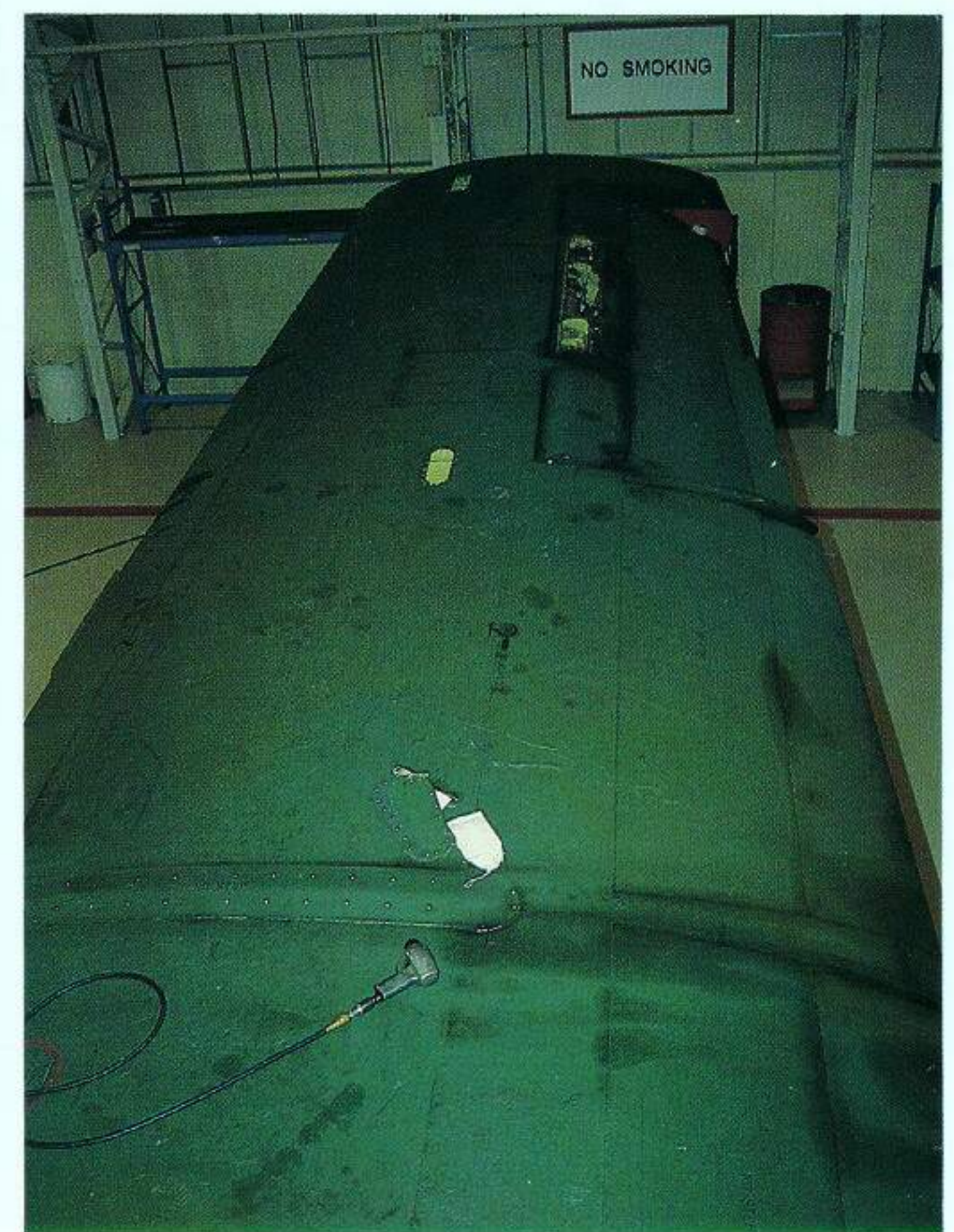
The front top fuselage with the panels described on the previous page at left. Note the shape of the aft side of the hood and the cover plate over the canopy actuating mechanism. Antenna designations can be found on page 20. The small exhaust at right and on top of the fuselage is the INS compartment coolant air outlet.
