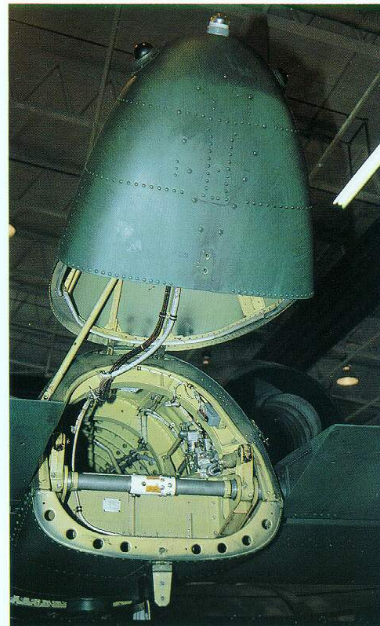
(Top) The complete tailcone can be raised to reveal the hydraulic elevator actuators and the elevator connecting bar. Feed lines running into the tail cone are for the tail-light and the radar warning antennas.
