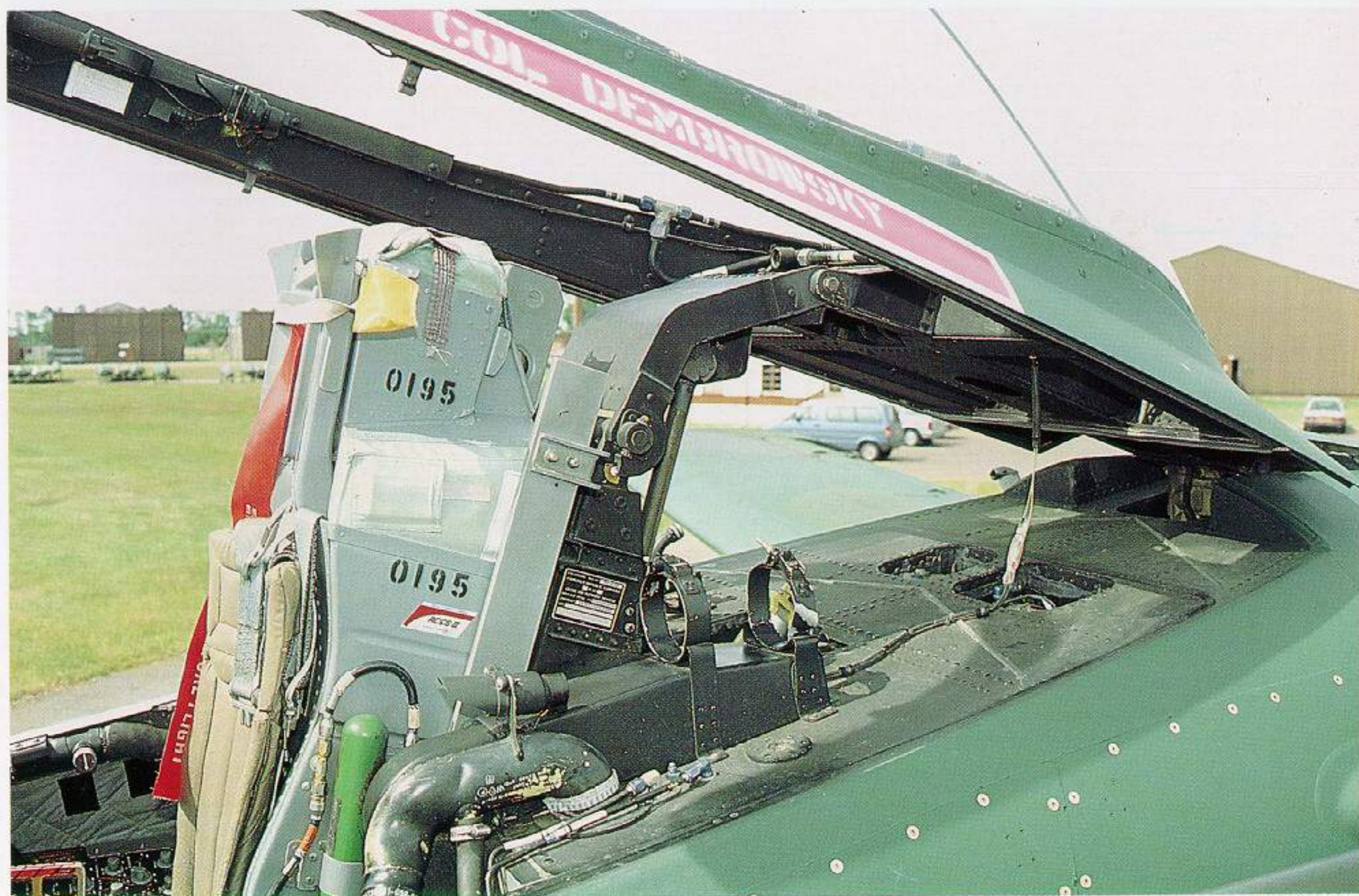
Side view of the ACES II ejection seat mounted in the A-10A. Noteworthy are the two canopy piercers atop the seat headrest, not found on the F-15 and the F-16 ACES II seat.
