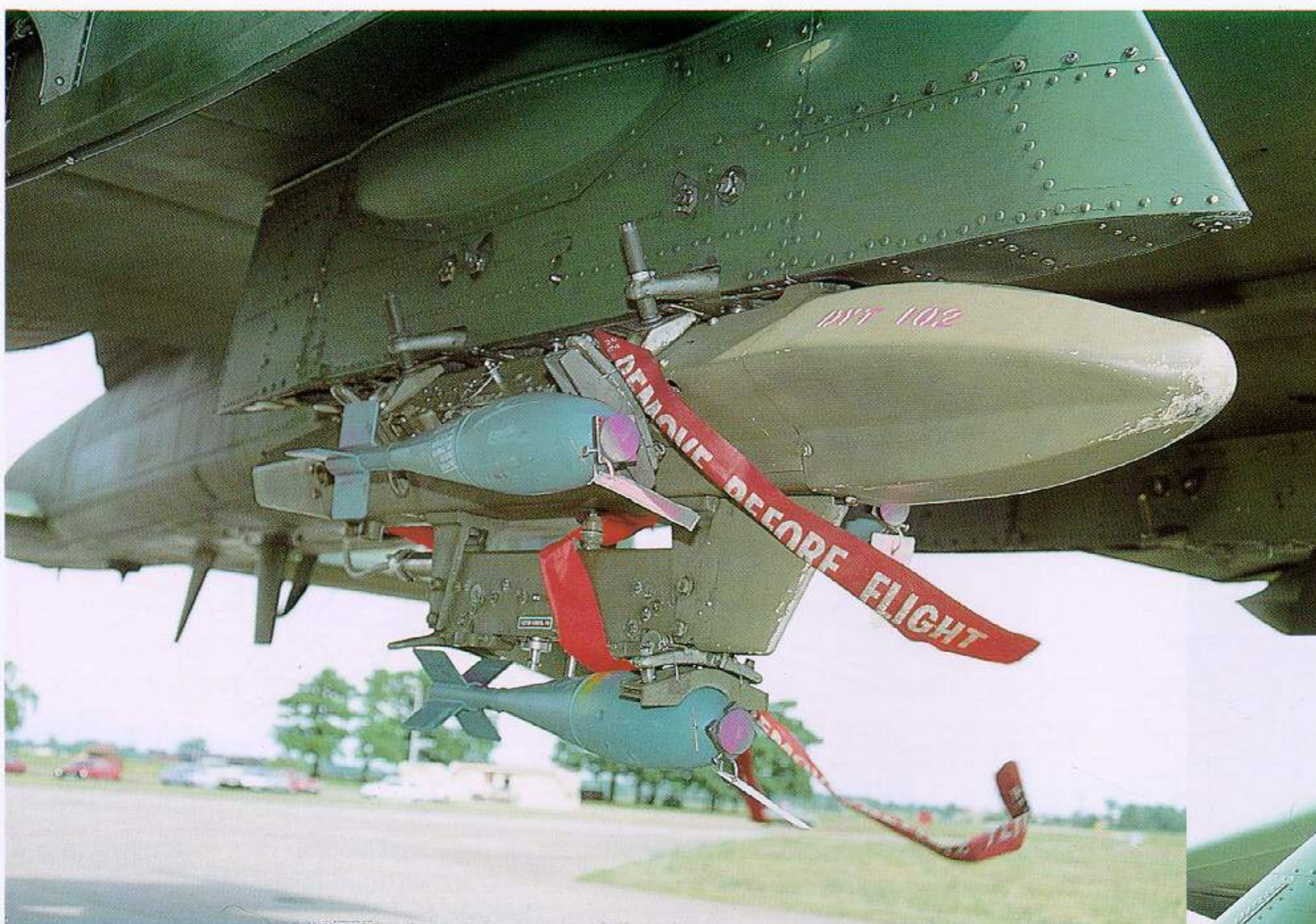
Three small BDU-33 practice bombs attached to a TER-9 or Triple Ejector Rack which is mounted to underwing station number 8. Note the different color of the TER-9 and the red and white stencilling.
