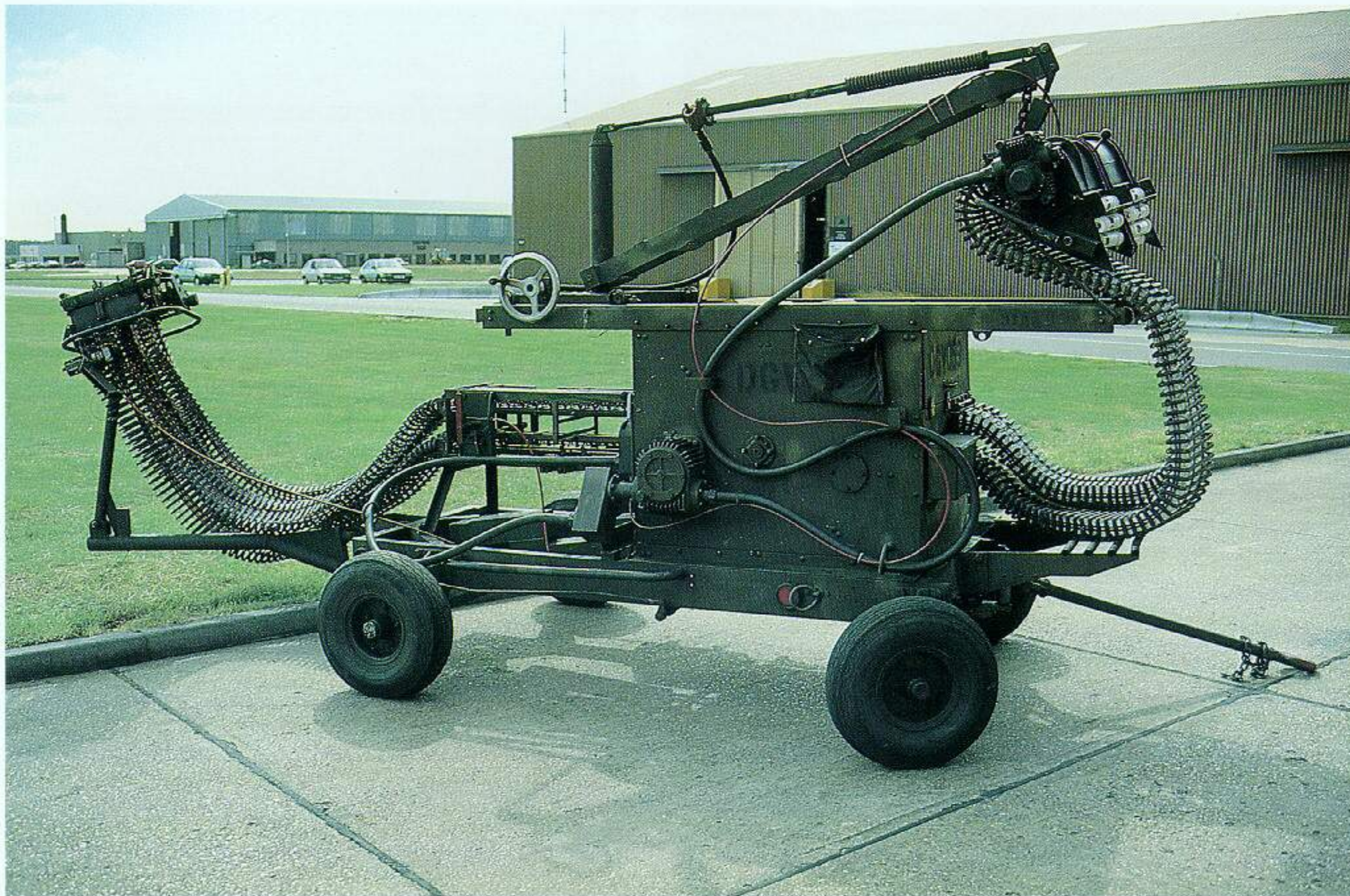
Loading the linkless A-10 ammo is done with this special piece of equipment, the Ammunition Loading System (ALS) platform. The principle is the same as that of the GAU-8/A gun itself. It loads rounds on one side and extracts empty cases simultaneously. A full load of 4,200 rounds can be changed in less than 12 minutes under forced loading conditions.
