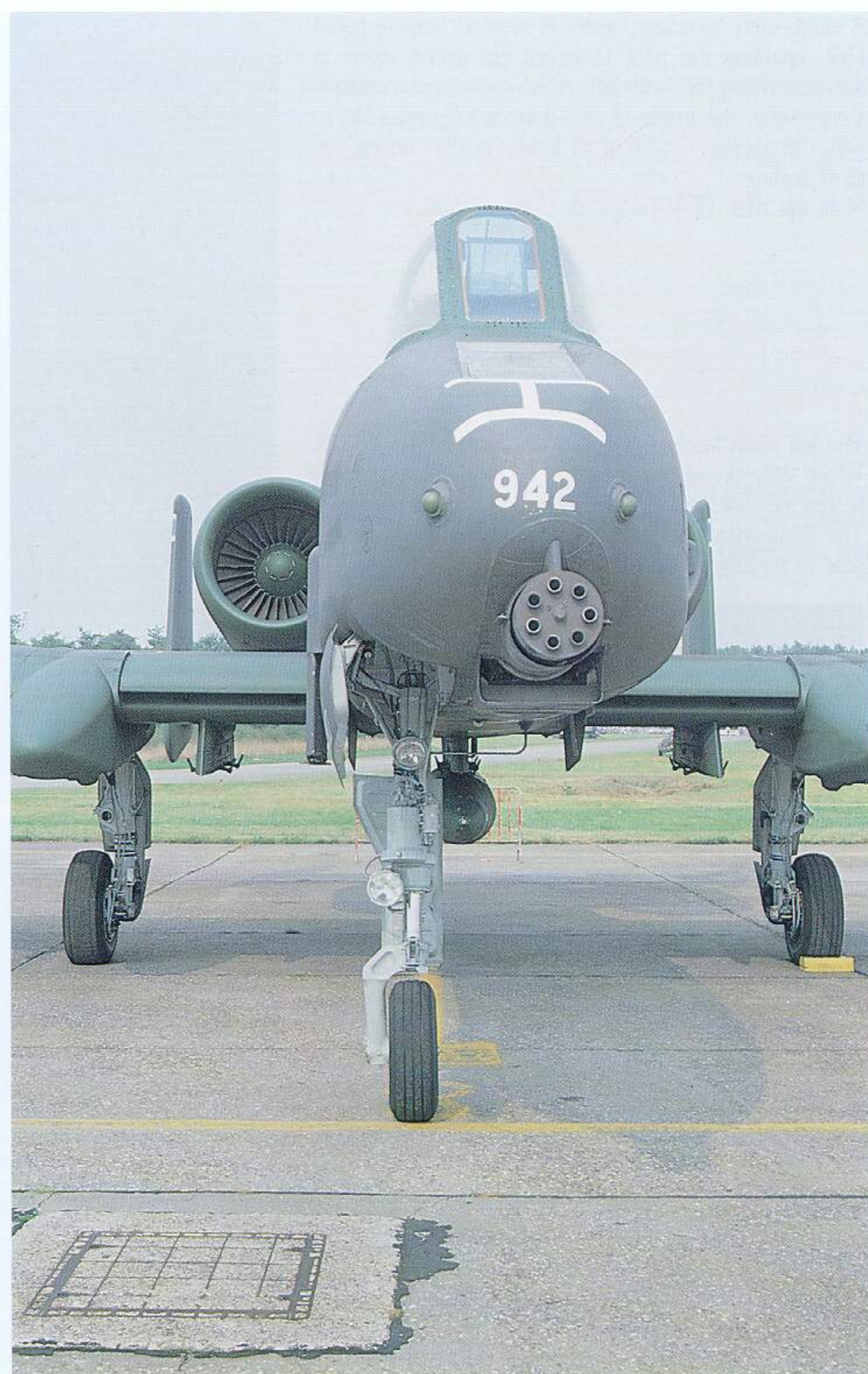
A further point of interest is the single-point in-flight refueling door on top of the nose section, with a white "H" marking in front of it. This marking is a reference point for the boom-gunner in the tanker aircraft. Because the refueling boom would remove most of the paint anyway, this panel is left unpainted showing its bare metal surface. Two more AN/ALR-69 radar warning antennas can be seen on either side of the nose.
