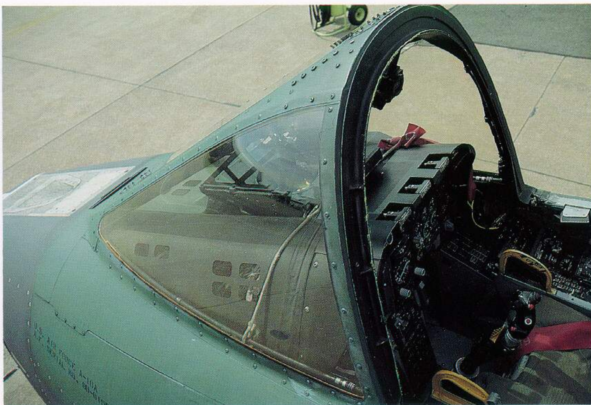
The front windshield and the instrument cover from the left. The HUD or head-up display, developed by Kaiser Electronics, can be seen under the windscreen. Note the inflight refueling panel at front and the raised assembling bolts on the cockpit framing.
