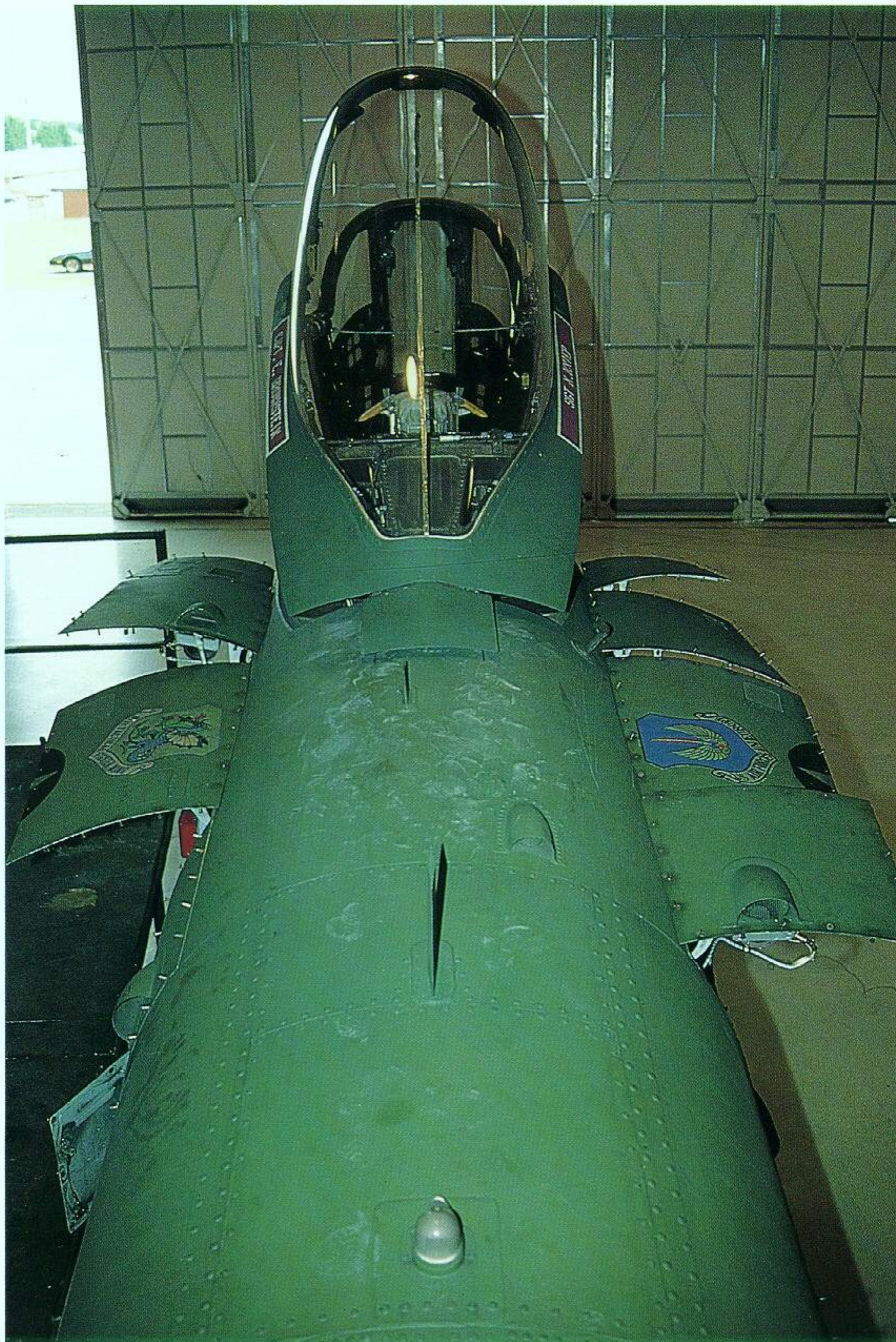
The front top fuselage with the panels described on the previous page at left. Note the shape of the aft side of the hood and the cover plate over the canopy actuating mechanism. Antenna designations can be found on page 20. The small exhaust at right and on top of the fuselage is the INS compartment coolant air outlet.
