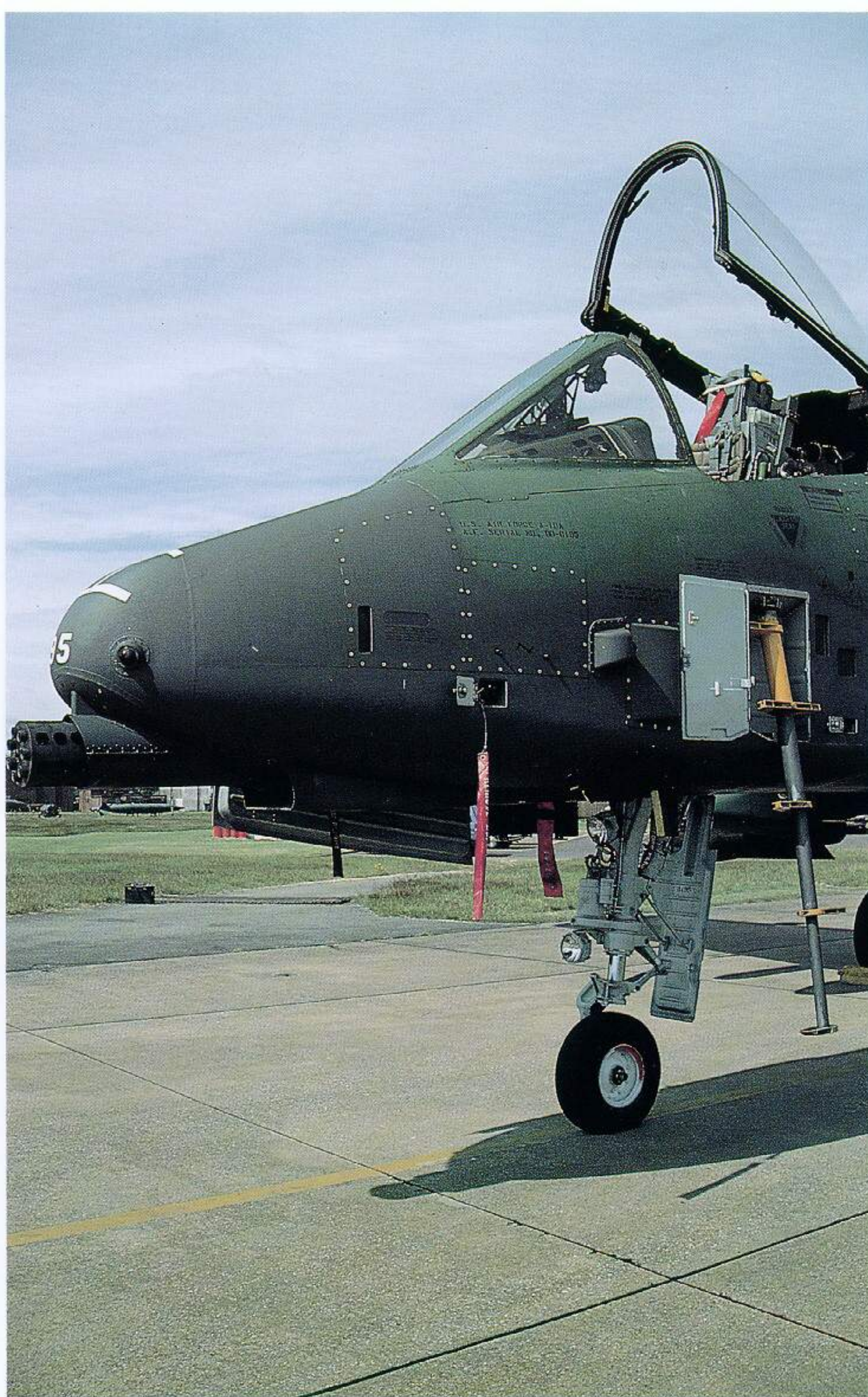
The business end of the A-10 "Warthog". The huge centerline mounted GAU-8/A 30mm "Avenger" gun caused the repositioning of the nose landing gear to the far right of the fuselage. Note the way the gun muzzle is incorporated in the nose section of the aircraft, retaining the A-10's pointed nose.
