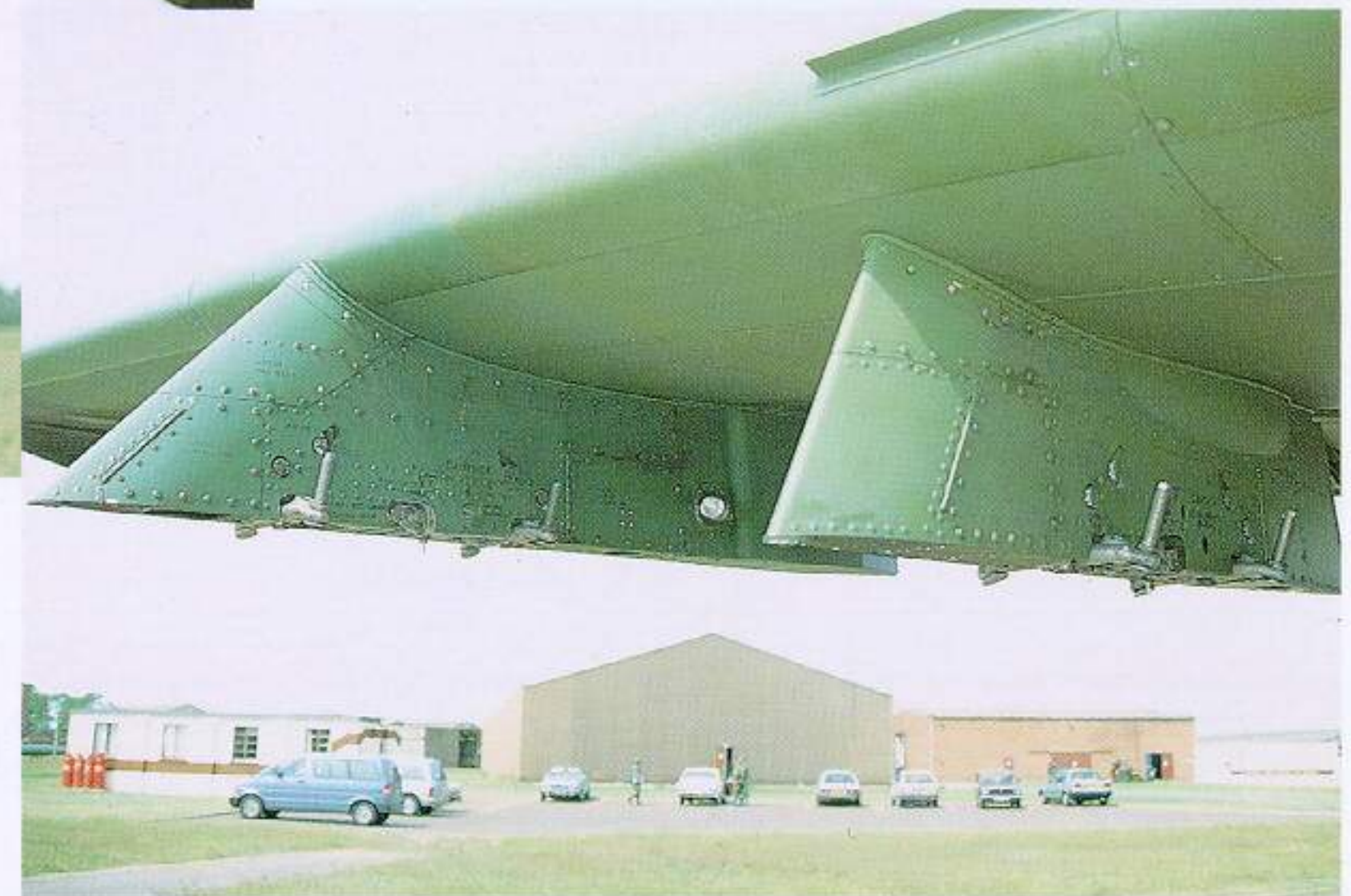
Pylon station number 10 and 11, the latter being the outmost hardpoint. Note this pylon is lacking the bulb just underneath the wing surface and the floodlight aft on the same pylon. This floodlight is used to illuminate the cockpit area during night-time operations.
