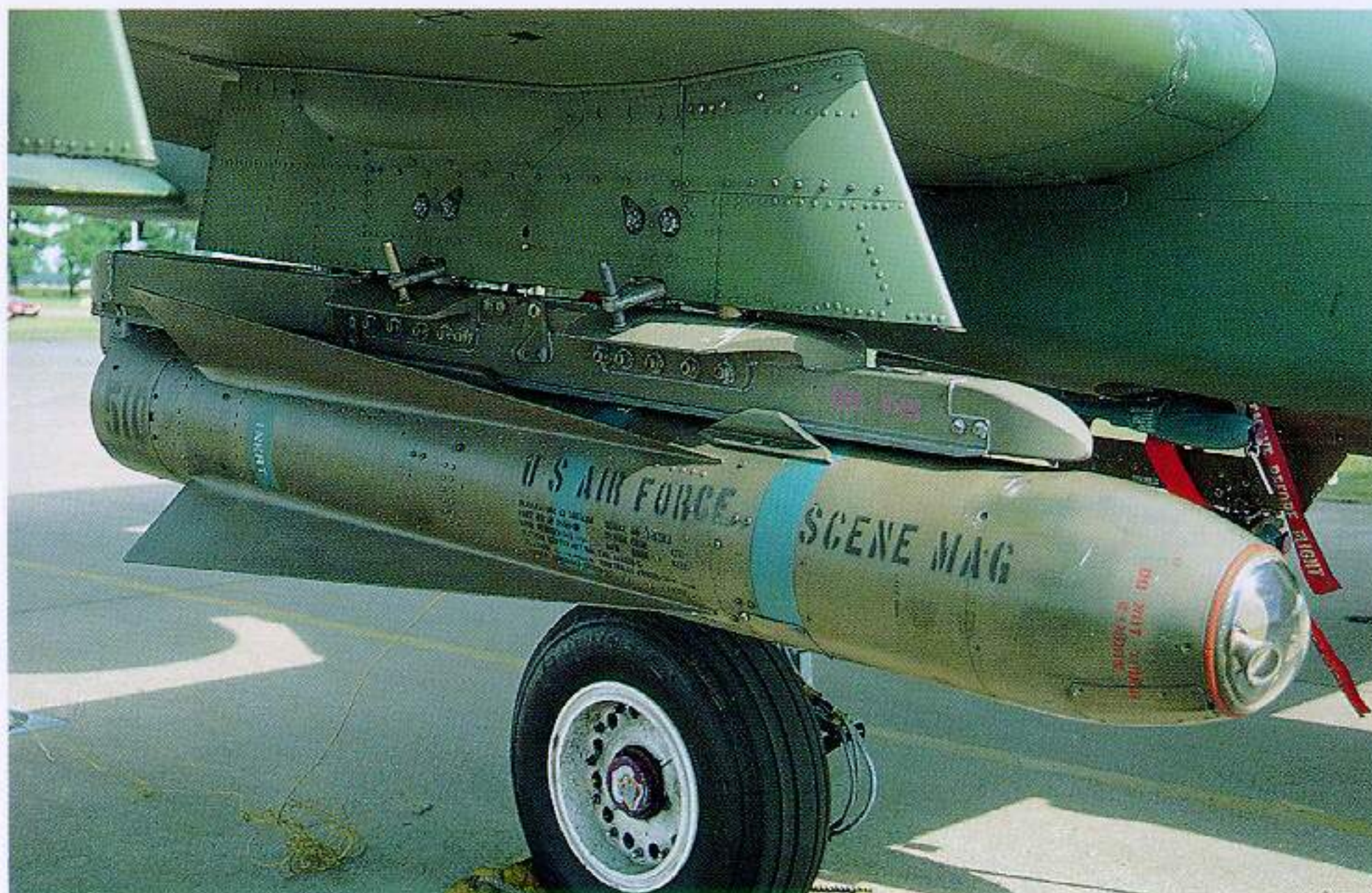
Left and right view of an inert version of the dreadful AGM-65B Maverick missile. The missile is mounted to a special launching rail underneath hardpoint number 9. Although not armed and lacking the motor and the guidance fins, this missile provides the pilot with TV images for simulated missile runs. The color of the missile and launch rail is similar to the TER-9 described above. The blue bands indicate this Maverick is used only for practice purposes.
