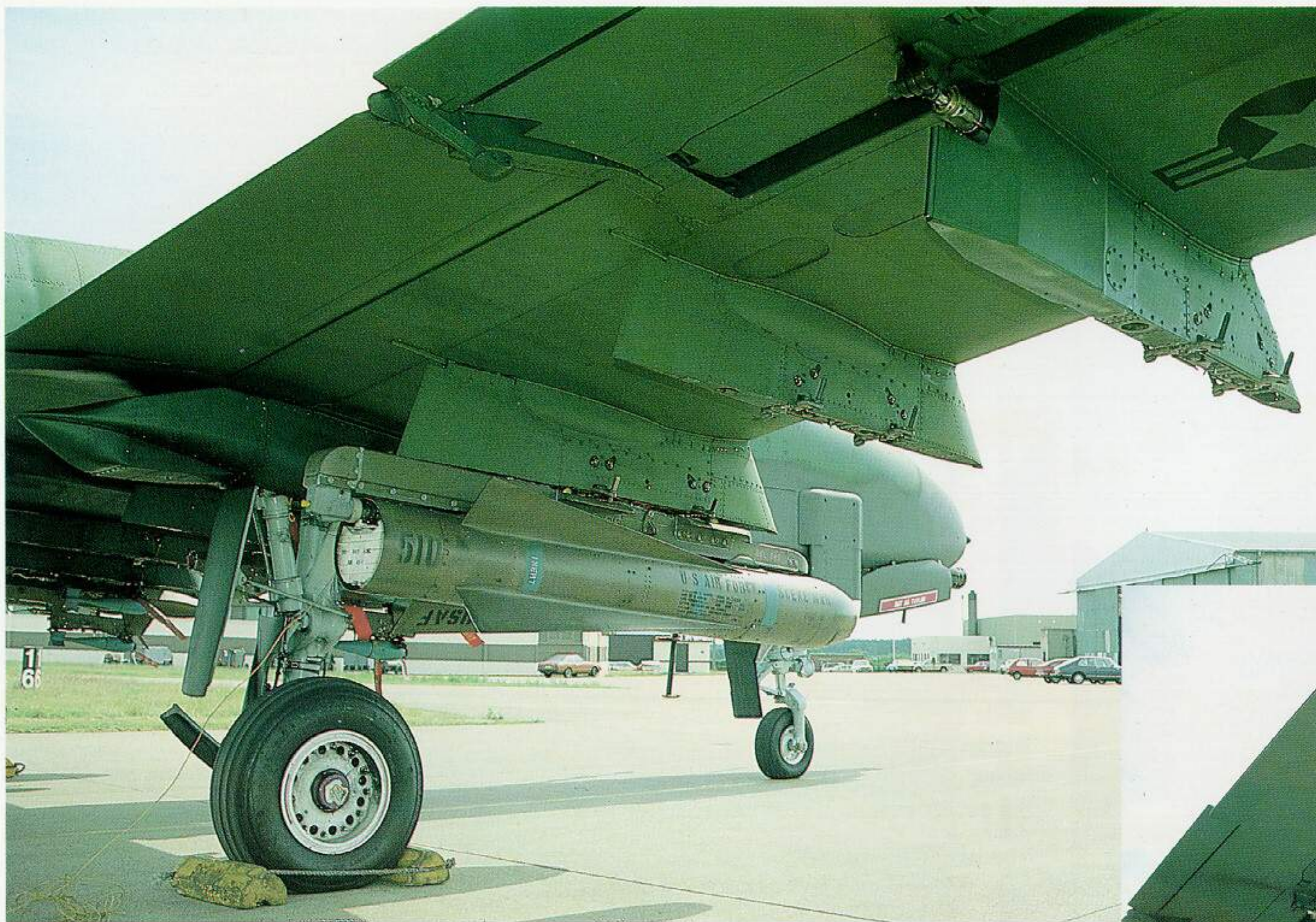
A different look at the underwing stores. Note the aileron actuating rod protruding from the rear of pylon 11, making the rear end of this pylon much wider than pylons 9 and 10. The picture at right shows the covered flare dispenser and wingtip navigation light. Part of the wingtip pitot-static boom can still be seen at right. Both bottom pictures show the right upper wing from above. Note the aileron trailing edge pitchup and the drooped wingtip.
