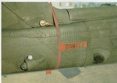
A look at the base of the vertical tail fin. A 42 degree change of direction of the tail rotor driveshaft is provided here. The oil level sight glass of the gearbox and a magnetic chip detector can clearly be seen, as well as the tail position light and the radar warning antenna to the front.
