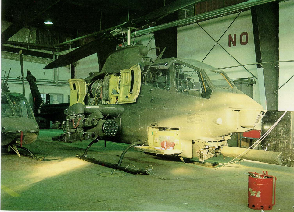
An AH-1S Cobra inside the maintenance hangar at Büdingen airfield in Germany. Note the protective cover over the gun barrels and the FOD can in front of the helicopter. Parked next to it is an OH-58 A scout helicopter, which is also part of the flight arsenal of this airfield.
