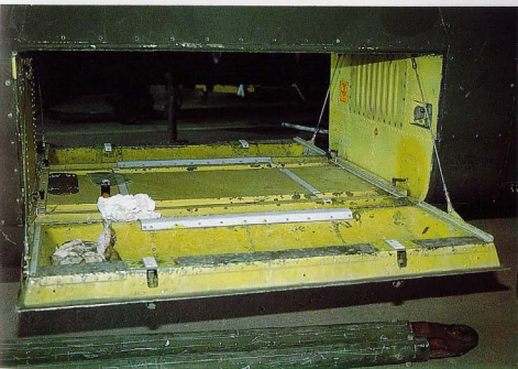
The empty ammo bay with the two doors/platforms hinged down. Note the four hold-back cables.
