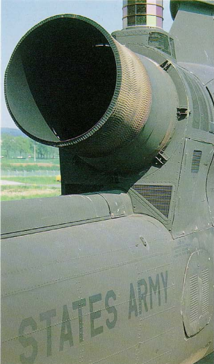
Closeup of the right side of the Cobra. Note the large ventilation door over the battery compartment and the IR jamming device on top of the engine outlet in the picture at left. Attentive readers already noticed this Cobra carries two TOW launch assemblies (on top of each other) under the right wing pylon.
