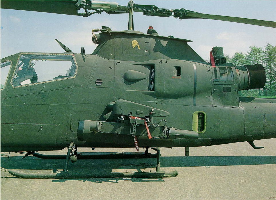
A beautiful shot of the left side of the Cobra with the single TOW launch system as main attraction. Note the red (left) position light on the outside of the wing holding the launch assembly and the landing light on the front skid support bar. Further interesting features are the cone on the transmission compartment door just in front of the engine inlet (left side only) and the anticollision light on top of the rotor shaft housing.
