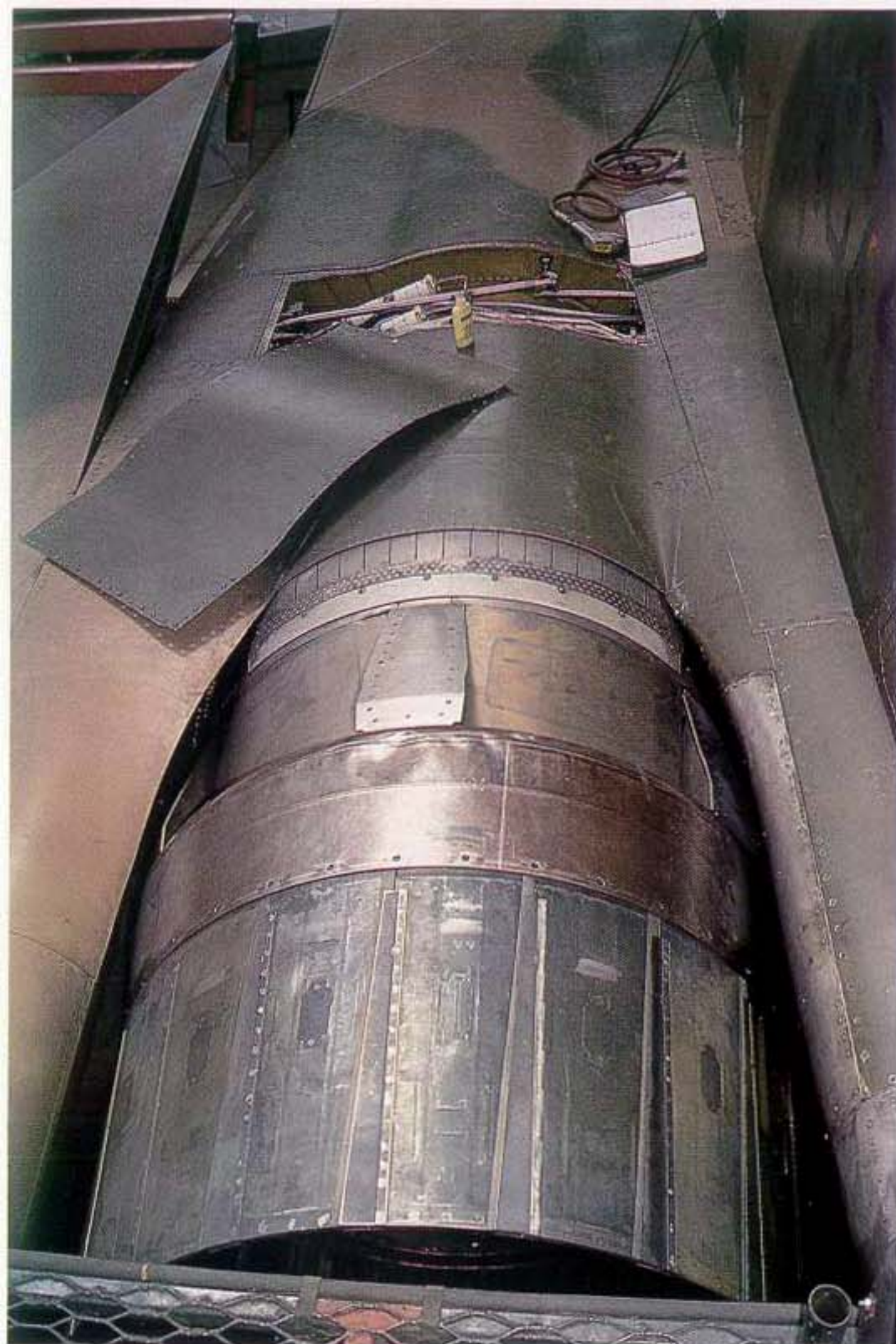
(Left) A clear view of the tail pipe from above which shows the tail feathers and the way the engine is fitted into the fuselage. Note the shape of the panel which has been removed here to execute some minor repair.
