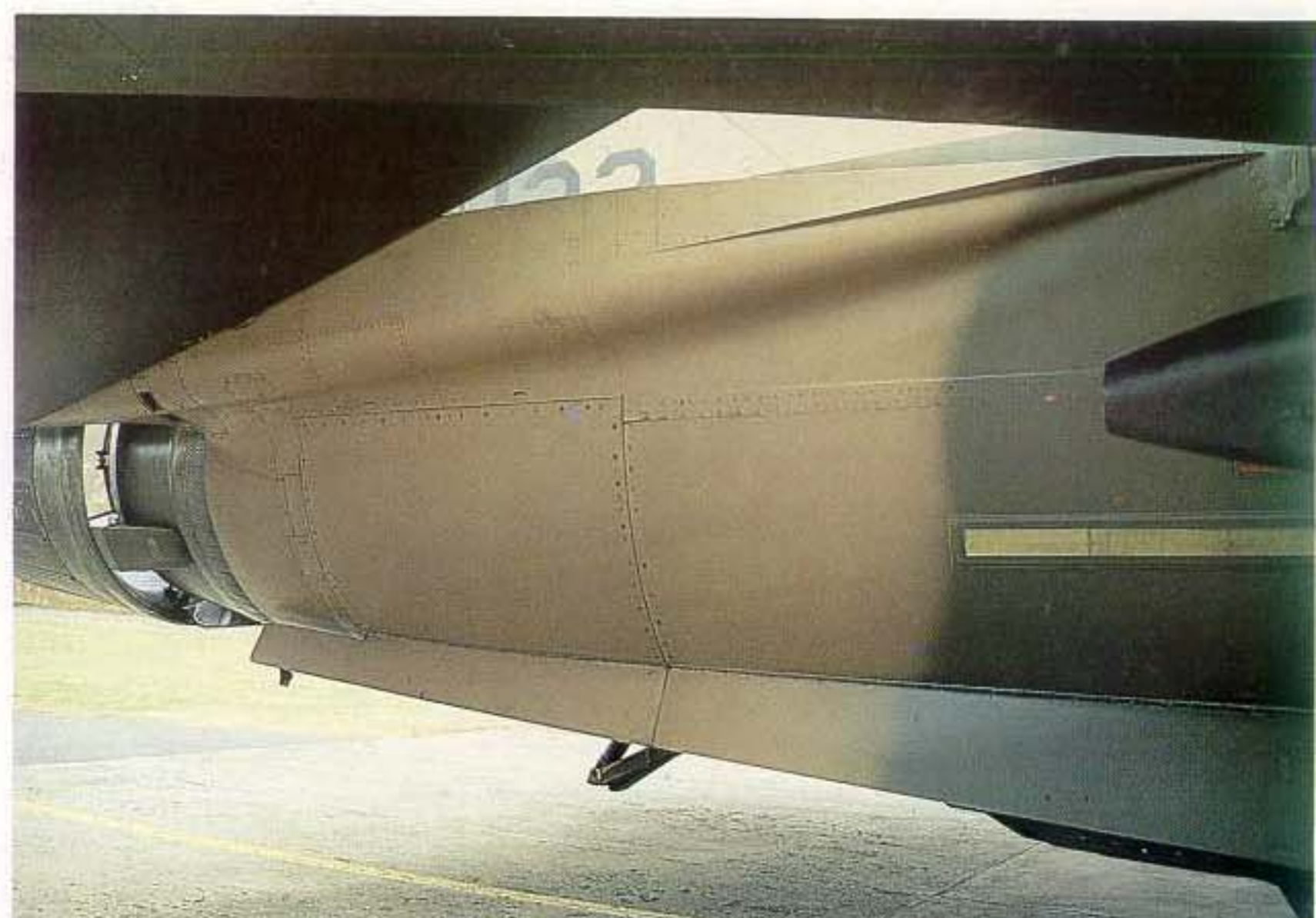
The same area looking aft with a view on the horizontal stabilizer servo actuator housing. Note the smooth overflow of the fuselage into the housing. A view of the exhaust nozzle from this side which most certainly will help the modelers get their kit right.
