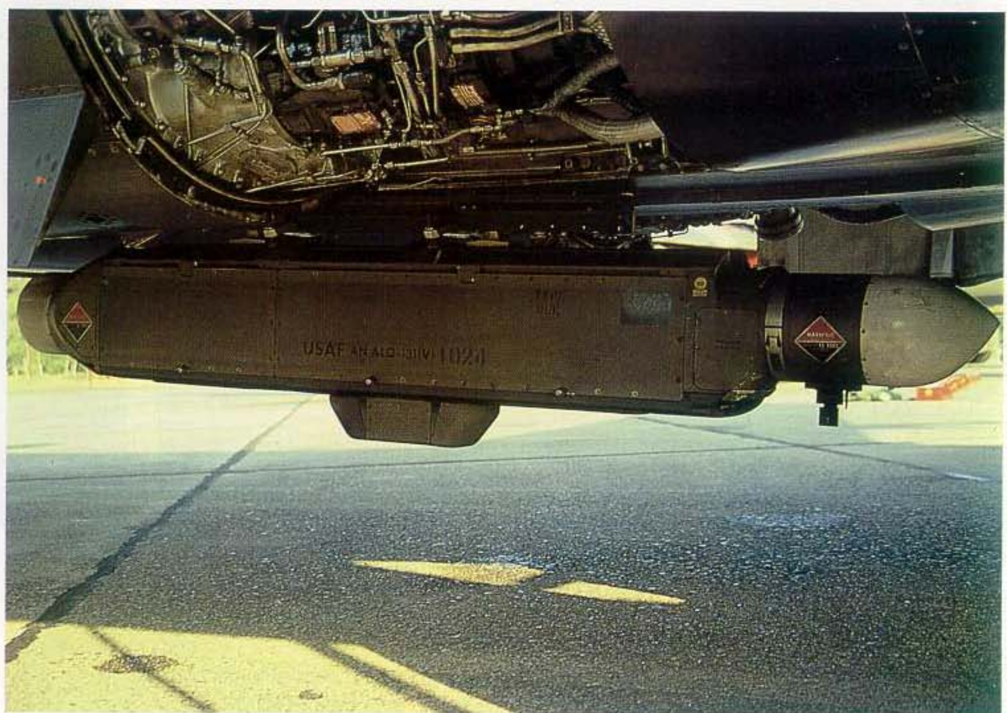
One of the main jamming devices on the F-111, the AN/ALQ131 (V). This is the newest of the ECM pods carried by tactical One-Eleven's which is of Westinghouse origin, one of the main contractors producing such equipment.
