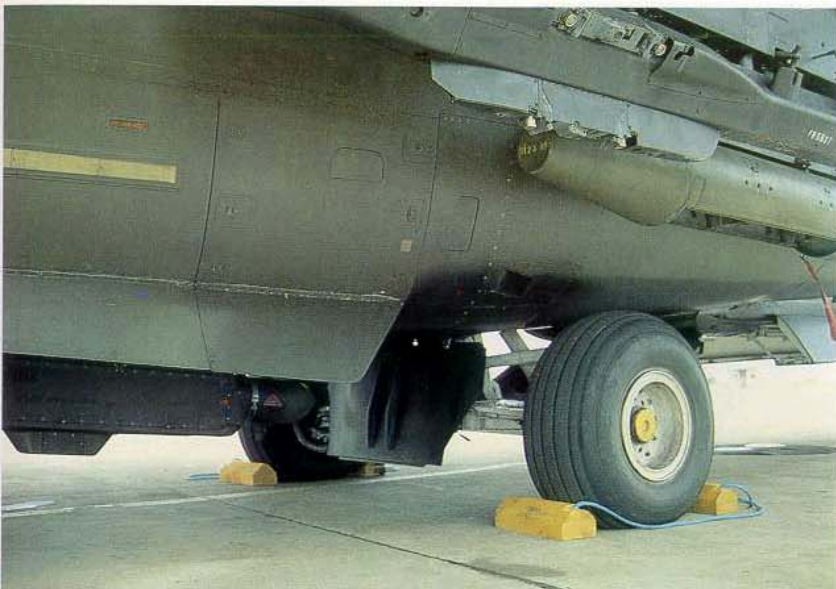
The aft side of the dispenser and the area behind the main wheel assembly. Note the low voltage formation strip above the ventral strake.
