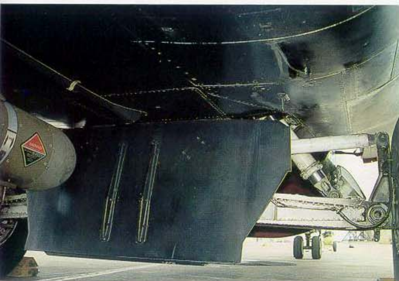
The rear main landing gear door from behind. Note the very peculiar shape of it and that it hinges to the fuselage in an upright position, unlike the first F-111's where it was locked parallel to the fuselage on the main landing gear assembly. Also note the small aerial slightly to the right and aft of the gear door. Part of the main landing gear/wheel connection can also be seen.
