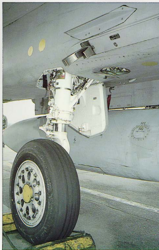
Main landing gear, rear view looking forward.
