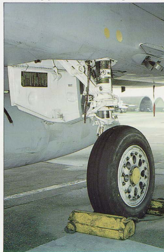
Main landing gear, frontal view looking aft.
