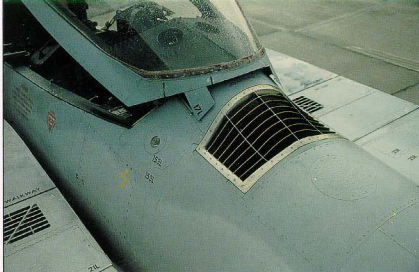
The cooling air exhaust duct of the air conditioning system on the F-15D.
