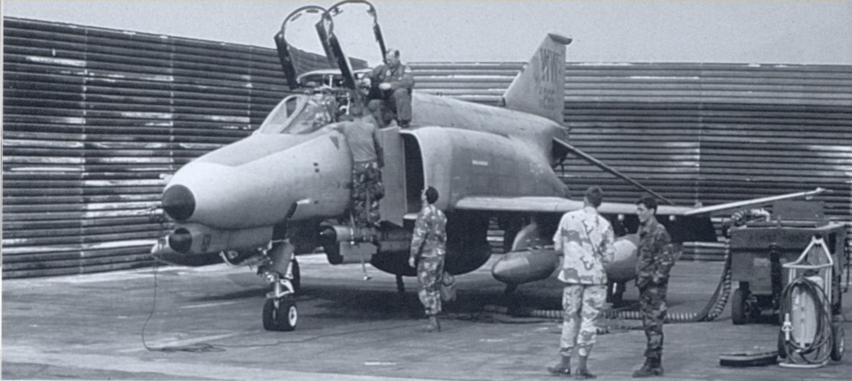
A 561st TFS F-4G-42, 69-265, in a revetment at Shaikh Isa AB on the island nation of Bahrain in the fall of 1990, where it was under the control of the 35th TFW (Provisional). The aircraft is carrying a baggage pod on the inboard pylons, with the crew members' personal effects inside. (USAF)
