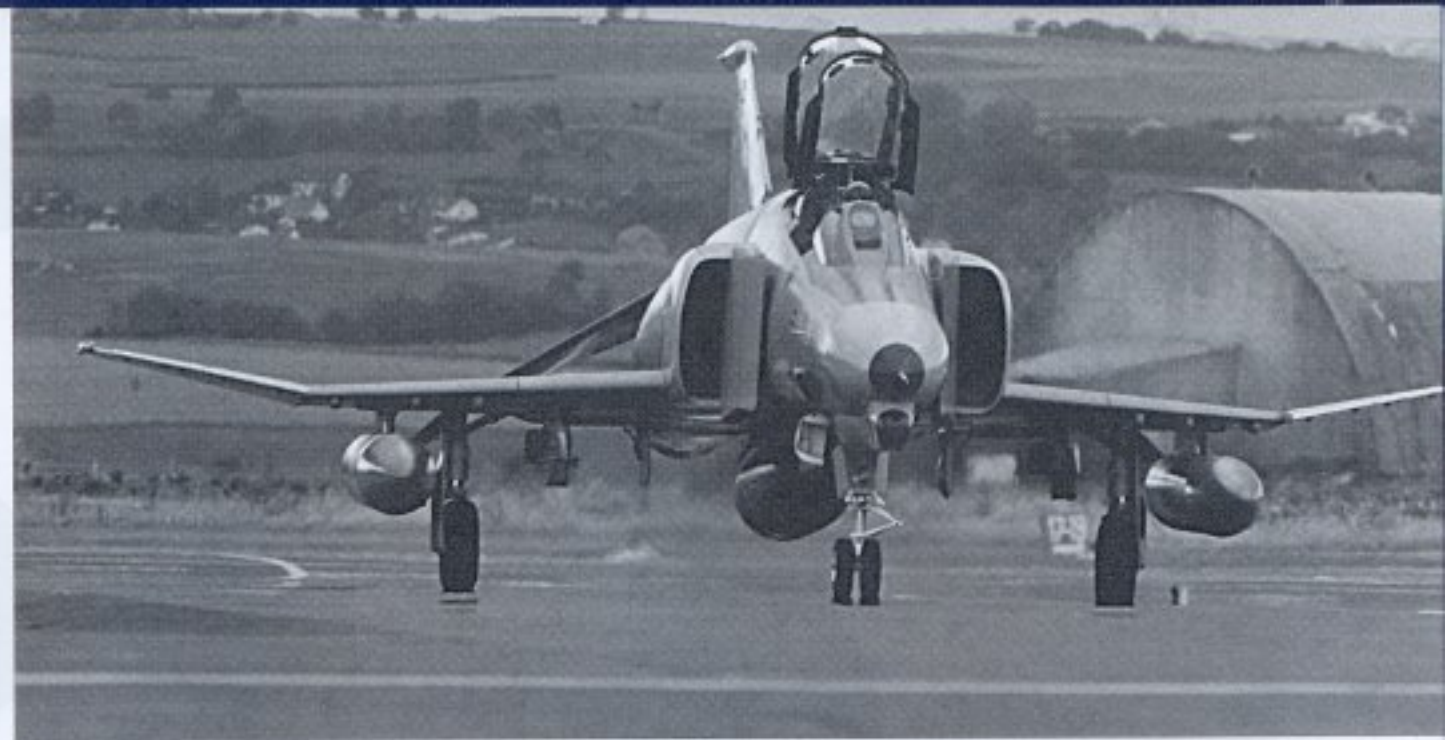
Looking like a large insect, an 81st TFS F-4G taxis back to its parking spot at Spangdahlem AB, West Germany. The up-angle of the new 600-gallon centerline tank can be seen. The older F-4 centerline tank had a down-angle when mounted. (G.A. Kromhout)
