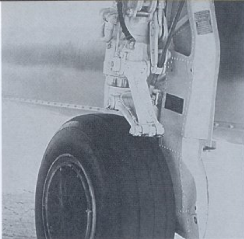
(Clockwise from left) The right main landing gear of the F-4E. The main wheel mounted a 30-inch-tall, 11.5-inch-wide 24-ply tire. (author)
