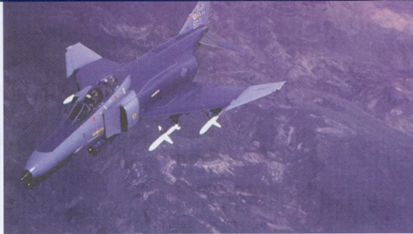
A 561st TFS F-4G shows off the upper surface camouflage during a live-fire exercise on the Nellis AFB firing range in 1988. The thin stripe atop the fuselage and intakes is the outline of the walkway areas. (USAF)
