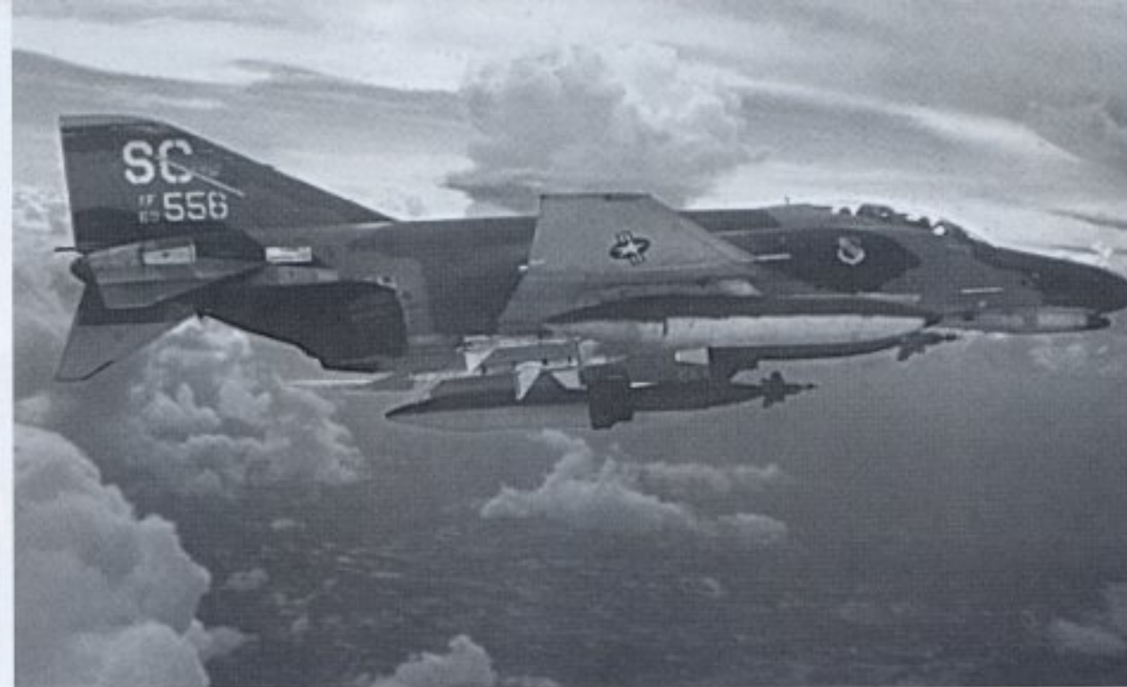
A 4th TFW F-4E-33 heads toward a target in Laos during 1970, carrying a pair of GBU-10 laser guided bombs. The GBU-10 used a Paveway II seeker head attached to a 2,000-pound Mk. 84 bomb casing. A designator aircraft, usually an F-4D, carried the guidance pod and directed the bombs to their target. (USAF)
