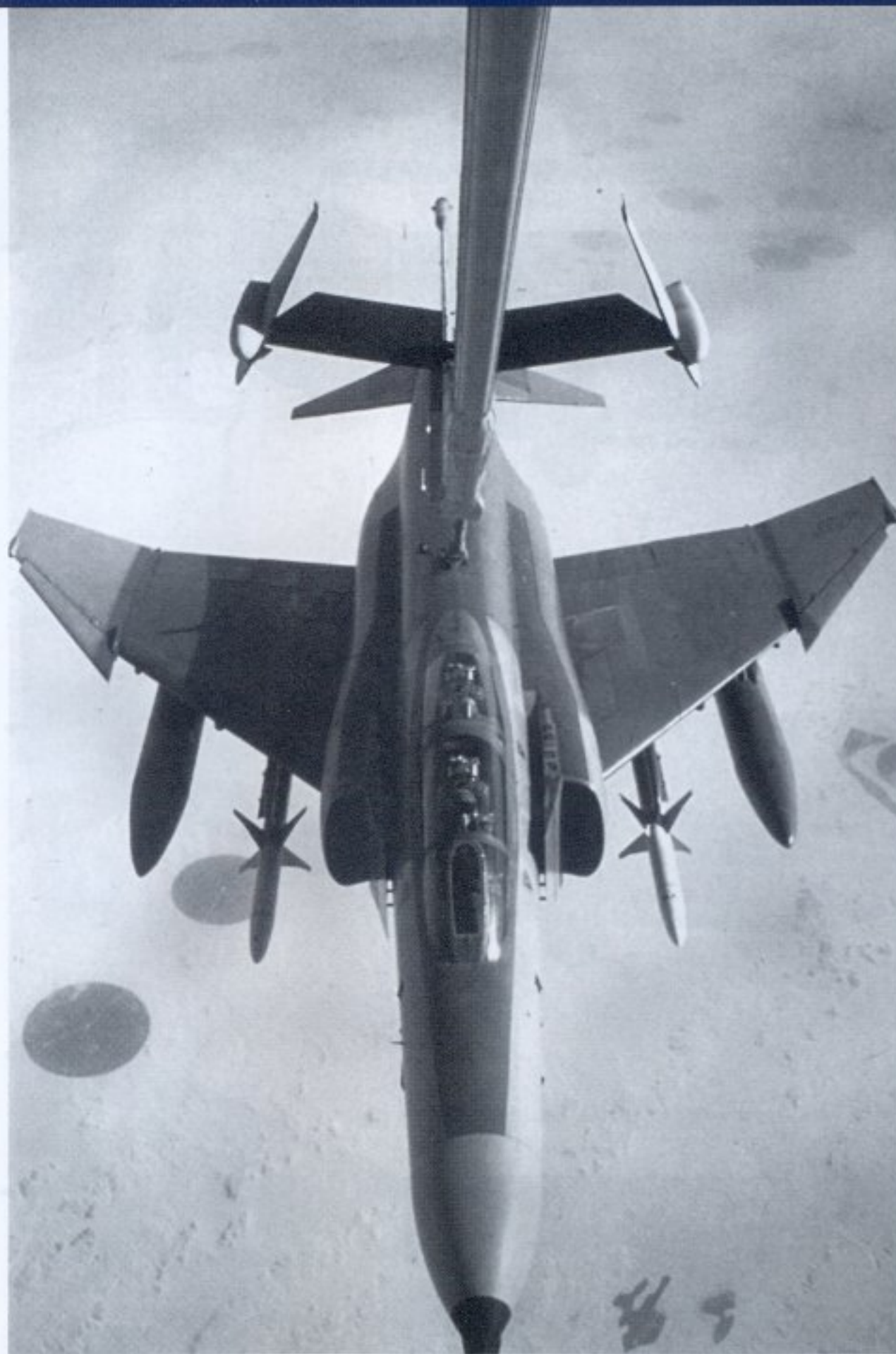
Hooked up and taking fuel from a KC-10 tanker, this 35th TFW (Prov) F-4G is bound for a SAM suppression mission near Baghdad as signified by the ordnance load — two HARM missiles and three drop tanks. (USAF)
