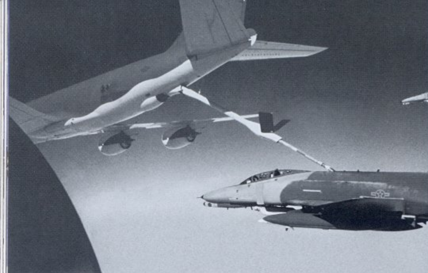
A 561st TFS F-4G takes on fuel prior to a mission in Desert Storm. Normal armament for a strike into Iraq was a pair of either AGM-45 Shrike ARMs or AGM-88 HARMs, two AIM-7 Sparrow missiles for defense, and an ALQ-131(V-14) ECM pod. (USAF)
