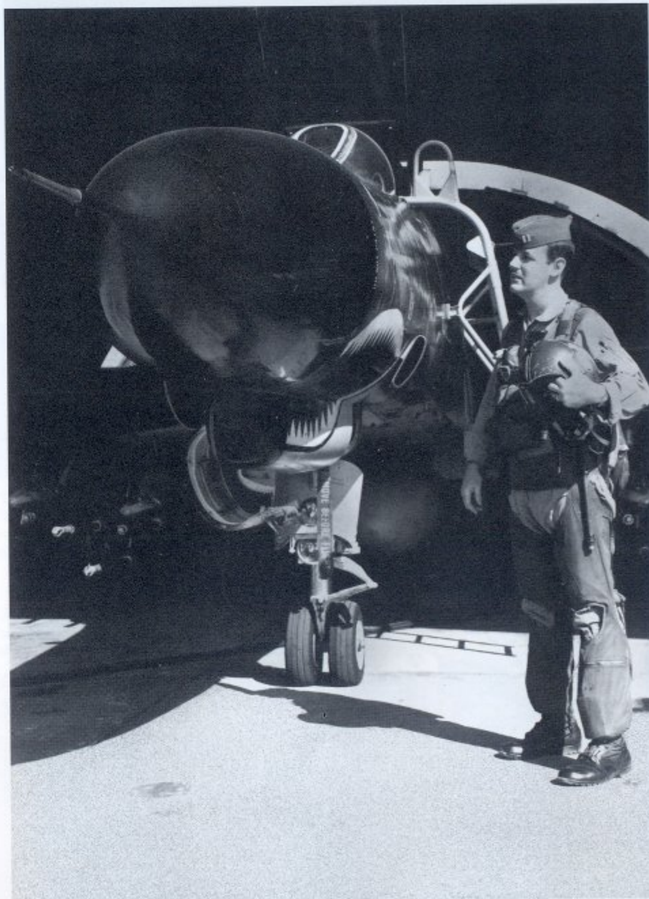
Capt. Pete Gillespie, a 366th TFW Weapons System Operator or WSO, stands next to the F-4E he was assigned to at DaNang in early 1970. The short muzzle cover over the Gatling cannon barrels, typical of early F-4Es, is clearly shown, as is the smaller radome that covered the APQ-120 radar unit. (USAF)
