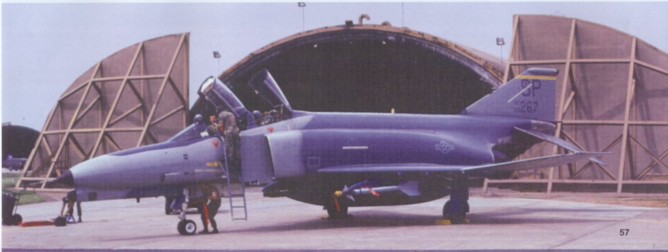
An 81st TFS F-4G-43 in front of one of the covered hard shelters at Spangdahlem AB, West Germany, in 1993. The aircraft carries AIM-9L Sidewinder missiles. The F-4G also carried two AIM-4 Sparrow missiles for defensive purposes. Because the F-4G had no internal gun, air-to-air missiles were its only defense against enemy fighters. (Paul Bigelow)
