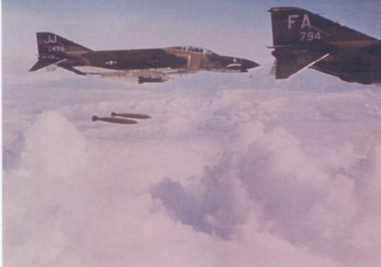
A 34th TFS F-4E drops a pair of M118 3,000-pound LDGP bombs on a North Vietnamese target in 1969. The M118 3,000-pound bombs could only be carried on the outer wing pylon of the F-4. (USAF)
