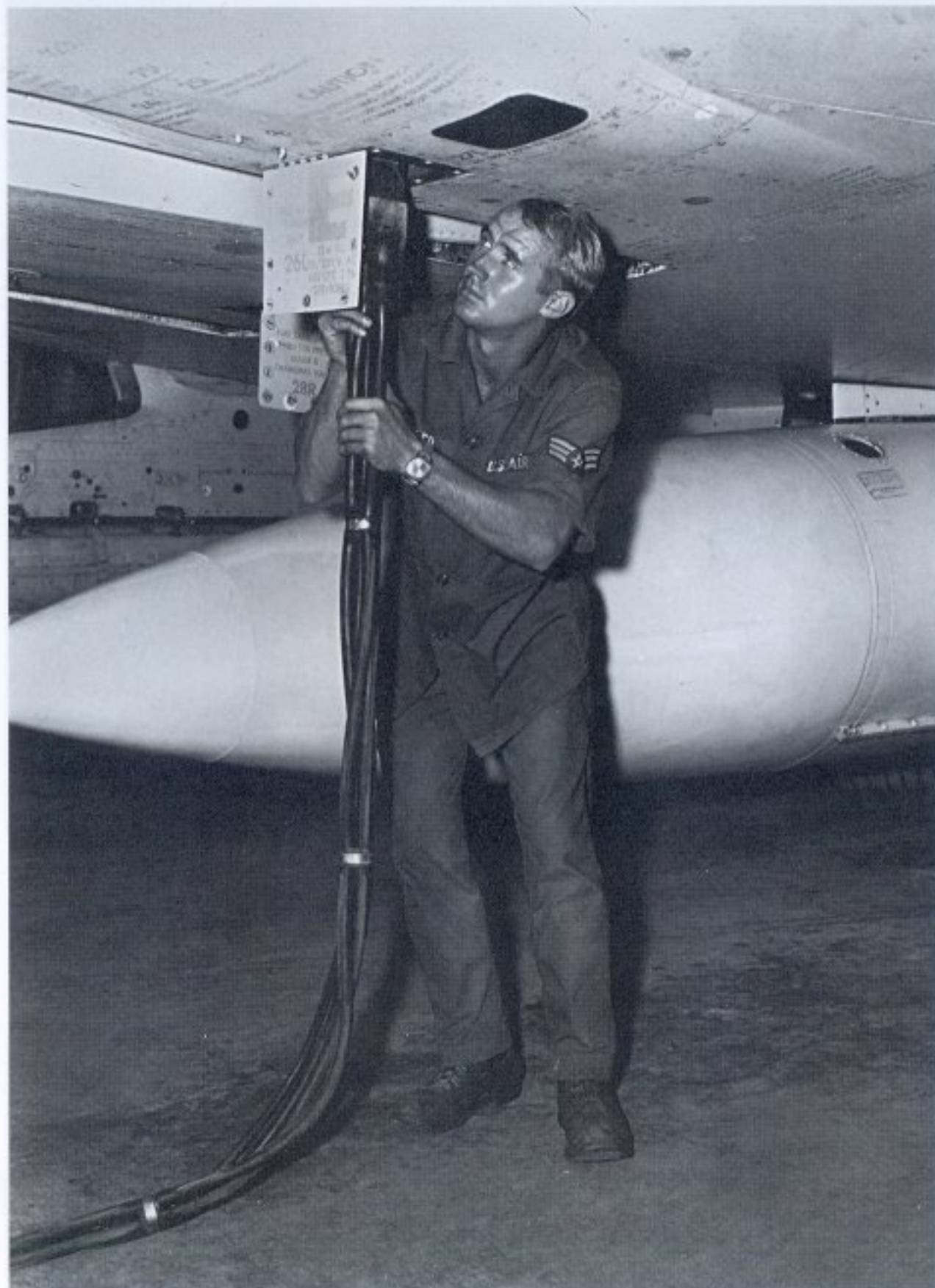
Sgt. John Miller hooks up the electrical starting cable to a 4th TFS F-4E at DaNang AB in September 1969. Electrical starting of the big J79s was much preferred over the cartridge start system. The heavy electrical cables ran from a large auxiliary power cart with a gasoline-fired generator. (USAF)
