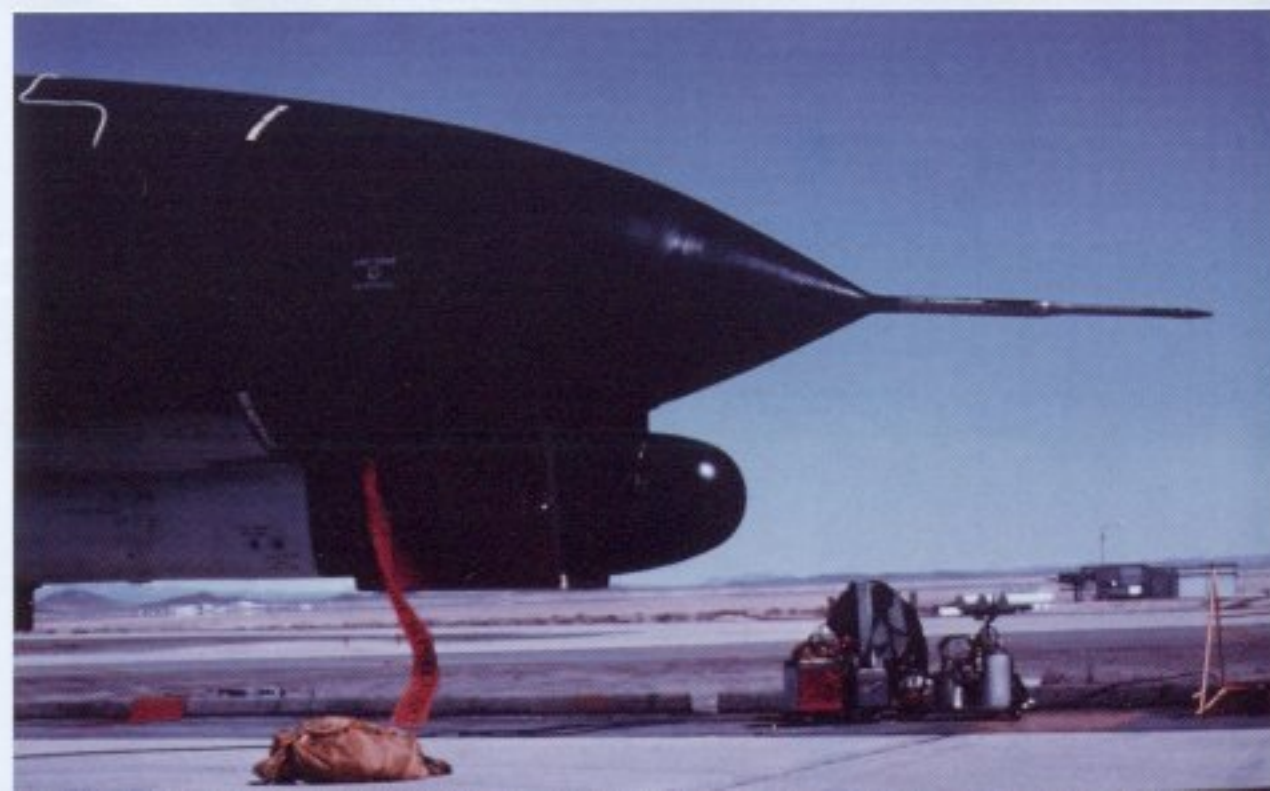
(Clockwise from above) This view of the tail of a 37th TFW F-4G showing the APR-38 aft receiver antenna housing, and another APR-38 low-band antenna blade in the middle of the forward "W." The small bumps on the parachute housing door are nonfunctional. (Paul Minert)
