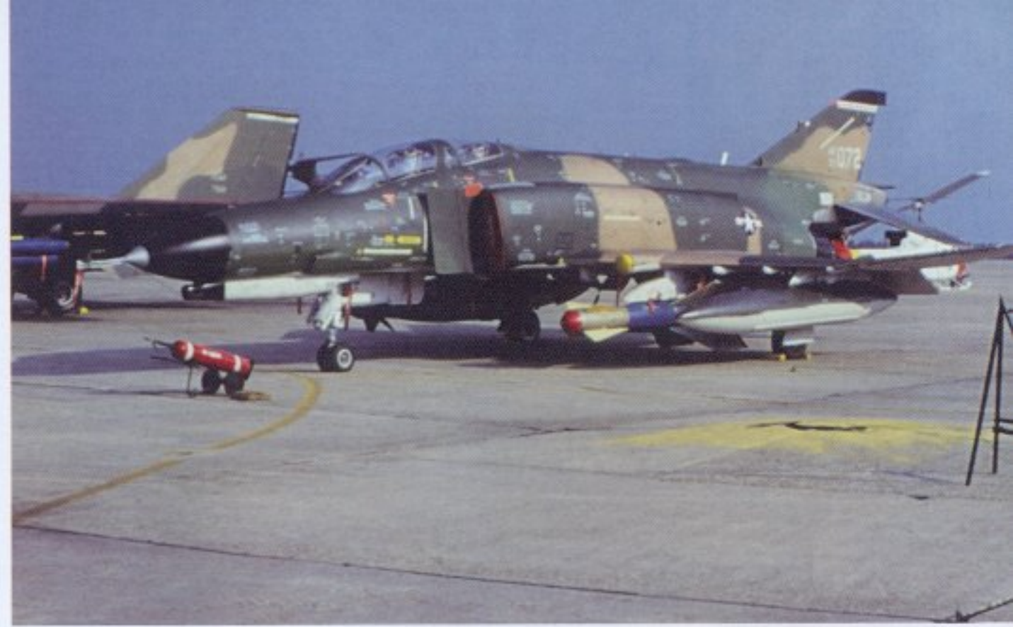
An F-4E-49 on the ramp at Langley AFB, armed with a GBU-15(V)-1 2,000-pound Modular Guided Glide Bomb on the left pylon and a standard GBU-10 2,000-pound Paveway LGB on the right pylon, during an open house in 1979. (Dick Starinchak)
