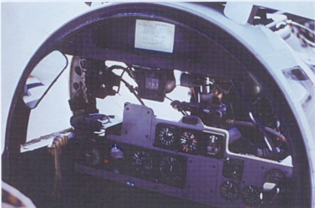
The upper rear instrument panel of noncombat F-4Es which contained basic engine and flight instrumentation. As with all Air Force F-4s, the F-4E could be flown from the rear cockpit and had a control stick and throttles. (Hugh Muir)
