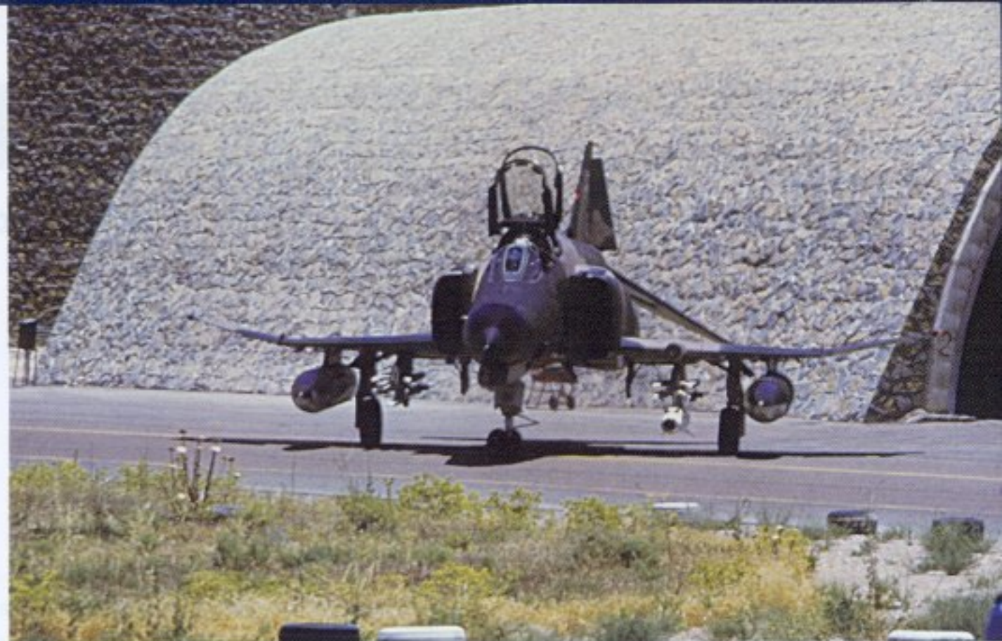
In 1977, in anticipation of equipping the Iranian Air Force with F-4Es, the 50th TFW deployed to Shiras AB, Iran, for a demonstration of the F-4E's capabilities, including the AGM-65 Maverick air-to-ground missile. The AGM-65 was carried on three missile launchers on the inboard pylon. (USAF)
