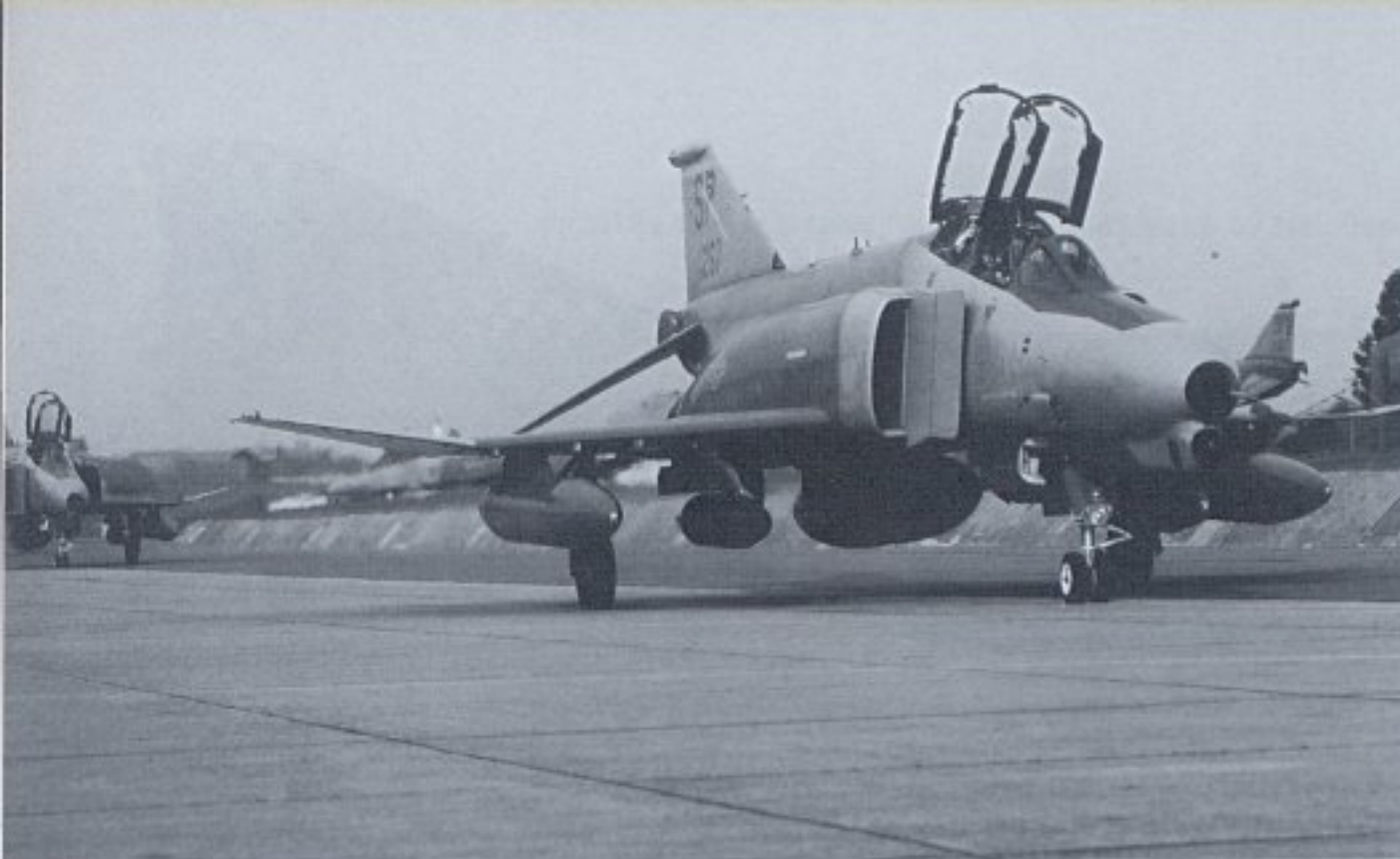
F-4Gs of the 81st TFS return to Spangdahlem AB, West Germany, following a tour of duty to the combat zone. Note that each aircraft carries two baggage pods on the inboard pylons — one for the pilot's effects and the other for the WSOs. (G.A. Kromhout)
