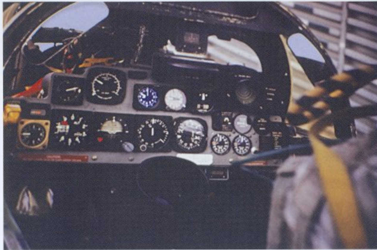
The rear instrument panel in a combat F-4E had a threat display panel attached at the top right of the panel. The large instruments in the center of the panel are flight instrumentation, while the smaller gauges on the right side are basic engine gauges. (Mick Roth)
