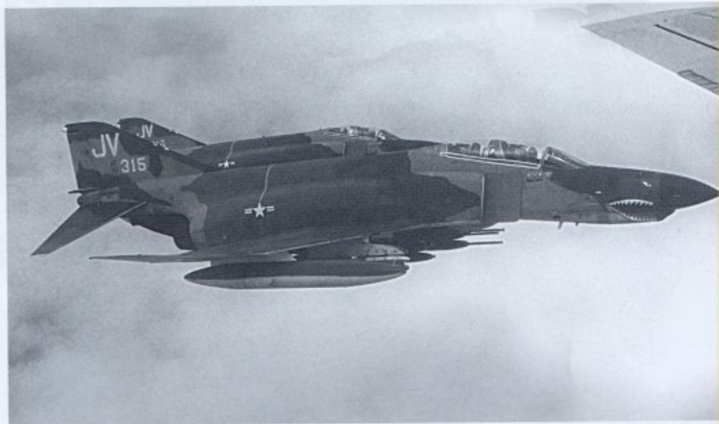
A pair of 469th TFS F-4Es depart the tanker en route to a target in Laos during May 1970. Note the interesting ordnance load. The right wing pylon has cluster bombs, while the left pylon carries three Mk. 82 500-pound LDGPs with 36-inch fuse extenders. On the centerline station are six Mk. 82 LDGPs. This was obviously an antipersonnel mission. (USAF)
