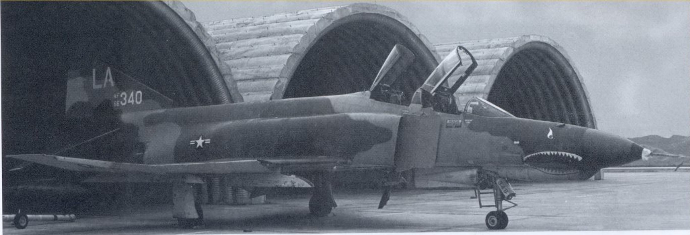
A 4th TFS F-4E sits outside a covered shelter at DaNang in 1970. Tail codes (LA for 4th TFS, LC for 421st TFS) were applied to all aircraft in Southeast Asia beginning in 1967. The drooped leading edge flaps can be seen. The 366th TFW adopted the shark's teeth marking that was a natural on the stepped F-4E nose, much as it was on the P-40 Warhawk during World War II. The shelter is constructed of steel tubing covered with twelve inches of concrete. (USAF)
