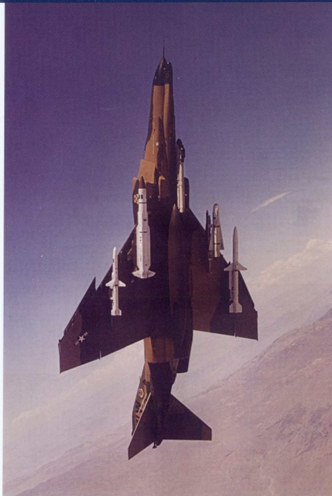
Publicity photo showing the full capabilities of the F-4G Advanced Wild Weasel aircraft. The F-4G could carry (from left) the AGM-45 Shrike ARM, AGM-78 Standard ARM, ALQ-119 ECM pod, AGM-65 Maverick air-to-ground missile, and the brand new AGM-88 High Speed Anti-Radiation Missile, or HARM. The wraparound camouflage is clearly shown. (McAir)
