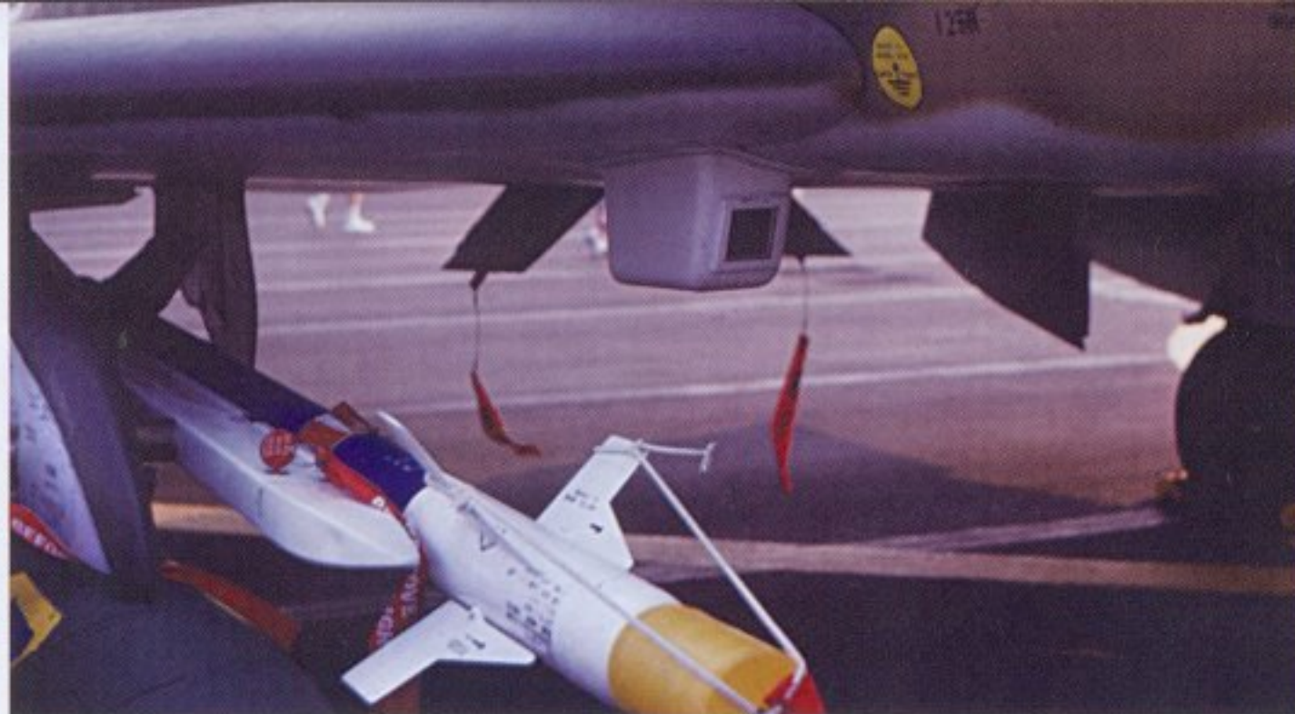
Under the right inner wing is the combat camera mount, not to be confused with the gun camera. Note the Yellow cover over AIM-9 seeker head. (author)
