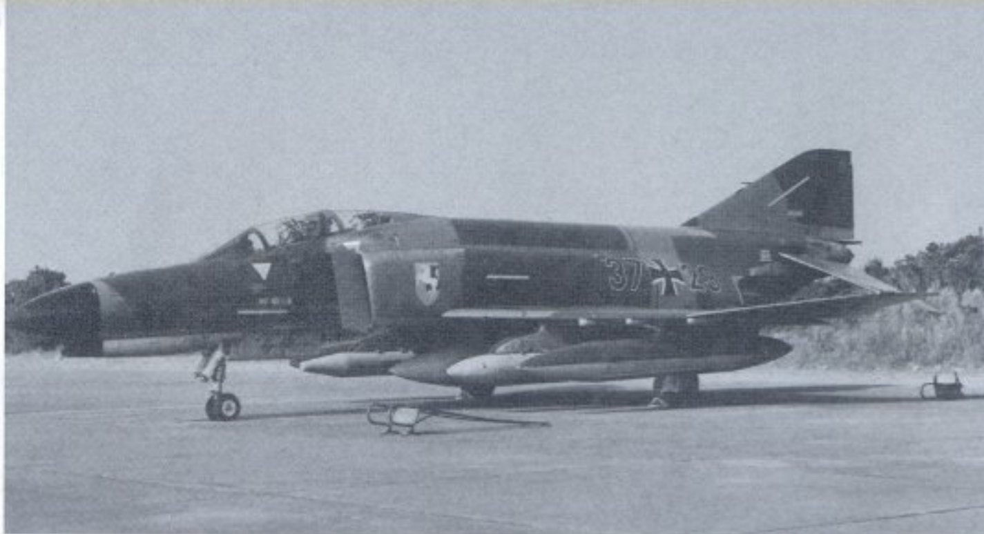
The West German Bundesluftwaffe F-4F was the first of the type to have the leading edge combat maneuvering slats that were eventually fitted to all USAF F-4Es. West German Phantoms were designated F-4F. This F-4F was assigned to JBG-36, and was delivered in standard West German hard-edged splinter camouflage (Norm 72) of RAL-6014 Olive Green and RAL-7012 Basalt Gray, with RAL 9006 Silver undersides. (Marc Rostaing)
