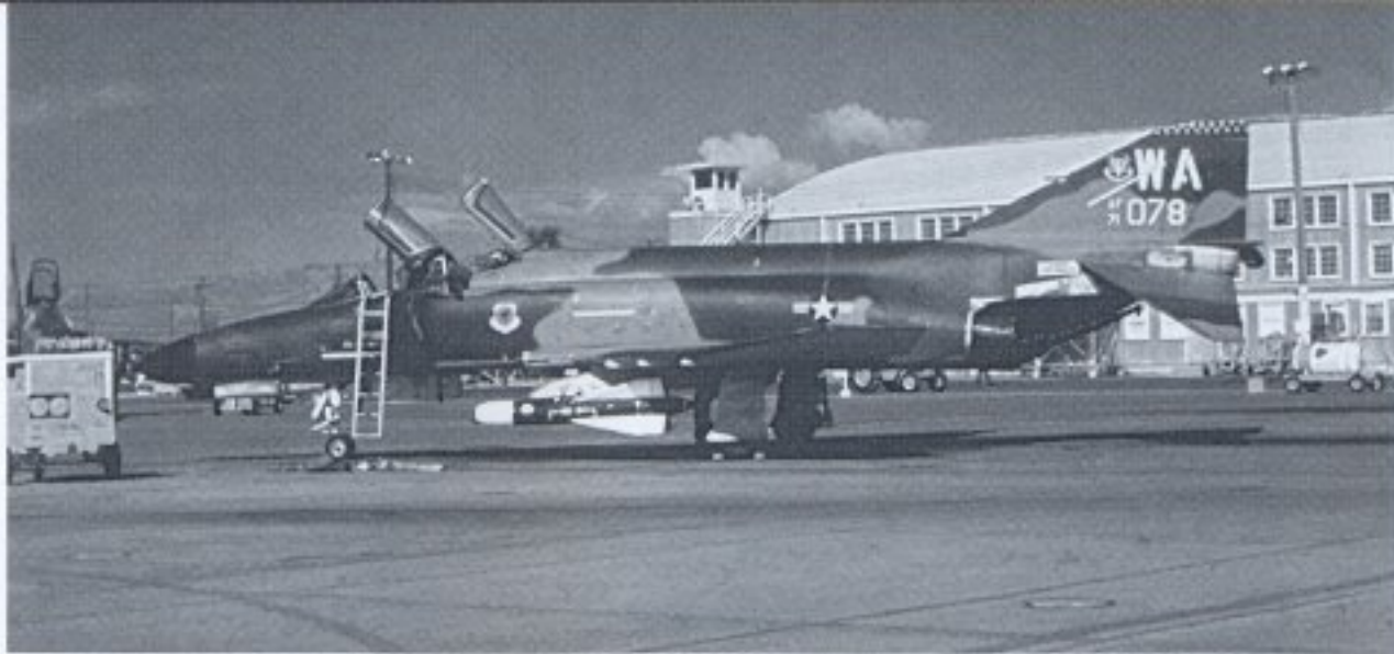
A 57th FWW F-4E-49 sits on the parking spot at Nellis AFB with a practice AGM-62 Walleye TV-guided missile. Practice ordnance, whether air-to-air or air-to-ground, was usually painted Blue and White. (Hugh Muir)
