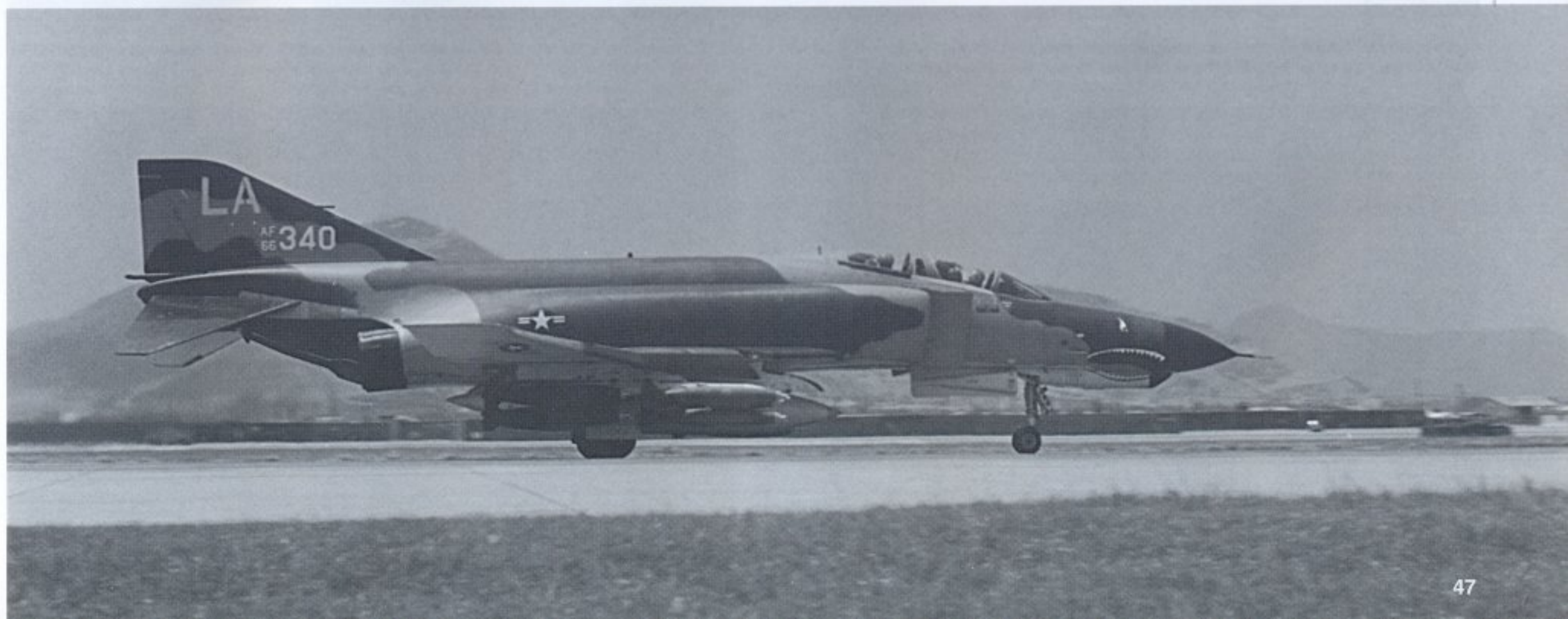
A 4th TFS F-4E-33 taxis to the active runway at DaNang in 1969, with twelve Mk. 82 LDGPs on MERs on the outboard pylons. Interestingly, there is no ordnance of any kind on the inboard pylons. The 4th TFS was assigned to the veteran 366th TFW, which had been operational in F-4s from DaNang since 1965. The leading edge flaps are deployed for takeoff. (USAF)
