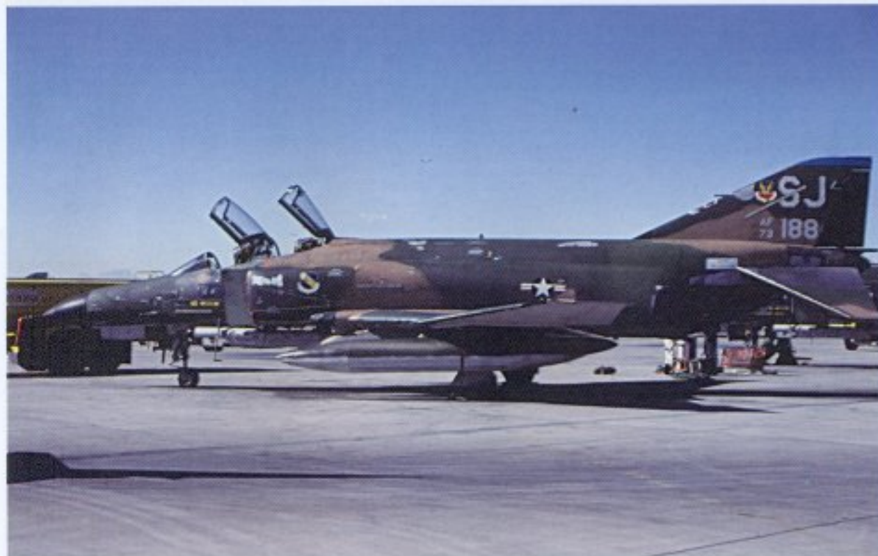
A 4th TFW F-4E-58 on the ramp at Seymour Johnson AFB with an ALQ-119 ECM pod in the forward Sparrow bay. The ALQ-119 was the pod of choice well into the 1990s, and could be configured to jam a variety of different enemy defenses. (author)
