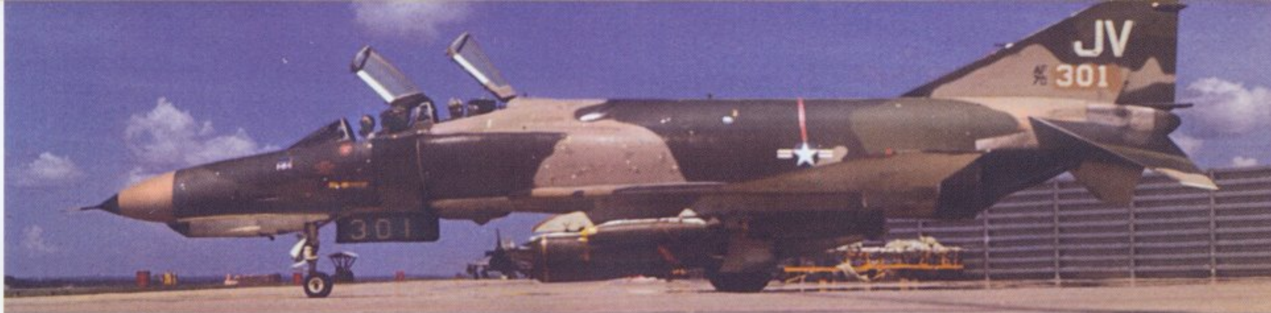
(Top photo) An F-4E-35 assigned to the 469th TFS at Korat in October 1969. This F-4E has the Light Tan radome seen on some early model F-4Es in the combat zone. Note the ordnance load, MERs on the outer pylons with five Mk. 82 LDGP bombs, and TERs on the inner pylons with three M117 750 GP bombs. The inside of the nose gear door is painted dark Green with the tail number repeated in White. (USAF)
