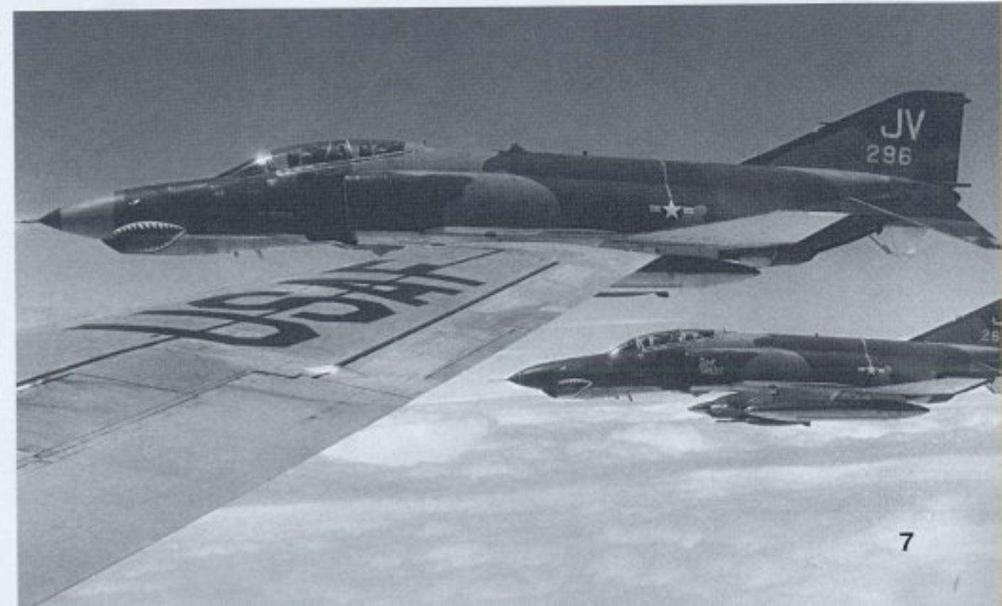
"Paper Tiger" (67-268) and another 469th TFS F-4E (67-296) get ready to take on fuel from the waiting KC-135 as denoted by the upraised refueling door on -296. Both aircraft carry a mixed load of CBUs and LDGP bombs. The light tan radome on -296 was unusual but not uncommon on the early F-4Es. (USAF)
