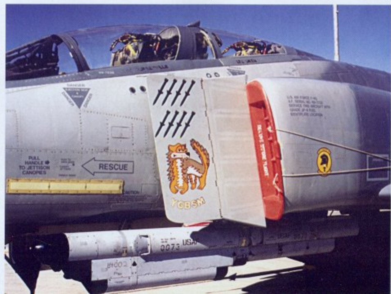
The standard ECM pod carried by combat F-4Gs in Desert Storm was the ALQ-131(V-14). This 561st TFS F-4G, 69-232, is a veteran of Desert Storm with eight confirmed radar site "kills." (Dan Simonsen)
