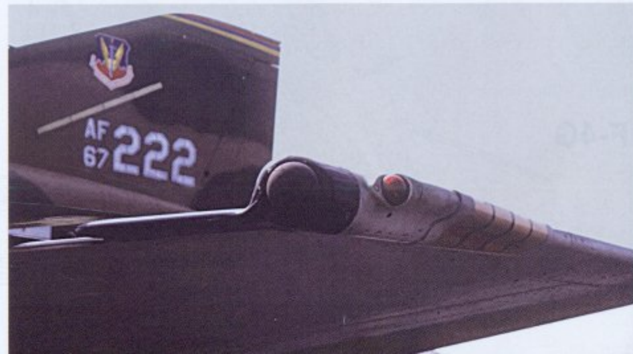
Close-up of the wingtip showing the ECM antenna and the Red formation light. (author)
