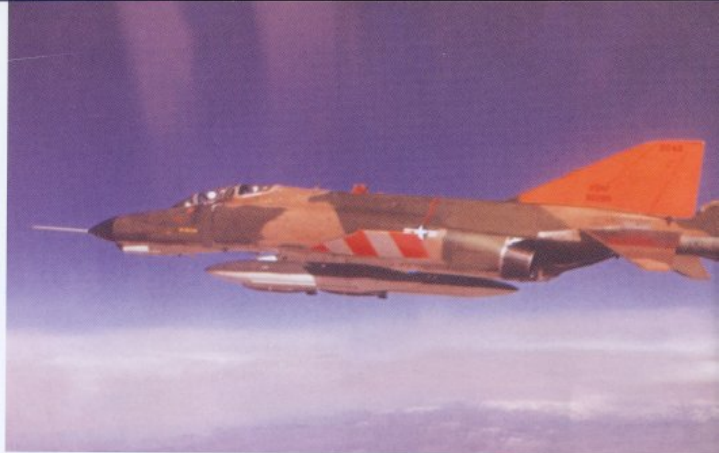
An F-4E modified for use as a spin test aircraft. The large protuberance from the aft fuselage carried a special drag chute which would induce the aircraft into a flat spin. The tail is painted Orange, while the outer wing panels are Orange and White for photo purposes. (USAF)
