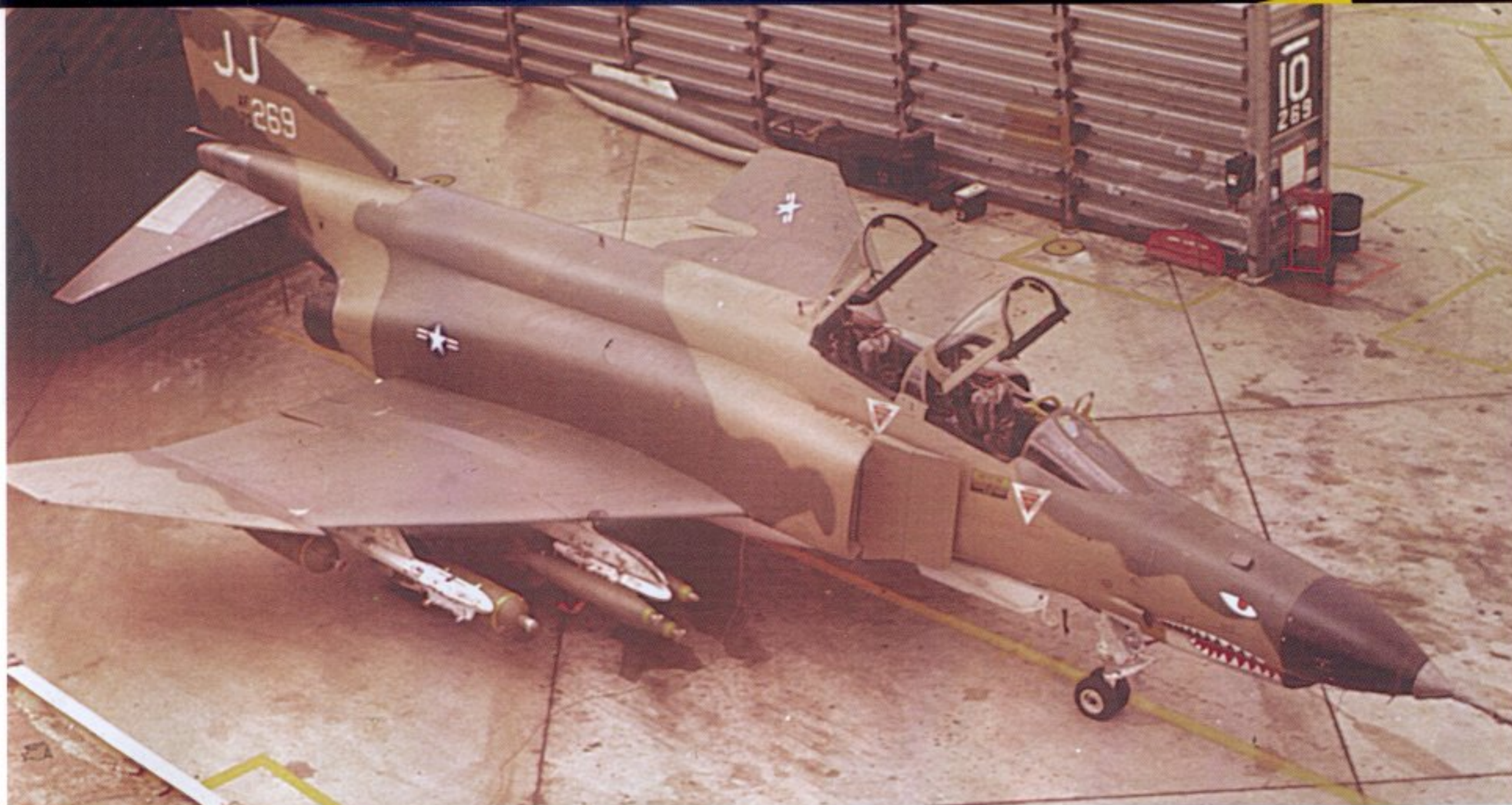
A 34th TFS F-4E, 67-269, in a revetment at Korat RTAB, Thailand in 1969. The upper surface camouflage is clearly shown. Camouflage paint of Air Force tactical aircraft was initiated in 1965, and the F-4Es were delivered in what is commonly referred to as the Southeast Asia or "Lizard" scheme of two greens (FS 595a: FS 34102 and 34079) and Tan (30219). The revetments were made of corrugated steel which was filled with dirt. (USAF)
