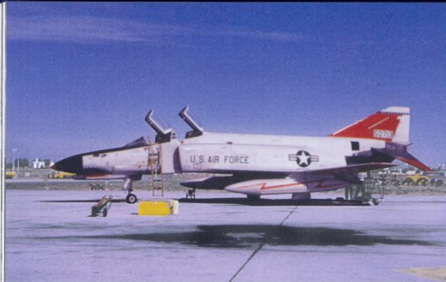
This YF-4E, 65-0713, was painted White with Red lightning bolts and Red tail when it was assigned to the Flight Test Center at Edwards AFB, California. The aircraft was actually built as an F-4D-28 and then modified to YF-4E specifications. It was used as a flying test bed for virtually all the modifications performed on the F-4E series. (Mick Roth)
