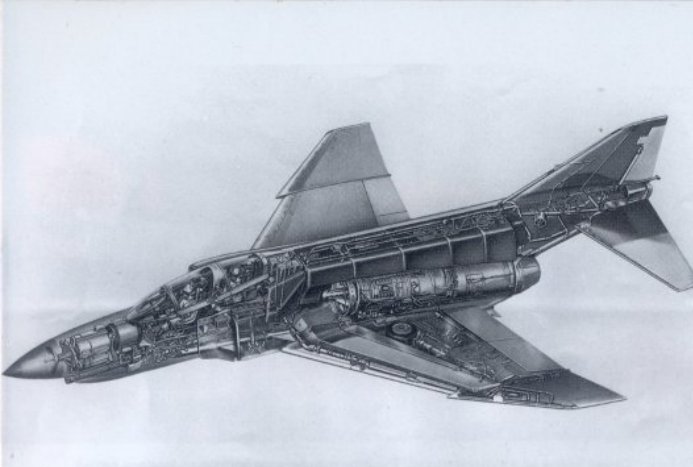
Cutaway drawing of the F-4E Phantom II showing the new APQ-120 radar unit and the M61A-1 Gatling cannon and ammo drum. (McDonnell-Douglas)
