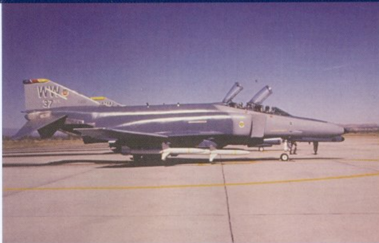
Just prior to Desert Shield/Desert Storm, the Air Force changed the tactical camouflage to a two-tone Gray scheme. This is the 37th TFW CO's F-4G on the ramp at George AFB in 1988. The two colors are Gunship Gray (36118) and Aircraft Gray (36270). The aircraft carries four AGM-88 HARM missiles. (USAF)
