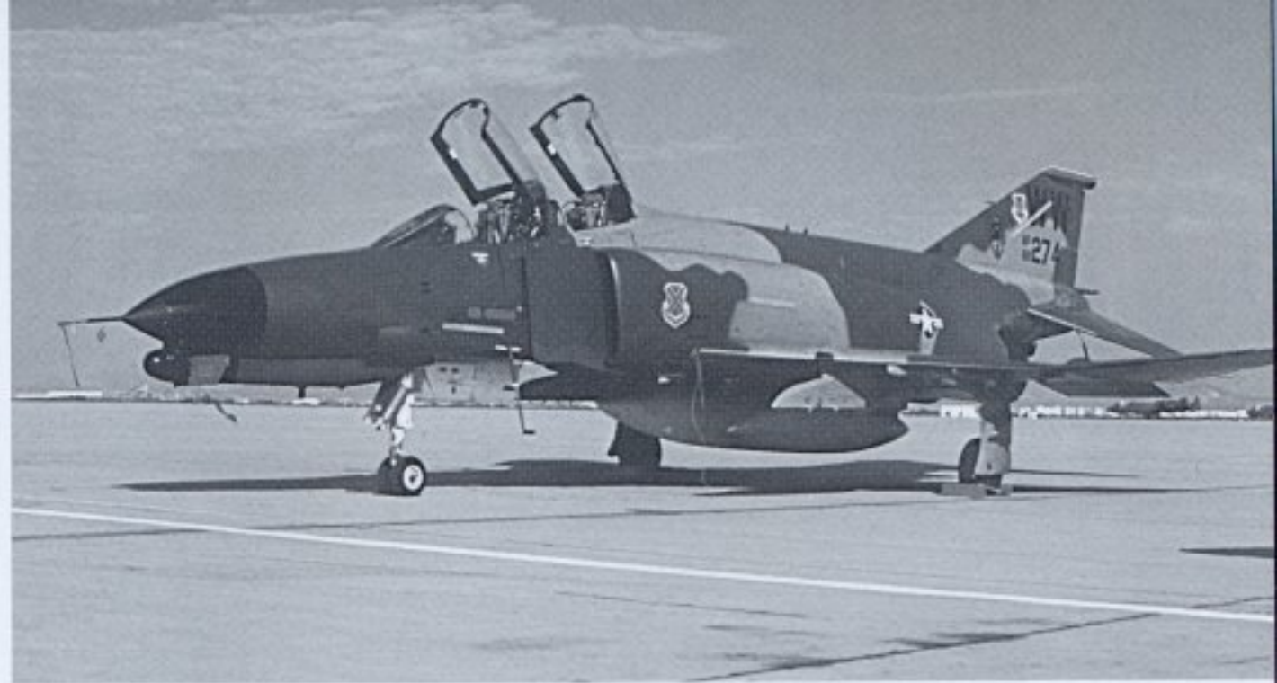
A 561st TFS F-4G-43 on the ramp at George AFB in May 1981. The 35th TFW was renumbered the 37th TFW on 30 March 1981, retaining its "WW" tail codes, and absorbing its squadron assets, including the 561st and 562nd squadrons F-4Gs. The F-4G carried the 600-gallon centerline fuel tank originally designed for the F-15 Eagle. (Brian Rogers)
