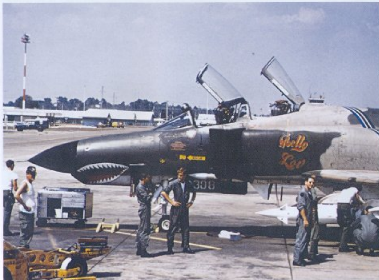
"Betty Lou," F-4E, 67-308, was the personal aircraft of Col. Allen MacDonald, the CO of the 388th TFW at Korat in 1968. The aircraft carries a pair of Douglas AGM-12B Bullpup missiles on the inboard pylons, for a strike against a bridge target on the Ho Chi Minh Trail in 1969. The inside of the nose wheel door is painted dark Green with the aircraft tail number in White. (Tom Brewer)
