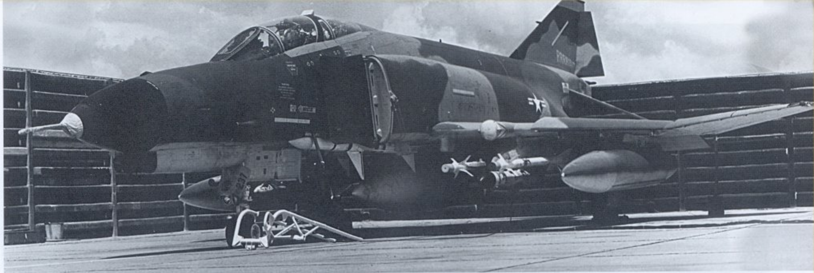
"RRRRibit," an F-4E-48, 71-237, assigned to the 555th TFS at Udorn in March 1974. The aircraft has all the latest improvements including leading edge slats. The object protruding from the leading edge is the Target Identification System Electro-Optical or TISEO, a powerful telescopic TV camera for identifying targets at extreme ranges. The F-4E is armed for a counter-air mission with four AIM-9J Sidewinder missiles, four AIM-7 Sparrow missiles, and ALQ-101 ECM pods. (Joe Bruch collection)
