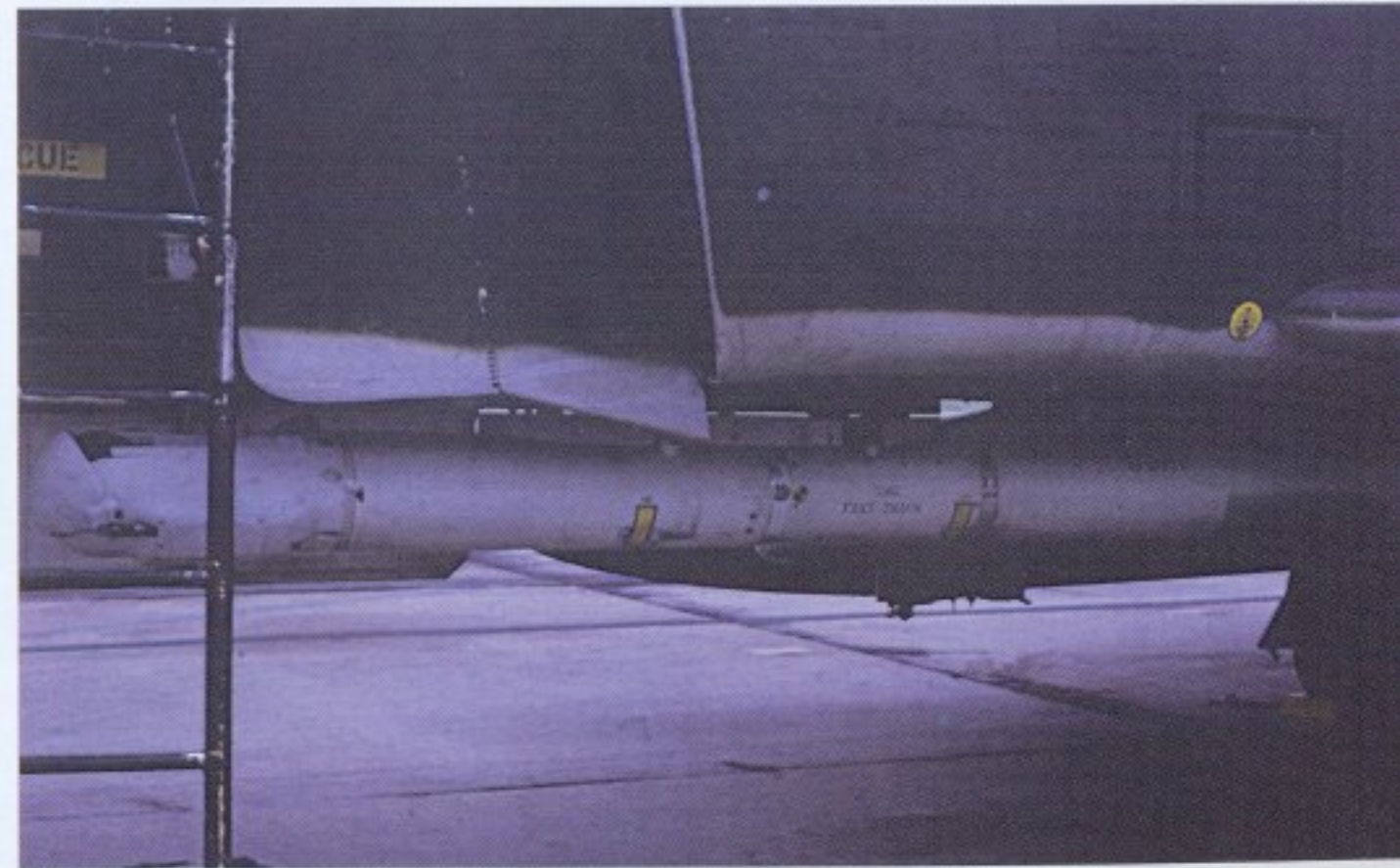
The Pave Spike pod was mounted in the left forward missile bay, and was used to guide several types of munitions to the target. (Mick Roth)
