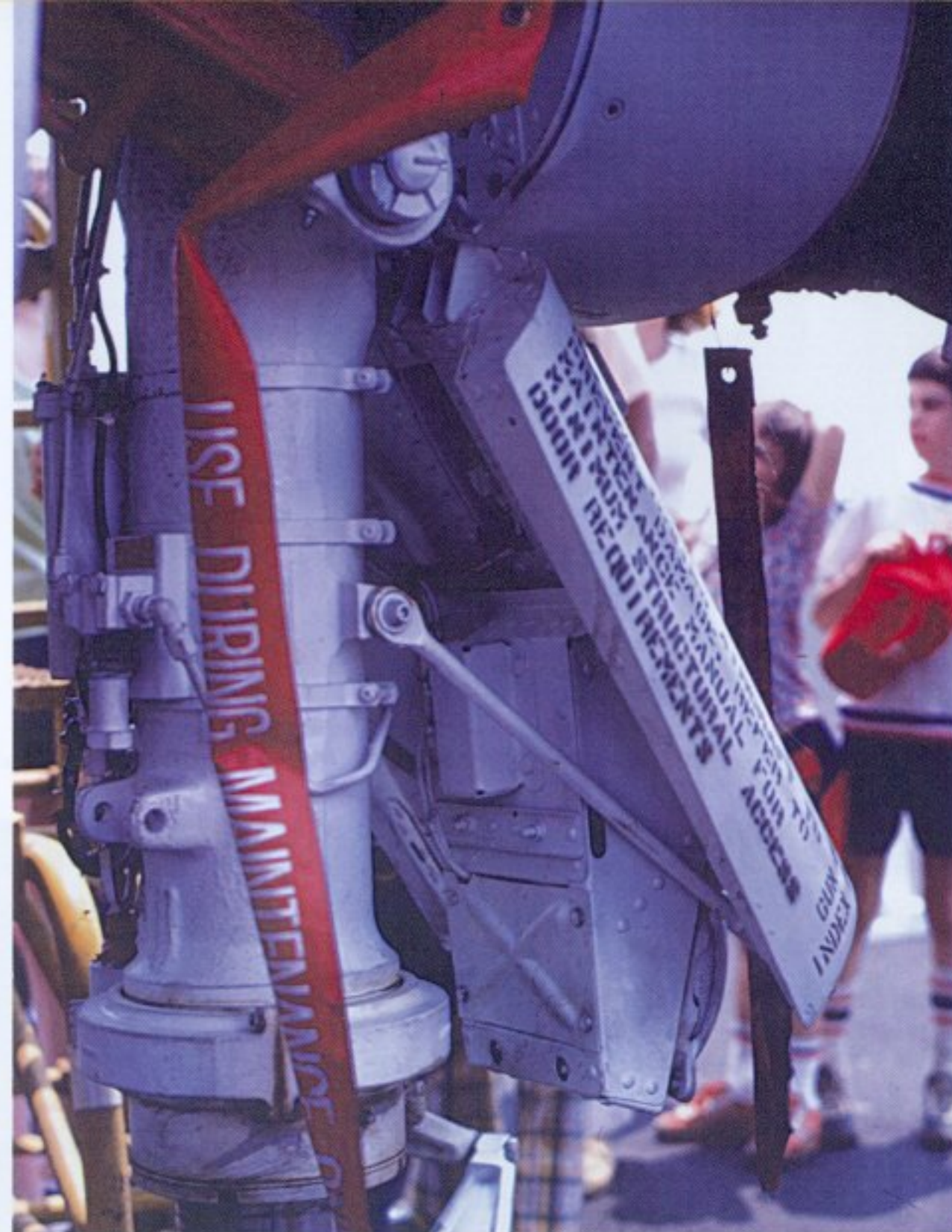
(Top left) The nose wheel strut showing the typical condition of the White paint that covered everything except the polished portion of the strut. (author)
