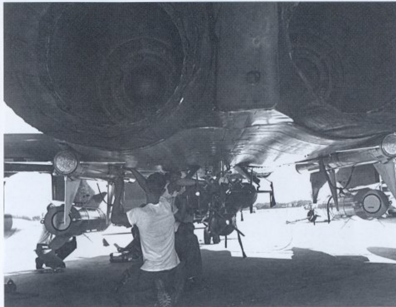
Sgts. Bill Spickerman and John Widner, armorers with the 388th TFW at Korat RTAB, Thailand, inspect the connections on the centerline bomb rack in 1969. The F-4E also carries a pair of AIM-4 Sparrow missiles recessed into the underside of the fuselage, and a pair of AGM-12B Bullpup missiles on the inboard pylons. This view also looks directly into the exhausts of the J79 engines. (USAF)
