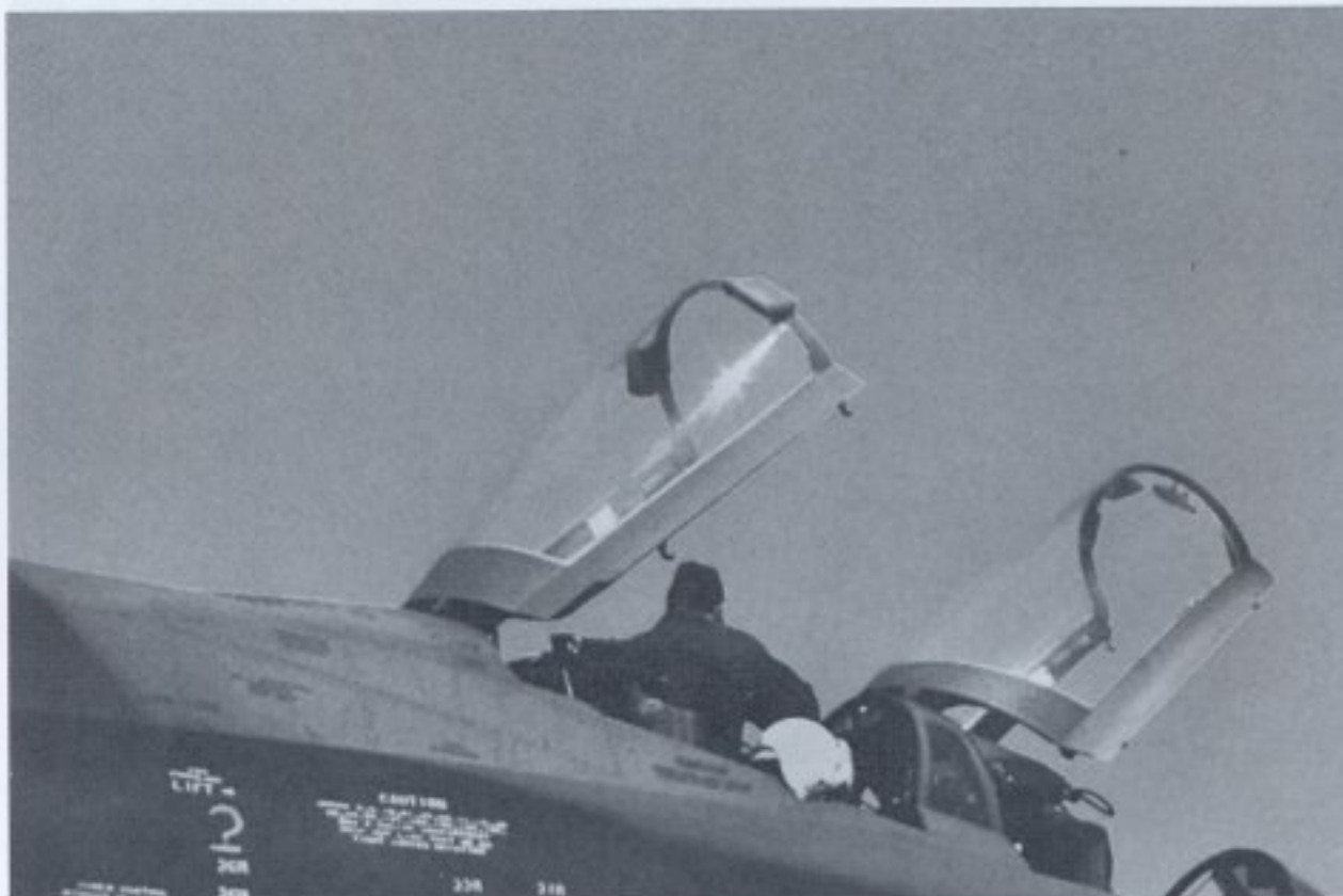
(Above photos) Two views of the underside of the canopy, which is Black, showing two different types of rear view mirrors. The hooks extending from the bottom of the canopy are locks. The object fastened to the front left side of the canopy frame is a knife to allow the pilot to cut through the Plexiglas canopy in case of an emergency, a very difficult thing with the sharpest knife. (author)
