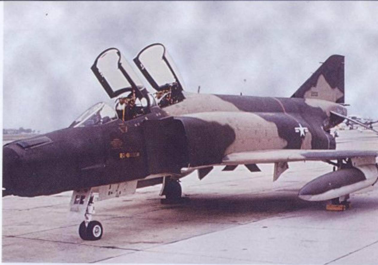
The RF-4C prototype, serial number 62-12200, was used to test the feasibility of mounting the General Electric M61A-1 20mm Gatling cannon internally in an F-4 airframe. Combat pilots in the skies over North Vietnam had loudly complained about a lack of a gun when all their missiles had been fired. McDonnell-Douglas answered their complaints with the F-4E. (Tom Brewer)
