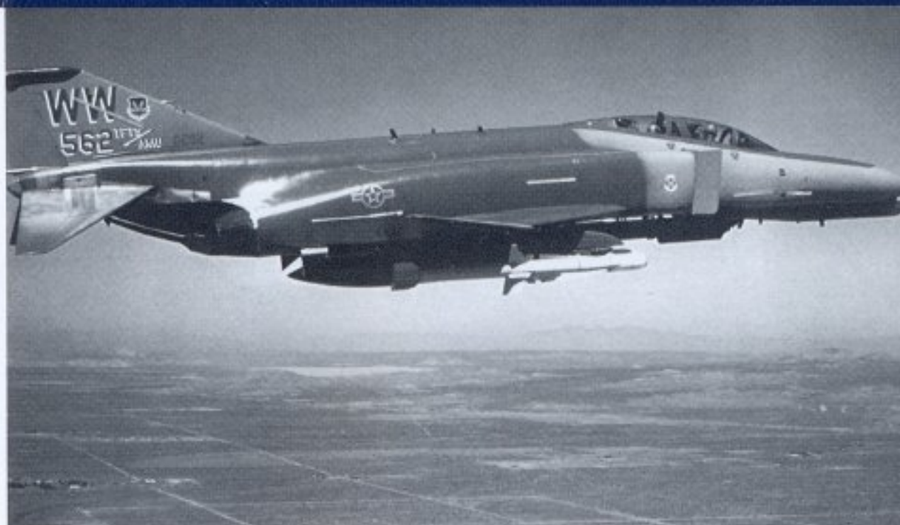
An F-4G-42 from the 562nd TFFS with a full load of live AGM-65 Mavericks and AGM-88 HARMs on its way to the live-fire range at Edwards AFB. All the squadrons within the 37th TFW were training units, thus the unit designation TFFS. (USAF)
