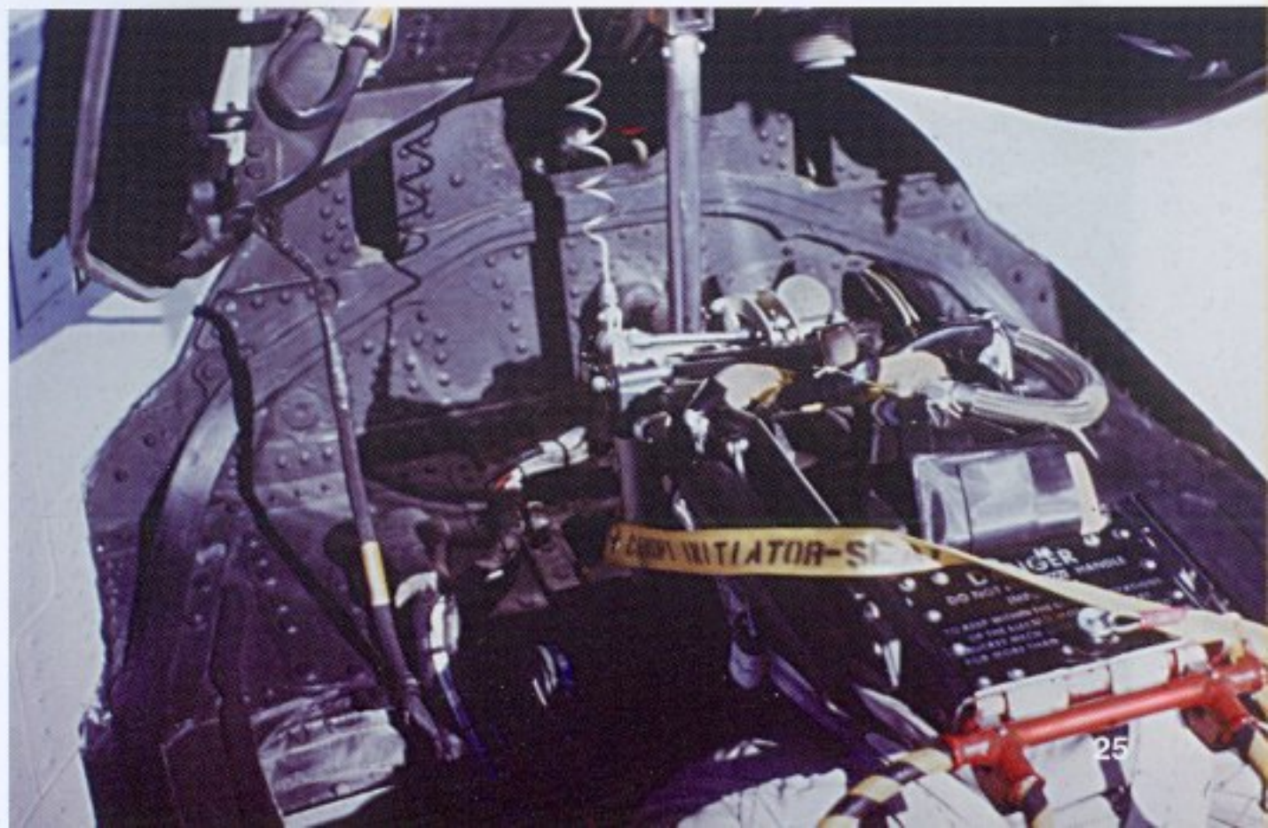
Behind the seat in the rear cockpit of an F-4E showing the canopy actuator. The spiral line is the canopy extractor line that blows off the canopy just prior to ejection. (Hugh Muir)
