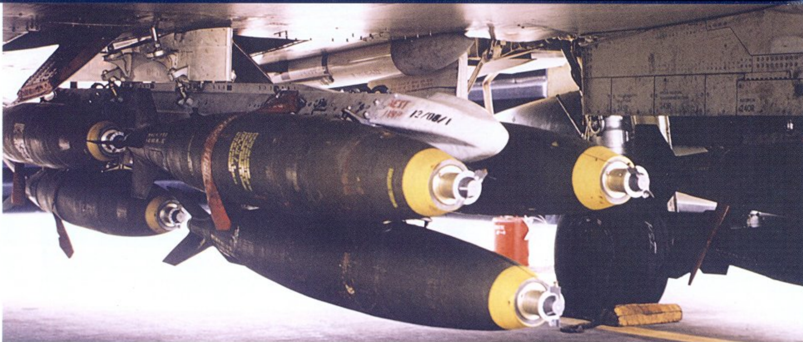
Close-up of the Multiple Ejector Rack mounted on the fuselage centerline of an F-4E at Udorn in 1972. The ordnance is six Mk. 82 LDGP 500-pound bombs. Note that the centerline pylon, the MER itself, and each bomb on the MER has its own stabilizing screws. (Tom Brewer)
