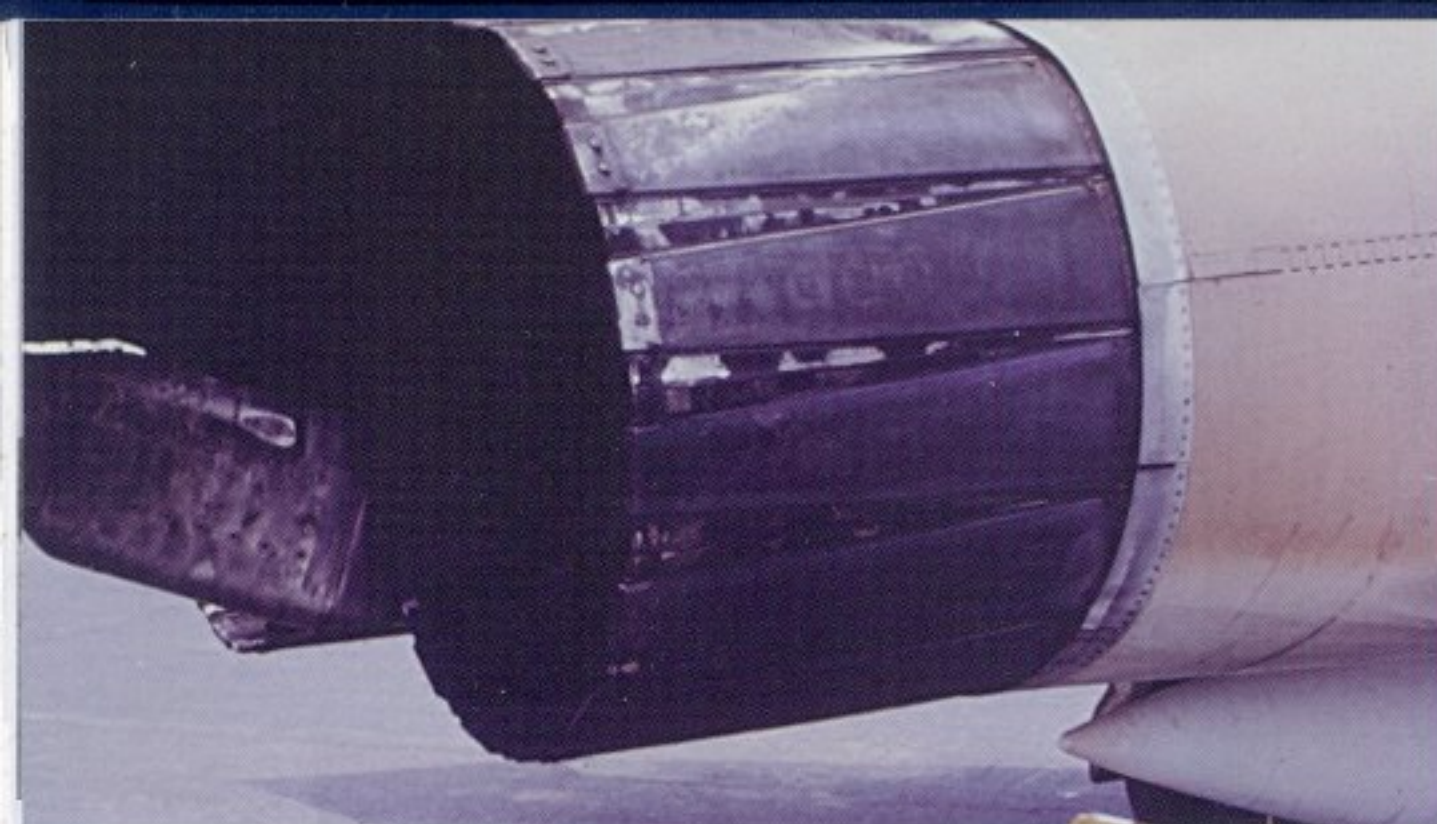
(Above photos) The afterburner exhaust pipes of the J-79-GE-17 engines. The exhausts are variable in size, which increases the thrust of the engines. (Bob Ulrich)
