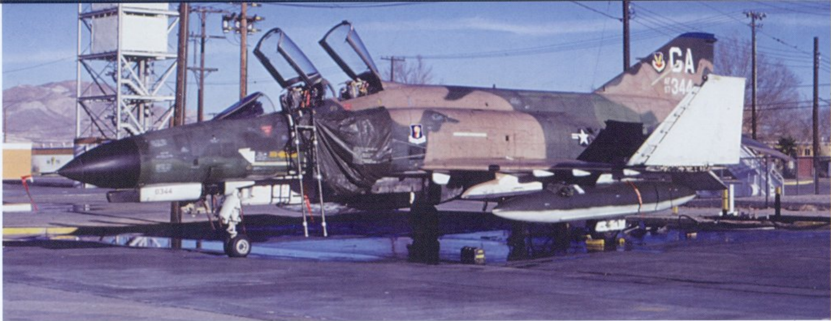
A 35th TFW F-4E on the wash rack at George AFB showing that even with leading edge slats, Air Force Phantoms retained the folding wingtip capability originally designed for Navy carrier operations. (author)
