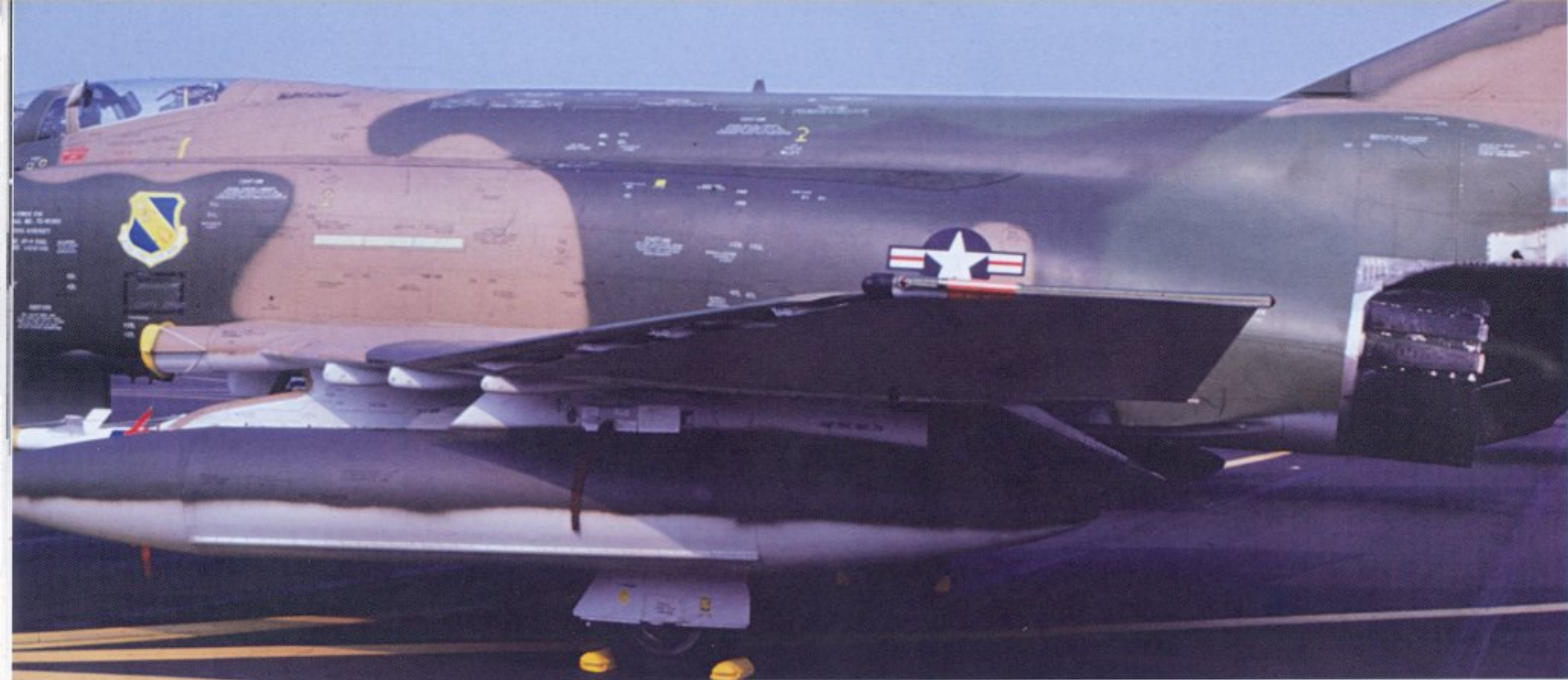
The left outer wing panel showing the wingtip formation light panel with a Red formation light on the front and rear of the wingtip, which had a dihedral of 12 degrees. The right wing had Green lights. This F-4E has the leading edge maneuvering slats. (author)
