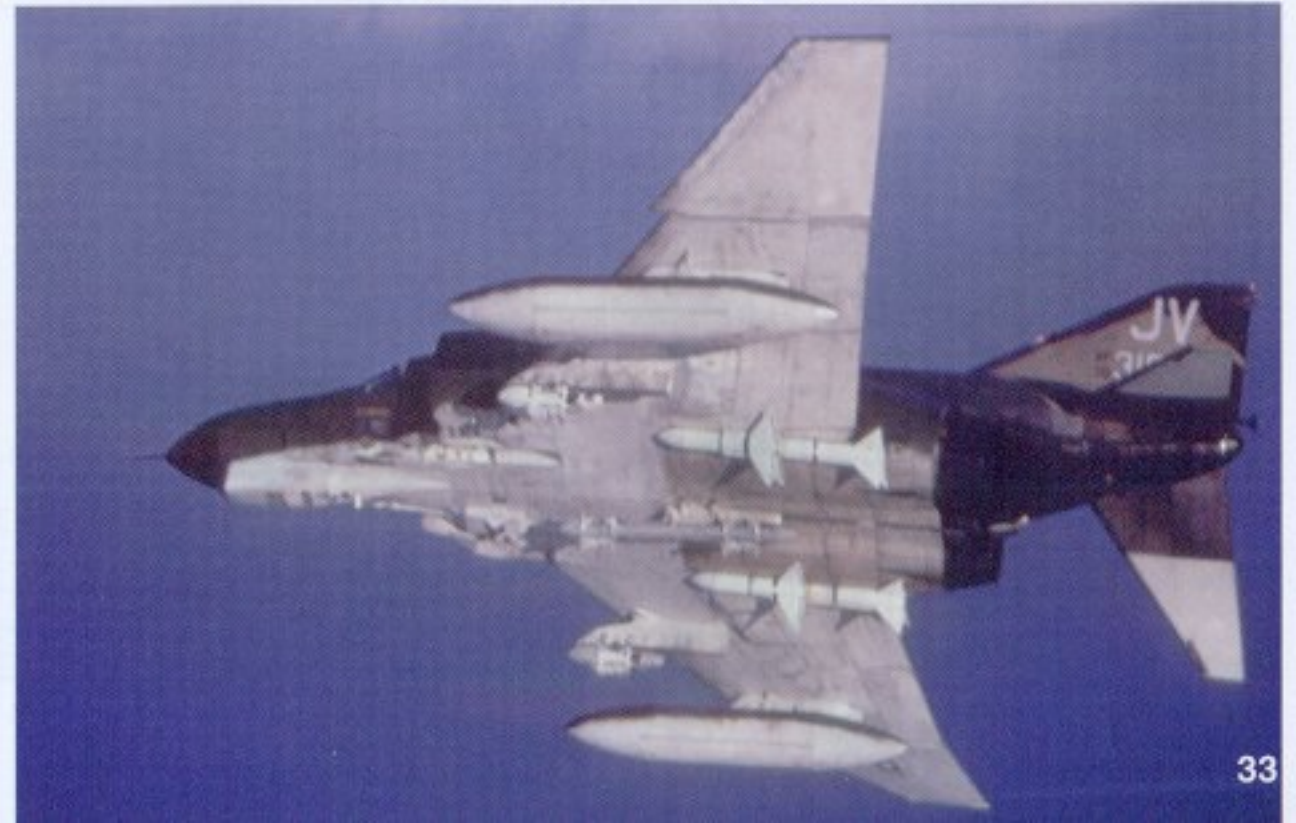
A 469th TFS F-4E, 67-315, banks away from the camera to show the full underside of the aircraft. The weathered areas and dirt around the engine bays are significant. The aircraft has a bomb damage assessment camera mounted in the left forward Sparrow bay. (Don Logan)
