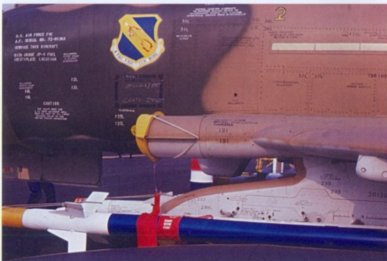
(Bottom two photos) Side view and top view of the TISEO camera mounted on the left leading edge of the wing. The AIM-9 Sidewinder launch rails are also shown to advantage. Note placement of the RBF tapes on the missile rails. (author)
