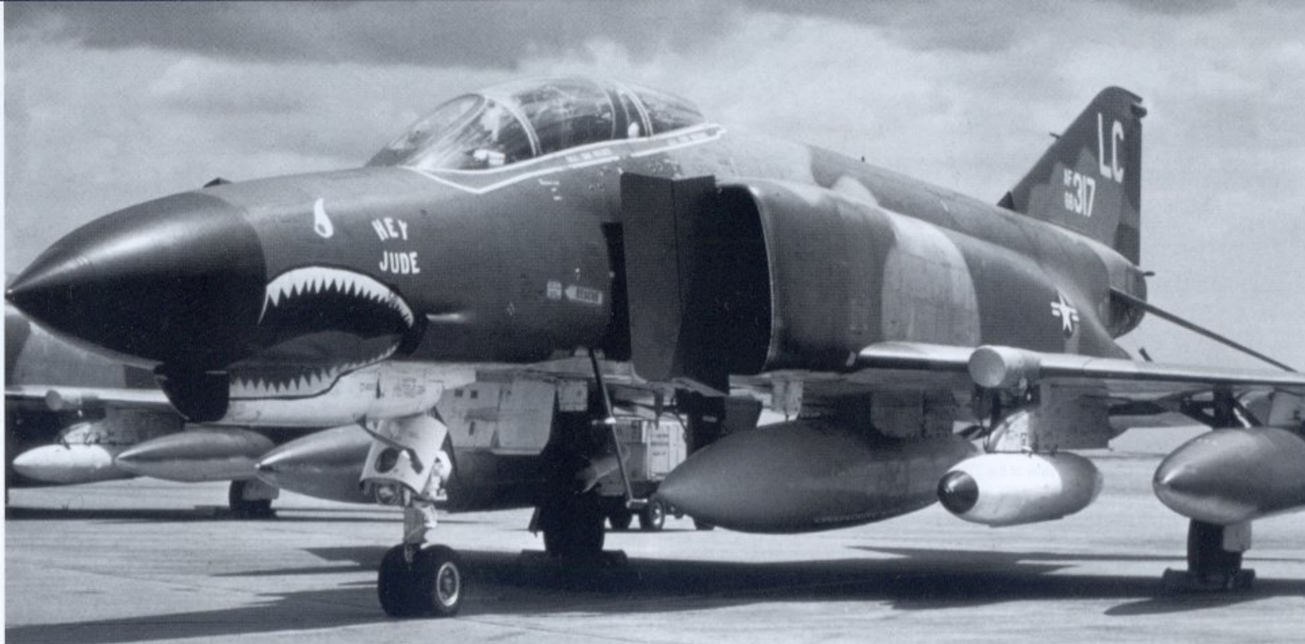
"Hey Jude," an F-4E-37 assigned to the 421st TFS at Udon in 1972. The aircraft has a TISEO unit on the wing leading edge, but it is not equipped with leading edge slats. On the left pylon is a baggage pod to carry the crew's personal items. The canopy trim is Red and White, while the tail tip is Red. The name is White. (USAF)
