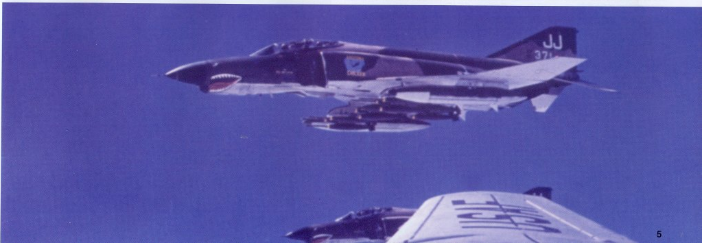
"Arizona Chicken" (68-371) and "Here Come The Judge" (67-208), a pair of 34th TFS F-4Es, form up just off the wingtip of the KC-135 tanker prior to turning toward North Vietnam in 1968. Both of these aircraft carry a full load of 500-pound Mk. 82 low drag general purpose (LDGP) bombs, some having 36-inch fuse extenders. (USAF)
