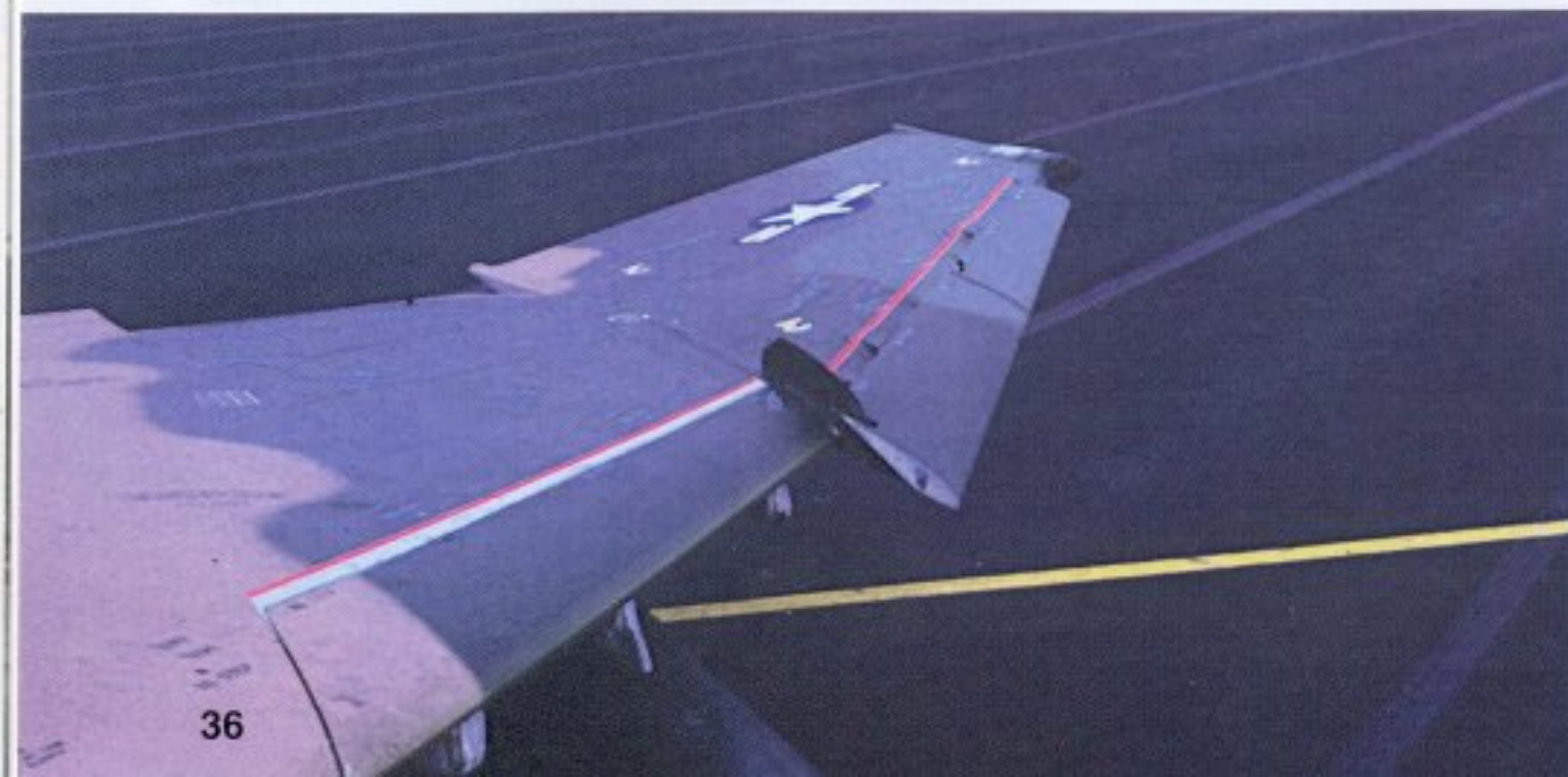
The upper wing of a slat-equipped F-4E showing the size, shape, and position of the flow fence. The Red and White stripe is a "no step" border for the main wing slats. (author)
