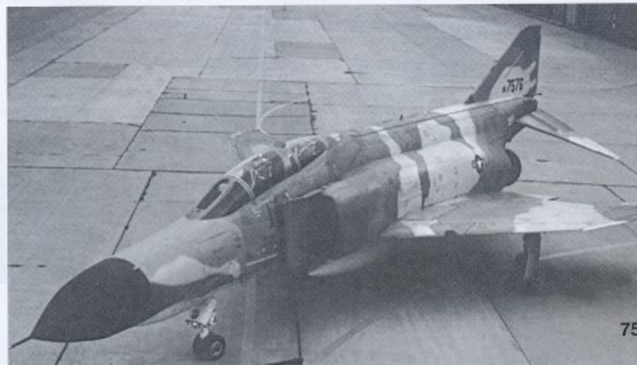
A very unusual aircraft was the F-4E(S), which was built for the Israeli Air Force. It was basically an RF-4E with a special HIAC LOROP camera for very high resolution photos. Only three were built, all for Israel. The Israeli camouflage scheme is seen. (Mick Roth)
