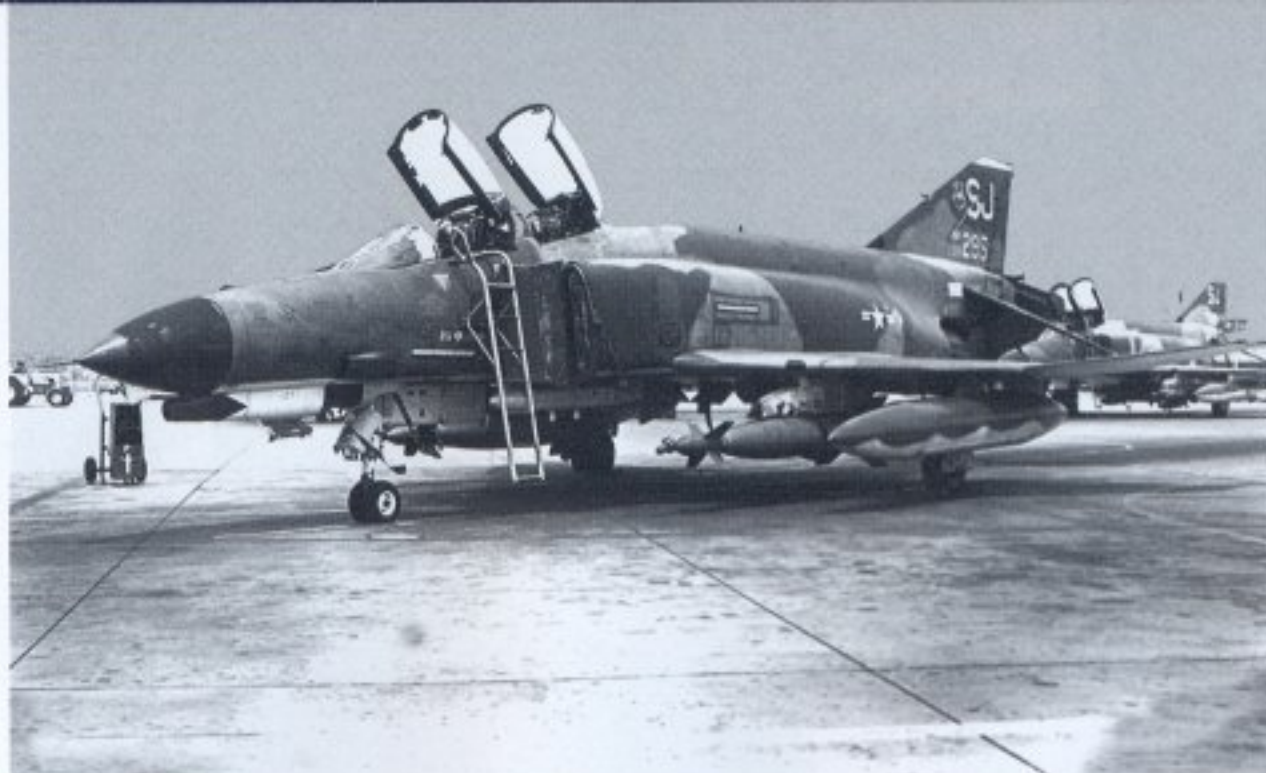
Another unit that deployed to Southeast Asia during the 1972 Linebacker operations was the veteran 4th TFW from Seymour Johnson AFB, North Carolina. This F-4E-42 is armed with a pair of GBU-10 2,000-pound LGBs. The F-4 would drop the LGBs near the target, and a target designator aircraft, usually an F-4D, would then guide the bombs to the target. (John Poole)
