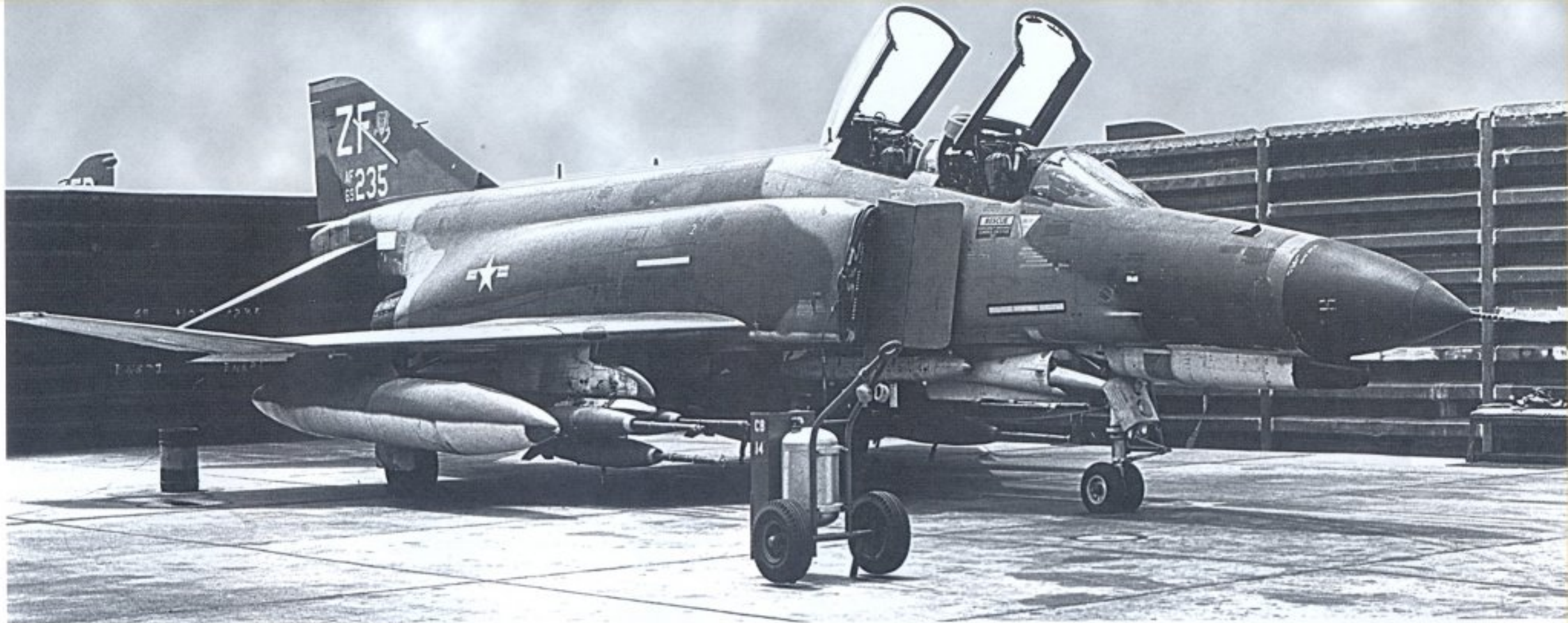
A 31st TFW F-4E-43 in a revetment at Udorn in 1972 armed with six Mk. 82 LDGPs with fuse extenders. The 31st deployed from Homestead AFB, Florida, to the war zone as part of Operation Constant Guard, which built up forces in SEA to counter the North Vietnamese Easter Offensive. (John Poole)
