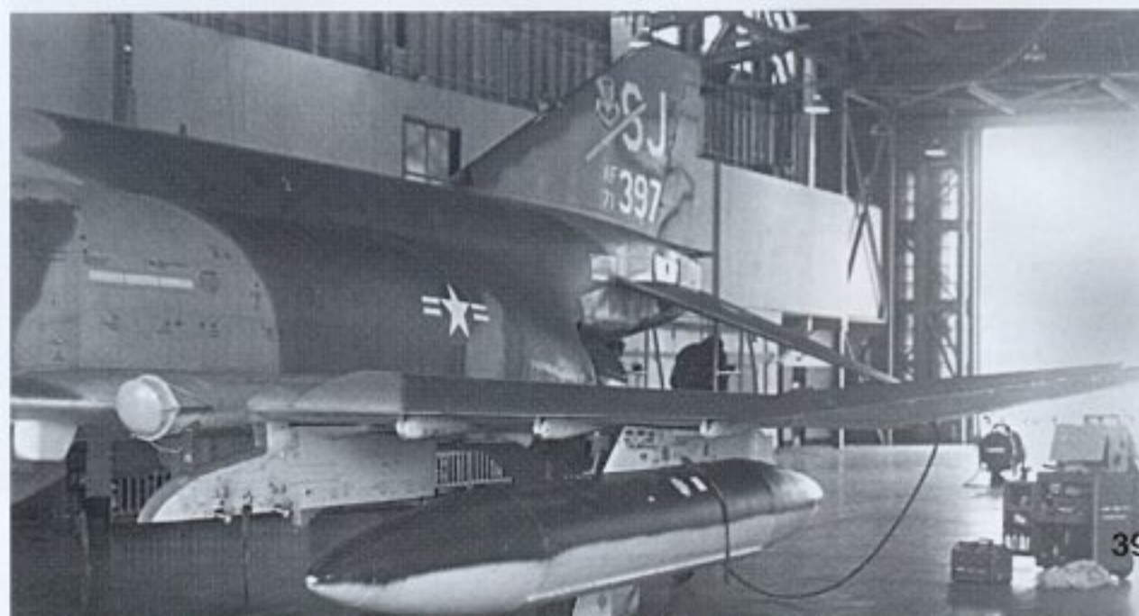
The wing showing the leading edge maneuvering slats in full deployed position. (author)
