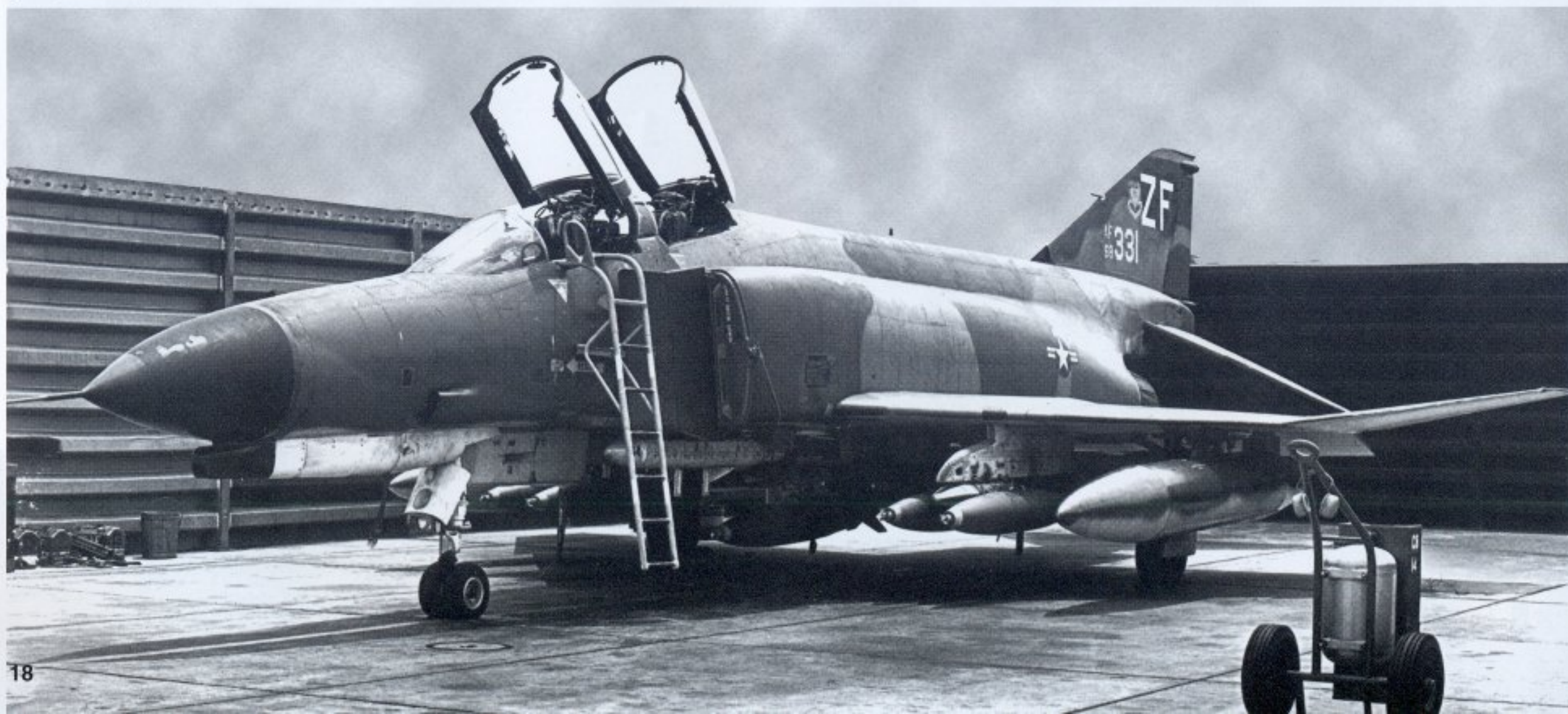
A 308th TFS F-4E-37 in a revetment at Udorn in 1972 armed with 500-pound LDGP bombs for a strike against North Vietnamese Army targets. The 308th TFS deployed from Homestead AFB, Florida, to the war in Southeast Asia as part of Operation Linebacker to counter the North Vietnamese Easter invasion of South Vietnam. Both front Sparrow missile bays contain ALQ-87 electronic countermeasures pods. (John Poole)
