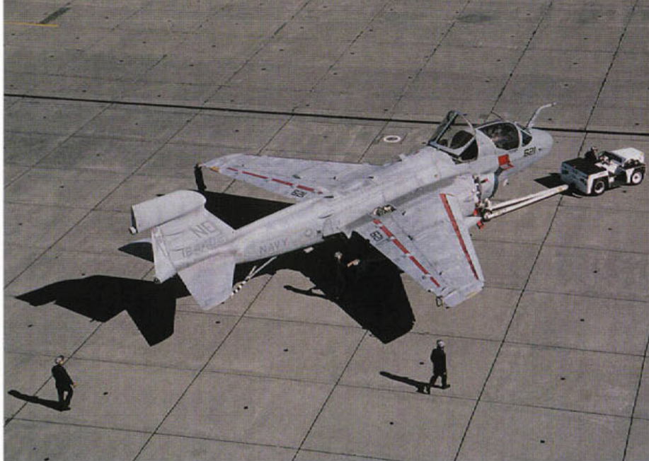
A tractor tows this EA-6B ICAP-II Block 86 (NE-621/BuNo 164402) assigned to VAQ-131 from the hangar at NAS Whidbey Island. The NE tail code was assigned to the air wing aboard USS CONSTELLATION (CV-64). Splotchy paint indicates the corrosion team's efforts to stay ahead of the constant problem associated with carrier-based aircraft. The 621 modex on the nose and flaps is Black for improved visibility on the flight deck. (B. Trombecky)
