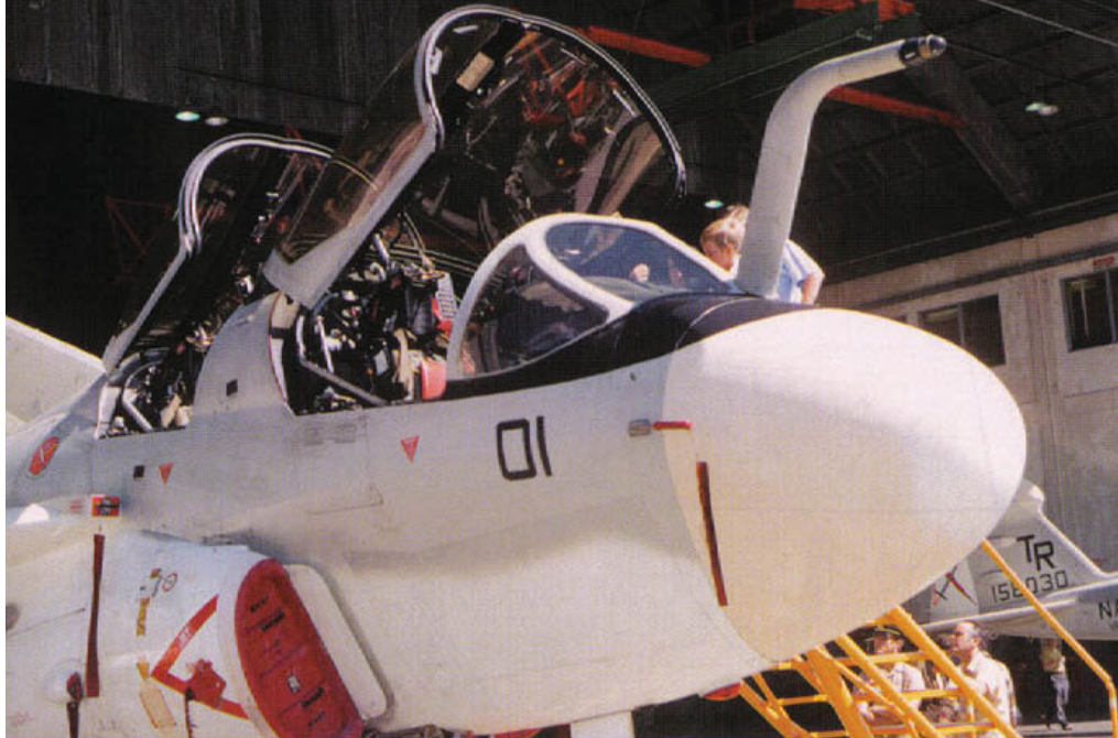
An EA-6B Prowler (Standard) assigned to Tactical Electronic Warfare Squadron One Twenty Nine (VAQ-129) undergoes maintenance at Naval Air Station (NAS) Whidbey Island, Washington in 1972. The refueling probe lacks the AN/ALQ-126 Electronic Countermeasures (ECM) receiving antenna, which was fitted to upgraded Prowlers. A red protective cover protects the starboard pitot tube that is immediately aft of the radome. (D. Barnes)
