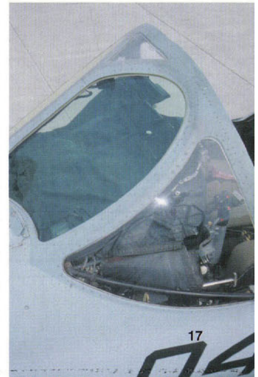
(Left) The EA-6B's windshield has untinted panels, in contrast to the gold-tinted canopies. This Block 89A Prowler's windshield consists of two forward panels, two quarter panels to the port and starboard sides, and a small triangular panel on the upper center section. The fixed refueling probe is canted 12° to starboard to improve the pilot's forward view.
