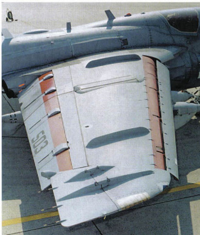
A tractor tows this EA-6B ICAP-II Block 86 (NE-621/BuNo 164402) assigned to VAQ-131 from the hangar at NAS Whidbey Island. The NE tail code was assigned to the air wing aboard USS CONSTELLATION (CV-64). Splotchy paint indicates the corrosion team's efforts to stay ahead of the constant problem associated with carrier-based aircraft. The 621 modex on the nose and flaps is Black for improved visibility on the flight deck. (B. Trombecky)
