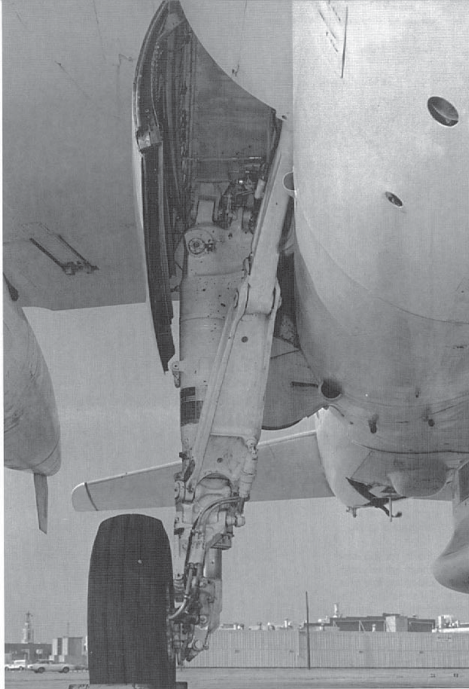
The EA-6B main landing gear strut is similar to those on other A-6s; however, the Prowler's struts are strengthened to support higher aircraft gross weights. The main gear system consists of an air-oil shock strut, a multiple-disk wheel brake, a single wheel and a 36-inch (91.4 cm) by 11-inch (27.9 cm) tire, plus a drag brace.
