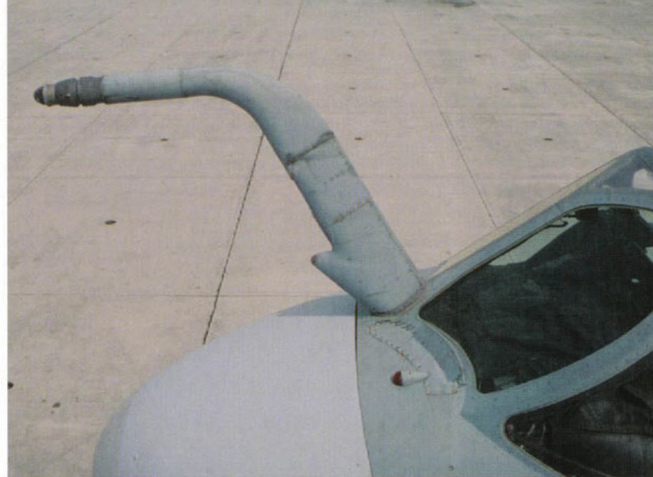
This Block 89A Prowler's refueling probe has a saw tooth housing at the base of the refueling probe which is angled to starboard. This housing incorporates the receiving antenna for the Sanders AN/ALQ-126 Noise Deception Jammer. This system – an update of the Sanders AN/ALQ-100 fitted to early EA-6Bs – is also known by its code name, CHARGER BLUE.
