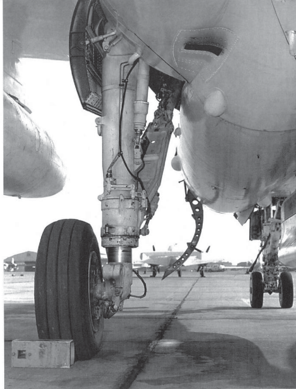
The port main landing gear, like the starboard unit, rotates 82° on retraction. This gear is pulled forward and inward into the wheel well. An anti-lock system is provided, and operates in conjunction with the weight-on wheels switch that prevents landing with locked brakes. The oleo (shock absorbing) strut is left in chrome, while the rest of the gear assembly is glossy Insignia White.
