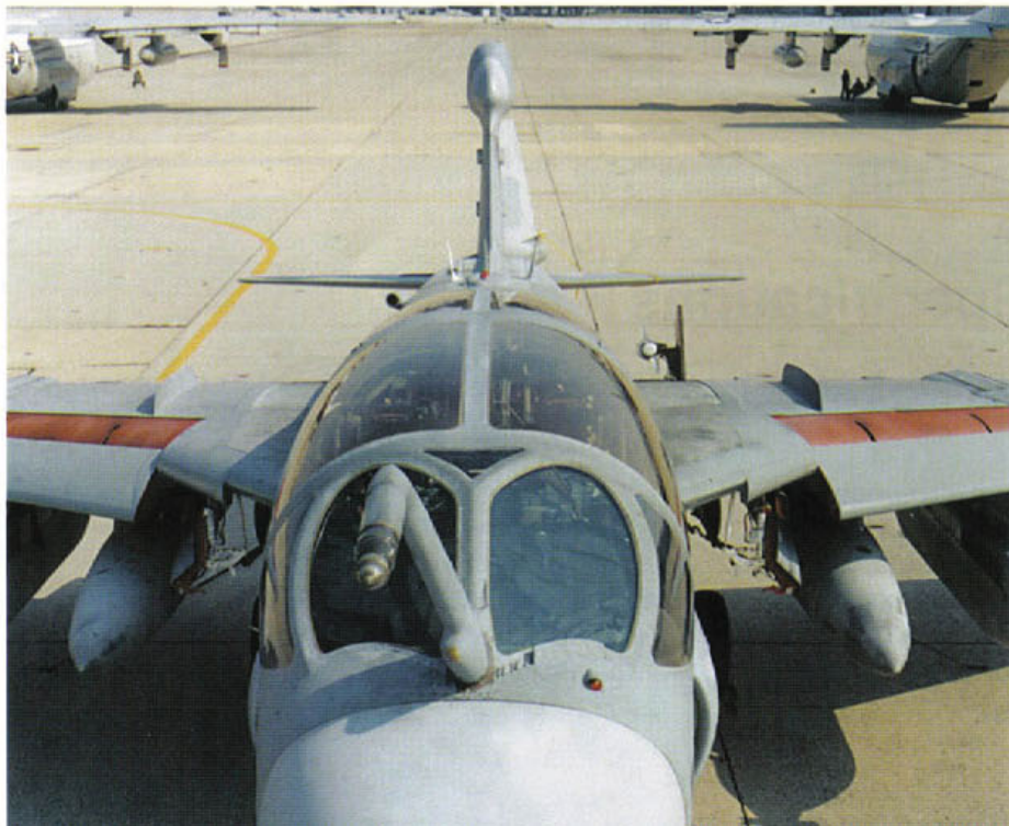
(Left) The EA-6B's windshield has untinted panels, in contrast to the gold-tinted canopies. This Block 89A Prowler's windshield consists of two forward panels, two quarter panels to the port and starboard sides, and a small triangular panel on the upper center section. The fixed refueling probe is canted 12° to starboard to improve the pilot's forward view.
