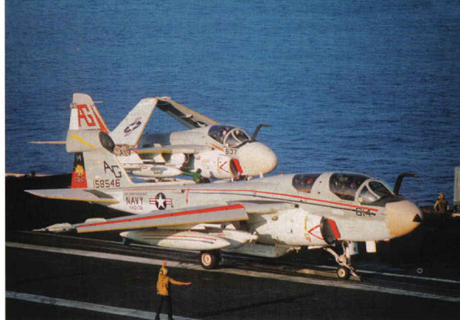
An EA-6B Standard (AG-614/BuNo 158546) from VAQ-136 'Gauntlets' prepares to launch from catapult No. 3 aboard USS INDEPENDENCE (CV-62) during July of 1977. A VA-65 A-6E Intruder (AG-507) on catapult No. 4 is also preparing to launch. This Prowler was written off (WO) on 13 May 1982. Tan (approximately FS13695) anti-corrosion strips are placed on the wing and tail leading edges. (US Navy)
