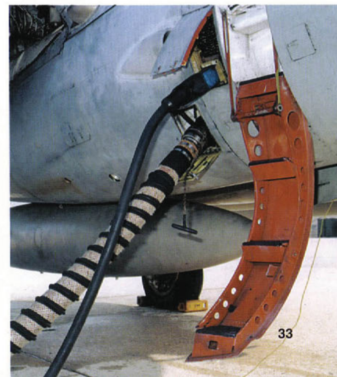
An external electrical power cable is plugged into the power receptacle, which is located on the starboard forward fuselage. The opened access panel for this power receptacle also has the external refueling panel. This panel is immediately forward of the single point refueling receptacle. An air hose from an External Power Unit 'Huffer' is connected to the engine bay receptacle. The EA-6B does not have self-starting engines; instead, compressed air starts the starboard engine, which then provides power to start the port engine.
