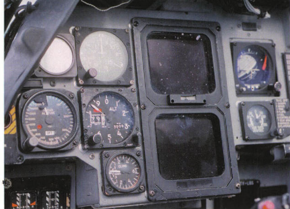
Five gauges are mounted on the port edge of the pilot's instrument panel. The Angle of Attack Indicator is located on the upper left, with the Radar Altimeter immediately below. The second column consists of (from top) the Mach Speed Indicator, the Servo Barometer Altimeter, and the Rate of Climb indicator. The two screens are the Electronic Attitude Director Indicator (EADI; top) and the Electronic Horizontal Situation Indicator (EHSI)
