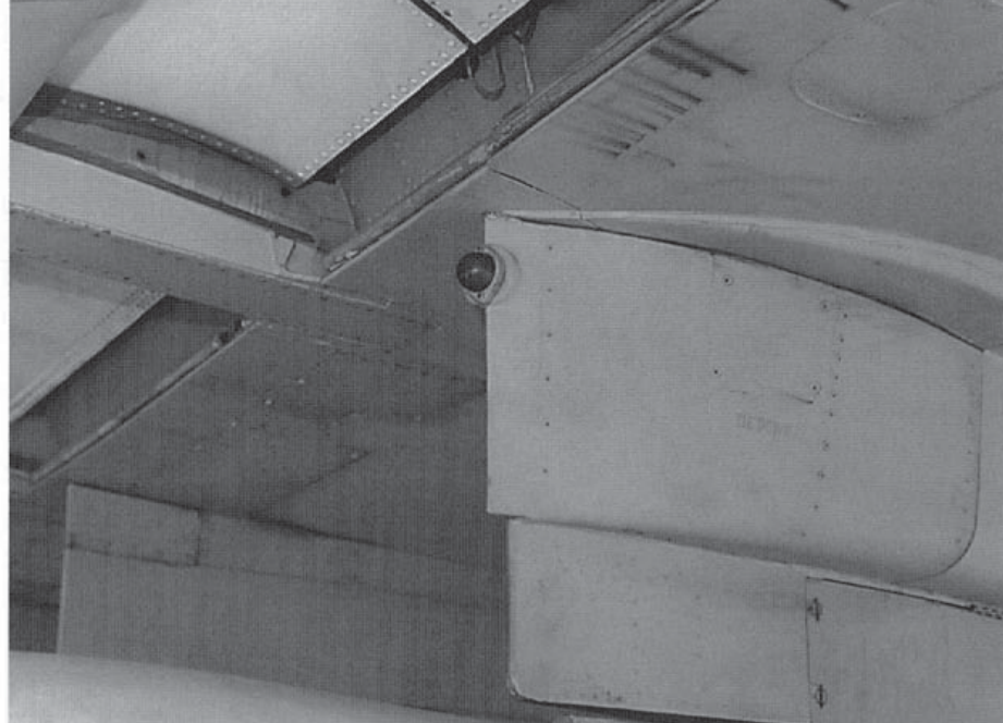
A green starboard position light is fitted to the aft end of the station No. 5 (outboard right) pylon. A red port position light is housed in the aft end of the station No. 1 pylon. A-6 Intruders had both the port and starboard lights in amber. These lights reflect off the lowered flaps and aid the Landing Signal Officer (LSO) during carrier recovery operations. The inner framework of the main wing section is the same color as the wing undersurface.
