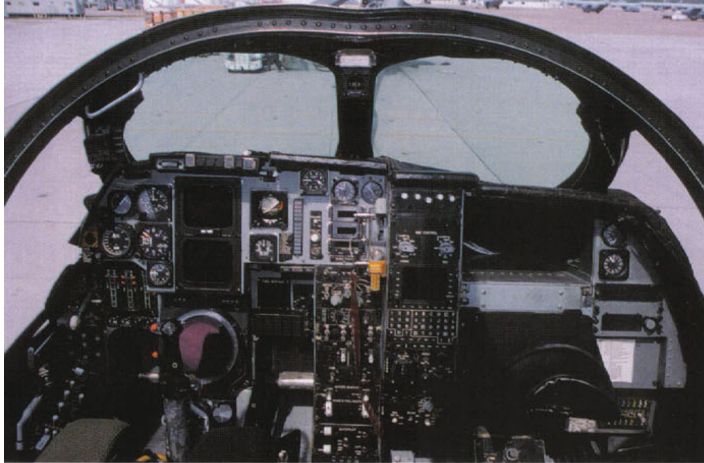
The pilot sits to port and the Electronic Countermeasures Officer One (ECMO-1) sits to starboard in the Prowler's front cockpit. This EA-6B ICAP-II Block 89A cockpit had slight differences in equipment fit from earlier Prowler variants. The gray front canopy control handle is mounted on the instrument panel's center section, immediately above the yellow canopy jettison handle.
