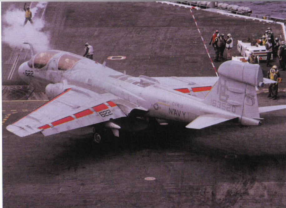
A VAQ-138 EA-6B ICAP-II (Block 86) (NG-622/BuNo 163520) taxis towards Number One catapult aboard USS NIMITZ (CVN-68). The Prowler was assigned to Carrier Air Wing Nine (CVW-9). Non-skid strips are used atop of the fuselage, the inner wing area that abuts the fuselage, and the horizontal stabilizer's inner area. The non-skid material's color ranges from white to black. (B. Trombecky)
