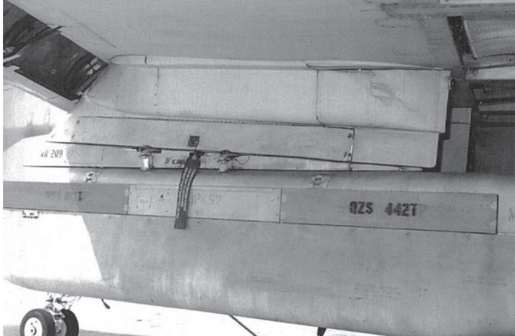
The station No. 1 (outboard left) pylon is painted the same Light Compass Gray (FS36375) as the Prowler's underside. A REMOVE BEFORE FLIGHT pin is inserted between the two sway braces on the pylon. The red flag attached to the pin has this information in white: REMOVE PIN BEFORE FLIGHT, INSERT PIN TO SHOULDER, DO NOT FORCE REMOVAL OF PIN.
