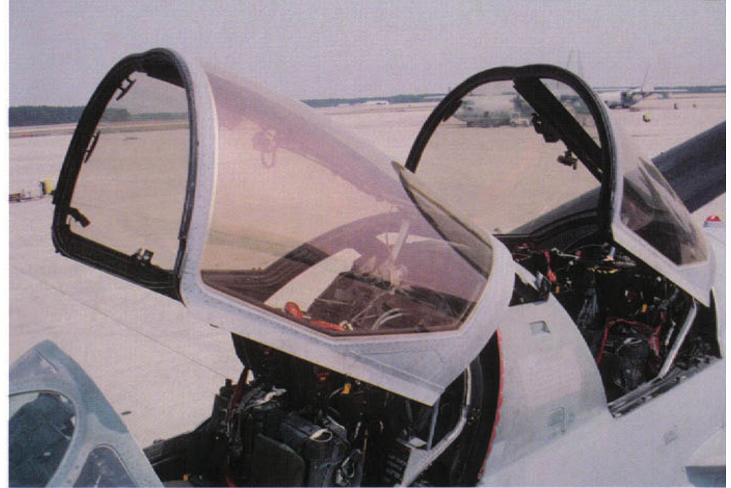
The EA-6B's forward canopy is larger than the aft canopy. Canopy frames flare outward at the base to align with the fuselage contours. Two handgrip locations with flush doors are positioned in the fuselage section between the canopies on both fuselage sides.
