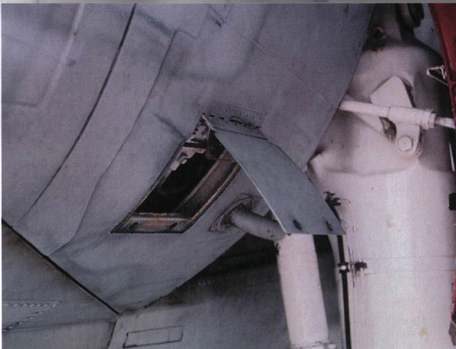
The opened panel provides access to the starboard main landing gear hydraulic system. The override valve inside this panel is identical to the one fitted on the port gear fairing. An engine oil drain pipe is located in front of the access.
