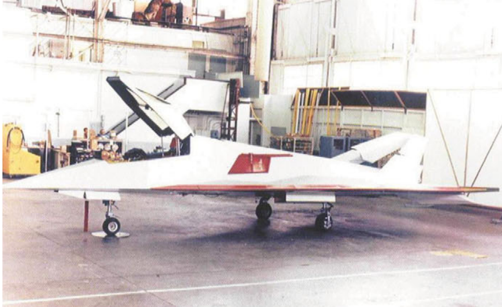
The first HAVE BLUE (1001) is fully assembled in Building 82 of the Lockheed Skunk Works facility in Burbank, California. Red covers protected the engine intakes from ingesting foreign objects and the wing's leading edge from damage to the Radar Absorbent Materials (RAM) on its surface. HAVE BLUE 1001 was later dismantled and flown on a Lockheed C-5A Galaxy to Area 51, where the HAVE BLUE was reassembled and began test flights in December of 1977. (Lockheed Martin via Tony Landis)
