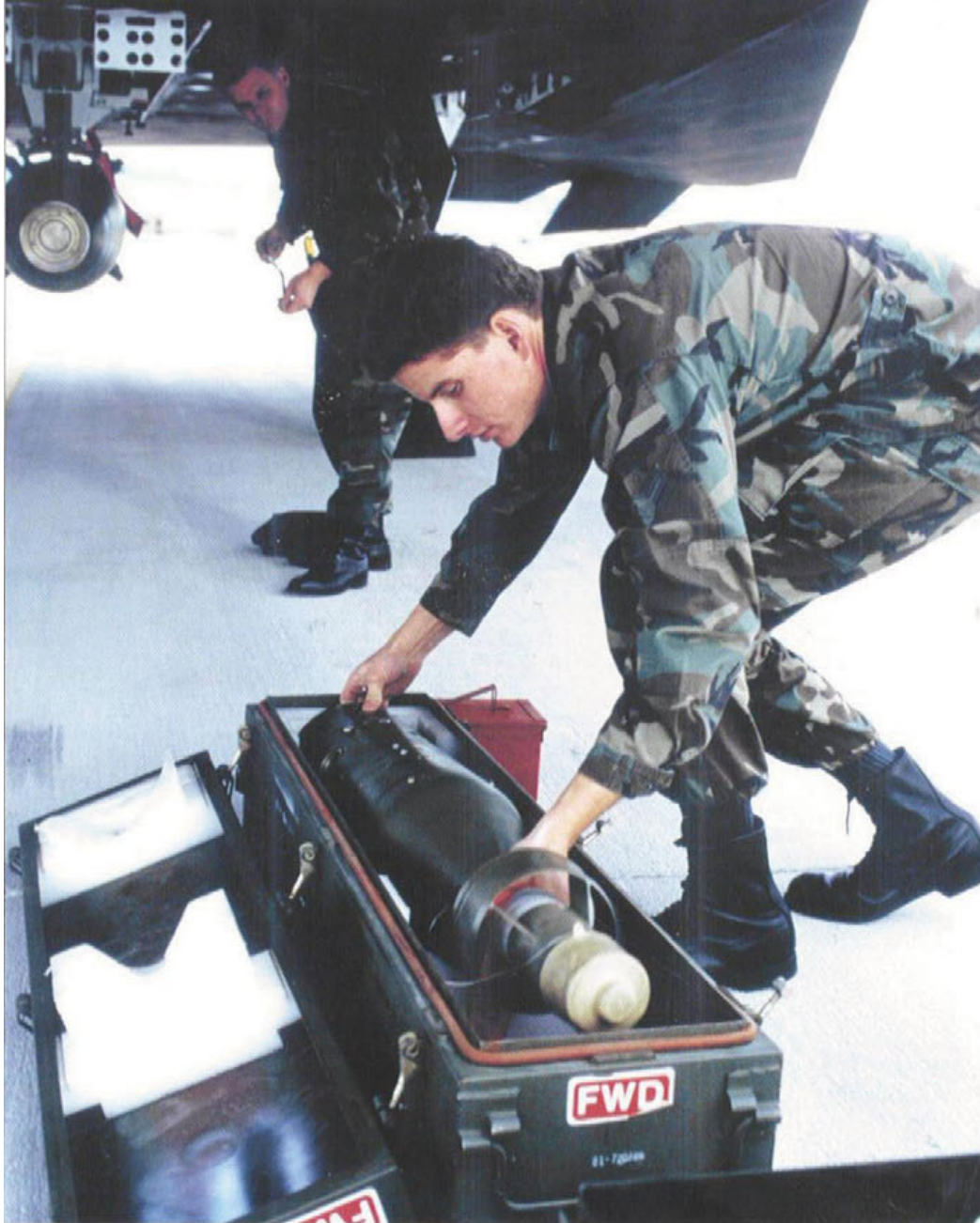
A weapons technician prepares to install the laser seeker head to a 2000 pound GBU-10 Paveway II laser guided bomb, which was fitted to the F-117A's port weapons bay trapeze. The weapon and the seeker are always shipped in separate containers to prevent the possibility of the weapon detonating accidentally. The seeker head focuses on a target 'illuminated' by a laser designator in either the launching F-117A, another aircraft, or from a Forward Air Controller (FAC) on the ground. (Paul Crickmore collection)
