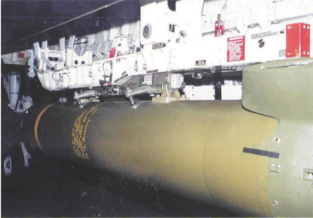
Members of the 410th Flight Test Squadron load a Lockheed Martin AGM-158 JASSM (Joint Standoff Air-to-Surface Missile) into a YF-117A (79-10782) at Air Force Plant 42, Site 7 in Palmdale, California. The JASSM is loaded into the weapons bay using a standard Air Force MJ-1 weapons loader. This weapon is a low-observable cruise missile with a 1000 pound (453.6 kg) warhead and a range of 115 miles (185.1 km). (Lockheed Martin)
