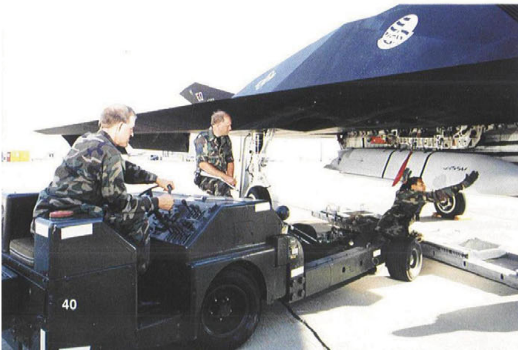
Members of the 410th Flight Test Squadron load a Lockheed Martin AGM-158 JASSM (Joint Standoff Air-to-Surface Missile) into a YF-117A (79-10782) at Air Force Plant 42, Site 7 in Palmdale, California. The JASSM is loaded into the weapons bay using a standard Air Force MJ-1 weapons loader. This weapon is a low-observable cruise missile with a 1000 pound (453.6 kg) warhead and a range of 115 miles (185.1 km). (Lockheed Martin)
