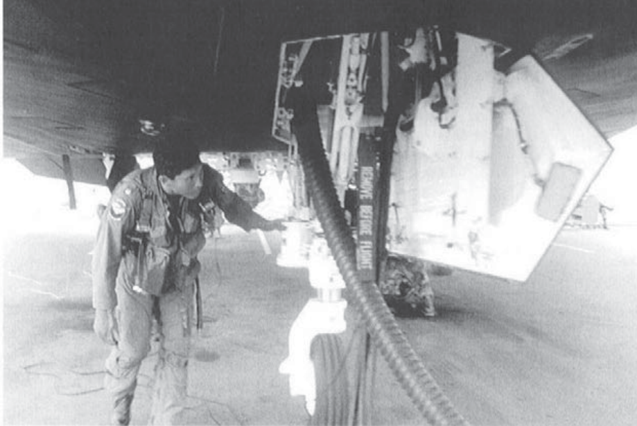
Maj Bowley performs a pre-flight inspection on his F-117A prior to departing Saudi Arabia for the US following Operation DESERT STORM. The hose connected to the nose landing gear well sends compressed air to the two engines' starters. The red REMOVE BEFORE FLIGHT tag is attached to the retraction strut lock, which will be removed by the crew chief prior to engine start. (USAF via G. Phillips)
