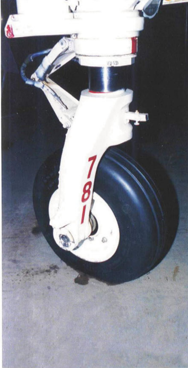
The Goodyear nose landing gear tire measures 22 inches (55.9 cm) in diameter by 6.6 to 10 inches (16.8 to 25.4 cm) wide. Most F-117As have the three-digit tail number painted in red or black on the nose wheel carry-through assembly. This number is derived from the last three numbers of the aircraft's serial number; for example, 781's full serial is 79-10781. (Jim Goodall)
