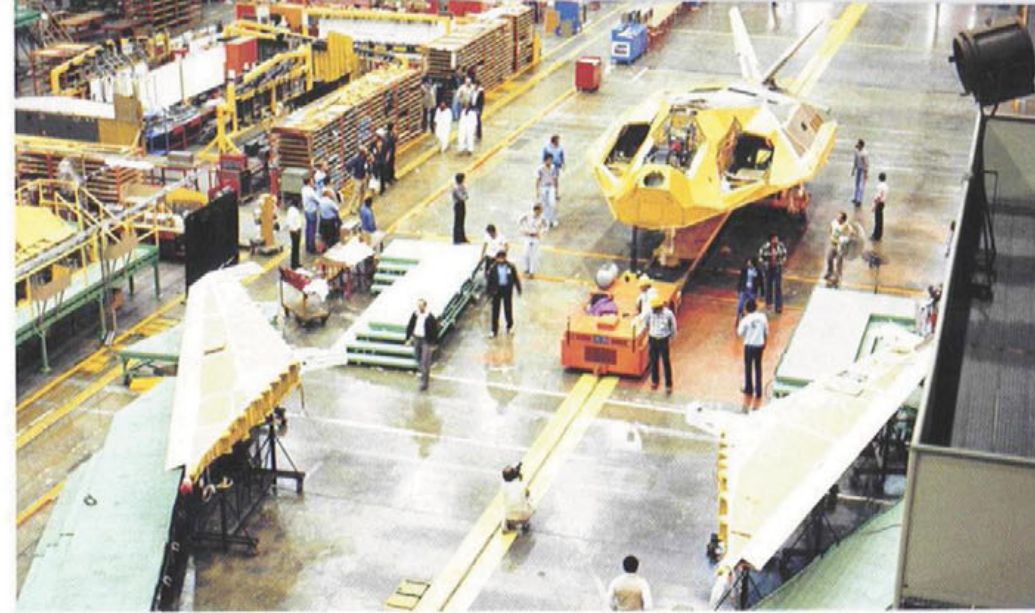
The first YF-117A fuselage assembly is moved down the production line at Burbank, where the wing assemblies await attachment to the fuselage. A tractor towed the assembly fixture carrying the fuselage to the next stage of assembly. Portions of the wing and fuselage assemblies were temporarily covered to protect the Radar Absorbent Materials (RAM) applied to these surfaces. (Lockheed Martin)
