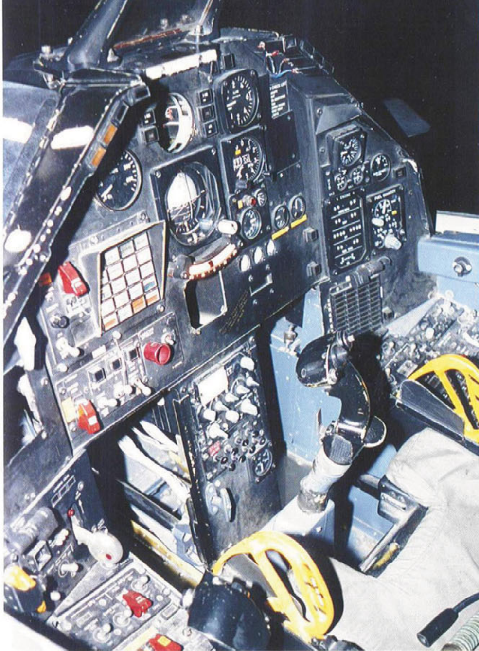
The five YF-117A SENIOR TREND prototypes used analog (conventional) flight instruments in place of the CMDIs and IRAD (Infra-Red Acquisition and Designation) system displays installed on production Nighthawks. The artificial horizon – the light blue and black sphere – was placed in the panel's center. Some test instruments were removed from the cockpit of this YF-117A on display at the US Air Force Museum. (Jim Goodall)
