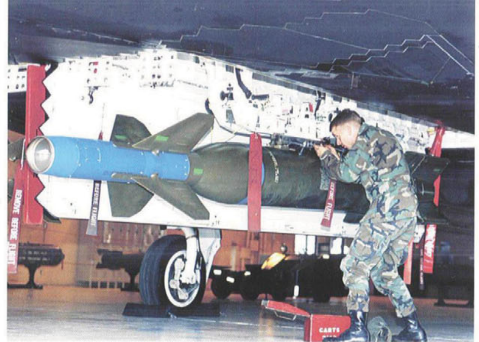
An Air Force ground crewman arms a practice GBU-27 LGB loaded onto an F-117A's port weapons bay trapeze. Removing the safety pins with their REMOVE BEFORE FLIGHT tags arms the weapon. US bombs are painted overall Olive Drab (FS34087); the seeker head and the band around the bomb's front are Dark Blue (FS35109) to indicate a training weapon. The two white perforated plates deployed ahead of each weapons bay are air defectors. These air defectors extend when the bay doors are opened to improve airflow for bomb release. The defectors retract when the weapons bay doors are closed. (Lockheed Martin)
