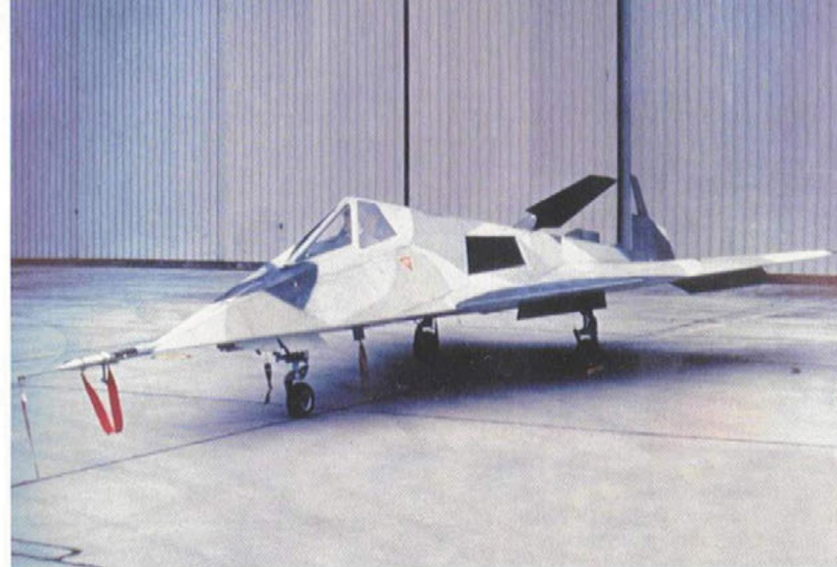
HAVE BLUE 1001 is parked in front of Hangar 13 at the south end of the Groom Dry Lake test facility. The aircraft was painted in a disruptive camouflage scheme of light gray, tan, medium gray, and black to disguise its appearance from Soviet reconnaissance satellites. The instrumentation boom on the nose collected static pressure to confirm flight control data. The Lockheed technician sitting in the HAVE BLUE's cockpit lent scale to this aircraft. (Lockheed Martin)
