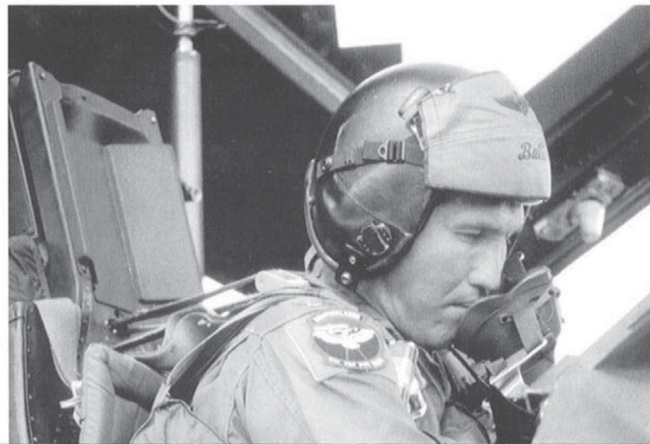
Maj Joe Bowley of the 415th Tactical Fighter Squadron, 37th TFW prepares for takeoff in his F-117A from Saudi Arabia following Operation DESERT STORM in early 1991. He wore a black helmet, which was sometimes chosen by F-117A pilots, although most pilots used the standard issue gray helmets. The shoulder harness on the ACES II ejection seat allows the pilot some forward movement within the cockpit, yet secures him back into the seat during ejection. (USAF via G. Phillips)
