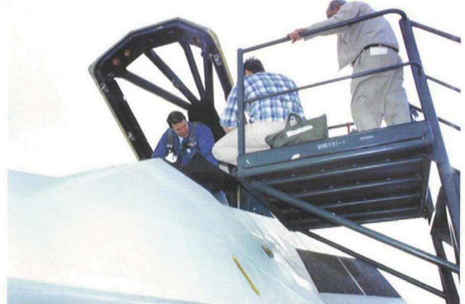
Lockheed test pilot Hal Farley begins his egress from YF-117A Number 780 (nicknamed 'Scorpion 1') after the aircraft's first flight on 18 June 1981. Two company technicians await Farley's departure from the SENIOR TREND. The Low Observable (LO) saw-tooth modifications to the canopy were not yet made at the time of the first flight. (Lockheed Martin via Tony Landis)
