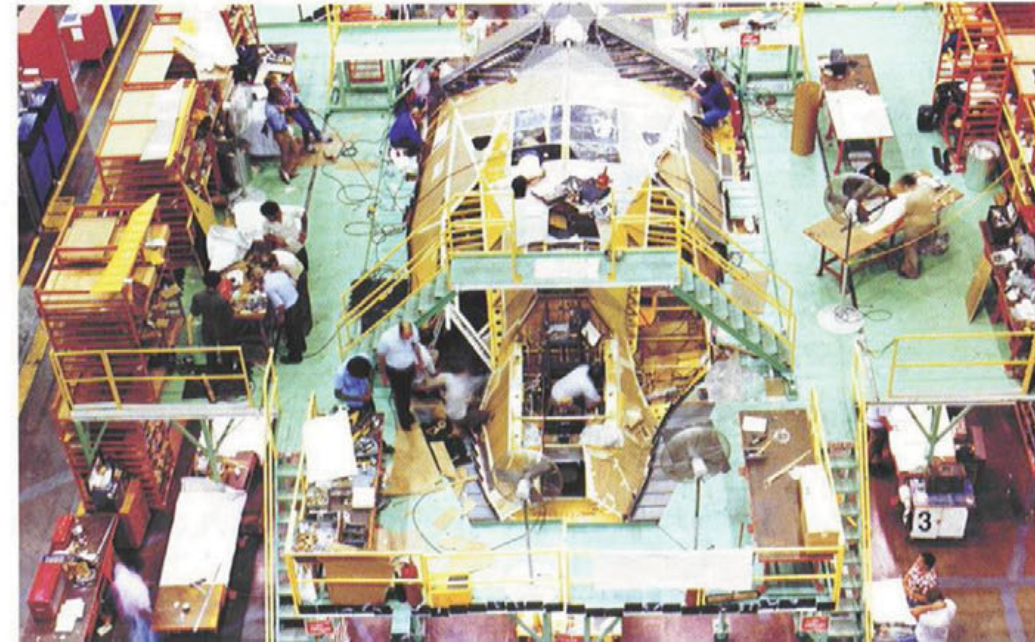
Construction of the YF-117 prototypes and F-117A production aircraft occurred at Lockheed's Burbank plant. Technicians attached the fuel lines, wire harnesses, and control cables to aircraft 780, after the wings (covered by work platforms) were attached to the fuselage. The ailerons were then installed onto the wings and a function test was performed on all aircraft systems. (Lockheed Martin)
