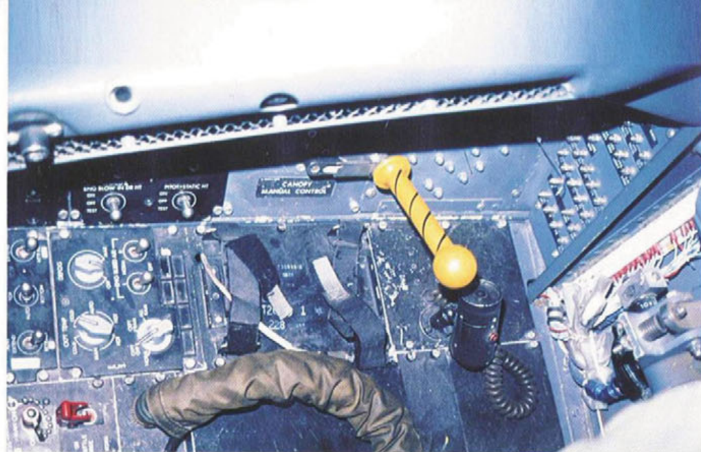
The yellow handle placed on the aft starboard instrument sidewall is the manual canopy control lever, which opens the canopy in the event of a hydraulic system failure. Circuit breakers are placed aft of the canopy handle, while a utility light is fitted near the handle's round knob end. The oxygen hose is a flexible wire-round unit covered with an Olive Drab (FS34087) Nomex sleeve. (Jim Goodall)
