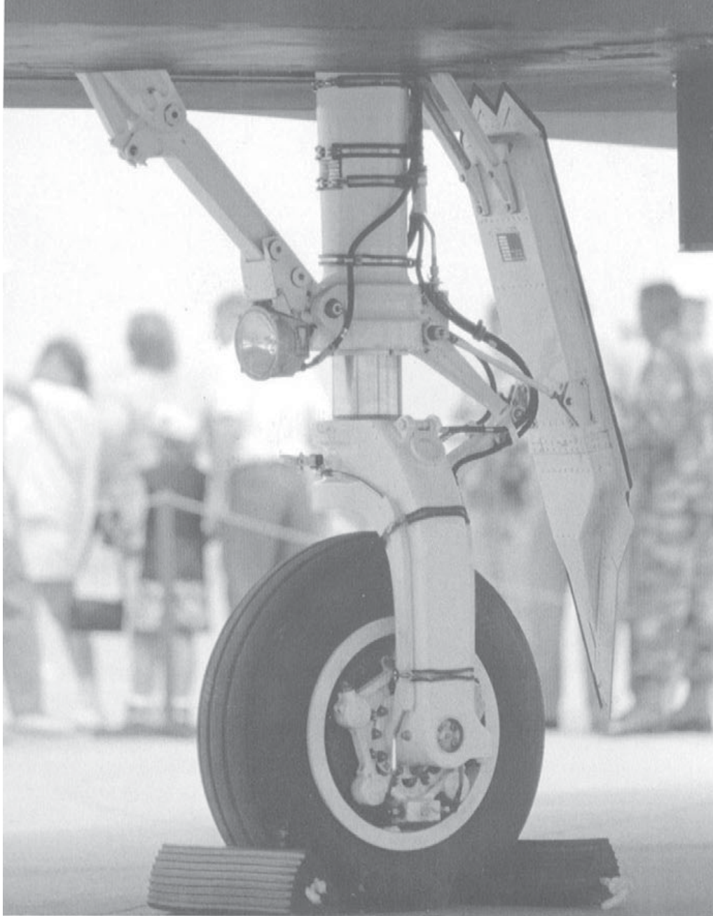
The production F-117A's main landing gear carry-through assembly is larger and shaped differently than on the YF-117As. The wheel axle from the main strut goes through the inboard wheel surface. Each main landing gear assembly is fitted with a landing light attached just above the oleo (shock absorbing) collar. The retraction strut pulled the main gear strut up and forward into the landing gear bay. A thin strut connected the gear door with the gear strut, while two hinges secured the door to the fuselage. (Jim Goodall)
