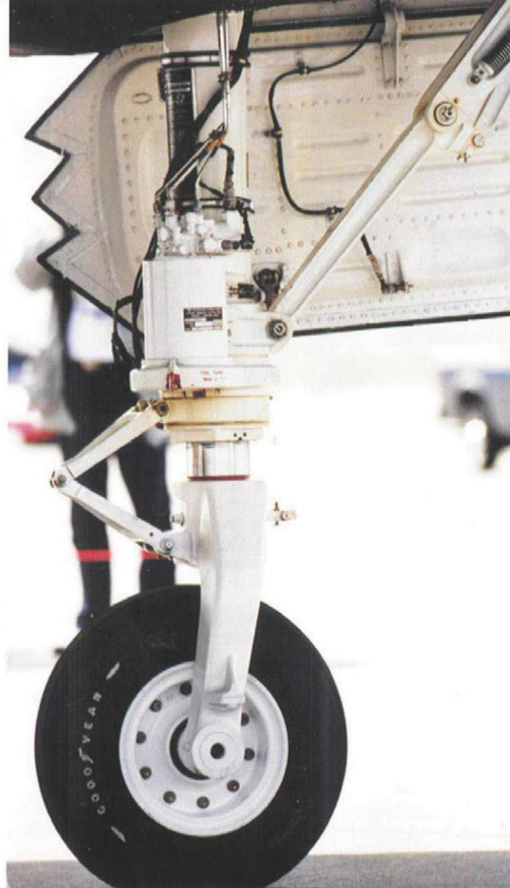
The nose landing gear was covered when retracted by a single gear door hinged to port. This door's saw-toothed edges reflected radar waves away from the aircraft. The retraction strut pulled the landing gear main strut up and into the gear bay. The Goodyear tire's brand mark was painted white for this airshow appearance; this mark is normally left in the natural tire color while the aircraft is in service. (Jim Goodall)
