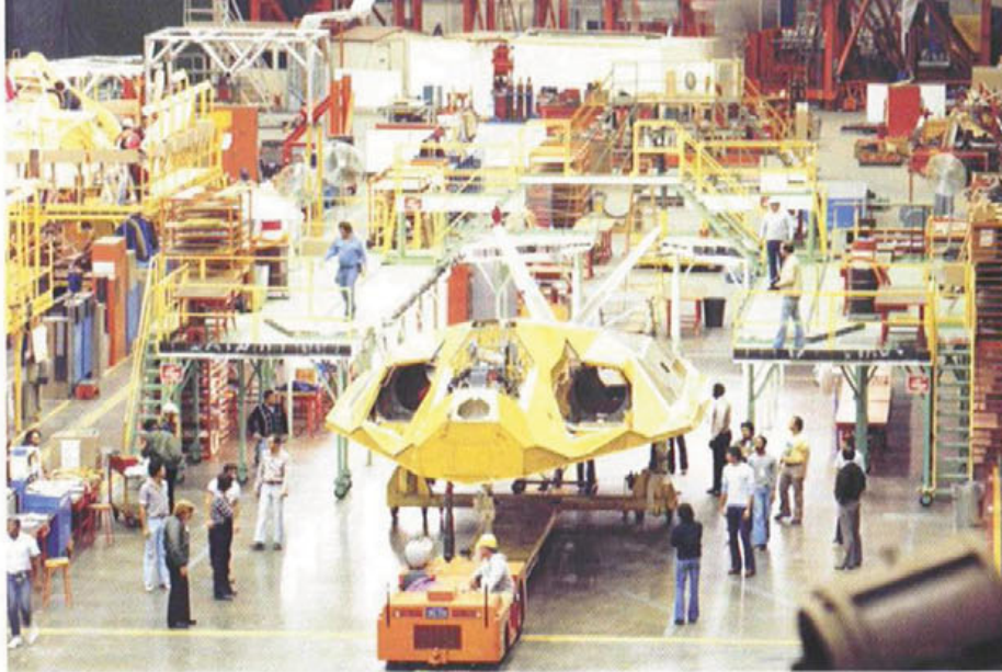
A tug moves the fuselage assembly of the first YF-117 (79-10780) down Lockheed's Burbank, California production line. This author was told that early on during the assembly of 780's fuselage, a tug bumped the assembly fixture. This seemingly insignificant contact moved the fixture and resulted in an asymmetrical aircraft. The problem was not discovered until the General Electric engines were being installed in both bays: one engine fit, but the other didn't. (Lockheed Martin)
