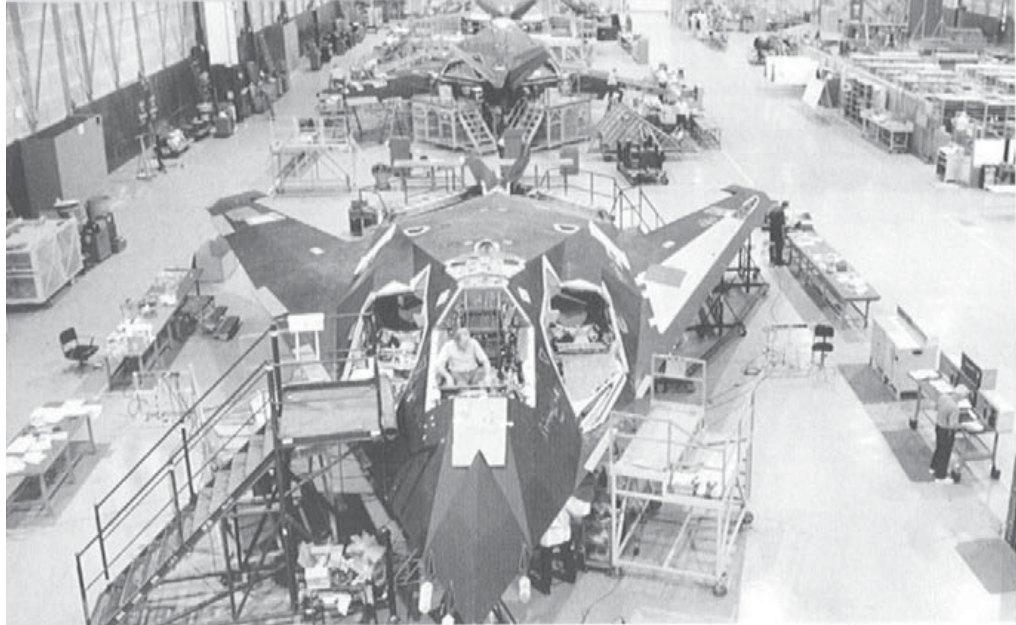
F-117A 810 (84-0810) undergoes depot level maintenance at Site 7 of Air Force Plant 42 in Palmdale, California. Site 7 – also called PS77 – is the Lockheed Martin/Air Force overhaul facility for the Nighthawk. Workers have removed the engine inlet assembly, the canopy, the ejection seat, and most of the cockpit from this Nighthawk. This step preceded the OCIP (Offensive Capability Improvement Program) Phase 3 upgrade of the cockpit and IRAD (Infra-Red Acquisition and Detection) system. (Lockheed Martin)
