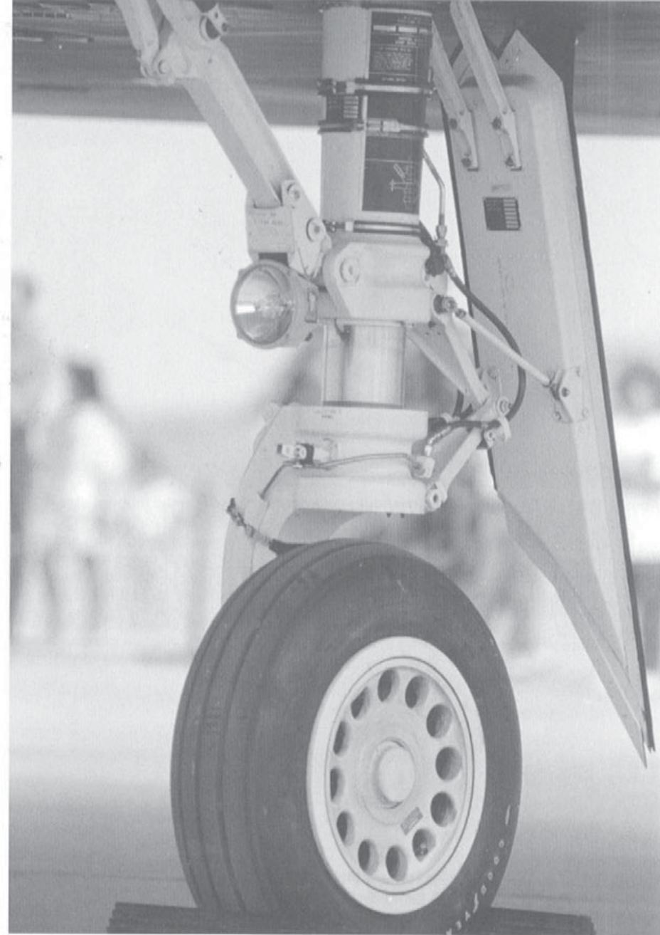
Early F-117As were equipped with Loral steel brakes and the wheels featured smaller openings than those associated with the F-15-type wheel and brake system retrofitted to the Nighthawks. A manufacturer's label placed around the upper strut assembly included maintenance instructions for ground crewmen servicing the landing gear assembly. The metal manufacturer's plate on the inside of the upper gear door area included the contract number, part number, and description. (Jim Goodall)
