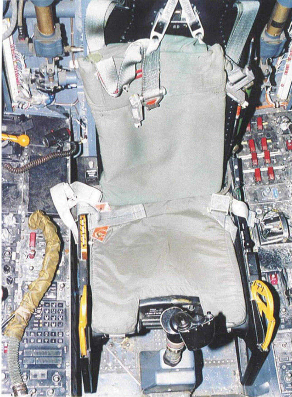
Aft of the instrument panel, the YF-117A's cockpit arrangement was virtually identical to that found on production F-117As. The pilot's oxygen hose – which connected with his face mask during flight – is draped long the starboard console. The oxygen hose was connected to a socket beside the seat. A 'Grimes light' – used for utility purposes by the pilot – is attached to a coiled handle at the aft end of the starboard console. (Jim Goodall)
