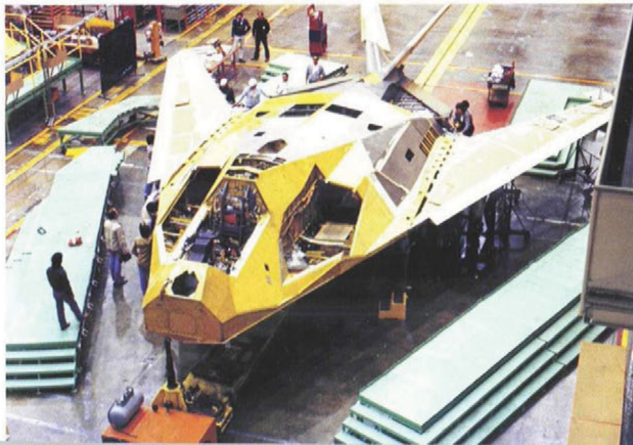
Lockheed technicians prepare to attach the wings to the fuselage and perform other tasks at this factory station. Light green work platforms beside the aircraft will be placed over the wings once the wings and fuselage have been mated. These platforms allowed workers to install the YF-117A's nose, control systems, and engines. (Lockheed Martin)
