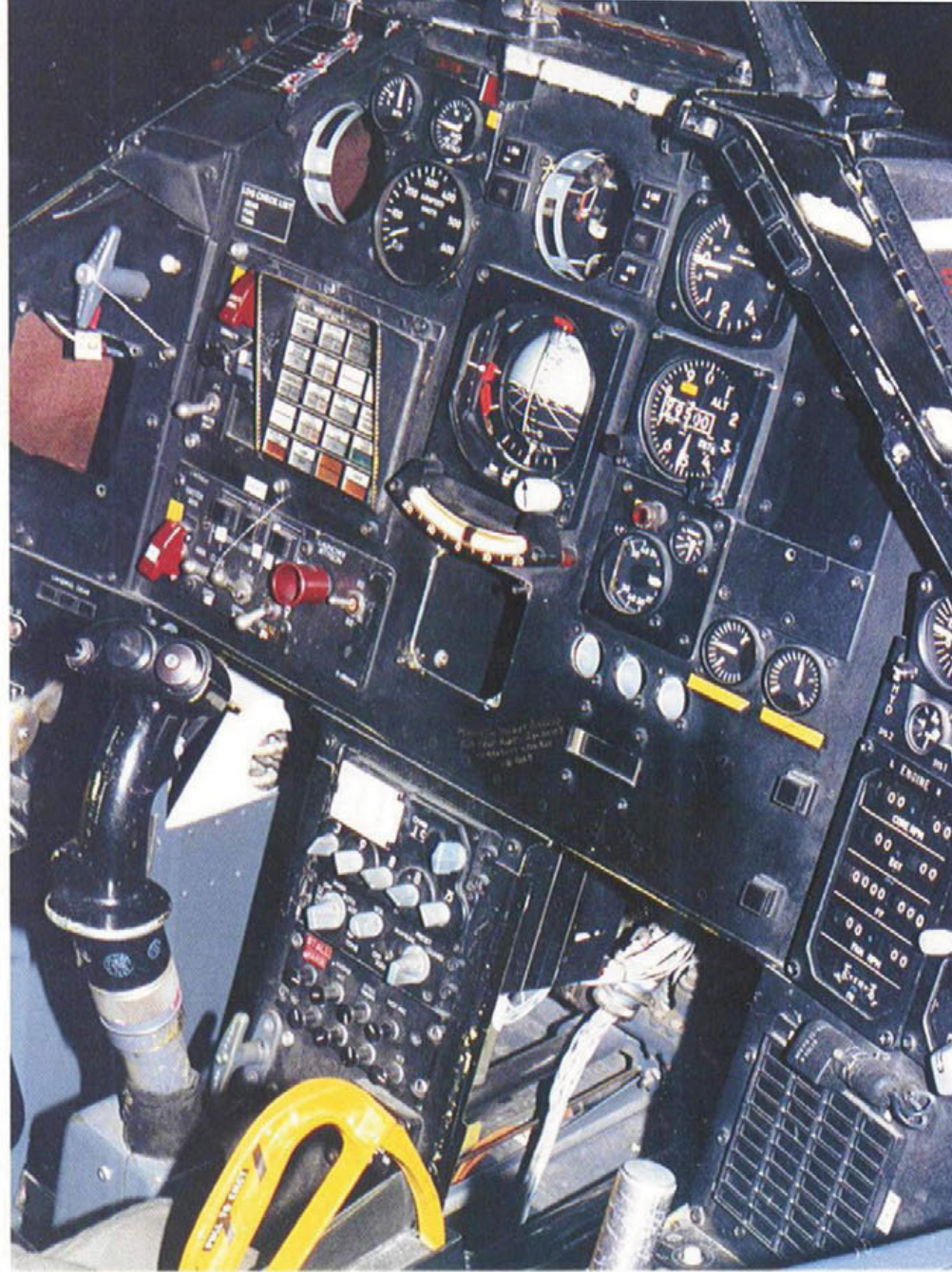
The starboard side of the YF-117A's instrument panel is the same as for operational F-117As, along with the control stick and the lower center instrument display immediately forward of the stick. Controls for the aircraft's radio and intercom systems were placed on the lower center display. The remainder of the YF-117A cockpit differed in composition from those found in the production Nighthawks. (Jim Goodall)
