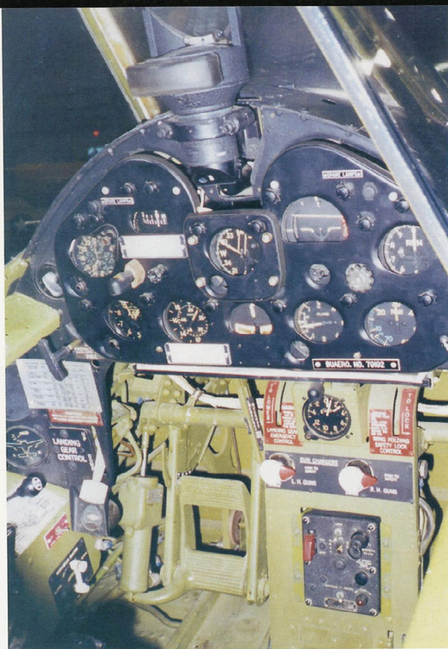
The instrument panel and rudder pedals on the New England Air Museum's F6F-5. The cockpit interior is painted in Interior Green with a Flat Black instrument panel. This F6F-5 is the most accurate restoration in the world today. The Black panel under the instrument panel is the rocket selector panel. (Larry Webster)
