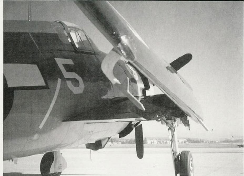
The pitot tube on the F6F was located under the starboard wingtip, near the wingtip position light. Like the earlier F4F Wildcat, the F6F had manually operated wing fold mechanisms. When delivered from the factory, the pitot tube was painted Red. (Author)
