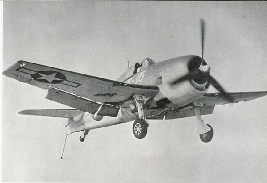
A late production F6F-3 in the landing configuration. The F6F-3 carried only one bomb rack, located on the starboard stub wing. The object hung on the bomb rack is a Mk 47 practice bomb dispenser. The oil cooler doors are in the open position. (Tailhook)
