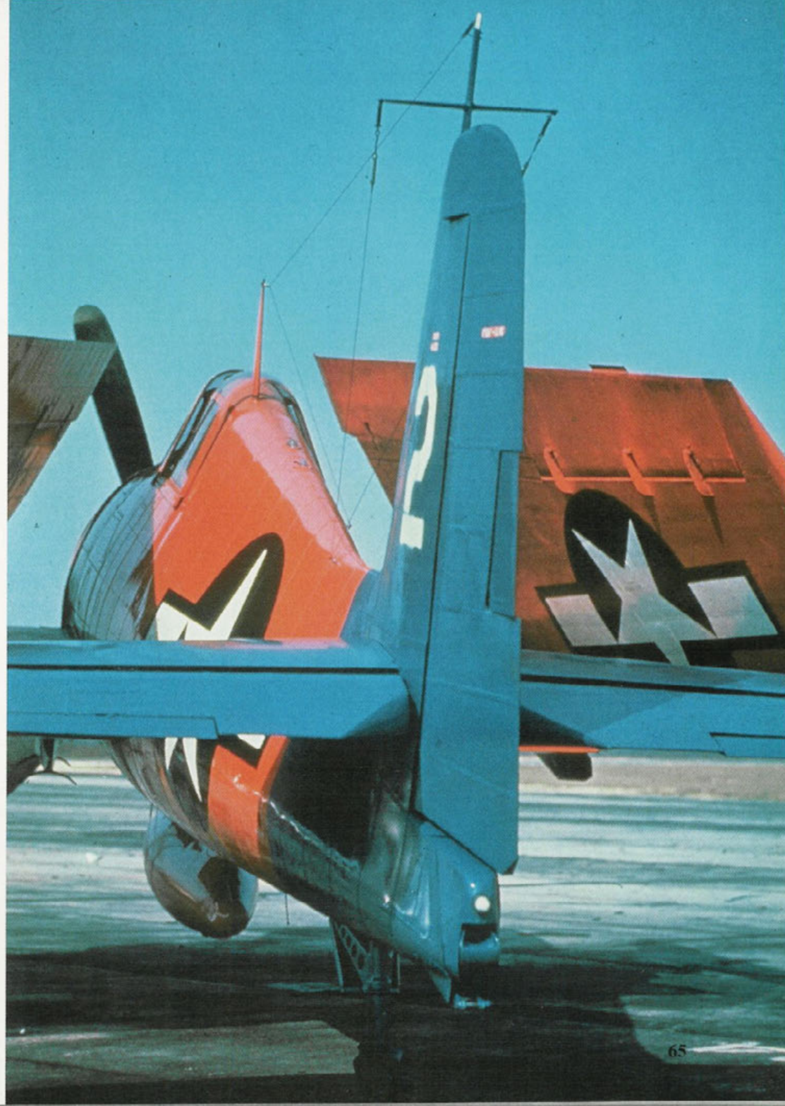
A line-up of F6F-3Ks with lengthened tail wheel struts. Because of this modification, the tail wheels were fixed in the down position. Tail colors denoted the assigned radio frequency of the drone. (Tailhook)
