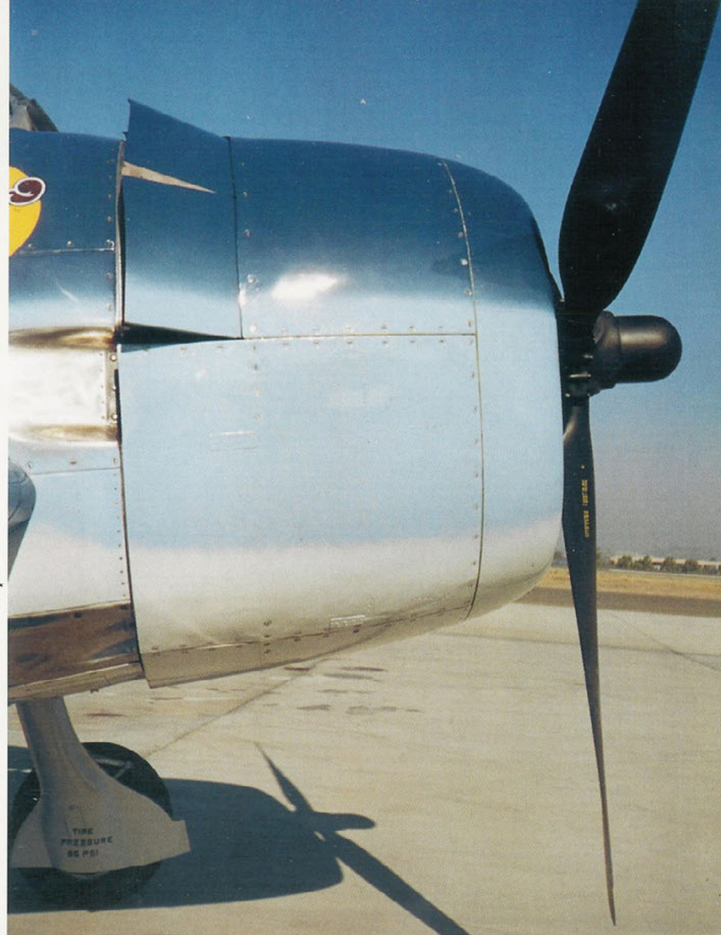
This late production F6F-3 (BuNo 41930) has two upper cowl flaps and no lower cowl flap. The engine was designed as a Quick Engine Change (QEC) unit, which was received from the factory complete with mount, oil tank, cowling, exhaust and ignition systems in place for quick installations. (Author)
