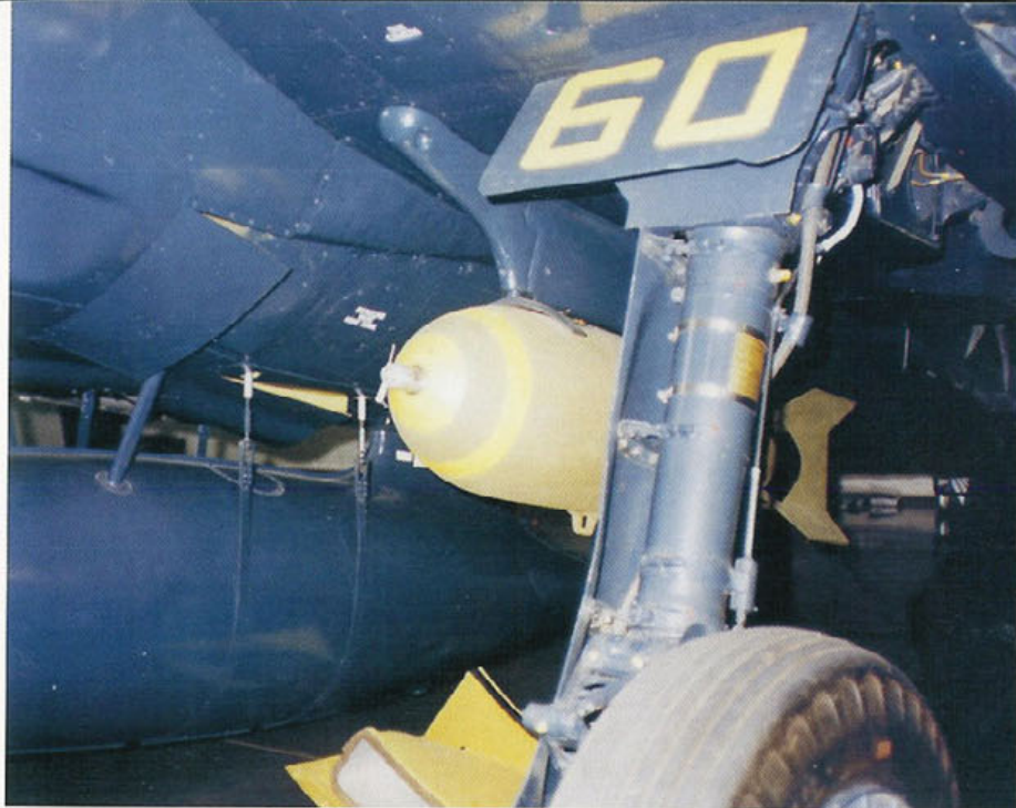
A 500 pound general purpose bomb (complete with nose fuse) hung on the bomb rack of a F6F-5. There is a small access panel forward of the bomb rack for access to the gun camera. (Larry Webster)
