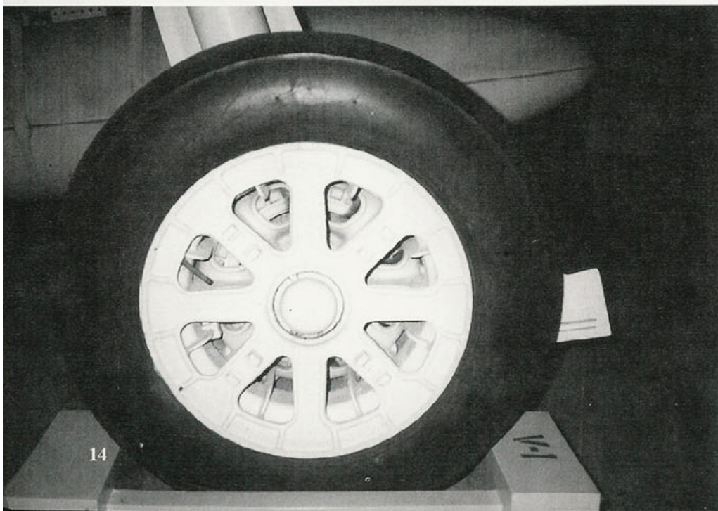
The tailwheel of the San Diego Aerospace Museum F6F-3 (BuNo 42874). Hellcats were equipped with a full-swivel hard rubber tailwheel that was ten and a half inches in diameter and four inches wide. There are at least three surviving F6F-3s, one at the National Museum of Naval Aviation, one at San Diego and a flyable example at Palomar Airport in Carlsbad, California. (Author)
