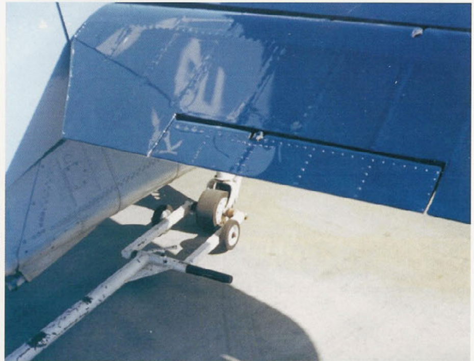
The vertical fin and rudder of F6F-3 BuNo 41930. Construction techniques for the Hellcat were similar to those used on the Wildcat. There were over 12,000 Hellcats built in just three years. Also visible is the elevator trim tab. Service F6F-3s were painted in non-specular (flat) colors. (Author)
