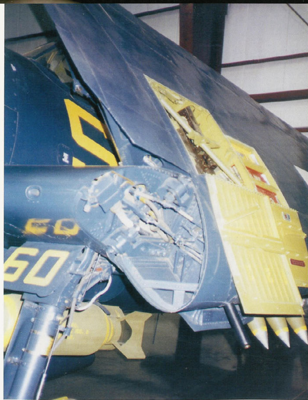
The Hellcat's primary armament consisted of guns, bombs and rockets. This Hellcat is armed with six .50 caliber machine guns, a 500 pound bomb and six 5 inch HVAR rockets. (Larry Webster)
