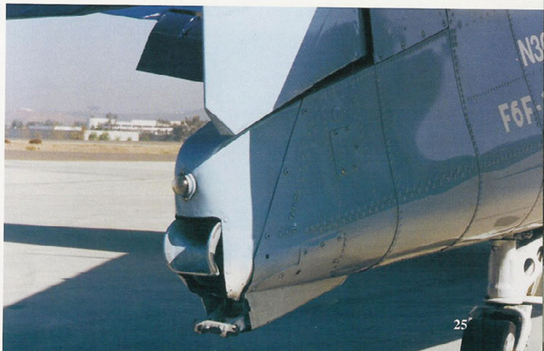
The extreme tail of the Hellcat housed the fully retractable arresting hook. The hook retracted into a space in the fuselage under the rudder. Just above the hook was a White position light. There is also a tie down/holdback fitting below the tail hook. (Author)
