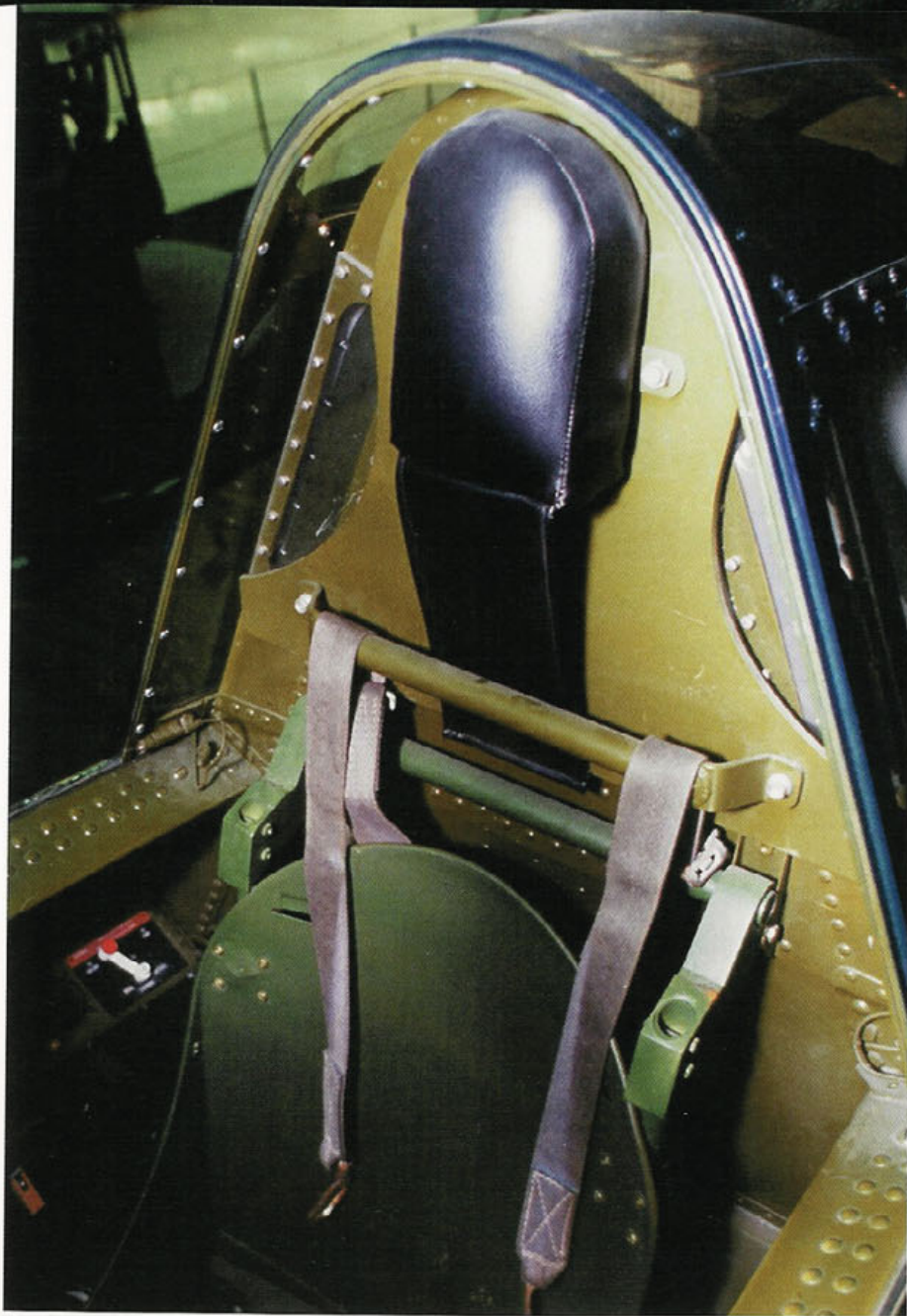
The headrest and back armor plate on Pensacola's F6F-3 Hellcat. The headrest has a leather extension that snaps to the armor plate just behind the seat. It is obvious that the Hellcat had poor rearward vision, even with the small windows on the F6F-3. These windows were deleted on the later F6F-5. (Lieutenant Ken Acosta)
