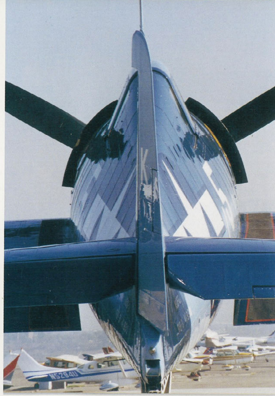
F6F-3 (BuNo 41930) has the engine cowl flaps in the full open position. The technique of building airframes from flat aluminum sheets on the fuselage sped up production of the Hellcat tremendously and made for an extremely strong structure. In just over three years, 12,275 F6Fs were produced. (Author)
