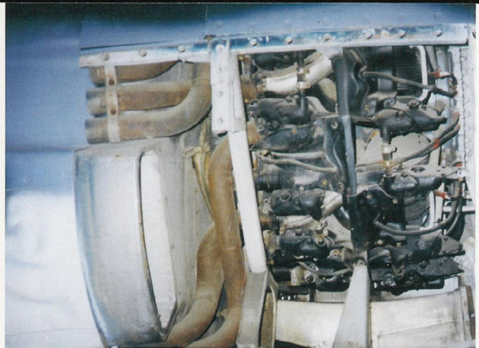
There are three exhaust stacks exiting on the upper side of the engine and two lower on the fuselage. The cowling was held in place by Dzus fasteners. Below the engine cylinders is the duct that supplies cooling air to the oil cooler and air to the auxiliary stage supercharger. (Author)
