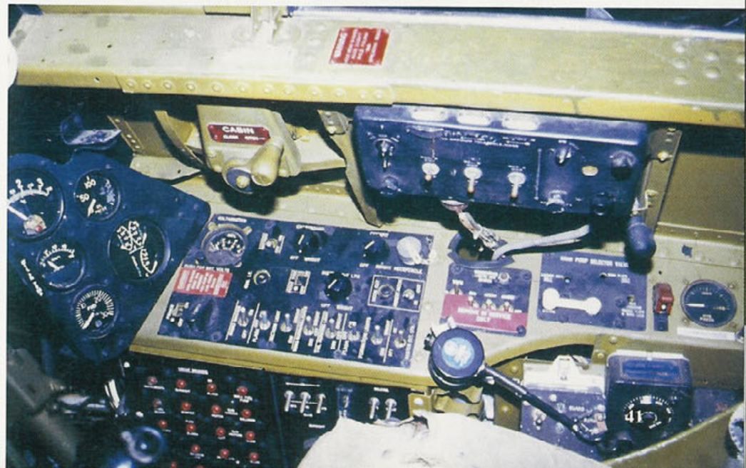
The right console of the F6F-5 is taken up with electrical and communications panels. This F6F has original IFF (Identification Friend or Foe) equipment. The round device near the center of the panel is the pilot's hand held microphone. (Larry Webster)
