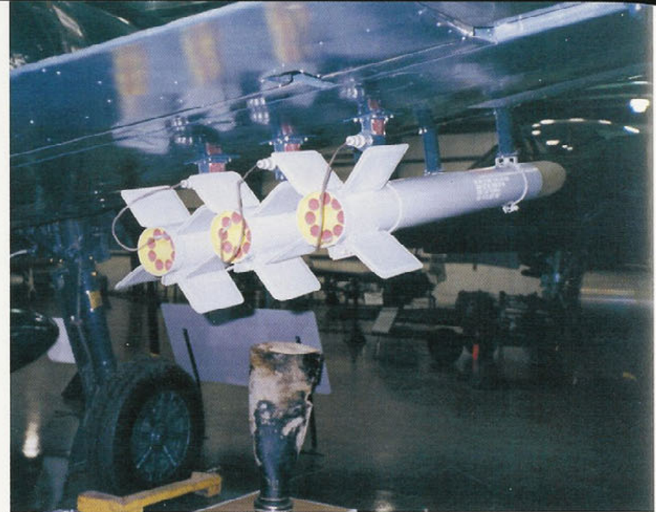
The Hellcat had provisions to carry the unguided 5 inch High Velocity Aircraft Rocket (HVAR). The rockets were first installed on the 3,451st F6F-3 (BuNo 42185) and all later production aircraft. There are metal blast covers on the flaps. (Larry Webster)
