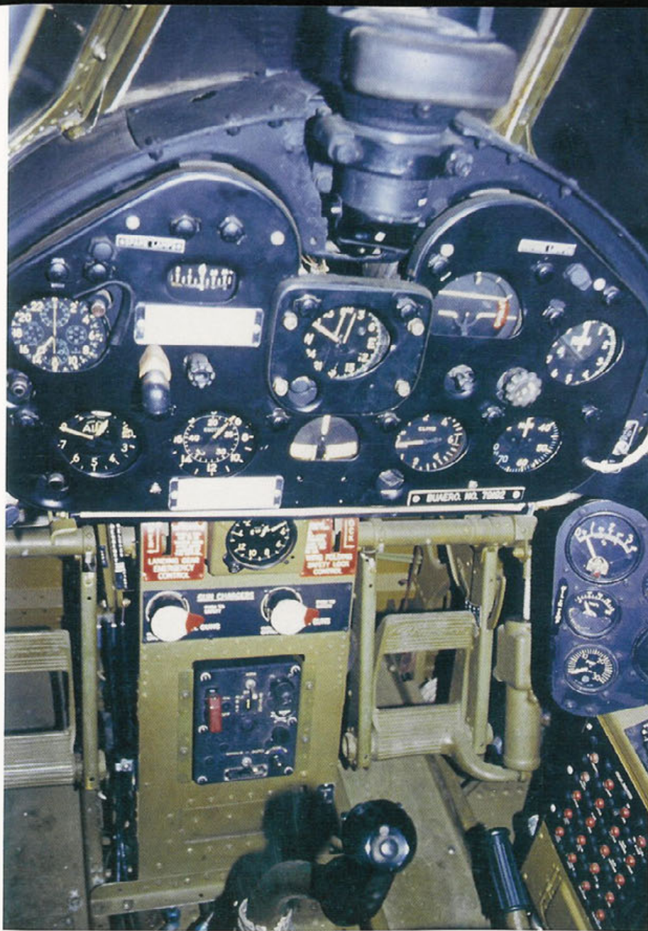
The New England Air Museum's F6F-5 is not intended to fly again and has been restored to stock condition, without the need for modern avionics. The instrument panel of the F6F-5 featured a night illumination system that would illuminate the instruments in Red. The gunsight is a Mk VIII type. (Larry Webster)
