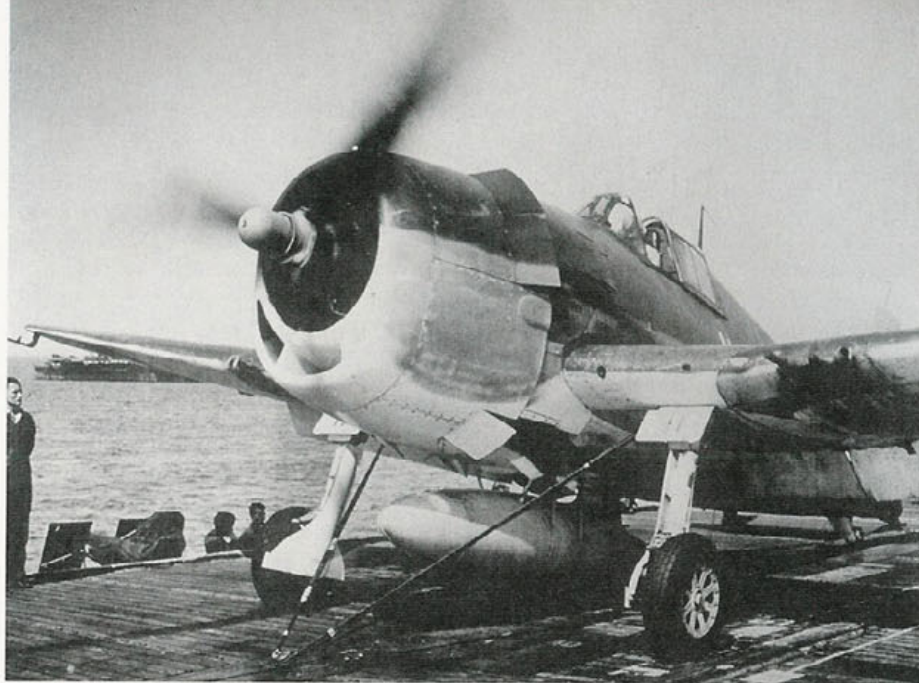
This F6F-3 of VF-11 illustrates the primary identification features of the F6F-3 including the early style windshield, lower cowl flaps (BuNos 04775-04958, 08798-09047 and 25721-26195). The small exhaust fairing was also found on these aircraft as well as BuNos 39999-40235, after which it was deleted. (Tailhook)
