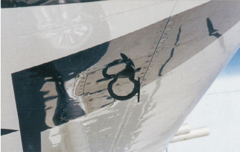
The Hellcat had a retractable tie down hook under each wing. When not in use, the hook retracted up into the wing. The hook was released manually by a push on the fastener. (Author)
