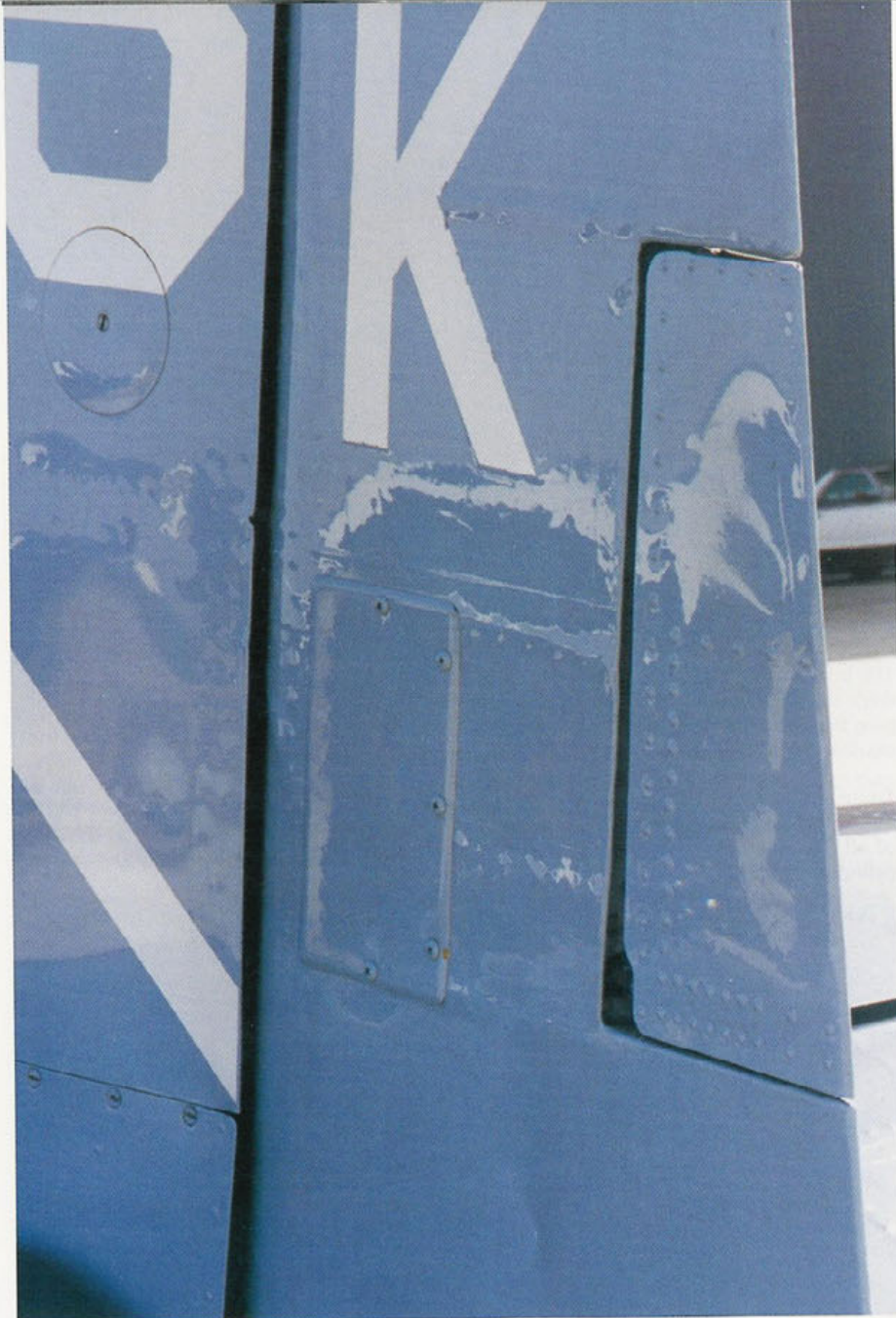
The rudder trim tab was controlled via a trim wheel in the cockpit. The rectangular plate in front of the trim tab was the trim tab inspection plate. The circular rudder hinge inspection plate was located just under the White 5 on the fin. (Author)
