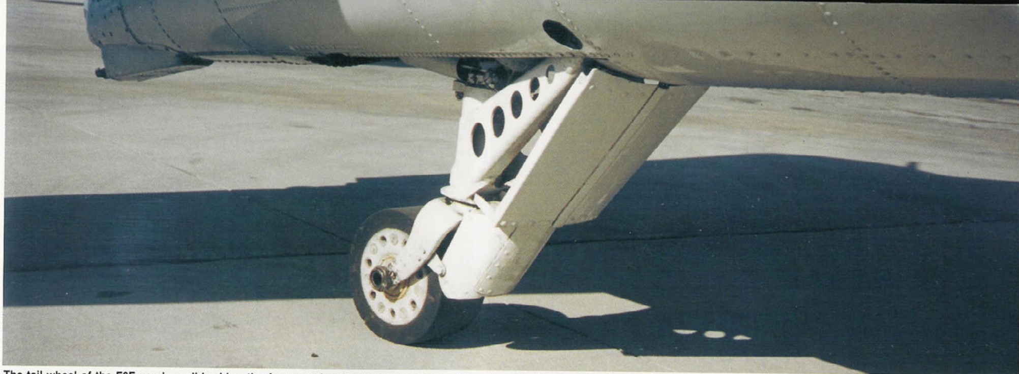
The tail wheel of the F6F used a solid rubber tire for operations from carrier decks. When the aircraft was shore based, the solid tire was replaced with a pneumatic tire. The tail wheel was fully swiveling and could be locked in position for takeoff and landings. The wheel was raised and lowered hydraulically. (Author)
