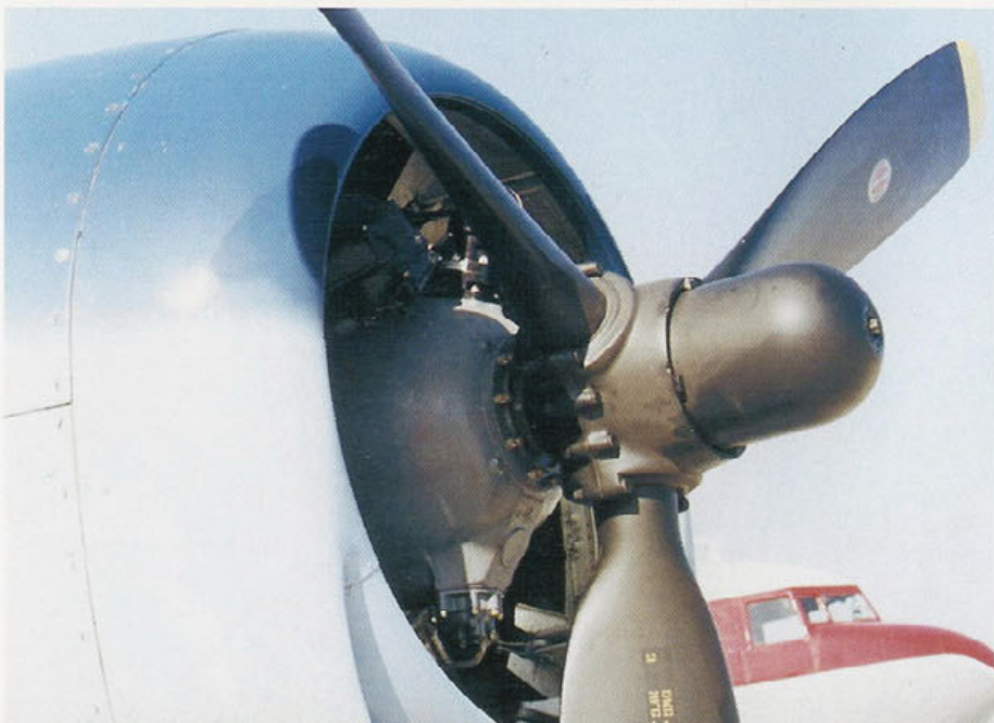
This late production F6F-3 (BuNo 41930) has two upper cowl flaps and no lower cowl flap. The engine was designed as a Quick Engine Change (QEC) unit, which was received from the factory complete with mount, oil tank, cowling, exhaust and ignition systems in place for quick installations. (Author)
