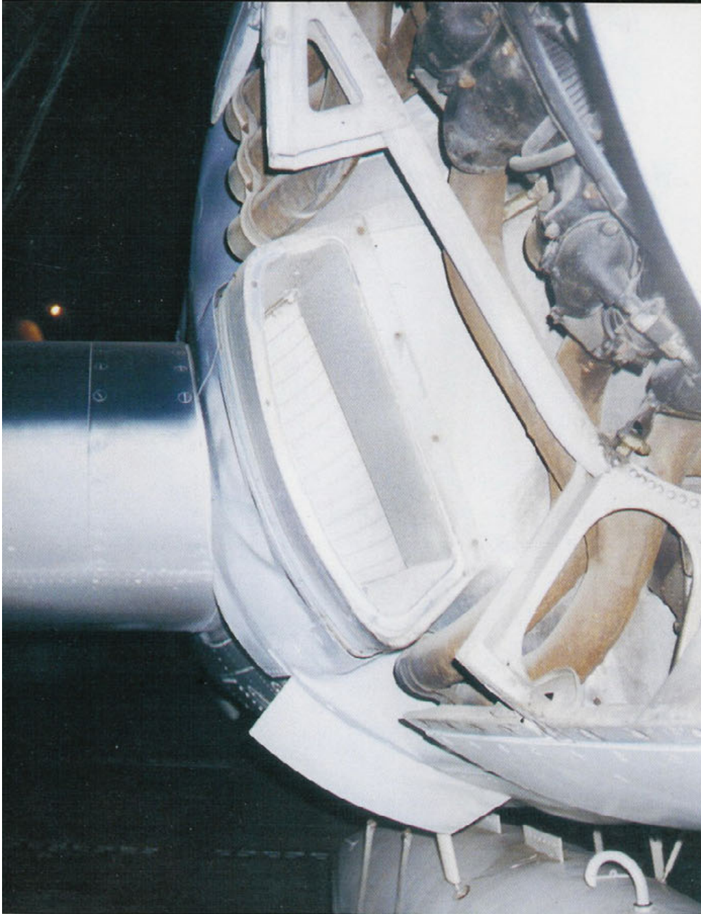
The lower starboard cowling panels have been removed to reveal the intercooler ducting. The intercooler cooled the superheated compressed air coming from the supercharger prior to entry into the carburetor. This reduced the chance of detonation and preignition. Also visible are the sway braces and banding straps that held the external Mk XII fuel tank in place. (Author)
