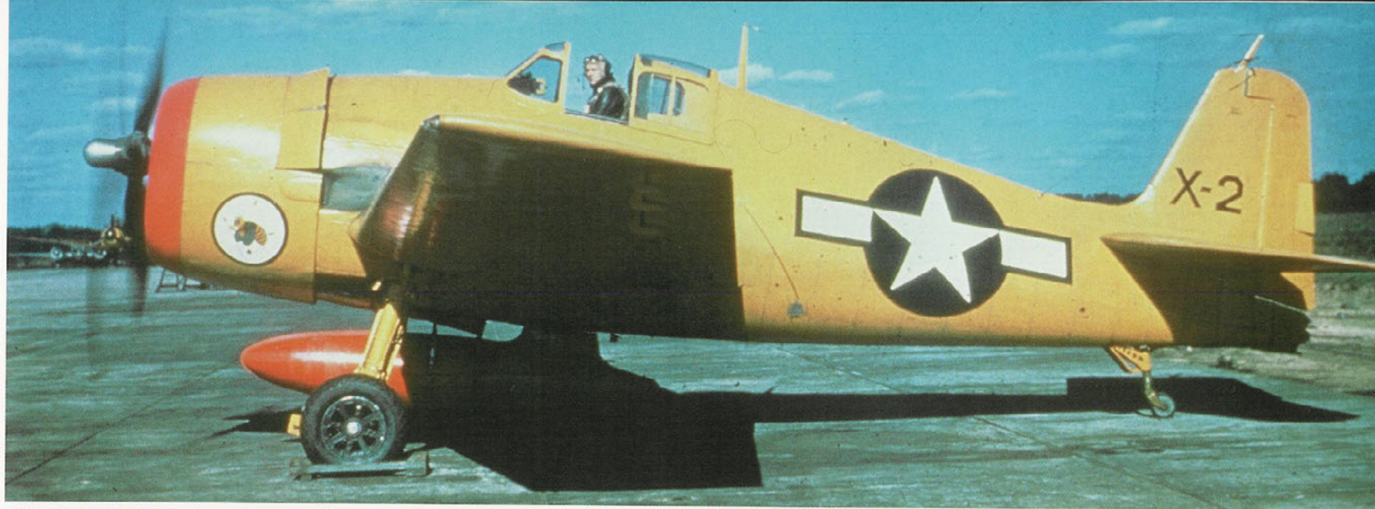
This colorful F6F-3 Hellcat was used as a drone controller aircraft at Naval Air Station Johnsville, Pennsylvania. Controller aircraft would fly formation with the drones, using electronic remote control to fly them. The controller aircraft were always given a highly visible color scheme. (Tailhook)
