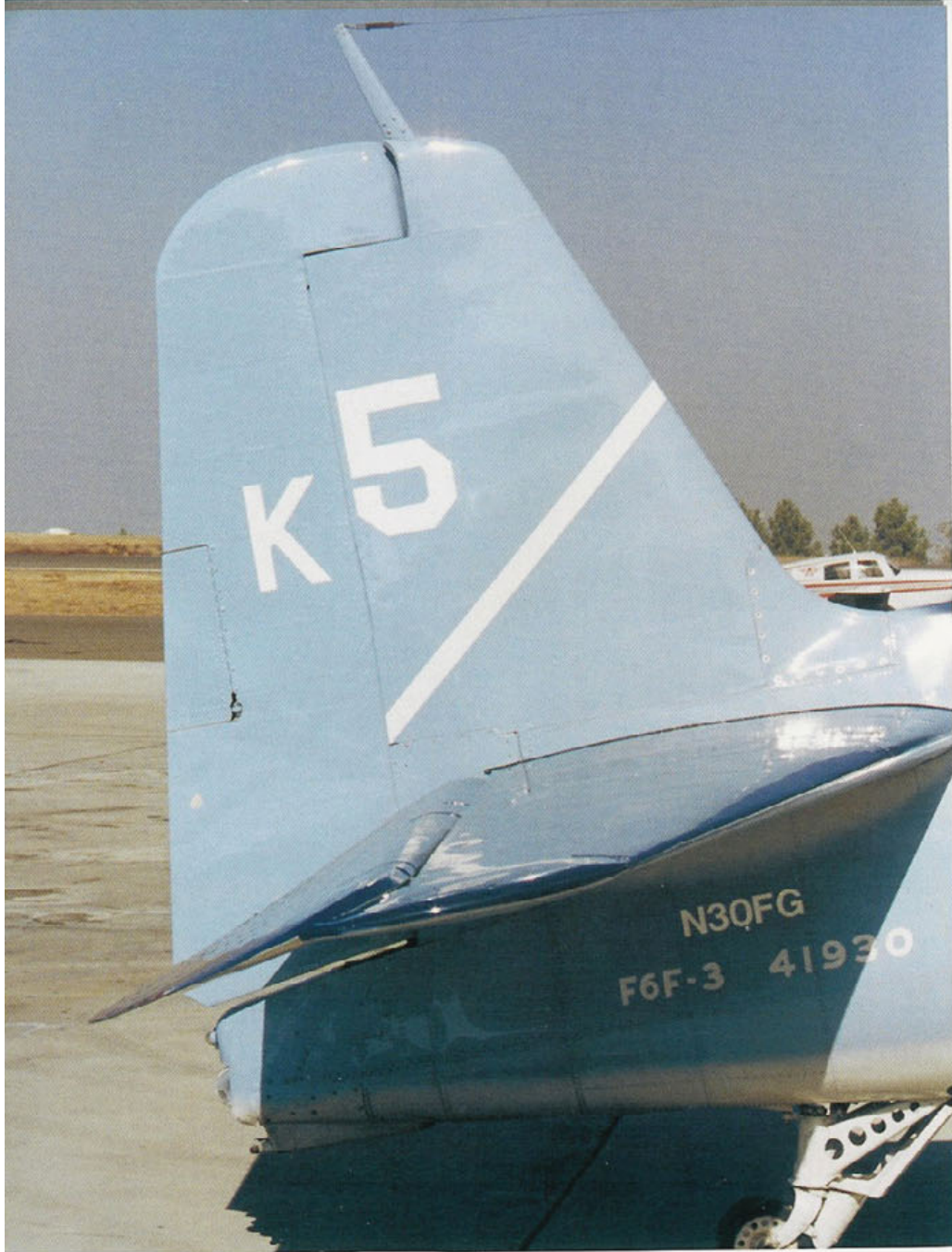
The rudder of a F6F-3 (BuNo 41930). The internally balanced rudder was a metal structure covered with fabric. The rudder trim tab was fully controllable via a trim wheel in the cockpit. The antenna post on the fin had a single wire that ran from this post to the antenna post mounted on the fuselage spine behind the cockpit. (Author)
