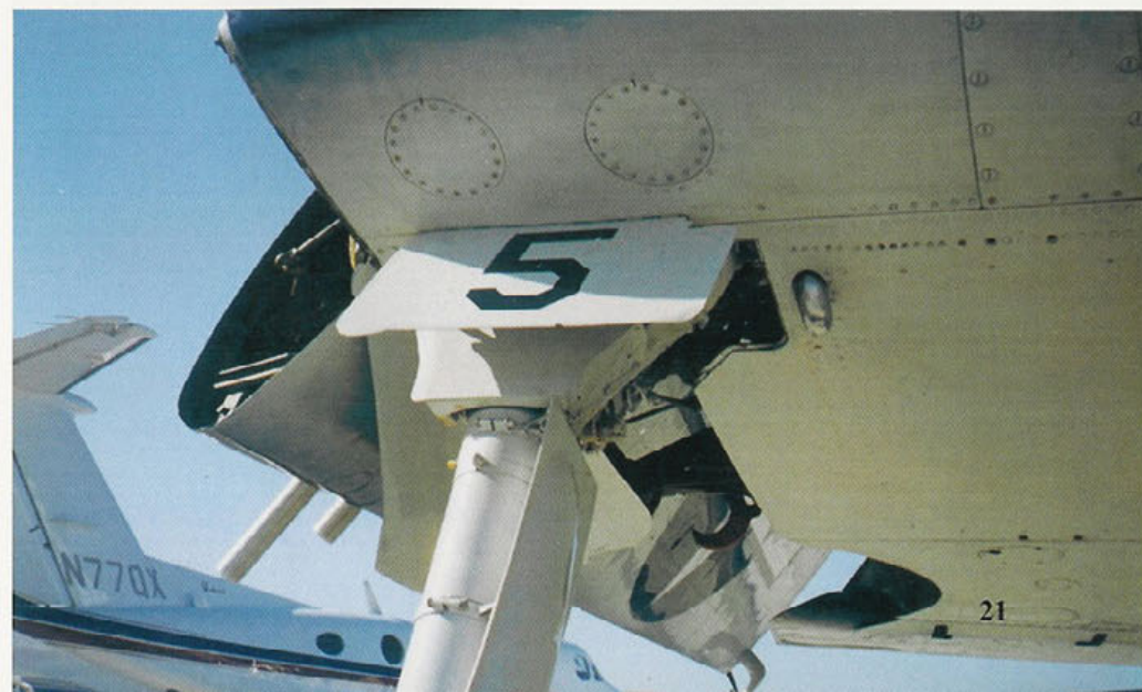
The landing gear was anchored to the main spar in the stub wing. With the wing in the folded position, the well was open on the outboard side. The small hook next to the landing gear is the catapult bridle hookup/jackpoint. (Author)
