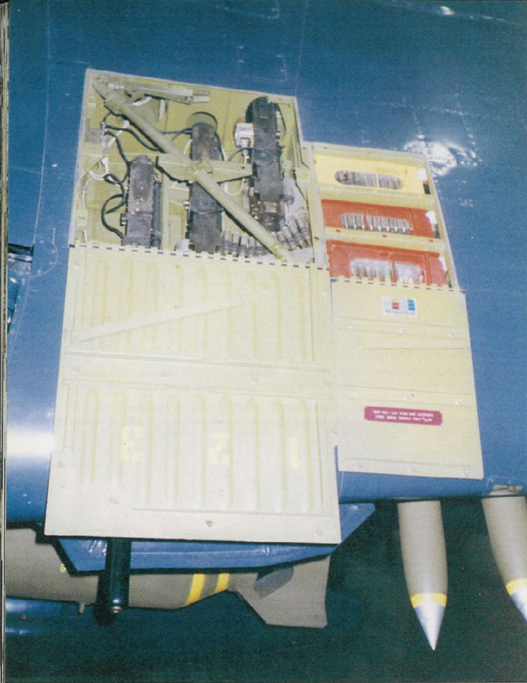
The New England Air Museum's F6F-5 was restored complete with gun bays and ammunition. Ammunition boxes were color coded according to size. The gun bay doors also acted as servicing platforms. This particular aircraft is equipped with the standard gun armament of six .50 caliber machine guns. (Larry Webster)
