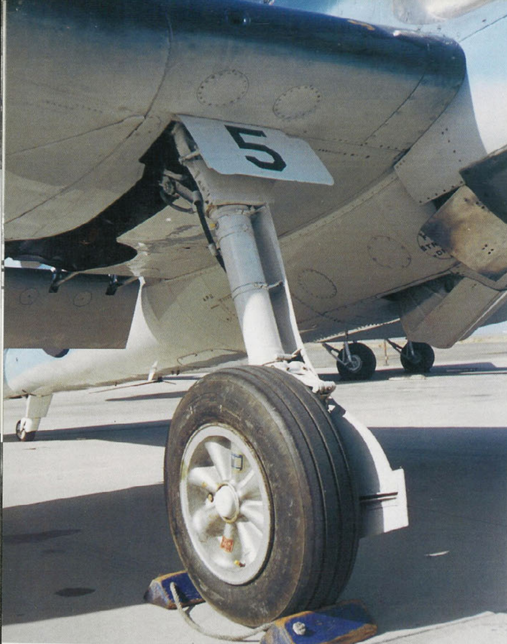
The main landing gear wheels are single piece aluminum castings. The wheel brake flex line is visible behind the top portion of the landing gear strut. The landing gear door was three parts; one fixed to the landing gear strut, a smaller strut mounted door and a smaller section attached to the wing. These are late F6F-5 wheels, which were also used on B-52 outriggers. (Author)
