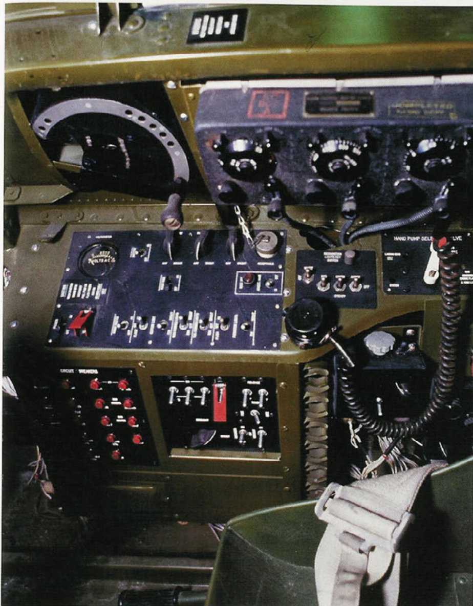
The electrical distribution panel was located on the right side of the cockpit. The row of clips that run vertically next to the seat are for pyrotechnic storage. The hydraulic hand pump is visible under the seat. The canopy crank handle is located at the upper left. (Lieutenant Ken Acosta)
