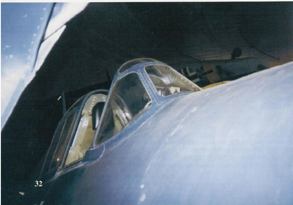
The windshield of a F6F-3 had a reinforcement brace running from the windscreen back to the rear frame. This restored F6F-3 is missing the armor glass normally mounted just behind the windshield. (Author)
