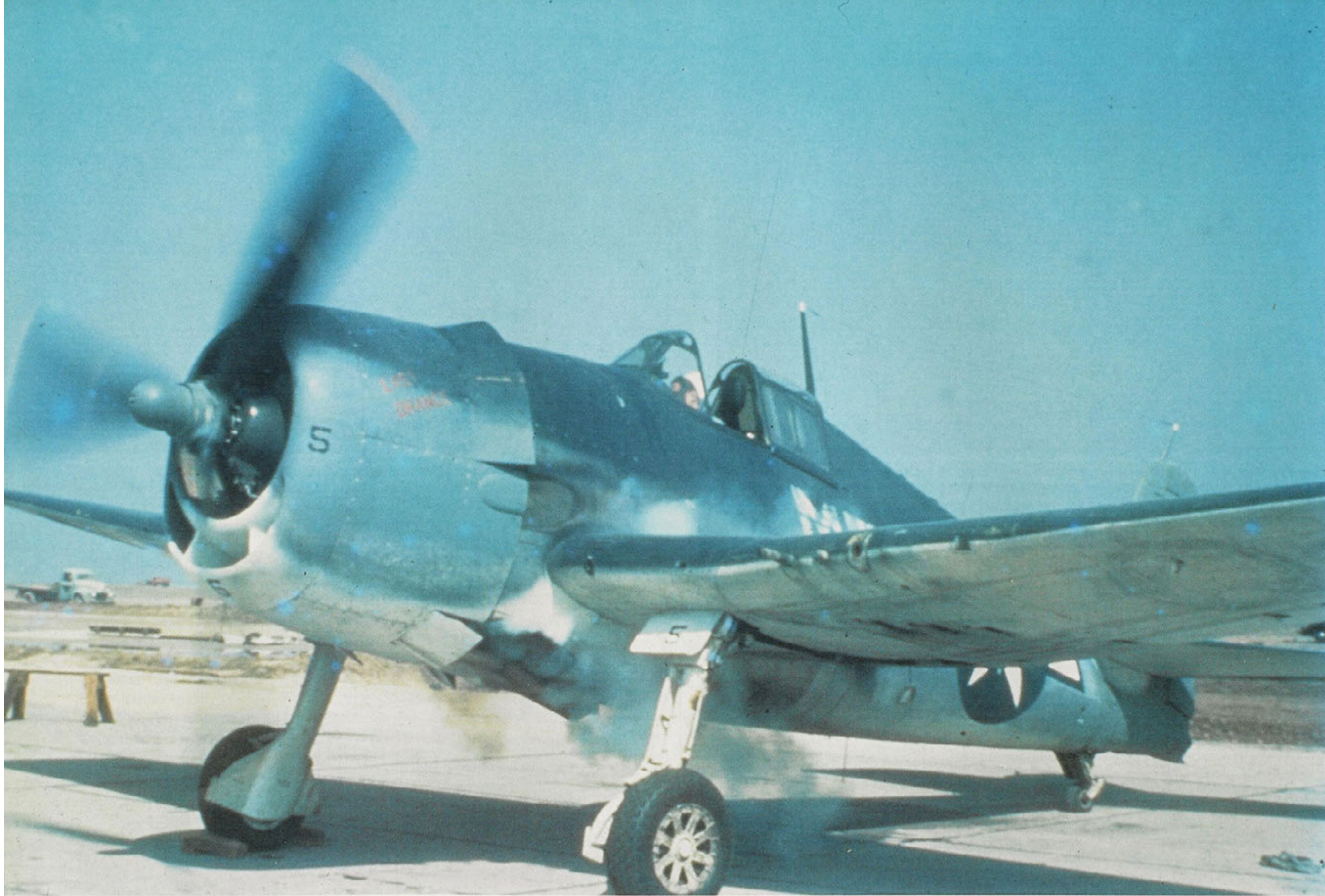
Belching smoke from its exhausts, an early production F6F-3 starts its Pratt & Whitney engine. The cowl flaps, intercooler doors, and oil cooler are all in the open position. It appears that this Hellcat was previously painted with the national insignia in six positions and has the port underwing position painted out. 4,403 F6F-3s were built from September of 1942 until April of 1944, at which time production shifted to the improved F6F-5 Hellcat. The aircraft number was painted in three positions on the cowling and on the upper landing gear doors. (Tailhook)
