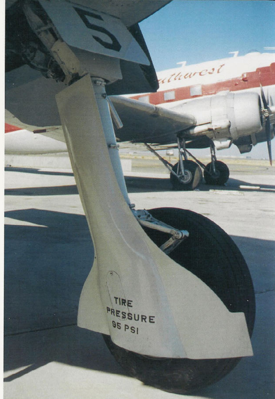
The port main landing gear and gear doors. In the center of the lower main gear door is an oval inspection and strut servicing panel. The V shaped objects visible behind the wheel are the torque links. This aircraft has the recommended tire pressure stenciled on the gear door to aid in servicing the aircraft. (Author)
