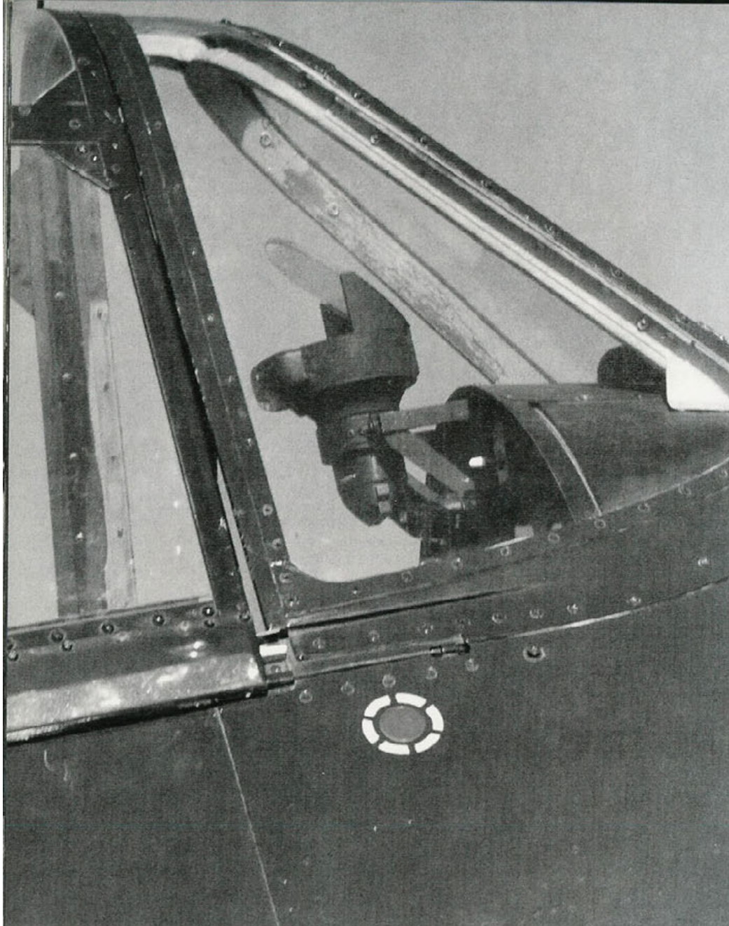
The windshield and gunsight of F6F-3 BuNo 41930. This aircraft has been modified with the later style windshield used on the F6F-3N, F6F-5 and F6F-5N. The aircraft is fitted with a Mk VIII gun sight (fully operational). The Red button on the side of the fuselage is the exterior canopy release. Service aircraft did not have this painted Red. (Author)
