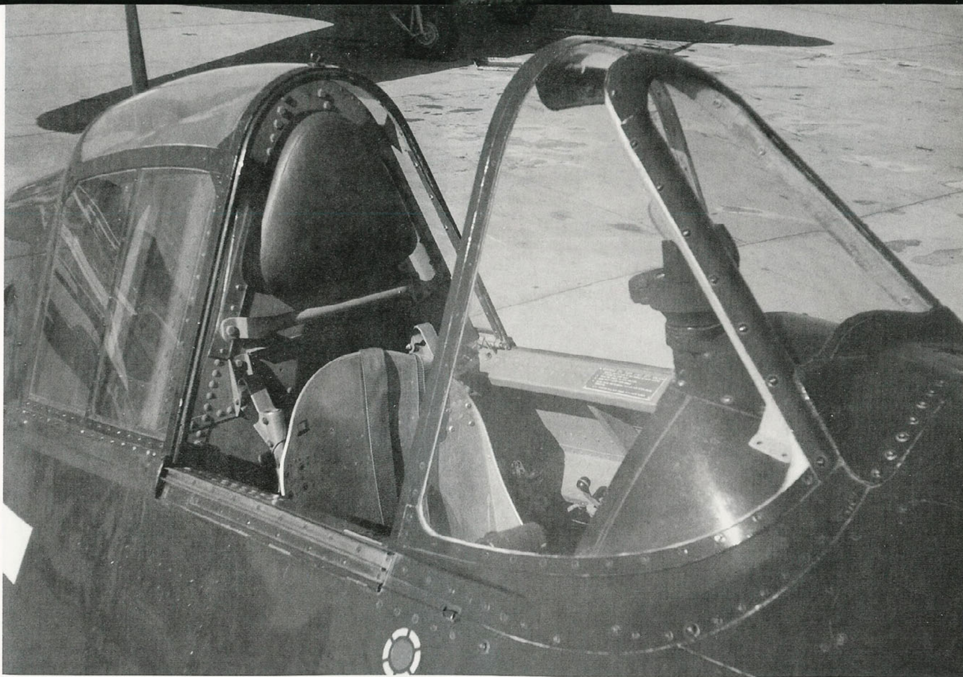
The canopy in the fully open position. The upper portion of the canopy was bulged upward to give the pilot more head room and was unframed for excellent upward view. The upper framing on the windscreen of the F6F-3 was deleted greatly improving forward view. The headrest in this Hellcat is made of Black leather and is attached directly to the rear bulkhead. (Author)
