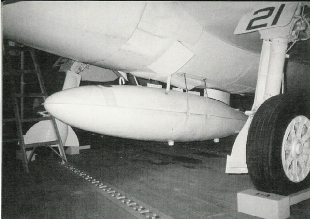
This is a late war modified Mk 12 under fuselage 150 gallon drop tank. This tank has the seam running horizontal and a straight pylon. (Larry Webster)
