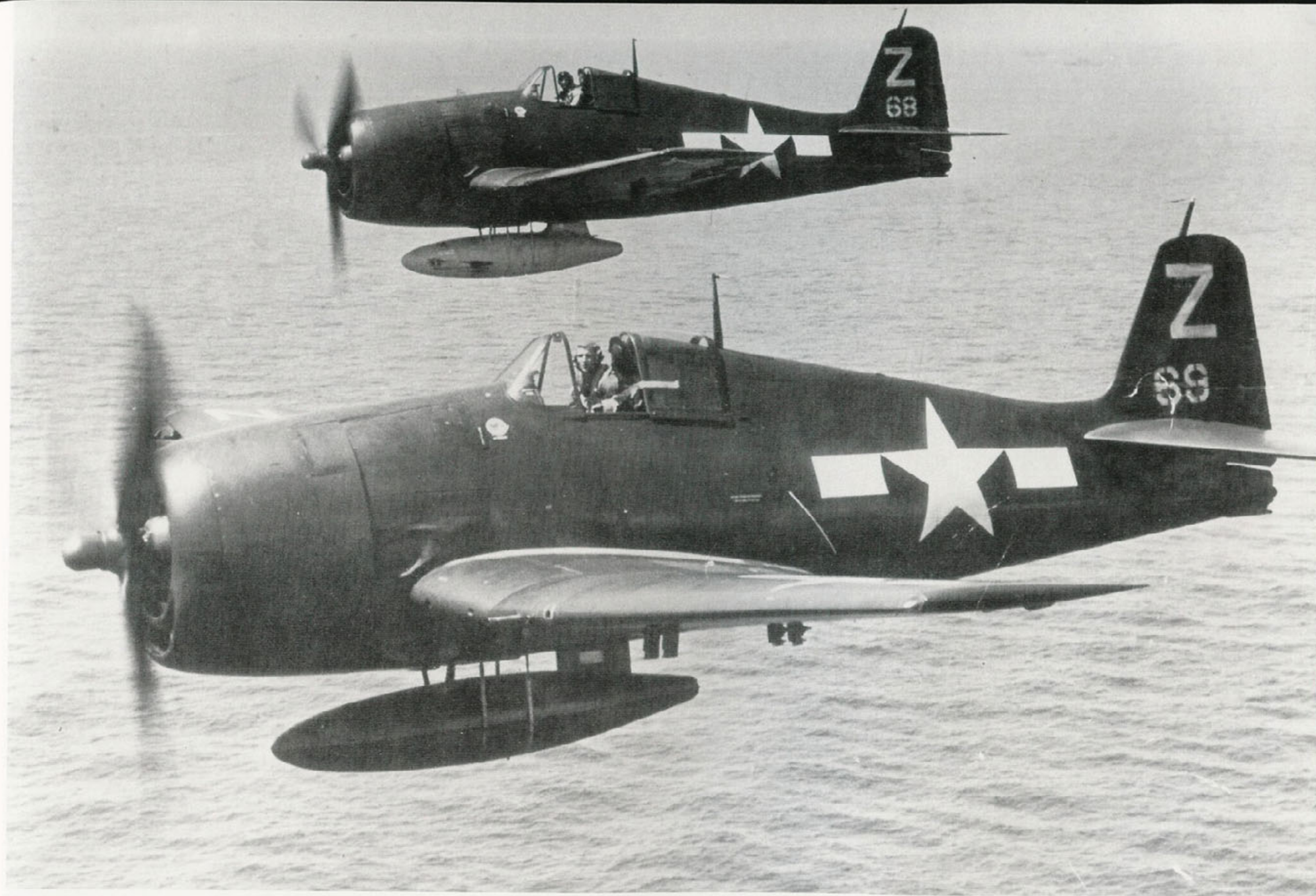
The Hellcat carried a number of different style drop tanks on the fuselage underside, although each was the same capacity, 150 gallons. Both of these Hellcats are carrying different tanks. The aircraft in the background has a White early style 150 gallon tank with a curved mounting pylon and vertical seams. The Hellcat in the foreground carries the late war style 150 gallon tank with a straight mounting pylon and horizontal seam. Both aircraft use stabilizing bands and sway braces to keep the tanks in place. (Richard Hargis)
