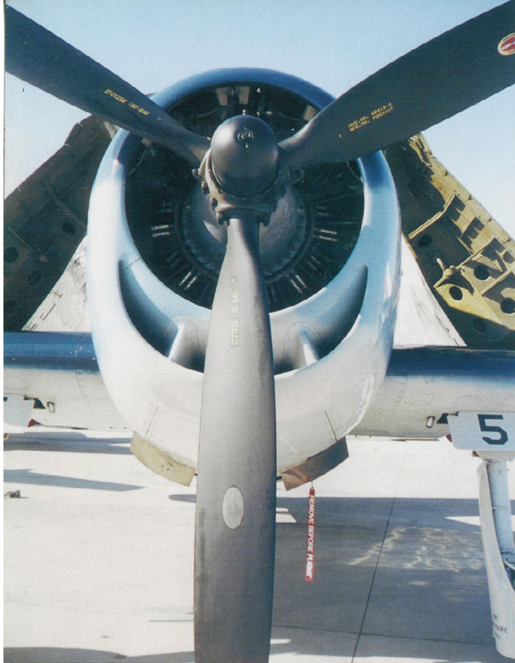
The power plant on the F6F-3 was the Pratt & Whitney R-2800-10 radial, which had a two stage, two speed supercharger and developed over 2,000 hp. The outer intakes fed the superchargers and the two supercharger intercooler doors are in the open position. The center intake fed the oil cooler. (Author)
