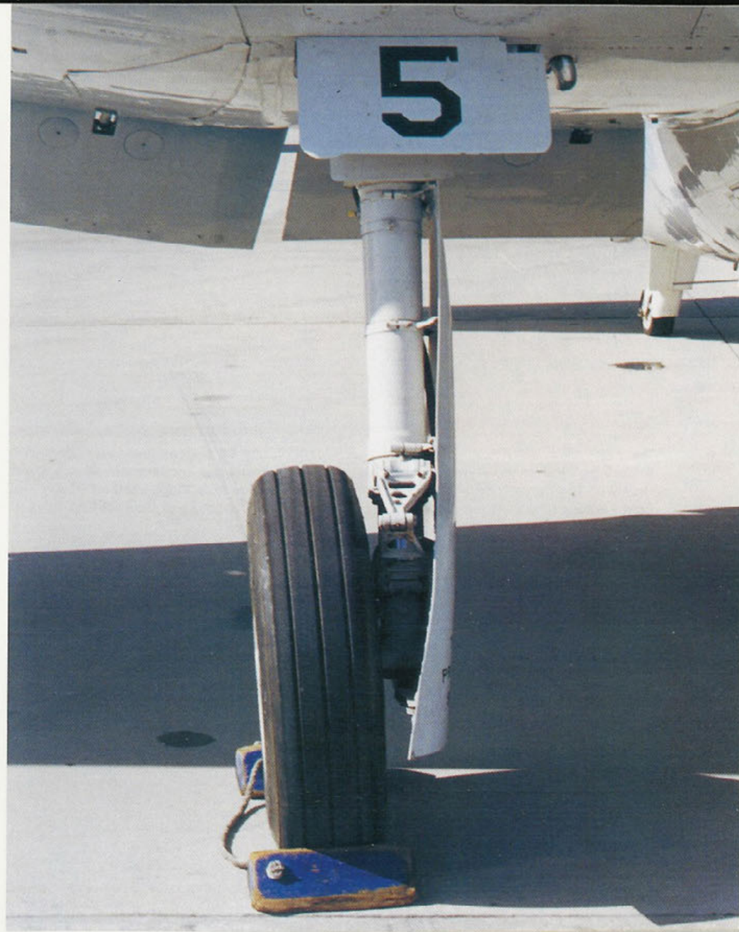
The F6F-3 uses thirty-two by eight inch Goodyear tires and multiple disk brakes. The brakes had an independent hydraulic system with a master cylinder attached to each rudder pedal. Braking action was started by pressing down on the top of the rudder pedals. Tire inflation pressure differed, depending on aircraft gross weight and whether the aircraft was shore based or carrier based. (Author)
