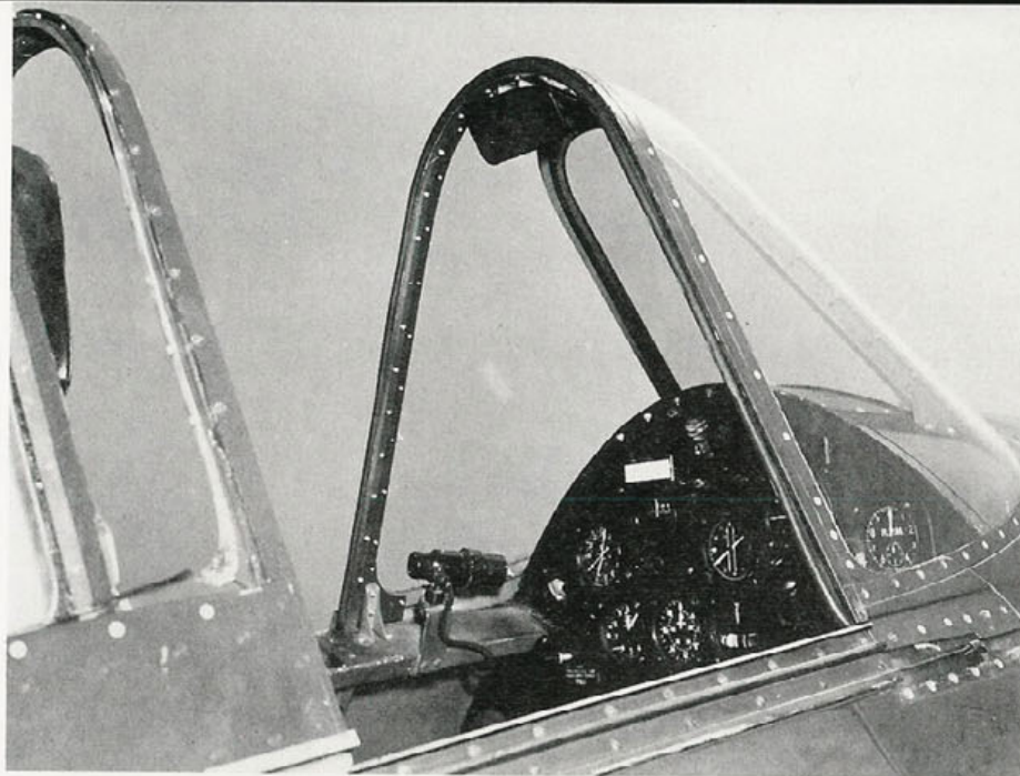
The primary identification feature of the F6F-5 from the F6F-3 was the windshield and canopy. The windshield was made of flat armor glass and had the upper brace deleted. (Grumman)
