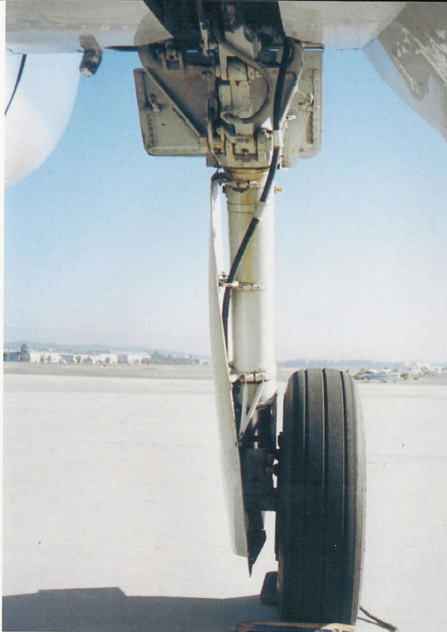
The landing gear on the F6F-3 was hydraulically operated from an engine driven hydraulic pump and rotated ninety degrees to lay flat within the wing. The landing gear control handle was located on the left side of the instrument panel. In case the hydraulic pump fails, the gear can be lowered by a hydraulic hand pump located on the right side of the seat. In the event of an total hydraulic failure the gear can be lowered by a nitrogen bottle , once. (Author)
