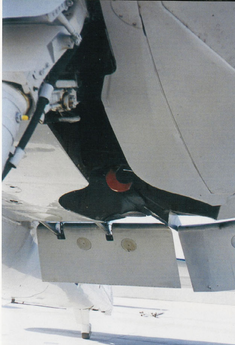
The main landing gear well of the F6F-3. The landing gear rotated ninety degrees to lay flat within the well. Also visible is the fully lowered inboard flap with its two circular inspection plates.
