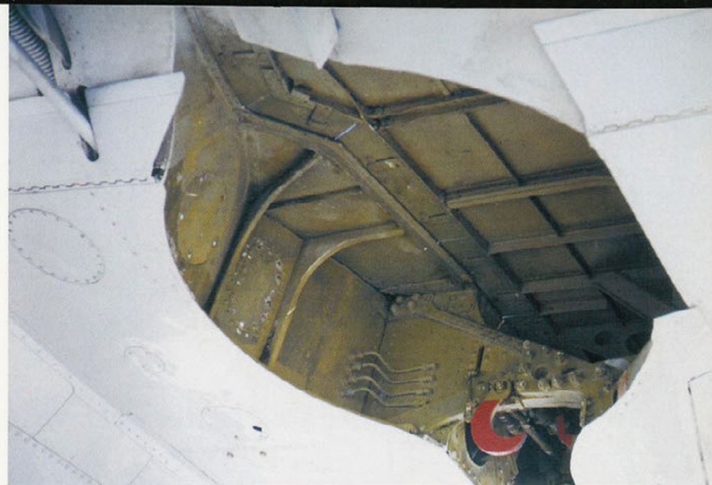
The interior of the starboard wheel well has a number of small hydraulic lines running through the lower corner. The red hook is the landing gear up lock that secured the landing gear into the well. Zinc Chromate Green was a non-standard color for Hellcat wheel wells, normally the well was painted in the same color as the surrounding exterior. (Author)
