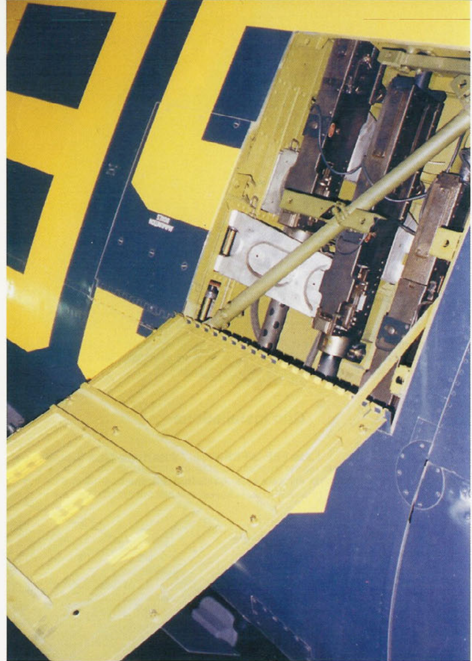
Guns four, five and six are installed in the starboard wing. The ammunition access panels are closed. The diagonal brace in the gun bay is removable, to provide more accessibility to the guns. (Larry Webster)
