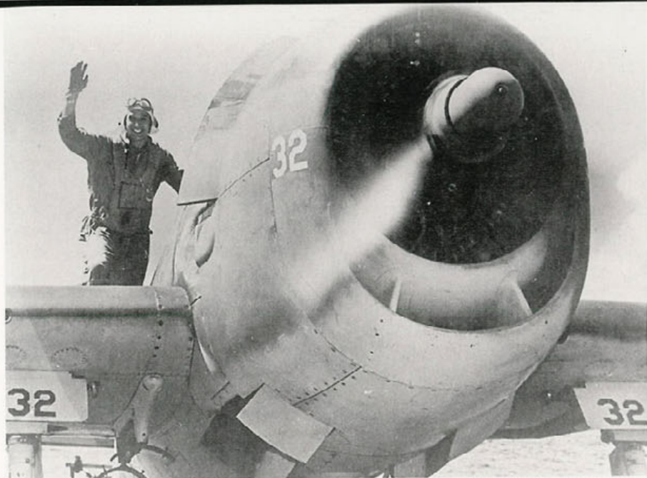
Navy Ace, Lieutenant (Junior Grade) Alex Vraciu on the wing of his F6F-3 of VF-6. The catapult bridle hooks are visible just inboard of the landing gear doors. The cowl flaps and intercooler doors are open and the starboard bomb rack is visible along with its sway braces. LTJG Vraciu finished the war with a total of nineteen kills. (USN via R. M. Hill)
