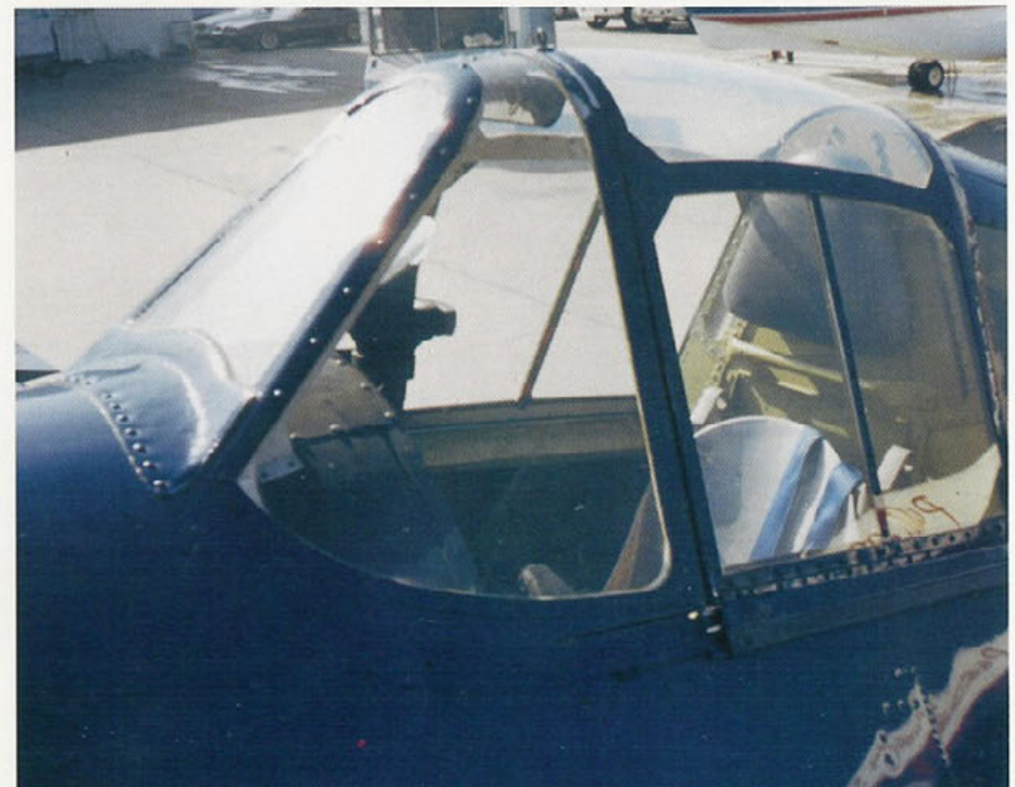
This late style windshield is mounted on a F6F-3, which is highly unusual. Normally, the late style windshield was used on F6F-5s. One of the main visual differences was the deletion of the brace. (Author)
