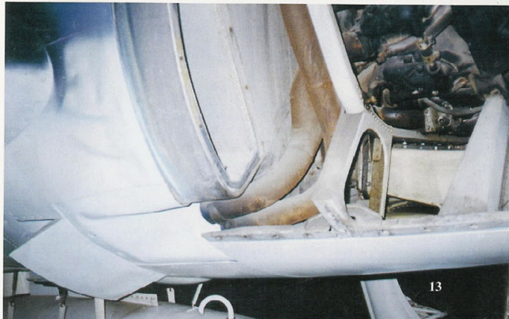
The lower set of exhausts stacks on a F6F-3. The intercooler shutter is directly behind the lower exhaust port. Also visible is part of the oil cooler/supercharger ducting. (Author)
