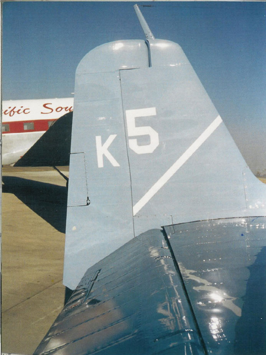
The vertical fin and rudder of F6F-3 BuNo 41930. Construction techniques for the Hellcat were similar to those used on the Wildcat. There were over 12,000 Hellcats built in just three years. Also visible is the elevator trim tab. Service F6F-3s were painted in non-specular (flat) colors. (Author)
