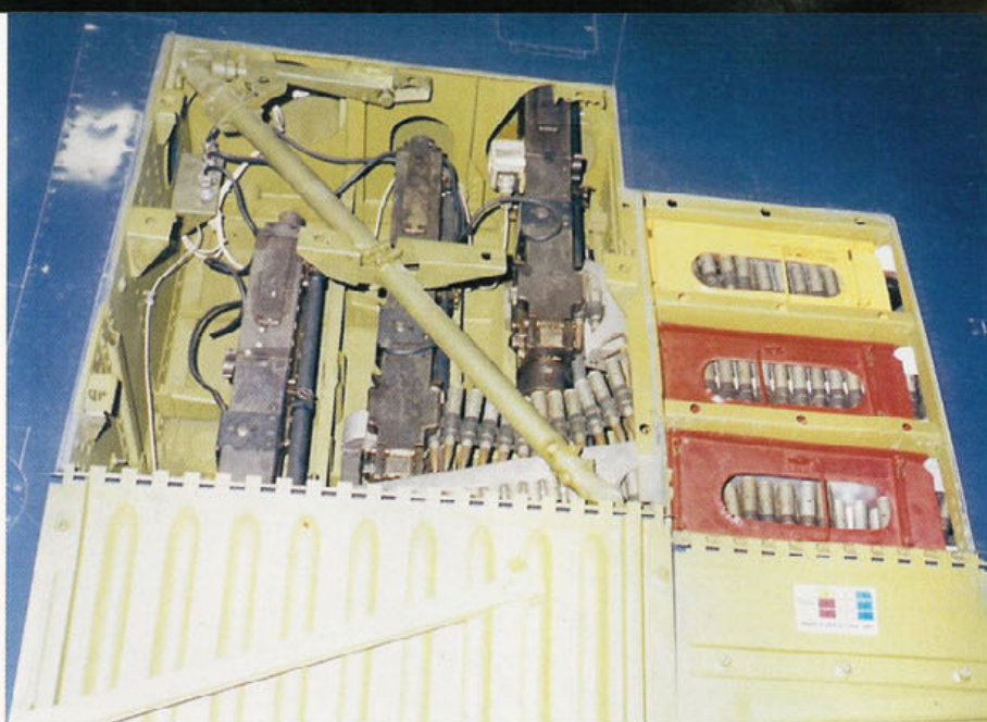
The port gun bay of a F6F-5. The guns are staggered withing the bay to ease ammunition feed problems. The Hellcat could carry a total of 2,400 rounds of .50 caliber ammunition. (Larry Webster)
