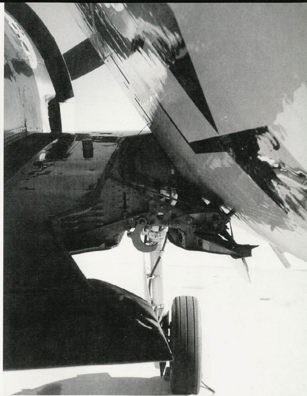
The Inboard landing gear well with the wing in the folded position. The hook in the center is the landing gear up lock, which swings outward and up to lock the landing gear in place in the wheel well when the gear is in the retracted position. (Author)
