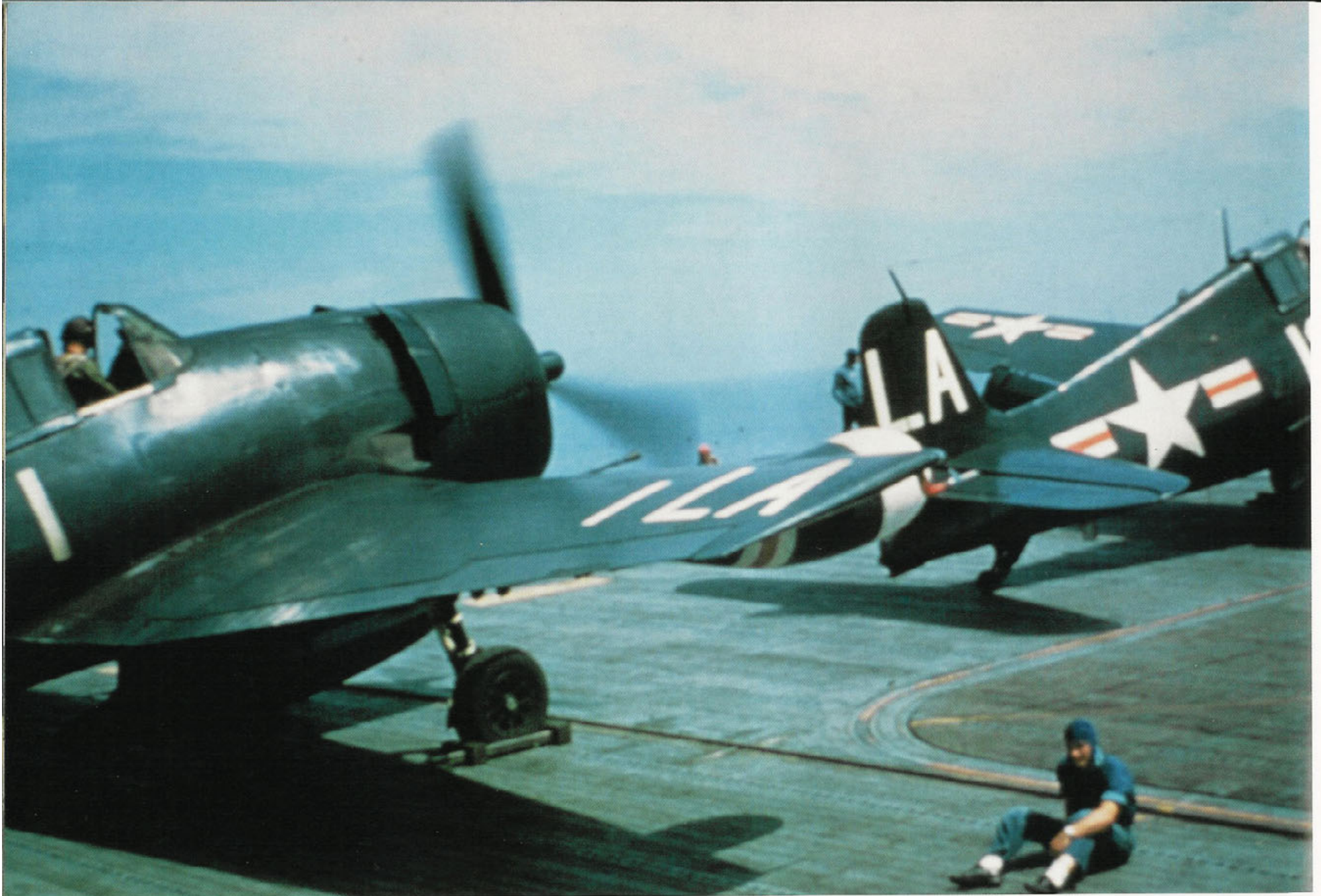
A pair of VCN-2 F6F-5N Hellcats await their launch from an unidentified carrier. The front of the AN/APS-6 radar was painted White. The aircraft in the foreground was armed with the alternate gun armament of two 20MM cannon and four .50 caliber machine guns. The pitot tubes of these aircraft are Gloss Red, the standard delivery color. The main landing gear doors and door attachment brackets are in Insignia White. (Tailhook)
