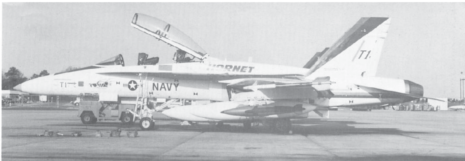
(Above) Bureau Number 160781 was the first two seat Hornet prototype. In addition to testing the two seat configuration, it was used to conduct armament separation tests of the AIM-7 and AIM-9 missiles. (McDonnell Douglas via Norm Taylor)
