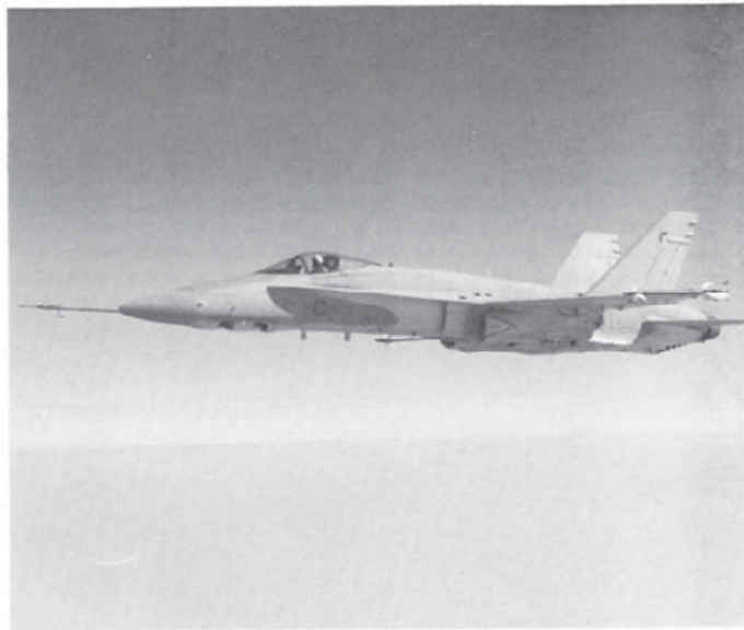
An RF/A-18A reconnaissance aircraft carries a camera pallet in place of the nose mounted cannon. The pallet carries two cameras or one camera and an infrared scanner which are compatible with TARPS, the Navy tactical air reconnaissance pod. (McDonnell Douglas)
