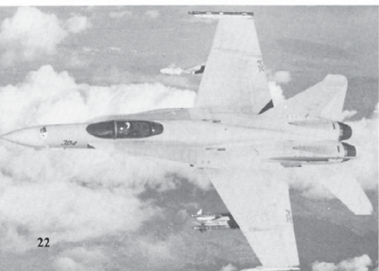
An F/A-18A testing what may become the optimum air-to-air configuration — a pair of Sidewinders on each outboard pylon. These are Blue painted inert missiles, suggesting that this flight was for aerodynamic testing of the paired missile configuration. (McDonnell Douglas)
