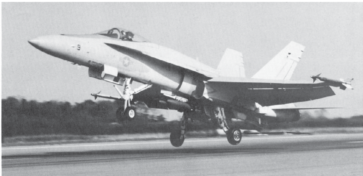
(Above) An F/A-18 takes off with Sparrows, Sidewinders, and a pair of 500 pound Snakeye low drag bombs on the centerline. The Hornet can carry up to 17,000 pounds of ordnance on nine external stations. (McDonnell Douglas)
