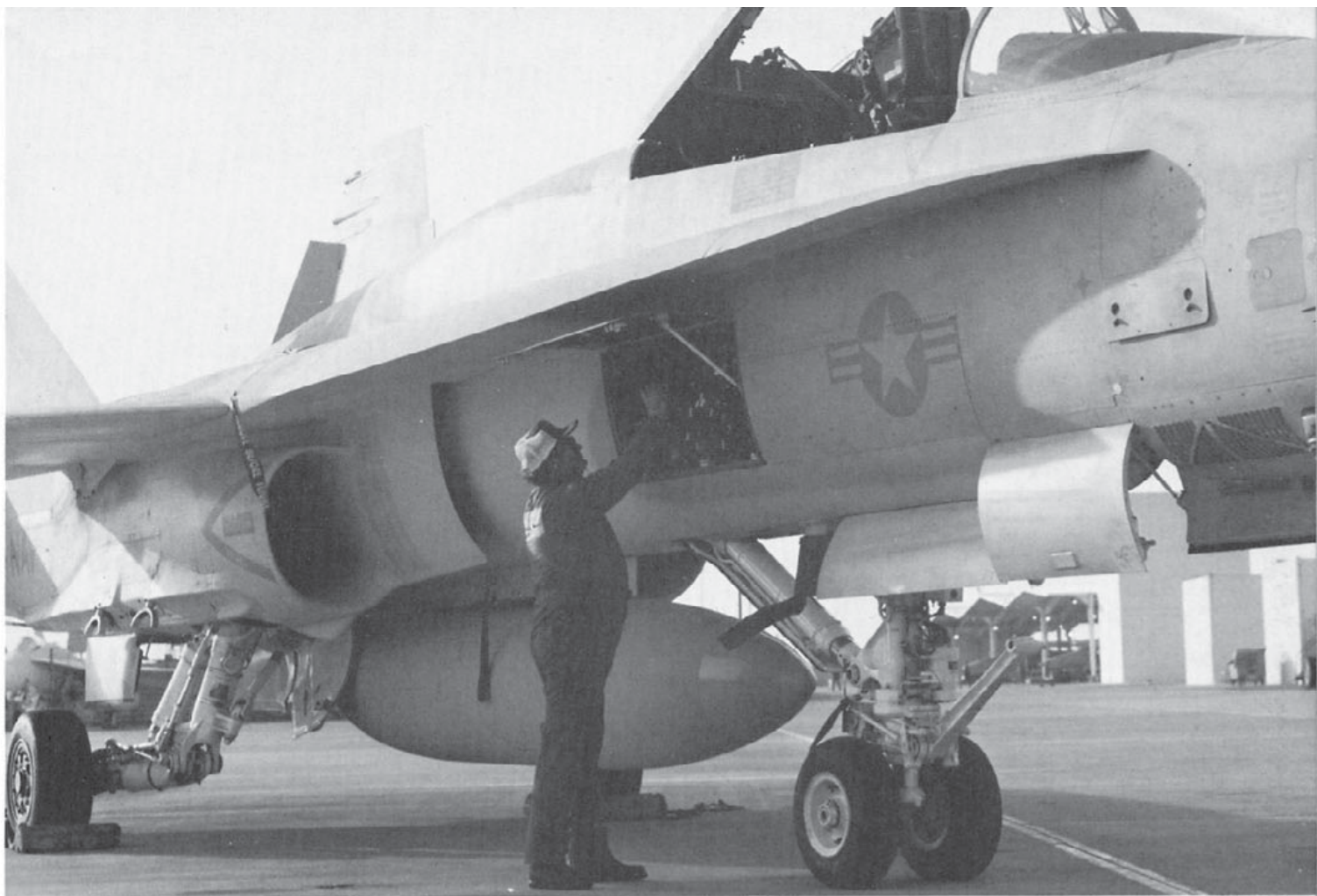
(Above) A McDonnell Douglas Aircraft Company electronics technician installs the AIMES computer in a Hornet on the St. Louis factory ramp. Ease of access is one of the keys to the maintainability of the Hornet, which gives the F/A-18 the best maintenance man hour/flight hour ratio of any modern fighter. (McDonnell Douglas)
