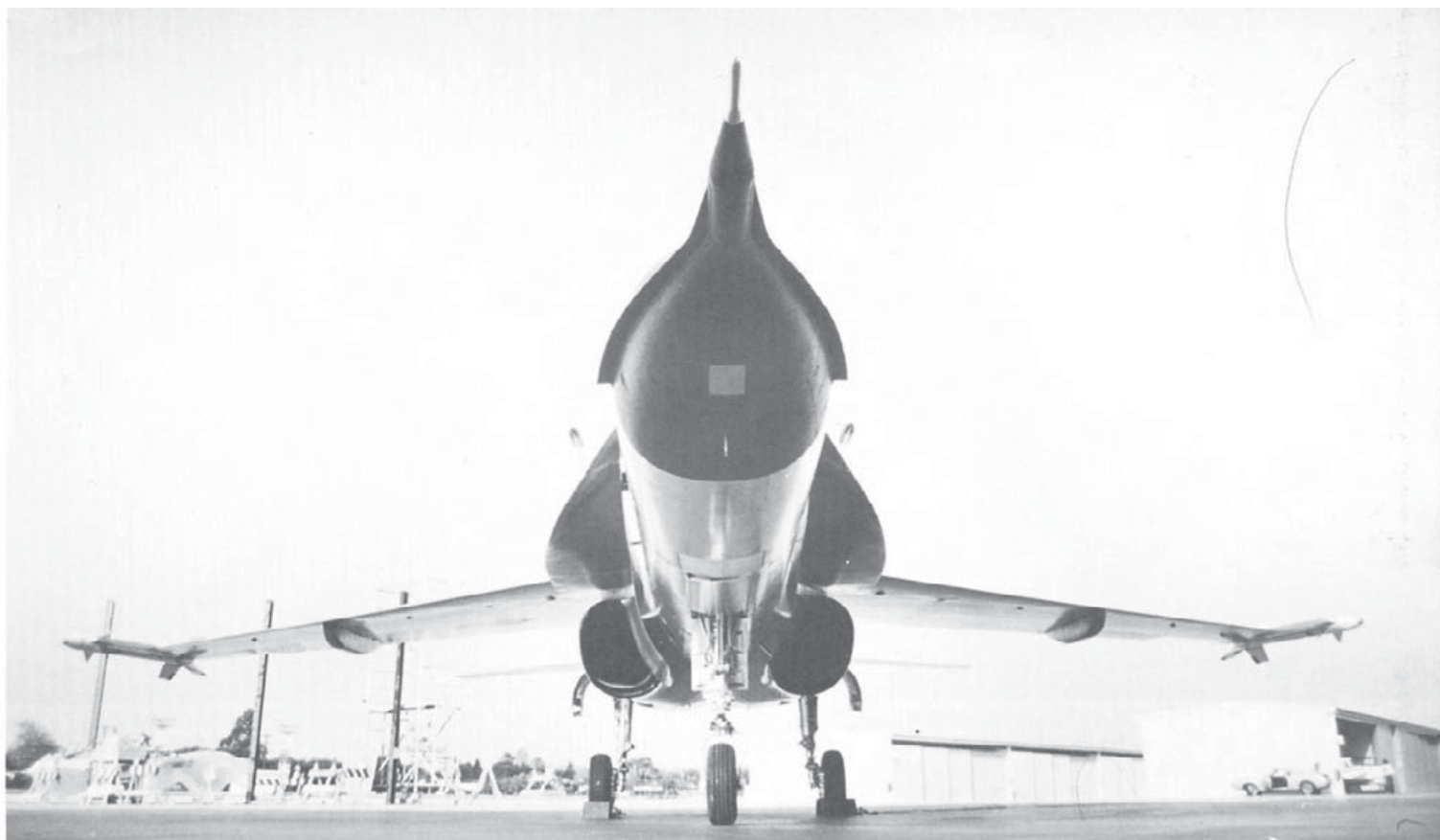
(Above) Head on the slim YF-17 reveals its simple light land based type landing gear, strakes on the sides of the nose, slots in the leading edge extensions, and lack of underwing pylons. (Northrop)
