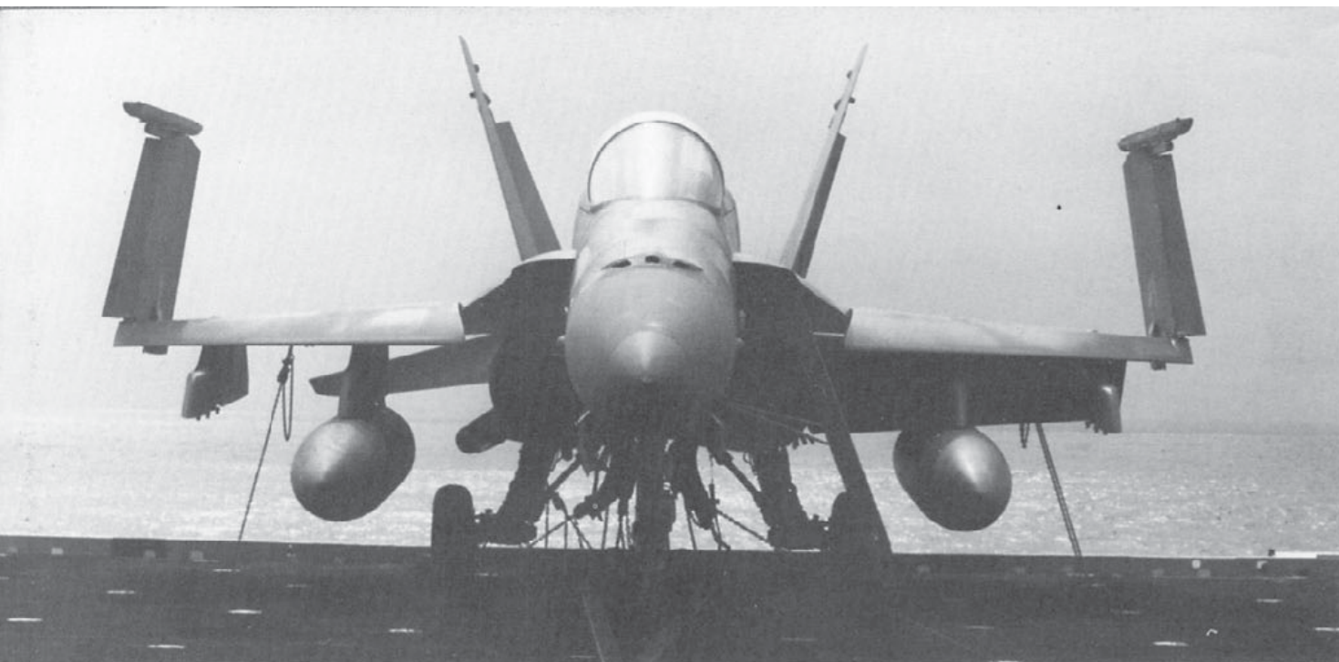
An F-18A Hornet chained down aboard ship with the wings in the folded position. The small port in the center of the nose behind the radome is the gun port for the M-61 Vulcan 20mm six barrel rotary cannon. (McDonnell Douglas)
