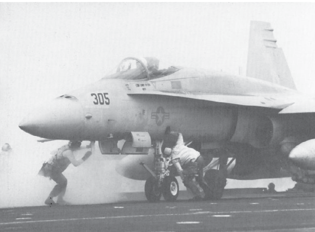
(Left) The catapult crew does a pre-flight check on an F/A-18 prior to hooking it up to the steam catapult. The Hornet, like other modern carrier aircraft, has a simplified attachment system consisting of a launch bar (in front of the nose gear) and a deck crew installed hold back. (McDonnell Douglas)
