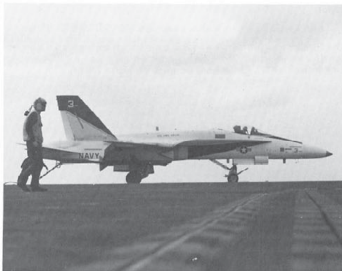
The number four Hornet (BuNo 160778) was used to test the structural integrity of the design, pulling up to 11.25 Gs during one symmetrical pull out and 9 Gs in a rolling pull out. (McDonnell Douglas)
