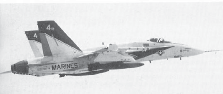
The Number four prototype armed with four Mk 84 low drag bombs. The Hornet can deliver conventional ordnance with almost three times the accuracy of the A-7 Corsair II. (McDonnell Douglas)
