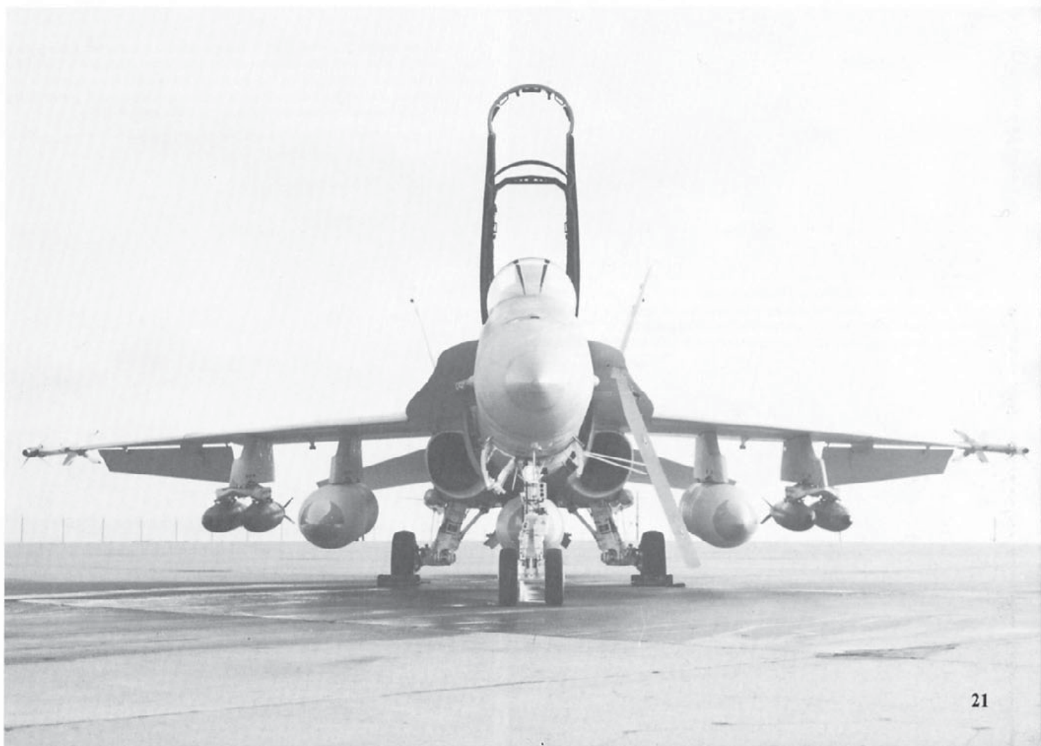
(Below) The F/A-18's heavy beefed-up carrier landing gear is one of the principal differences between the Hornet and the earlier YF-17 lightweight fighter. The internal boarding ladder folds into the bottom of the port leading edge extension. (McDonnell Douglas)
