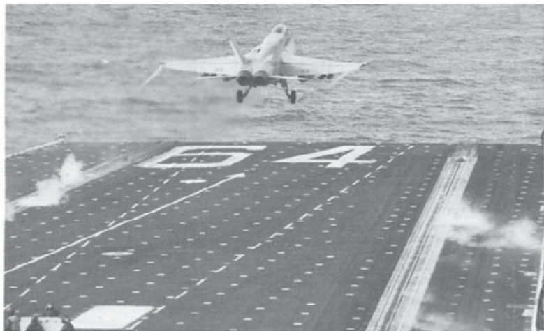
An F/A-18 of VX-5 launches from the port catapult with the rudders tied-in. Project pilots of VX-5 were responsible for two weapons programs each during the tests conducted for the Operational Test and Evaluation (OPEVAL) program. (McDonnell Douglas)
