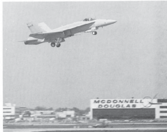
The first F/A-18C takes off from the McDonnell factory in September of 1987, with company test pilot Glen Larson at the controls. The F/A-18C has a faster, higher capacity computer, new radar jammer, and is capable of carrying the advanced medium range AAM (AMRAAM) and infrared Maverick. (McDonnell Douglas)
