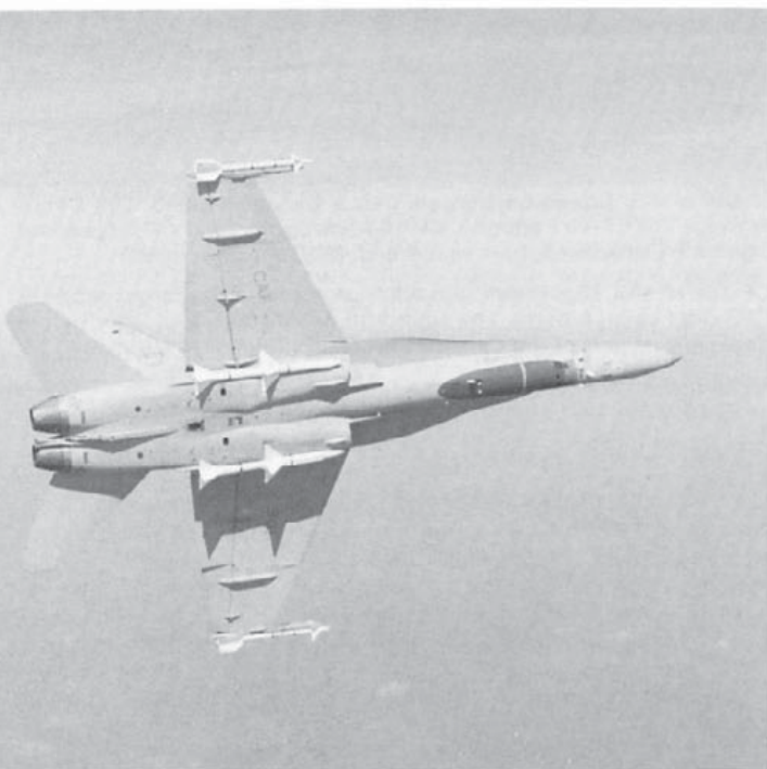
(Above) CF-18A (serial 188106) reveals the false canopy painted on the undersides of all Canadian Hornets. In a turning fight, the false canopy might convince an enemy pilot that the Hornet is turning into him when it is actually turning away. (via Norm Taylor)
