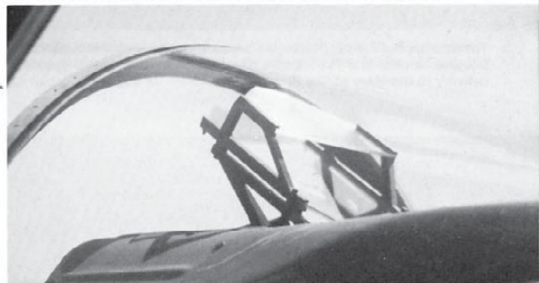
The canopy opening actuator rod is located behind the pilot's ejection seat. The 'V' shaped assembly on the canopy rail is the canopy locking lug. (Dave Mason)
