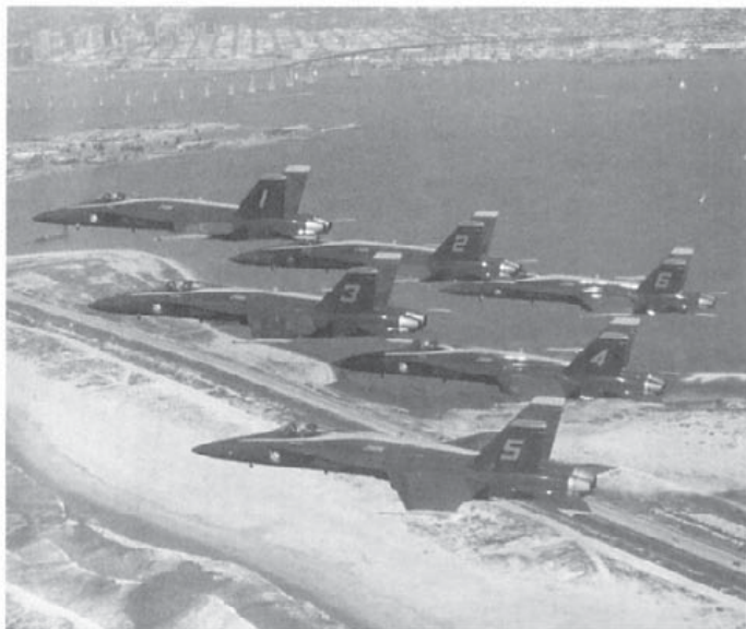
The Blue Angels fly over the Silver Strand near NAS North Island, San Diego. The Blue Angels' Hornets are modified with a smoke generating system and a new seat harness to keep the pilot in place during negative G maneuvers. (McDonnell Douglas)
