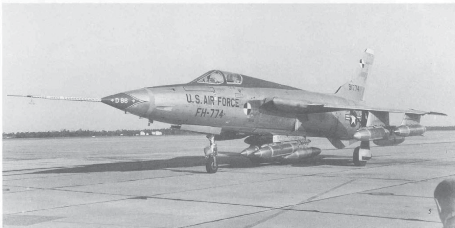
(Below) F-105D-6-RE loaded with napalm (BLU-1B) for drop tests. The Black and White segmented circles on fuselage and tail are to aid in photo interpretation. (Republic)
