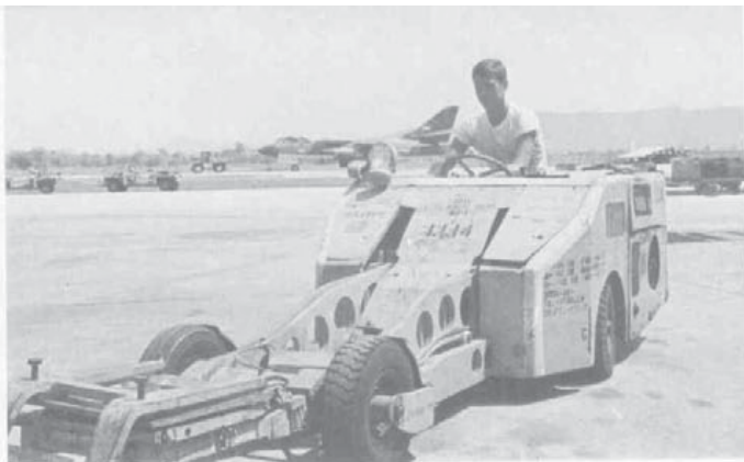
(Above) The MJ-1 bomb loader was the primary vehicle for up-loading and down-loading stores on the Thud. (John Coon)
