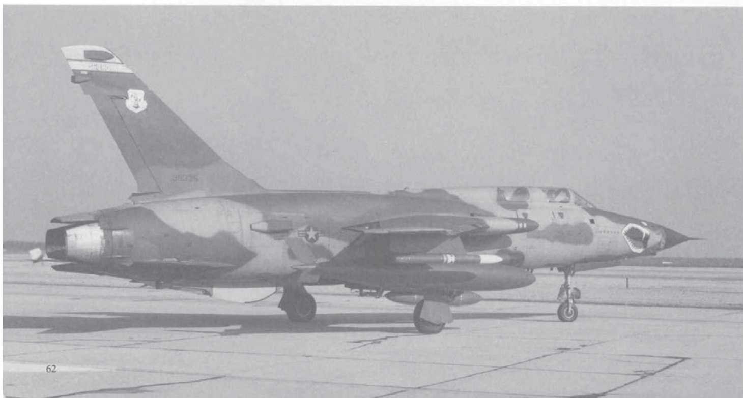
(Below) F-105G of the 128th TFS, Georgia ANG, taxis at Shaw AFB, SC on 11 February 1982. It features wrap-around camouflage, and is carrying a captive Shrike, 450 gallon tanks, and a traveling pod is on the centerline. (Norman E Taylor)
