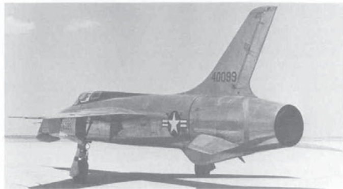
(Above) The second of two YF-105A prototypes which flew with the Pratt & Whitney J-57-P-25 engine. This was the only Thunderchief to fly with a non-segmented exhaust. Edwards AFB, 25 May 1956. (Republic)
