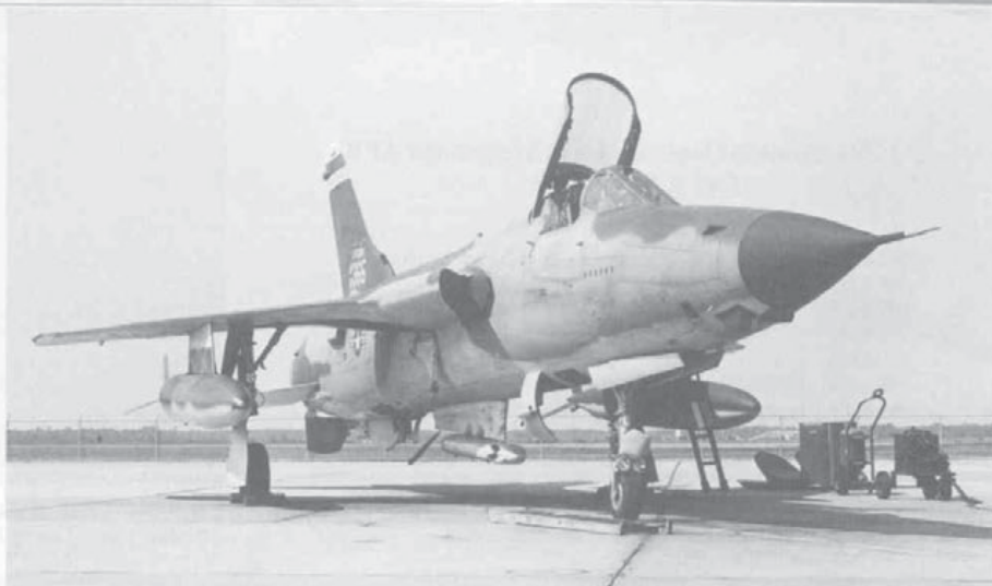
(Right) F-105D-31-RE belonging to the 149th TFS, of the Virginia Air National Guard at Byrd Field, Sandston, VA on 27 April 1976. It carries an SUU-20 practice bomb dispenser on the centerline. (Jim Sullivan)
