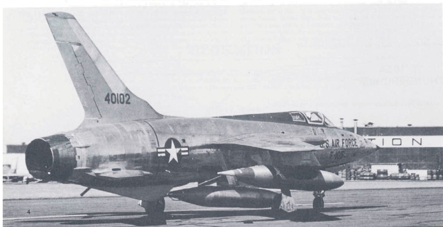
(Below) The third F-105B taxis out for takeoff at Farmingdale. Early B models featured small windows behind the canopy. (Republic)
