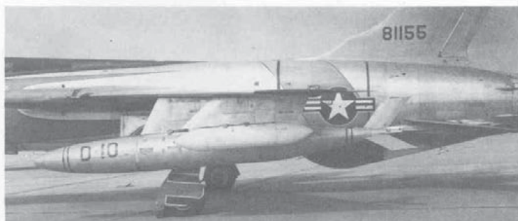
(Below) F-105D-6-RE loaded with napalm (BLU-1B) for drop tests. The Black and White segmented circles on fuselage and tail are to aid in photo interpretation. (Republic)
