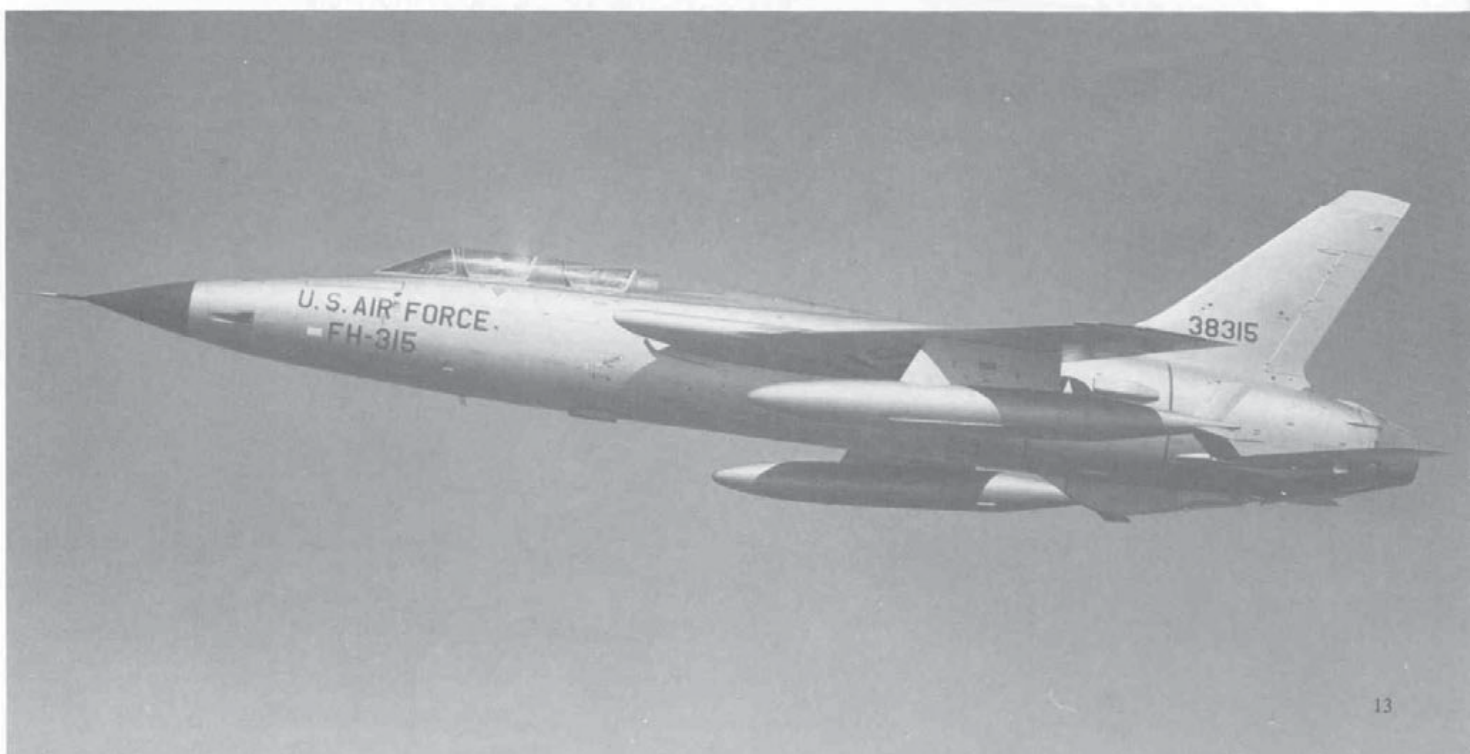
(Below) F-105F fresh from an Inspect and Repair as Necessary (IRAN) overhaul in 1964, with its last coat of Silver paint (the following year all F-105s began to come out of IRAN with camouflage). Afterburner cooling scoops have been added to the rear fuselage. (Republic)
