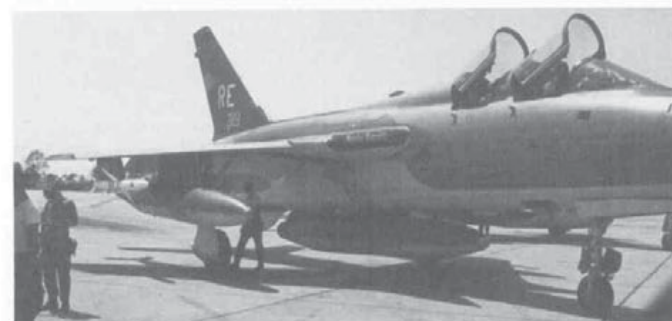
(Above) 'Sinister Vampire' of the 44th TFS Vampires, an F-105F loaded for a Wild Weasel mission with Shrike Anti-radiation missile. (John Coon)
