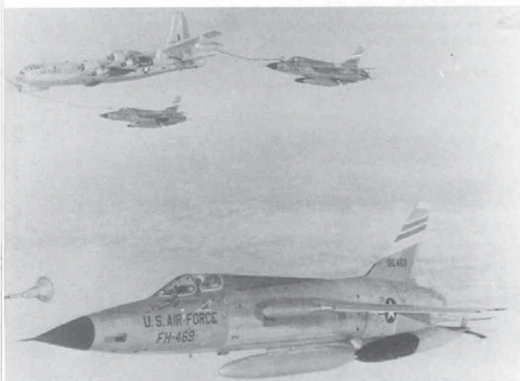
(Above) F-105Ds of the 36th TFW refuel from a KB-50 tanker. The relative angle of attack of the tanker and the fighters tells all! The tanker is going downhill in order to maintain enough airspeed to keep the Thuds from falling off the hose. (Republic)
