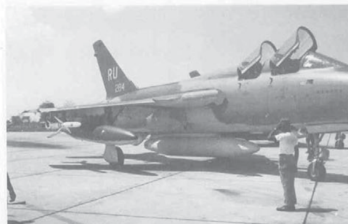
(Below) 'The Glenna B.' of the 357th TFS carries a 650 gallon tank on the centerline, a 450 gallon on the inboard pylon and a Shrike missile on the outboard pylon. (John Coon)
