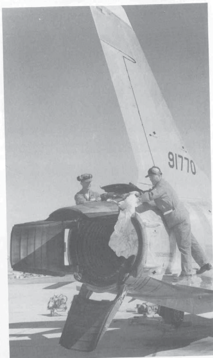
(Below Left and Below) Two views of the drag chute installation on the F-105D. The aircraft on the right is a D-6-RE which does not have the arresting hook that would be installed on later models. (Republic)
