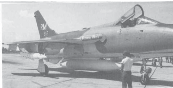
(Above) 'Running Gun V' of the 333rd TFS loaded with AGM-12 Bullpup on the port wing and a 650 gallon centerline tank. (John Coon)
