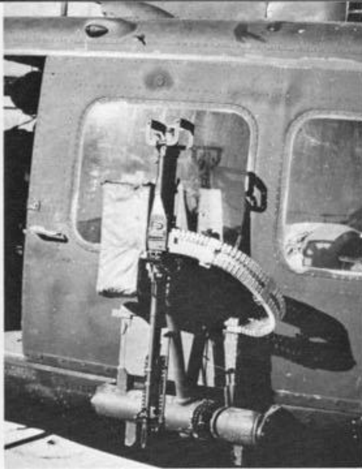
Stock M-60 mount, including feed chute and ejection control bag. (Wallace Van Winkle)
