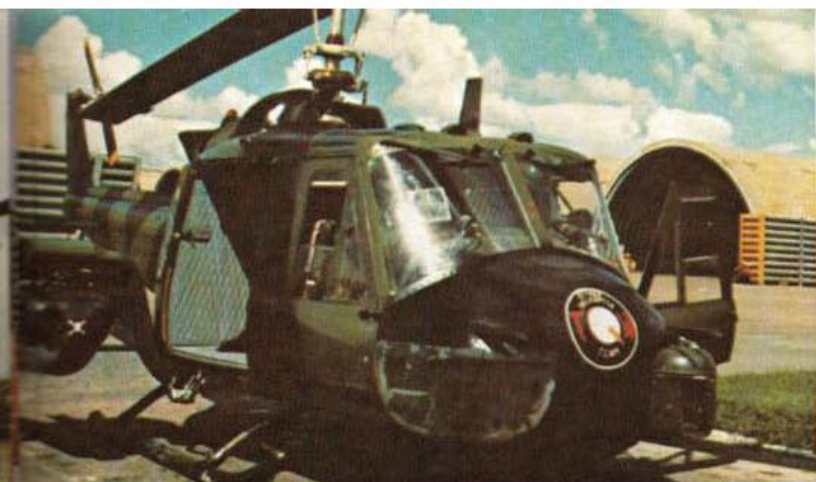
TOW equipped UH-1Bs carried TOW emblem on nose, with the words "Whispering Death" in Red barely visible under the word "Team". They were fitted with heat masking exhaust devices. Seen loading
