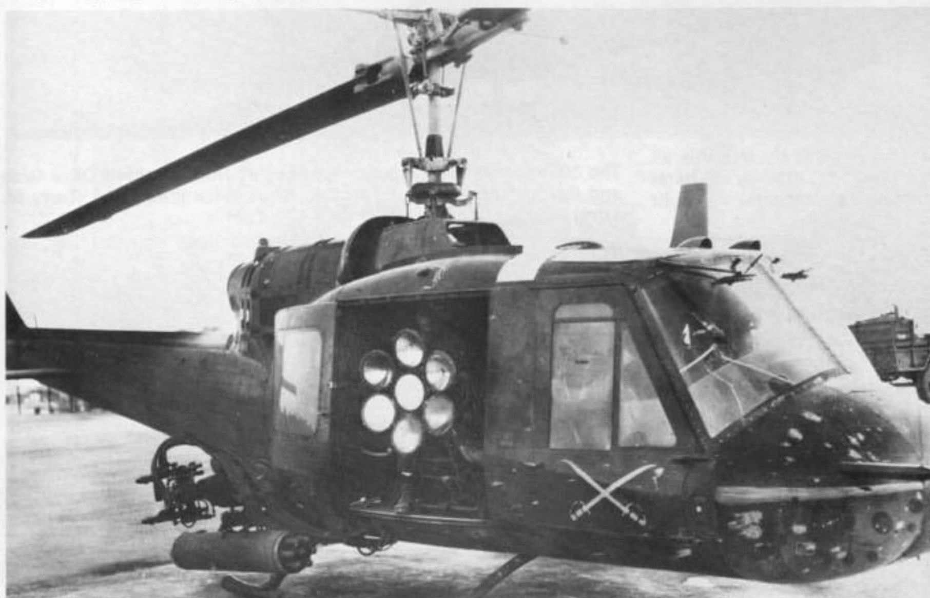
UH-1B of the 13th Aviation Battalion at Soc Trang during 1966 with "Lightning Bug" searchlight modification. (Bell)
