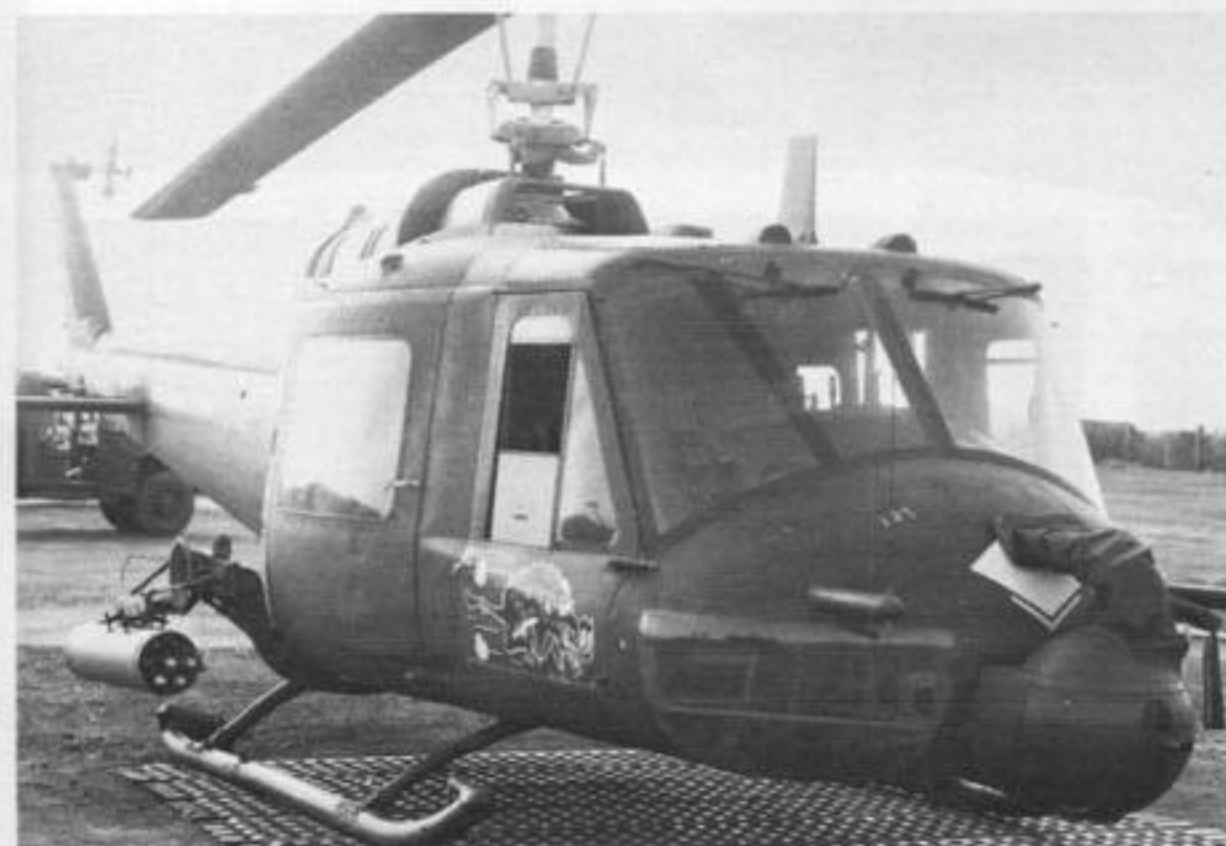
UH-1B of the 120th AHC "Razorbacks" armed with XM-5 and XM-157 systems, at Tan Son Nhut, 28 March 1966. (U.S. Army via Mutza)
