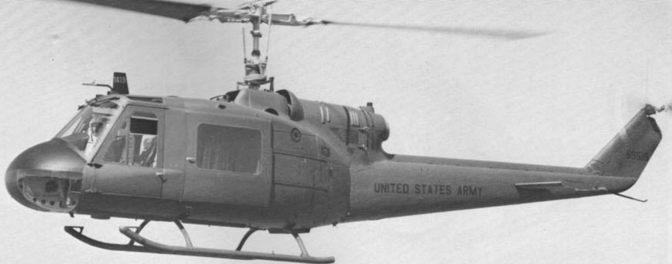
Factory fresh UH-1C on its acceptance flight showing the larger vertical tail surfaces that mark the major difference between the B & C models. (Bell)
