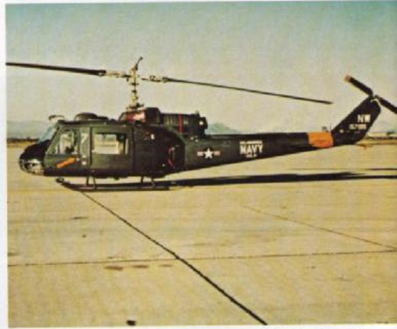
HH-1K is the Navy version of the UH-1E, with T-53-L-13 engine, at Davis Monthan AFB, 1981. (Wallace Van Winkle)
