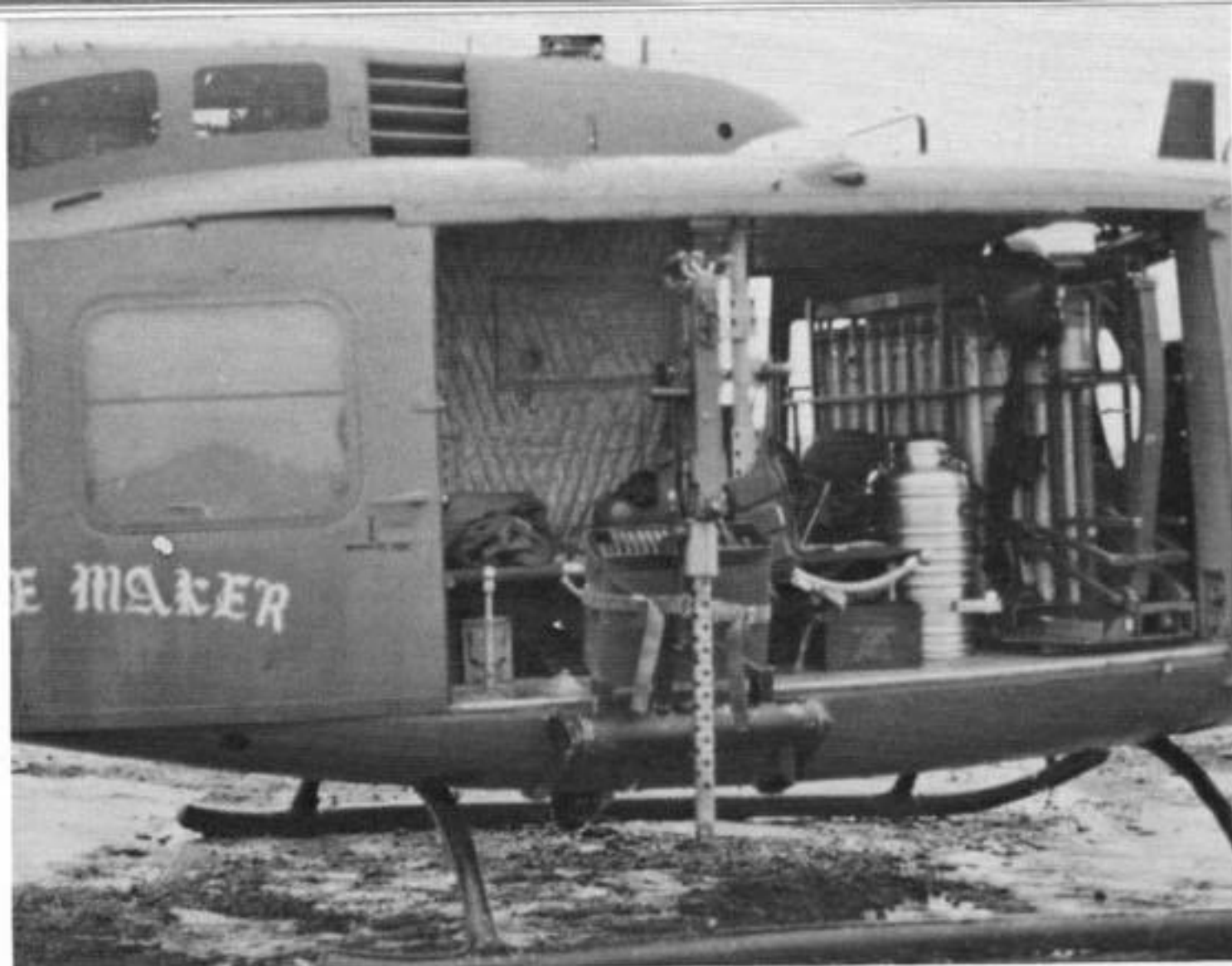
"Peacemaker" was the chase ship of 3/4 Cav, which retrieved shot-down aircrew. It was armed with .50 caliber machine gun, twin M-60s, "free 60s", MK-24 flare dispenser, crash bags, spare Cobra gun pod, litter, extra ammo, and a Medic. Cu Chi, RVN. (Wayne Mutza)
