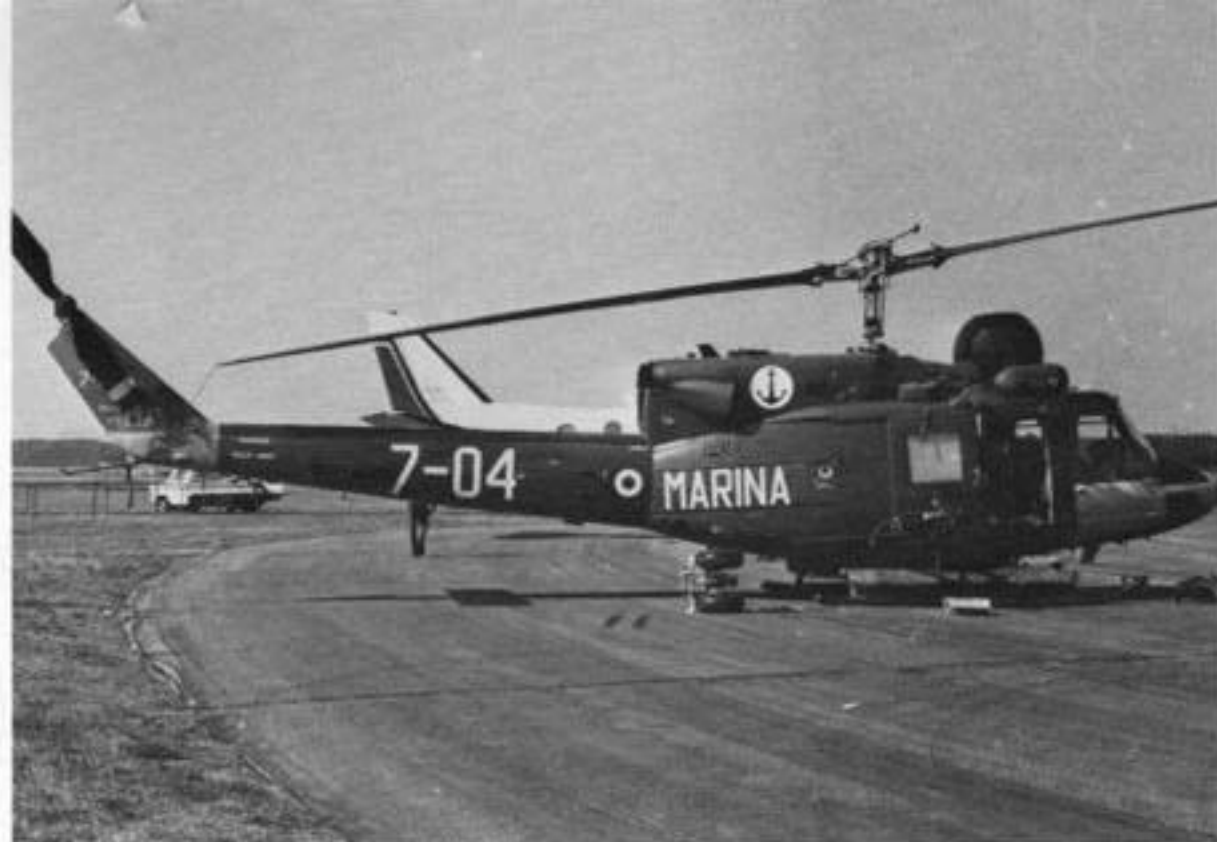
(Above, Below Left and Below) The AB-212ASW first entered service in 1976, with 5 Gruppo Elicotteri, based at Luni. It is the same basic aircraft as the 212, with modifications made for the ASW role, including all-weather capability in the anti-submarine role. It is operated by the navies of several countries. Illustrated are AB-212ASW aircraft of the Italian and Spanish navies. (Michel C. Klaver and Salvador Mafe Huertas.)
