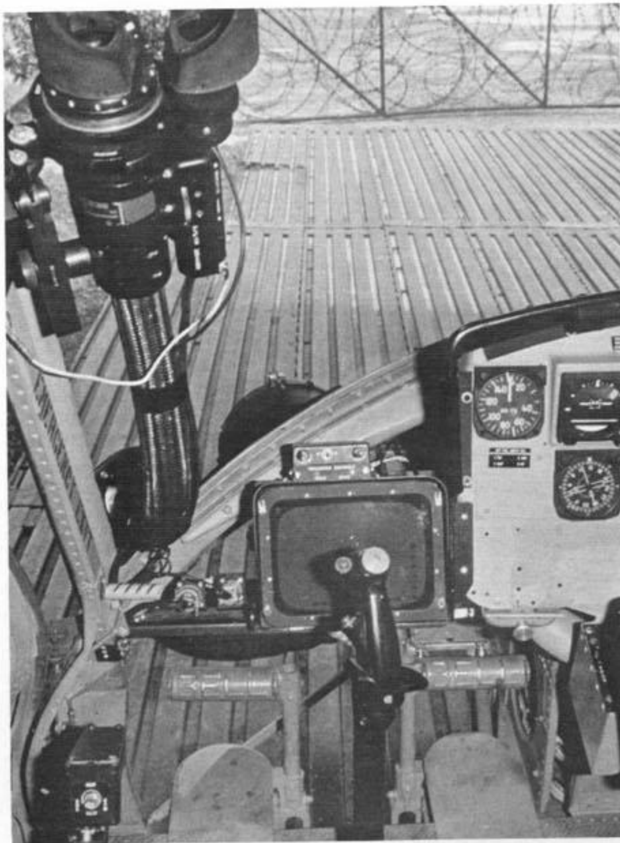
Gunner/Copilot position in the INFANT equipped UH-1M of the 11th Aviation Group. Camera monitor is the large screen on the left of the panel, with the flexible sight for the miniguns in the stowed position at upper left. (U.S. Army)
