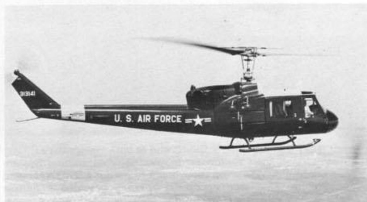
The UH-1F was developed for USAF, using the General Electric T-58 engine, which required a revised exhaust position. The Fs tail boom is also two feet longer than other Hueys as a result of inclusion of a baggage compartment. (Bell)
