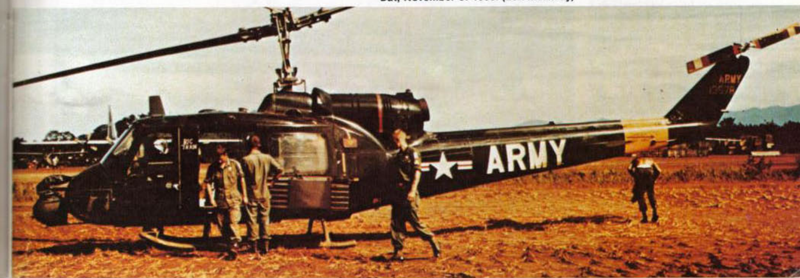
"Big Train" a UH-1B gunship with the M-5 grenade launcher in the nose and M-3 48 shot rocket packs which made it a "Huey Hog" at Vo Dat, November of 1965. (Lex McAulay)
