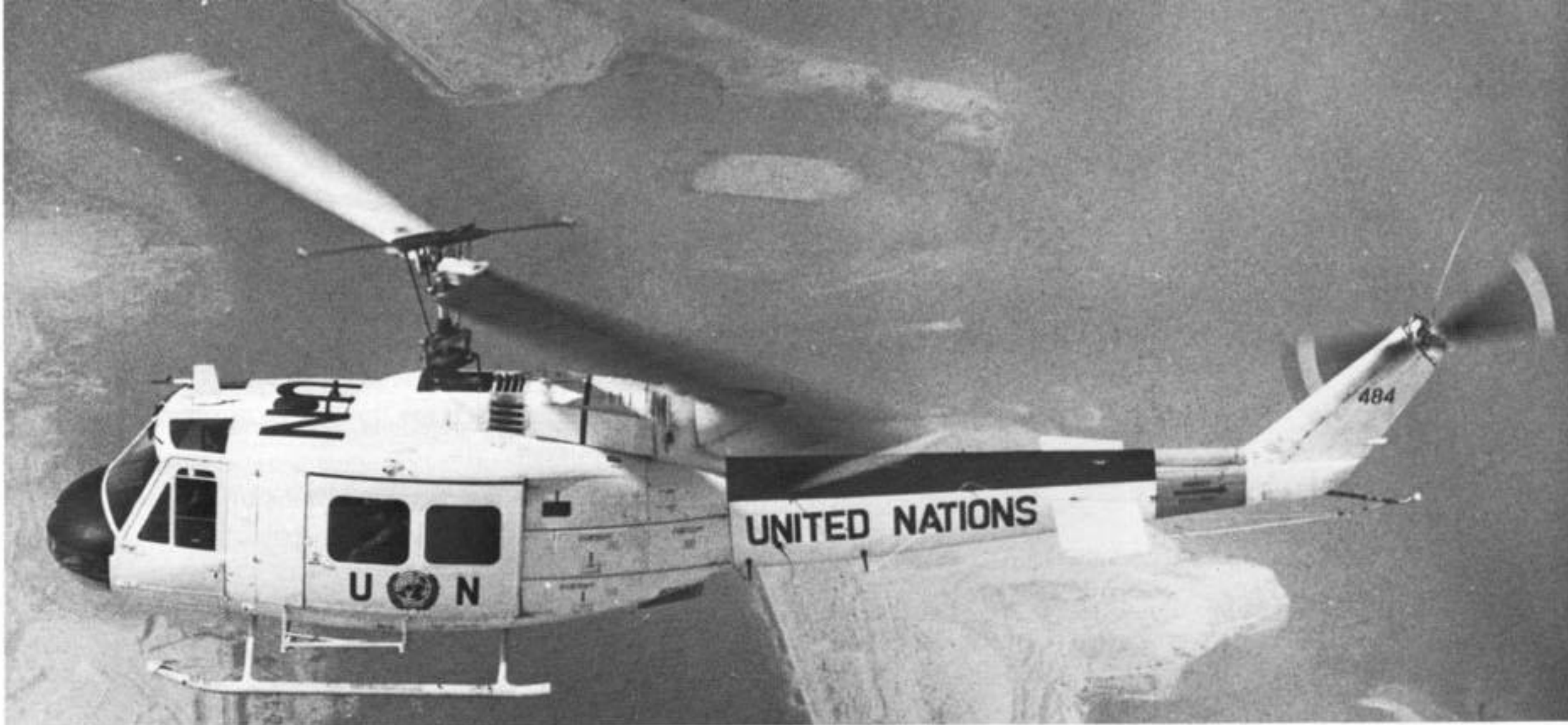
The United Nations operated the UH-1H in its peacekeeping mission in the Mid-East. The dangers inherent in that mission are indicated by the installation of the exhaust shield kit fitted to guard against heat-seeking missiles. (Bell)
