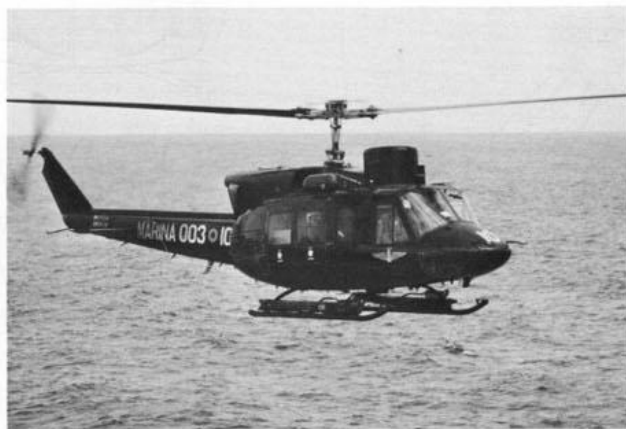
(Above, Below Left and Below) The AB-212ASW first entered service in 1976, with 5 Gruppo Elicotteri, based at Luni. It is the same basic aircraft as the 212, with modifications made for the ASW role, including all-weather capability in the anti-submarine role. It is operated by the navies of several countries. Illustrated are AB-212ASW aircraft of the Italian and Spanish navies. (Michel C. Klaver and Salvador Mafe Huertas.)
