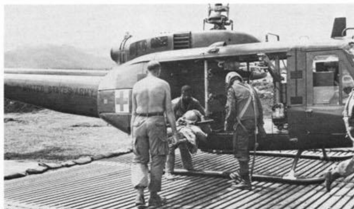
UH-1H of the 101st Airborne Division configured for the "Dustoff" mission with litters and internal hoist. The Crew Chiefs "Chicken Plate" (body armor) and "Monkey Strap" (restraint harness) are clearly visible. (Wayne Mutza)
