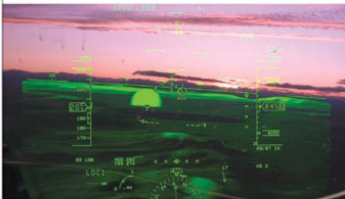
Rockwell Collins's SVGS on the head-up display reveals the airport under a virtual dome, with an extended runway centerline marker, runway border highlights and terrain.
