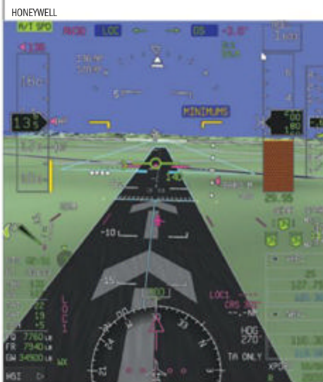
This screen shot from a Honeywell flight test shows the SVGS view on the primary flight display of the landing environment just below the proposed 150-ft. decision height.
