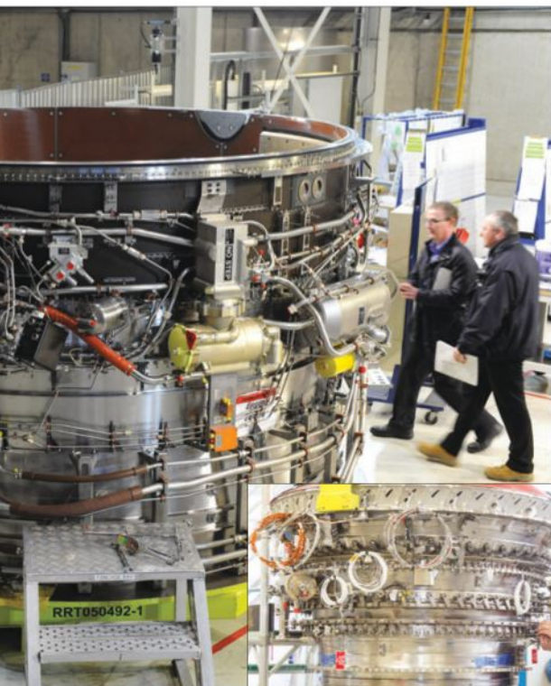
Fan case (left) and core (below) for first flight-test XWB-97 come together in Derby, England.
