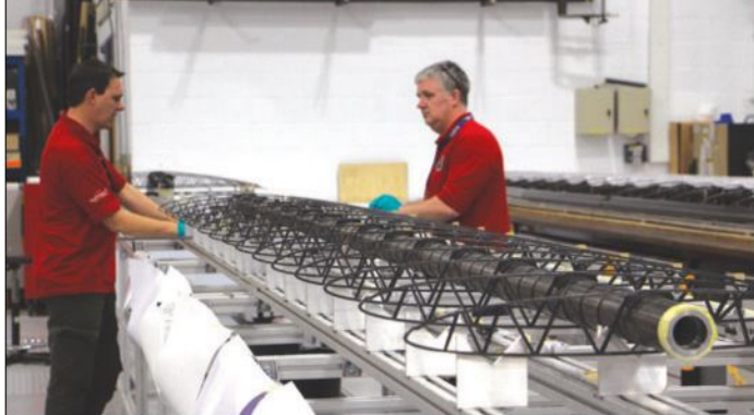
Airbus Defense and Space technicians build a wing section of the Zephyr 8 aircraft.
