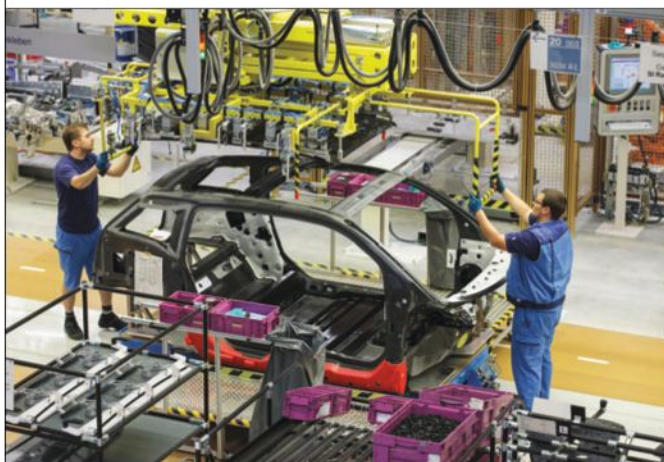
BMW's i3 electric car has a carbon-fiber passenger cell.
