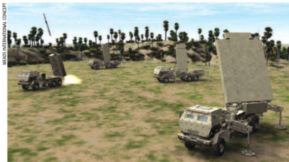
The Meads system was designed to provide 360-deg. radar coverage in the X- and UHF-bands.
